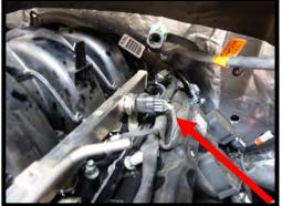
24. Using a 3/8" fuel line removal tool, remove the feed line from the factory port injection system to the direct injection mechanical pump. Slide removal tool between the lines, securing the DI side until it releases. NOTE: THIS FUEL LINE HAS A CHECK VALVE, DO NOT FLIP ORIENTATION. DO NOT REMOVE FROM DI PUMP TO ELIMINATE CONFUSION. 90-DEG END ALWAYS CONNECTS TO FUEL FEED SUPPLY!
