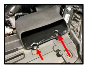
99. Install the supplied panel filter to the airbox lower. Install the upper airbox to the top of the filter. Secure the top to bottom using the supplied (6) 6mm x 16mm BHCS. Torque to 50 in-lbs. \*Caution: Over torqueing can result in pulling an insert out of plastic box.
