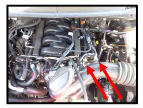
13. Remove the driver side valve cover PCV line quick connect fittings from the inlet tube by squeezing the connector and pulling away. Remove from valve cover by squeezing the connector and pulling away.
