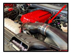
102. (Stock throttle body installations) Install the supplied 5" ID x 2 1/4" silicone hose over air inlet tube and airbox lid. Install the supplied reducer silicone hose over air inlet tube and stock throttle body. Connect the other end to the stock throttle body. Secure all ends with the supplied hose clamps (2) #80, (1) #64 and (1) #56 on throttle body.
