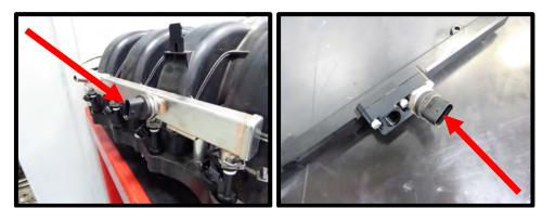
42. Install the supplied (1) #2-906 Viton oring to the (1 of 2) 45mm long 9.49mm inlet fitting. Apply light amount of grease to oring for ease of installation. Install fitting to the fuel inlet block.
