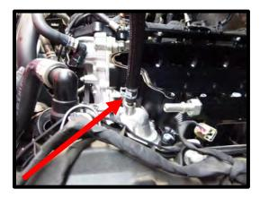
71. Connect the factory heater hose quick connect to factory heater tube (bank 1).
