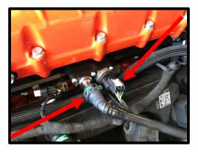
65. Slide the EECPV to previously installed bracket. Connect factory plastic quick connect fitting to EECPV until it clicks and locks into place. Connect 2-way electrical connector to EECPV, press locking tab back in place.
