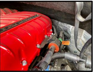
63. Connect the factory passenger side rail fitting to the DI pump factory hose, press until it clicks and locks in place.
