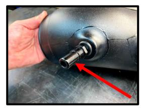
101. (Whipple 132mm Crusher throttle body) Install the supplied 5" ID x 2 1/4" silicone hose over air inlet tube and airbox lid. Install the 4 3/4" x 3" silicone hose over throttle body. Install the air inlet tube between the filter and throttle body. Slide silicone hose over throttle body. Secure all ends with the supplied (4) #80 hose clamps.
