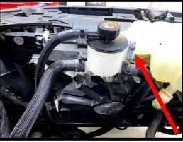
97. Install the ¾" ID rubber hose (#18F150-HS006) from the Bank 2 (OUTLET) IC fitting to the IC filler neck. Secure both ends with supplied pinch clamps. NOTE: NEVER SWITCH THE INTERCOOLER ROUTING, BANK 2 IS ALWAYS THE OUTLET!
