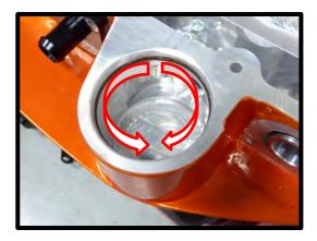
62. Apply generous amount of grease to the (1) #2-230 Viton bypass oring. Install the supercharger lid to the supercharger housing by carefully placing the bypass down. Secure the SC lid using the (17) 6mm x 30mm HHFCS and (3) 6mm x 70mm HHFCS (*marked green*) using the following pattern. Slide the EECPV bracket under bolts 3 and 5 from image (bank 2). Torque to 90 lbs-in using an 8mm socket.
