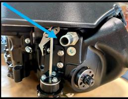
51. Using the supplied 5/16" OD silicone tube, install the (1) 80 1/2" cord. Start as shown with green arrow, go in a clockwise motion, to the front, then around the perimeter. End at yellow arrow position. Bunch it up so it has no gap at the end as any gap will be an air leak of un-intercooled air. Install the (1) 6.5" cord in the front section shown with the blue arrow.
