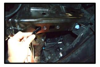
87. Install the IC reservoir to the (2) nut plates using the (4) 8mm x 25mm flanged hex headed bolt. Start (1) on each side to align holes to bushing. If off, you can use screwdriver to align the nut plate and bushing before installing the final (2) bolts. Torque to 15 lb-ft using a 13mm socket.
