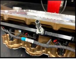
44. Install the supplied (2) #2-906 orings to the (2) inlet/outlet fittings. Install these (2) fittings into rear side of fuel rails. Apply light amount of grease to oring for ease of installation. Using a ¾" wrench (or ¾" deep socket) on both the front and rear fittings, tighten both.
