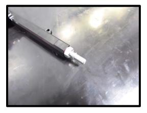
45. Install the supplied (1 per injector port) .515" injector shims to be installed to the injector port of the SC housing, to hold the injector up to its proper position. Install the fuel injectors to the fuel rail, apply generous amount of grease to oring for easy installation.
