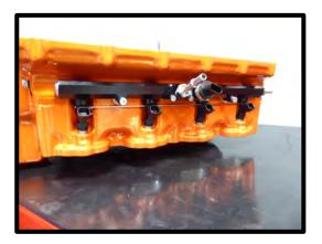
48. Install the supplied 3/8" fuel cross over line around the back of the supercharger by pressing until they click and lock in place.
