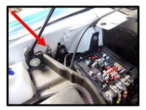
107. Pull the red 10amp fuse from position **#F17** (ABS). Install the 10amp red fuse in the unused fuse slot on the fuse tap. Install the supplied fuse tap into position **#F17** (ABS). **Note:** 10amp red fuse should be in bottom slot, 5amp should be in top slot. Make sure wire has enough room when fuse cover closes, route around fuses for clean installation.
