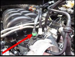
18. Remove the second brake booster quick connect line from intake manifold by squeezing locking tab and pulling away.
