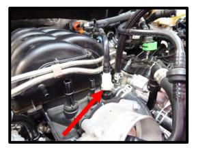
19. Remove the brake booster vacuum line from check valve and IMRC vacuum lines from brake booster line (separate where the arrow points). The check valve closest to the brake booster connector will be utilized.
