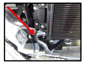
89. Connect the ¾" ID molded/formed (33") hose (#18F150-HS009A) from the LTR driver side bottom fitting that you previously installed, to the IC pump outlet barb. Secure with supplied pinch clamp. **NOTE: Ensure that this hose cannot kink or rub anything overtime.**
