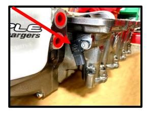
54. Install the supplied (8) manifold orings into the Whipple intake manifold.
