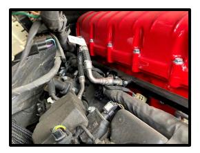
64. Connect the factory fuel inlet line to the driver side fuel fitting, press until it clicks and locks in place. Connect factory fuel psi sensor connector to sensor, press safety lock until it clicks into place.
