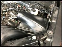
100. Install the (1) supplied 13/16" to ½" rubber grommet into the supercharger inlet tube. Install the supplied ½" to 15.82mm quick connect fitting.
