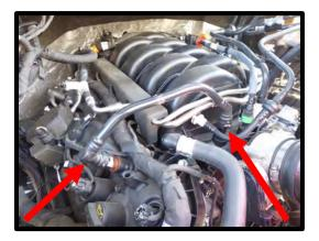
14. Unclip the airbox lid by flipping the (2) tabs to release. Using a 5/16" nut driver, loosen the factory hose clamp securing the air inlet tube to the air box lid and throttle body. Remove airbox lid from engine. Remove air filter from airbox.
