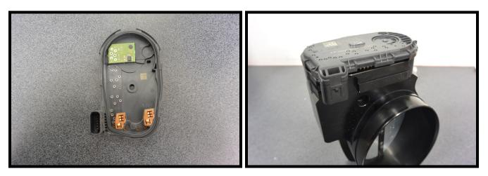
7. Reuse the (6) throttle body cover tabs by pressing on until they click and lock in place.
