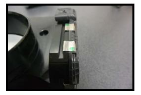
2. Remove the factory cover from the throttle body.
