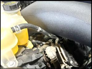
12. Reconnect crank case ventilation hose to air tube fitting previously installed.
