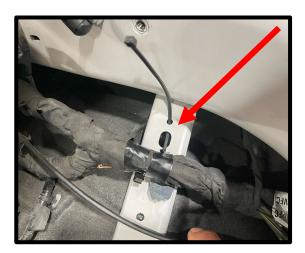
9. Install the supplied airbox into factory (2x) hole locations. Using the supplied (2x) 1.1" L x .30" W plastic push pins, secure front of snorkel to factory location.
