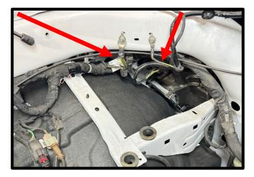
5. Remove wiring loom plastic retainer from vehicle to relax the wiring harness.
