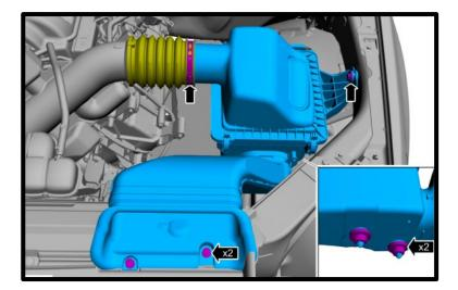
4. Lightly bend the (2x) ground wire so it goes below the frame. **NOTE:** Failure to do so will rub airbox and push airbox towards firewall and cause fitment issues.
