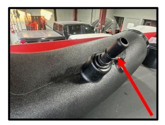
11. Install the supplied 5" ID x 2 1/2" hose over air inlet tube and airbox lid. Install the 4 1/2" x 4" hose over throttle body. Install the air inlet tube between the airbox lid and throttle body. Slide hose over throttle body. Secure all ends with the supplied hose clamps. \*NOTE: Route coolant vent line under air tube.
