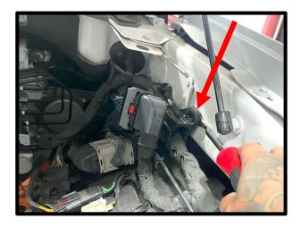
6. Cut the plastic push pin coming up from the **LH** inner fender so it only has .125" protruding.
