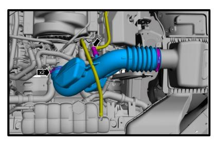
3. Loosen the clamp from the intake tube to airbox. Remove the (1x) bolt and (2x) push pins. Lift air cleaner assembly up and away from vehicle.
