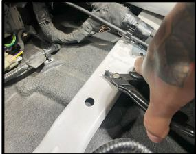
7. Remove the plastic retainer from the wiring loom.
