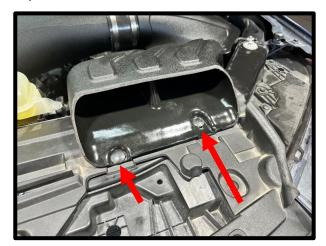
10. Install the (1x) supplied 13/16'' to 1/2'' rubber grommet into the inlet tube. Install the supplied 1/2'' to 15.82mm quick connect fitting.
