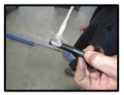
38. Using a 13mm socket, remove the upper left bolt form the idler pulley (or PS pump) assembly and the water pump bolt directly above the belt tensioner.
