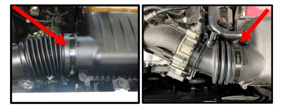
16. Remove the factory air box by using an 8mm nut driver on the (1) air box mounting bolt. Remove the rubber breather line from the air box. Lift the airbox straight up and away.
