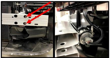
90. Mount IC pump to bracket, using the supplied T-Bolt clamp. Install rubber strip around OD of bump to rubber isolate in clamp. Secure clamp to bracket using the supplied (2) 6mm x 12mm HHFCS bolts.
