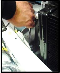
89. Install intercooler pump bracket to LH side of front bumper support, under head light, secure using the supplied (2) 8mm x 25mm HHFCS through the bumper support outer bolt holes, secure bolt with the supplied (2) 8mm flanged nuts.
