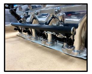
55. Install the (3) #2-906-V75BR orings to the (2) -6 ORB to 9.49mm and (1) -6 ORB to 9.49mm fittings. Apply light amount of grease to orings to ease installation. Install the 9.49mm fuel feed fitting on the LH/Driver side rail -6 port. Install the (2) 9.49mm fittings to the rear ports of each rail (fuel cross over).
