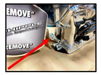
62. Install the (2) 9.89mm fittings and (1) 7.49mm quick connect fittings with the (3) #2-906-V75BR orings, to SC inlet. **NOTE:** 7.49mm fitting goes to front port (red arrow). Apply light amount of grease to oring to ease installation.
