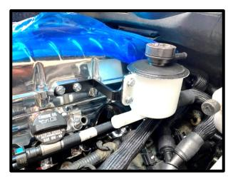
67. Install the supplied u-bend bypass hose to bypass actuator and 1/4" fitting.
