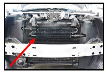
80. (Late model) Install the heat exchanger brackets to heat exchanger prior to installation. Use the supplied (4) 8mm x 25mm HHFCS bolts and (4) .813" sleeved washer per bolt.
