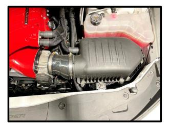
98. **(MY 06-10)** Locate stock make-up air hose. Install stock end to airbox lid. Install the supplied  $\frac{1}{2}''$  hose coupler to end of hose. Install supplied 90deg rubber hose end to hose coupler. Install this to make-up air barb in manifold.
