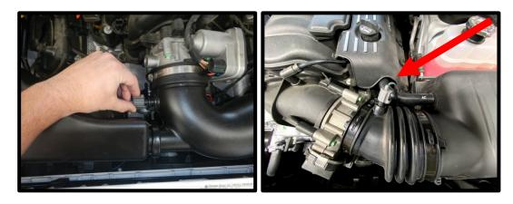
14. Disconnect the electronic throttle electrical connector by pulling the locking tab back and then squeezing the connector to release.
