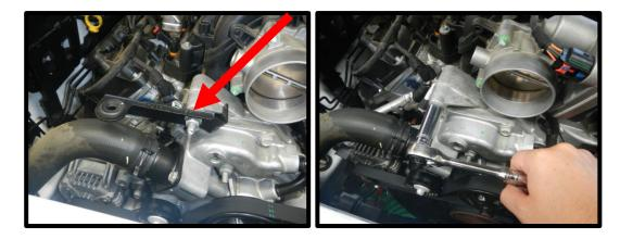
18. Remove the throttle body from the engine by removing the (4) mounting bolts, use an 8mm socket and ratchet.
