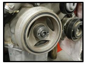
35. Use the supplied ¼" drill bit (it has a stop at roughly 2.875" from drill bit tip), drill 2 holes into the crankshaft thru the (2) holes in the pin adapter. Blow off debris when done drilling. Remove the pin adapter using an adjustable wrench.
