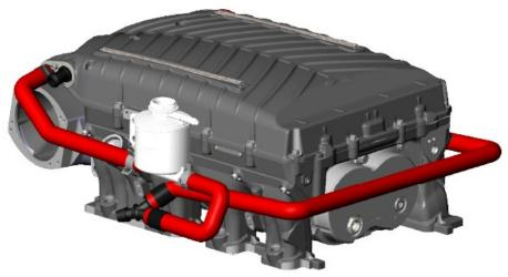
77. Install supplied RH side intercooler front fitting, intercooler outlet fitting. Route to supplied Y fitting below reservoir. Secure hose to Y fitting with supplied constant tension clamp. Secure hose to IC outlet fitting using black worm clamps.
