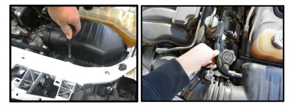
17. Remove the factory steel air inlet tube support bracket from the engine using a 16mm deep socket and ratchet (when applicable). Remove the factory bolt that the steel support inlet was bolted too using a 15mm deep well socket and ratchet.
