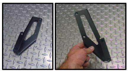
85. (**Early models**) Install the passenger side and driver side heat exchanger brackets over the previously installed 8mm bolts, secure with the supplied (2) 8mm flange nuts to just hold the bracket in place. The brackets will remain loose until all heat exchanger hardware is installed.
