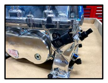
44. Remove the tape from the supercharger runners. Install the (10) factory manifold orings to the supercharger runners. Apply light amount of grease for ease of installation. Remove the tape covering the intake runners.
