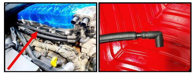
70. (LH/Driver side EVAP mount) Remove rear coil bolt and install EVAP bracket. Install EVAP solenoid to bracket. Install the supplied 3/8" x 33" EVAP hose with 90deg 9.89mm quick connect fitting. Route to front of fuel rail, under SC inlet and connect to bottom quick connect fitting previously installed. NOTE: PCV needs to go to top port on this type of installation.
