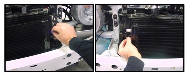
87. (**Early models**) Adjust the brackets as necessary to align the lower holes and install the final two 8mm flat head socket cap screws. Once centered, using a 5mm allen, torque the 8mm bolts to 18 ft/lbs.
