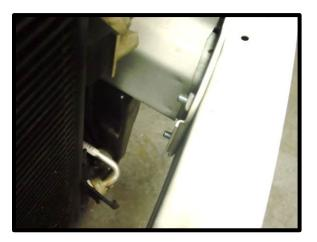
84. (**Early models**) Locate the passenger side and driver side heat exchanger brackets.
