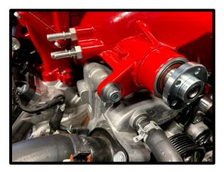
49. (Electric power steering-based vehicles) Remove the stock idler pulley from factory mount using 13mm socket. Replace with supplied 90mm idler pulley. Use factory hardware to secure in place. Torque to 18 ft-lbs using 13mm socket.
