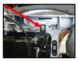
31. Remove the upper radiator mounts (2) using a 10mm socket and ratchet. Remove the lower mount bolts (4) using a 13mm socket/8" extension and ratchet. Carefully lower the radiator assembly to remove the electric fan assembly. If the vehicle is on jack stands, it will come out easily from the bottom.
