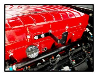
66. Install filler reservoir to bracket using the supplied (2) 6mm x 12mm HHFCS. Torque to 75 in-lbs using 10mm socket.
