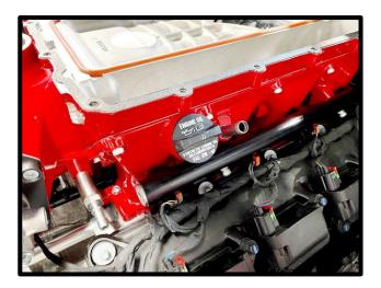
61. Install the (1) #2-906-V75BR oring to the -6 ORB to 9.89mm fitting. Install the (1) 9.89mm fitting in the LH side of SC inlet. Apply light amount of grease to oring to ease installation.
