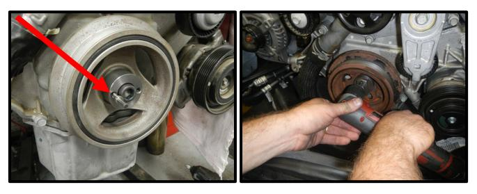
36. Install the supplied 1/4" dowel pins with a generous amount of green Loctite #648. Use a hammer and punch or drift pin to tap in so they are flush.
