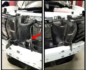
111. Mock up the front fascia to the front of the vehicle. Note that you may need to slightly notch the front grille area. There should be .25" clearance to the intercooler exchanger.
