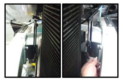
86. (**Early models**) Set heat exchanger behind bumper brace. Loosely install the upper two 8mm flat head socket cap screws on each side.
