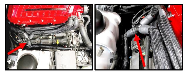
96. Connect the previously routed IC pump outlet hose to the filler reservoir Y fitting. Connect the filler reservoir breather hose to the filler reservoir top fitting. Secure ends with supplied constant tension clamps. Route down along the filler outlet hose, down away from exhaust. **NOTE: This can burp if system exceeds 10psi, do not run next to exhaust.**
