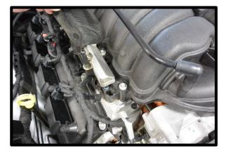
13. Disconnect the factory air temp sensor located in the factory air intake tube by squeezing the electrical connector and pulling from sensor.
