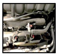
22. Remove the factory brake booster line from the back of the intake manifold and the brake booster. It's easier to remove from the brake booster and then snaking through when you're removing the intake manifold. Remove the factory 90deg plastic adapter from the brake booster hose end for later use. Note: 11-14 models must disconnect electrical connector at the brake booster by squeezing the connector to release.
