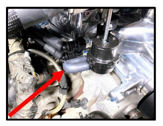
68. Install supplied 3/8" molded hose with 90deg end from SC inlet bottom 9.89mm quick connect fitting to PCV valve previously installed. Secure 90deg rubber hose with supplied #6 worm clamp.
