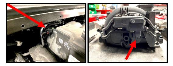
21. Remove the factory fuel supply line by squeezing the connector and pulling back or use a 3/8" fuel line removal tool (varies by year/application). It's a good idea to wrap a shop rag around this before you pull to catch any fuel that may drip. Disconnect the fuel injector connectors (8) by pulling the locking tab back and then squeezing the connector to release.
