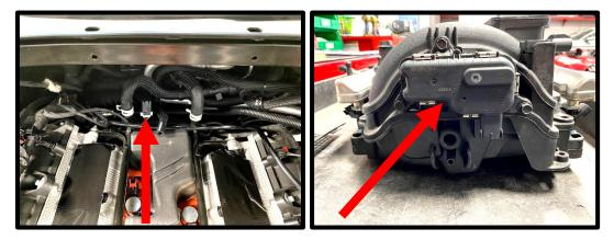
43. Install the supplied TMAP sensor to supercharger, apply light amount of grease to oring to ease installation. Secure to SC using supplied 6mm x 14mm FSHCS. Torque to 88 in-lbs using 10mm socket.
