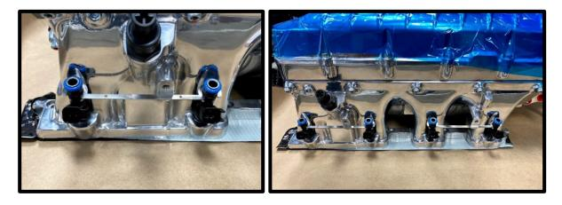
54. Secure rails to supercharger using the supplied (4) 6mm x 16mm SHCS. Use **Blue Loctite #243** on the threads of each bolt. Torque to 80 lbs-in.
