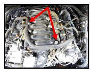
17. Disconnect the ventilation hose from the front left-hand side of intake manifold.
