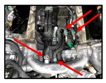
42. Using a 12mm socket on ¼" drive, remove the (4) nuts securing water cross-over from engine. This will not be reused. Clean the cross-over surface for installation prep, new gaskets are supplied, discard used gaskets.
