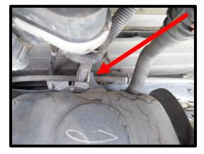
104. Start to lower tank another 4-6 inches and stop. Remove the fuel pump plastic cover for access to the electrical connectors.
