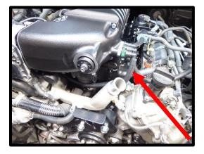
68. Using a flat head screw driver and cutters, release throttle body harness from stock bracket and zip-tie. Pull TB wires out of loom to give enough slack so throttle connector can reach throttle body, in a relaxed position. Wrap exposed wire with high grade electrical tape. Connect throttle body connector to throttle body.
