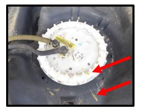
119. Ensure that the fuel lines running to the fittings are properly retained at the top of the tank.
