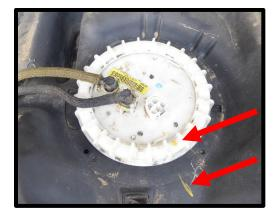
107. Use a fuel tank lock ring tool to remove the outer lock ring. As you loosen the ring, you will have to unclip the (3) lock tabs on top of the pump assembly every 1/3 rotation. Remove the fuel pump assembly from the tank along with the oring. Cover the tank opening to prevent debris from contaminating fuel/tank.
