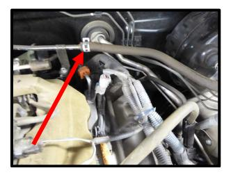
20. Disconnect the VSV and ACIS electrical connections.
