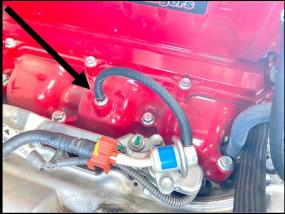
53. Install the supplied (3) 9.89mm quick connect to 6AN ORB fittings to SC inlet using a 11/16" socket or wrench. \*NOTE: Each fitting uses (1) viton -6 oring.
