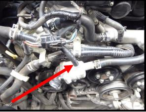
63. **(2014+)** Install the stock TB coolant hose from throttle body to thermostat housing. Secure both ends with stock hose clamps.
