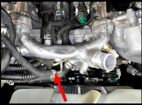
24. (When applicable) Remove and discard the wire harness support bracket from right hand side of engine, using 10mm socket (1 bolt and 1 nut).
