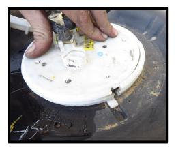
118. Use the lock ring tool to tighten the ring. Make sure yellow mark lines up on the hat lines up with the yellow mark on tank. Reinstall the fuel lines to hat assembly, ensure the yellow locking tabs snap in place.
