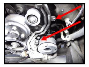
41. (2014 and up models) Disconnect the (2) heater hoses and 4 clamps from the valley of the block.
