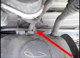
101. Disconnect the (3) hoses from the tank to filler neck junction. Follow these lines to the frame rail and release from retaining clips.
