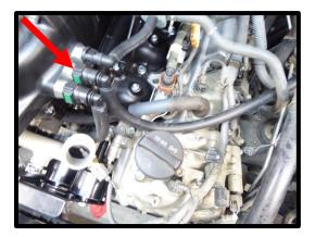
67. Install sheaving and heat shrink to hose (TUNDHOSE-0004). Install the supplied 3/8" x 10" hose to the PCV located in valley of block and front 9.89mm quick connect fitting.
