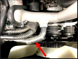
49. (2014+) Due to manifold clearance, lightly bend the center most hose barb end down .20".
