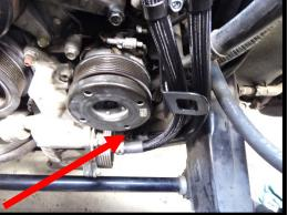
78. Secure oil cooler hoses to hose guard brackets using the supplied (4) dual cable ties. Mount to brackets using supplied (4) 6mm x 25mm HHFCS.
