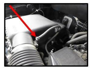
12. Use an 10mm socket or nut driver to loosen the (2) hose clamps securing the air inlet tube to the throttle body and MAF housing. This tube will no longer be used.
