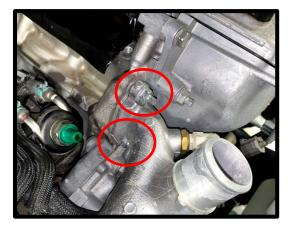
44. Using a 12mm socket, remove the (1) bolt from engine timing chain cover. This will not be reused.
