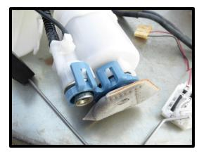
114. Remove the fuel pump and unplug the 2-way electrical connector.
