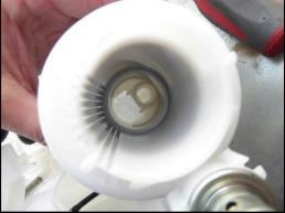
113. Remove the (5) fuel pump retainer clips from the fuel pump. Its important to go one at a time and ensuring each tab stays disengaged as you remove the others.
