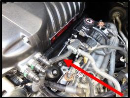
66. Install sheaving and heat shrink to hose (TUNDHOSE-0005). Connect the supplied  $3/8" \times 22 \frac{3}{4}"$  hose to middle 9.89mm quick connect fitting and route to brake booster.
