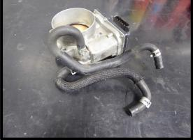
23. Using a clamp tool, disconnect the throttle body coolant hose from the water cross over barb (07-13MY). 2014+, disconnect from throttle body to PCV coolant hose barb.
