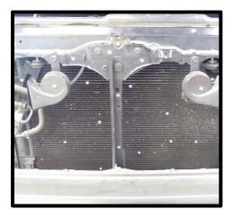
84. Remove the stock horns by removing the (2) bolts and disconnecting the electrical connectors.
