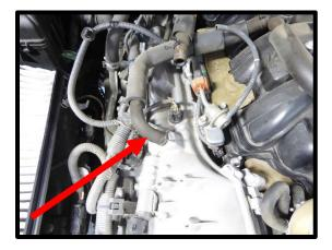
16. Using a 10mm (rear bolt) and 12mm (front bolt) socket, remove the (2) bolts from the ventilation hose support bracket. Remove the hose assembly from the engine.
