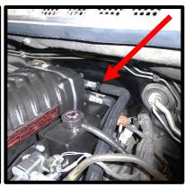
94. Install sheaving to hose (TUNDHOSE-0012). Install the intercooler reservoir outlet fitting hose (3/4" x 54") to IC reservoir forward facing 3/4" barb. Route down around the stock radiator, next to the IC feed hose previously routed. Then down to the IC pump. Secure both ends with supplied constant tension clamps. \*NOTE: Ensure hose cannot bind or ever kink.
