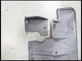
98. **(Flex Fuel vehicles disregard pump installation)** Raise the vehicle to access the fuel tank. Remove the tank protective cover by removing the (2) bolts and (2) nuts.
