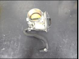
55. (2014+) Remove heater hose from throttle body hose barb as shown, this will be replaced.
