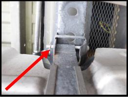
103. Remove the harness clip located at the top of the fuel tank on upper left side of the tank near frame. It helps to lower fuel tank 2-3 inches for better access.
