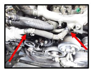
38. Remove the hose clamp from hose connecting the oil cooler hard line to rubber line loose.
