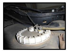
105. Unplug fuel pump electrical connecter from the top of fuel tank fuel hat assembly. Slowly lower the fuel tank, ensure it doesn't have any other connections as you lower, if so, disconnect and continue lowering.
