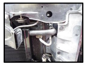
97. Test fit the lower splash guard if vehicle equipped with. Modify corner to clear IC pump. Reinstall lower splash guard using factory fasteners.
