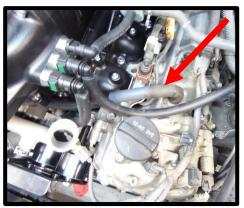
72. Install supplied silicone hose to airbox and throttle body. Secure using stock clamps. Secure stock valve cover vent hose to middle straight barb, secure with stock clamp. Install previously routed ½" hose from opposite valve cover to 90deg barb.
