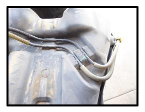
120. Follow the previous fuel tank removal and reverse to reinstall the fuel tank. Torque the factory fasteners for the (2) fuel tank straps to 30 lb-ft. Reinstall the factory tank protector if previously removed.
