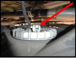
106. With the fuel tank lowered, clean the top of the tank and fuel pump hat from any debris. Remove the clip from the (2) tank fittings, then pull the fittings out. Wrap ends in a rag and gently move them out of the way. \*Note: The tank and hat are marked in yellow for the proper position, this is critical during reinstallation to realign.
