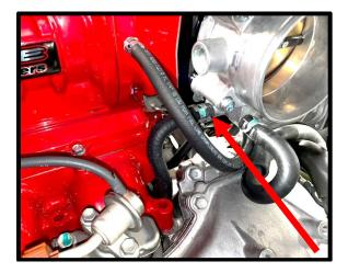
65. Install the VSV to the IC reservoir bracket. Secure to bracket using supplied 5mm x 10mm SHCS. Reconnect VSV 2-way connector. **(07-13)** Install supplied 5/16" x 4" hose (TUNDHOSE-0003) to VSV barb and 9.89mm quick connect fitting. **(14+)** install supplied 7/16" x 3 ½" hose (TUNDHOSE-0016) to VSV barb and 9.89mm quick connect fitting. Secure both ends with supplied (2) #10 hose clamps.
