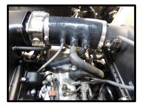
73. Install supplied hose mounting bracket #3102933 to engine timing cover, slide over stock stud and use supplied 6mm x 12mm HHFCS to secure. Torque to 80 in-lbs using 10mm socket.
