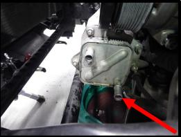
35. Using a 12mm wobble with 11" extension, remove the (2) nuts and (2) bolts securing A/C compressor to engine. Slide the compressor away from the engine while keeping it on the 2 studs (compressor does not need to be removed).
