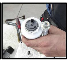
116. Clean the stock fuel tank to fuel hat oring using a degreaser. Install oring back in tank top. Apply grease to all sides of the oring to ease installation of the fuel hat.
