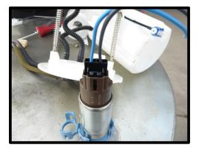
115. Remove the OEM oring and spacer from stock pump (oring may still be in inner housing). Install spacer and new supplied oring to new fuel pump. Apply light amount of grease to oring for ease of installation into fuel assembly. Assemble the pump assembly following the previous steps in reverse.
