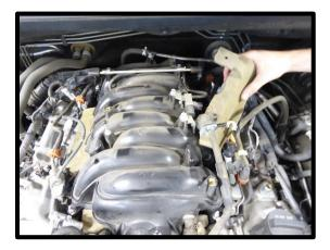
22. Disconnect throttle body connector from throttle. Using a 10mm socket, remove the (4) bolts securing TB to manifold. Remove the hose from the throttle body and thermostat housing by removing clamp and pulling hose away.
