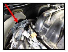
25. Remove wire harness clip from fuel rail on right hand side of engine, for manifold removal.
