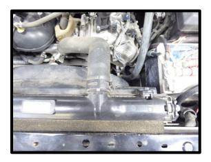
9. Disconnect the 2-way connector from the coolant temp sensor located at the water cross over.
