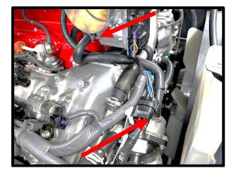
64. (2014+) Install the previously routed PCV to TB coolant hose from PCV. Secure to throttle body using stock clamp.
