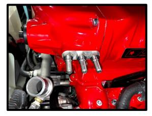
54. (2007-2013) Remove heater hose from throttle body hose barb as shown, this will be replaced.
