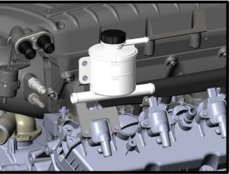
78. Install the IC pump bracket to RH frame rail, below the radiator by removing factory nut, install bracket and secure using factory nut. Install pump clamp to bracket using the (2) 6mm x 10mm HHFCS bolts. Install pump in clamp and secure in place.
