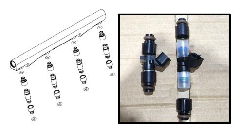
72. Install the fuel rail to the engine using the supplied (4) 6mm x 60mm HHFCS bolts and the (4) 39mm spacers. Torque bolts to 89 in-lbs, then an additional 90deg.
