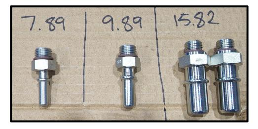
88. Install the (1) 15.82mm fitting to RH top port of SC inlet using 7/8" deep well socket. Install the (1) 7.89mm fitting to RH bottom port of SC inlet using 11/16" deep well socket.
