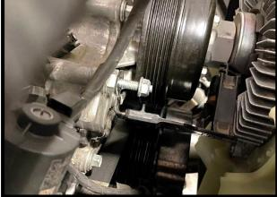
48. Remove the cooling fan using a Ford service tool 303-214 (T83T-6312-B) wrench. Note: Use a universal pulley holder (such as a Gearwrench 3900 or equivalent. Position upper radiator hose rearward. Raise fan up, rotate and remove the cooling fan.
