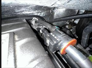
76. Install the intercooler filler reservoir to the LH valve cover, #5 (front) coil. Remove coil bolts using 8mm socket, install bracket, secure using stock bolt. Torque to 62 in-lbs, then an additional 45deg.
