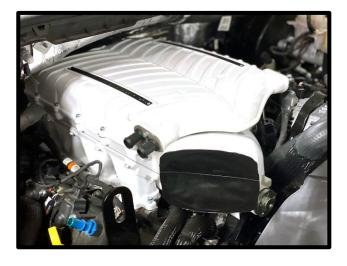
60. Pull supercharger forward so inlet is touching idler plate. Install supplied (1) 8mm x 25mm SHCS. Torque to 60 inlbs to pull SC forward (final torque is after SC to motor) using 6mm allen socket.
