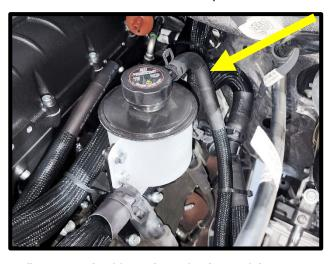
85. Install the supplied ¾" x 65 ½" IC pump feed hose from the forward-facing IC reservoir barb (secure with supplied pinch clamp), route to the pump inlet fitting, secure with supplied #16 pinch clamp. Secure previously routed 3/8" filler reservoir vent hose to this line. Secure hose with zip ties for clean installation. **NOTE:** Watch for any kinks.
