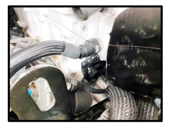
92. Install supplied 3/8" preformed hose #3103181 EVAP purge valve to 9.89mm fitting on LH side, bottom fitting previously installed.
