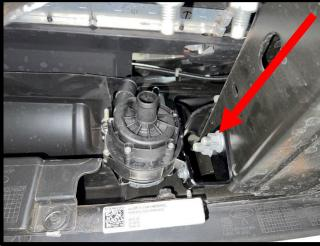
79. Set the heat exchanger brackets into position on the factory radiator. Secure the R bracket (RH side) using the (2) 6mm x 25mm HHFCS bolts. Secure the L (LH side) bracket using the (3) 6mm x 10mm HHFCS bolts. Secure LTR to brackets using the (4) .813" sleeve and (4) 8mm x 18mm HHFCS bolts.
