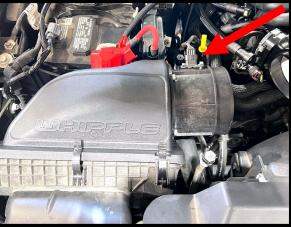
98. Install stock MAF sensor element and oring, in stock orientation to new MAF housing. Secure using the supplied (2) 4mm x 6mm SHCS. Torque to 17 in-lbs. \*\*DO NOT USE STOCK BOLTS\*\*. \*TIP: Verify arrow position for airflow direction. Reconnect MAF sensor electrical connector until it clicks and locks in place.
