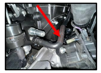
93. Modify the factory brake booster lines as shown below. Route the stock 15.82mm fitting to the 15.82mm quick connect fitting previously installed. Use supplied 3/8" x 60" vent hose around from booster, around back of supercharger, towards inlet of supercharger for later installation. **NOTE:** Vehicles equipped with Hydro-boost brake systems must skip this step.
