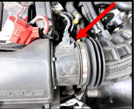
102. Connect the supplied MAF to IAT pigtail harness to MAF sensor. Route to the rear of the engine, connect to previously installed TMAP sensor, route single wire towards PCM ON RH firewall. Zip-tie harness for clean installation. **NOTE:** Remove any harness plastic fasteners from wiring loom that may rub or interfere with wiring or hoses.
