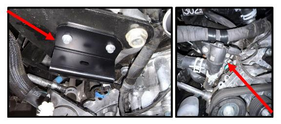
45. Install the supplied heater tube to the factory position previously removed. Using supplied locking bracket and factory bolt to secure, torque to 89 in-lbs. Install the supply 60deg preformed hose to heater tube using #16 clamp. Secure 60deg hose to factory hose using supplied 34" barb fitting. Secure with supplied pinch clamp and stock pinch clamp.
