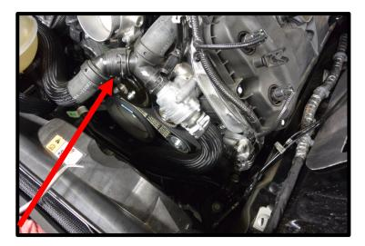
29. Remove the thermostat housing hose using a constant tension clamp tool. Pull away from thermostat housing. Remove the (2) bolts securing the thermostat housing body together using a 8mm socket.
