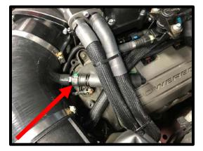
153. Connect the previously routed ¼" vent line to the stock overflow tank, secure with stock clamp. Secure this hose to the radiator hose and heater hose using multiple zip-ties.
