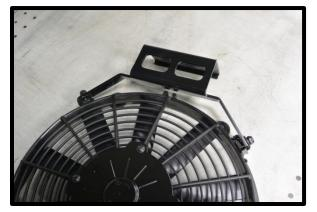
112. (**Dual fan installation**) Carefully set both fan assemblies on top front of the LTR, space these evenly before installing.
