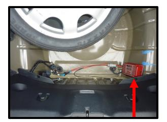
59. (Stage 2 and 3 FPVB) Using the factory stud in the spare tire area, install the ground wire from the FPVB to the stud. Secure stud using the supplied washer and nut.
