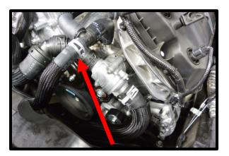
47. Using needle nose pliers, rotate the factory clamp at the water neck towards the driver side for future clearance of the SC. **NOTE:** Image shows clamp with SC installed to illustrate max clearance.
