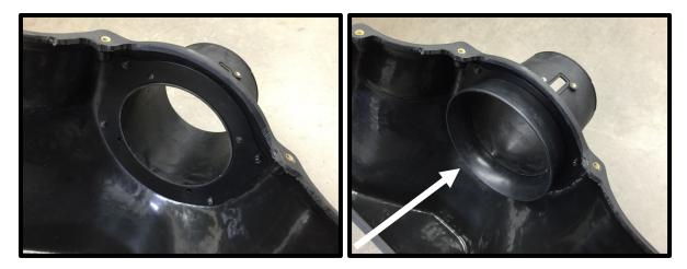
131. (Competition Kits) Using the supplied MAF housing and 123mm plastic venturi ring, mount to the new cold air box with the (4) 6mm x 16mm SHCS (5mm allen ball socket). Torque to 75 lbs-in.
