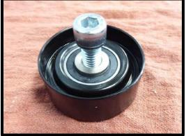
67. Remove the factory plastic smooth idler pulley from the engine. Replace with the supplied steel idler pulley. Use the factory fastener to secure. Torque to 18 lbs-ft with a 13mm socket. **NOTE:** Image shows proper direction of idler assembly.
