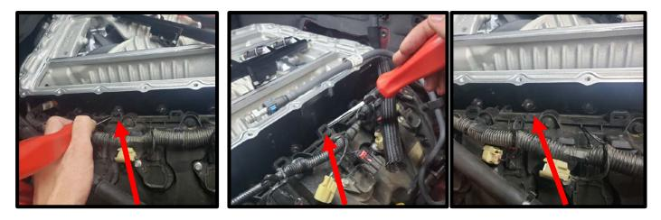
34. Remove the driver side heater tube from engine by removing the (1) bolt using an 8mm socket.
