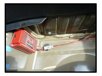
60. (Stage 2 and 3 FPVB) Using a razor blade, make a small incision in the factory rubber grommet, just below the FPVB. Install the supplied 1/8" ID rubber hose to the end 1/8" barb fitting on the FPVB (secure with zip-tie). Route the 1/8" ID hose through the grommet to the engine compartment. Follow the factory EVAP and fuel line from the rear of the vehicle to the front. Use zip-ties to secure this line away from heat.
