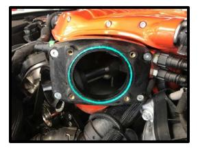
145. (Stage 1) Install the stock throttle body using the (4) 6mm x 50mm FHSCS bolts using a 10mm socket.
