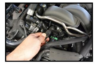
18. Remove the EVAP vent line quick connector from the EVAP solenoid by pushing the (2) locking tabs away and squeezing the tab, then pull away. Pull this line away from engine (goes down to driver side lower firewall area).
