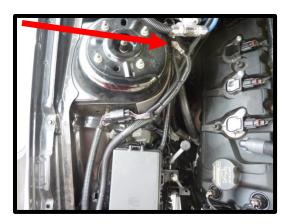
54. Pull the blue 15amp fuse from position **#49**. Install the 15amp blue fuse in the unused fuse slot on the fuse tap. Install the supplied fuse tap into position **#49**. Note: 15amp blue fuse should be in bottom slot, 5amp should be in top slot. Route wire above power stud and between center fuses. **NOTE:** Make sure wire has enough room when fuse cover closes. **NOTE:** Failure to install stock fuse back will result in ABS faults.
