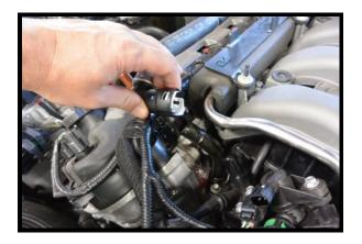
24. Remove the quick connect fitting on the heater tube, drivers side. Push hose to the back of the engine for later use.
