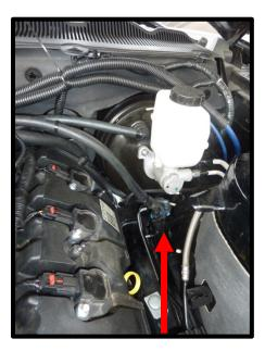
62. Using a 10mm socket, remove the (3) factory fasteners from the timing chain to head cover and (1) from water pump (for new idler plate).
