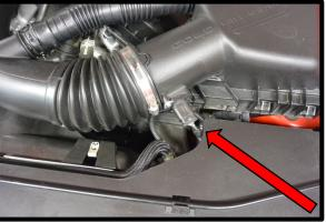
15. Release the locking tabs securing the upper airbox lid to the lower airbox. Disconnect the MAF wiring harness retainer from the front edge of the upper airbox lid and remove the lid from the vehicle. Remove the airfilter from the airbox. Using a 10mm socket, remove the (1) bolt securing the airbox to the inner fender. Remove airbox lower from vehicle. *NOTE: The stock cold air snorkel will be reused for the enclosed airbox.*
