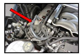
17. Disconnect the EVAP solenoid connector by squeezing locking tab and pulling away.
