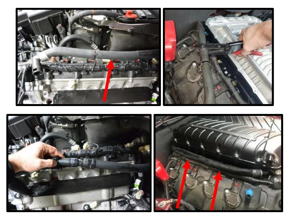
44. Install the supplied driver side heater tube to driver side of block (bracket has step in it). Install the supplied oring to the tube and apply light amount of grease to oring surface. Install tube into block and secure with the factory bolt using an 8mm socket. Torque to 89 lbs-in. Install the supplied tee and 90deg hose (18MST-1010 bag) to the driver side heater tube you just installed. Secure with the supplied constant tension clamp on the 90deg hose to heater tube.
