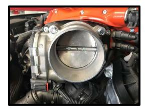
146. (Whipple 132mm Crusher throttle body) Remove the cream colored gear from throttle body by lifting up and away.
