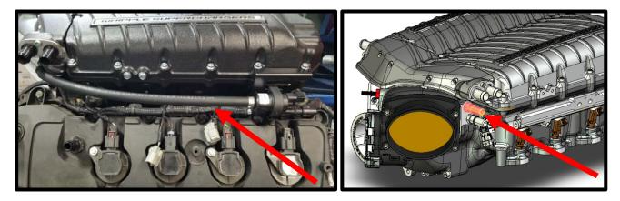
102. (**GT Version**) Install the supplied 3/8" x 20 ½" hose from the EVAP solenoid rear fitting to the EVAP fitting located under the brake booster. Connect 2-way electrical connector to EVAP solenoid.
