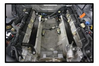
33. Using a hack-saw or cut off wheel, remove the 3<sup>rd</sup> wire loom support mount (from front) from both valve covers. Cut flush and grind the edge for a clean cut. **NOTE:** This is needed to clear fuel rail blocks.
