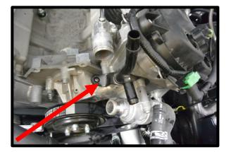
35. Loosen the (3) bolts securing the water pump pulley (while belt is on) using a 10mm socket. Remove the belt from the engine by using a 15mm socket on a 1/2" breaker bar and rotating the spring-loaded tensioner in a clockwise direction. Remove the spring-loaded tensioner from the engine using a 13mm socket. Using 10mm socket, remove water pump pulley from engine (will be reused later).
