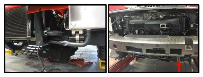
128. Install the supplied ¾" ID molded hose (#COYO-1300) from the IC OUT fitting to the airbox area for later installation. Secure end with supplied worm clamp. TIP: For hood clearance, ensure that the nut of the clamp is not on top.
