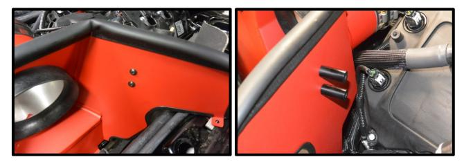
139. (Competition Kits) Install the intercooler filler neck to the (2) aluminum threaded stands using the (2) 6mm x 12mm flanged BHCS (4mm allen socket).
