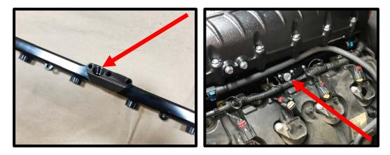
87. Install the supplied (2) #2-906 orings to the (2) inlet/outlet fittings. Install these (2) fittings into rear side of fuel rails. Apply light amount of grease to oring for ease of installation. Using a <sup>3</sup>/<sub>4</sub>" wrench (or <sup>3</sup>/<sub>4</sub>" deep socket) on both the front and rear fittings, tighten both. Install the (2) supplied 6AN 180deg swivel fittings to front port on each rail. Using a <sup>3</sup>/<sub>4</sub>" wrench, secure fittings to fuel rails.
