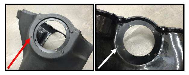
130. (Complete Kits) Using the supplied MAF housing and 123mm plastic venturi ring, mount to the new cold air box with the (4) 6mm x 16mm SHCS (5mm allen ball socket). Torque to 75 lbs-in.
