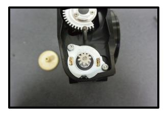
149. (Whipple 132mm Crusher throttle body) Reinstall the cream colored factory gear to the throttle body by lowering onto the pressed in shaft. Move until it falls into place.
