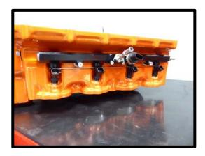
91. Install the supplied 3/8" fuel cross over line around the back of the supercharger by pressing until they click and lock in place.
