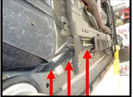
61. (Stage 2 and 3 FPVB) Route the hose to the engine compartment through the same passage as the EVAP and fuel hose. Route up along the fuel feed line and under the EVAP solenoid. Install the supplied 1/8" NPT to 1/8" ID barbed fitting into the intake manifold just below the EVAP solenoid. Install 1/8" ID FPVB line to barb fitting. Secure with zip-tie.
