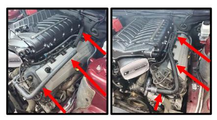
46. Reinstall the factory coolant overflow hose to the new supplied tee fitting on the driver side. Secure using stock clamp.
