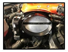
151. Install the supplied inlet tube from MAF to throttle body. Stock throttle body uses #56 clamp on stock throttle and #80 on MAF. 132mm TB uses #80 clamp and the MAF uses the #80 clamp.
