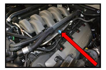
27. Remove the (4) bolts from the top of the intake manifold that secures the (2) heater hose trays. Use a 10mm deep well socket. Once bolts are removed, remove tray and foam material.
