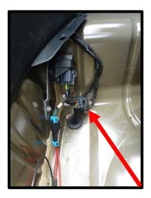
58. (Stage 2 and 3 FPVB) Connect the 2-way wire harness into the fuel pump driver module pigtail. Connect the other end to the FPVB. Mount the FPVB to the spare tire area (passenger side) using the supplied Velcro.
