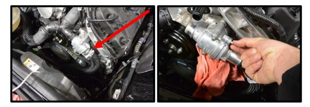
Remove the stock water neck using a 10mm socket. Install the supplied water neck. Secure using the supplied (1) 6mm x 25mm and (1) 6mm x 45mm bolts.
