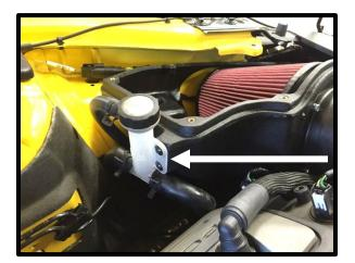
141. Connect the <sup>3</sup>/<sub>4</sub>" ID molded rubber hose you previously installed to the IC (**OUT**) fitting and connect to the IC filler neck. Secure with supplied pinch clamp.
