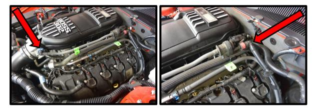
20. Remove the EVAP tubing from driver side valve cover (remove support from valve cover) and down below brake booster.
