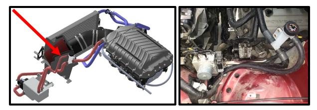
143. Install the previously routed hose from the Y fitting, to the LH core inlet fitting. Secure with worm clamp. **TIP: For hood clearance, ensure that the nut of the clamp is not on top**. Secure inlet and outlet lines with zip-ties for clean installation and protection from the belt.
