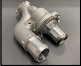
45. **(Dual Alternator)** Apply pipe sealant to threads of supplied 1/8" NPT to 5/16" barbed fitting, install to open 1/8" port on housing.
