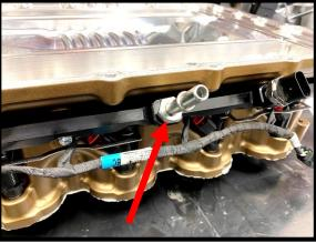
56. Install the supplied (1x) #2-906 Viton oring to the (1 of 2) 45mm long 9.49mm outlet fitting. Apply light amount of grease to oring for ease of installation, install to rail.
