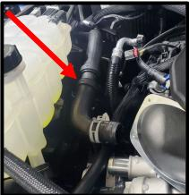
49. (**Dual Alternator**) Reconnect factory quick connect fittings to new coolant tubes.
