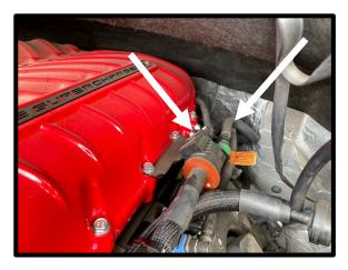
82. Install the supplied 3/8" ID x 13" with 55deg quick connect fitting hose to the EECPV barb fitting and **upper** quick connect fitting on SC inlet. Push until it clicks and locks into place.
