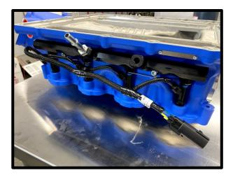
60. Install the supplied ¼" ID bypass actuator to the bypass nipple and ¼" 90deg nipple on SC inlet bypass hose. **CAUTION:** Do not open/close bypass actuator by hand. This may damage actuator internally. It only moves properly with equal vacuum/boost at the actuator reference port.
