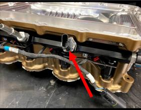
55. Install the supplied (1x) #2-906 Viton oring to the (1 of 2) 45mm long 9.49mm inlet fitting to fuel rail. Apply light amount of grease to oring for ease of installation, install to rail.
