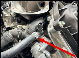
36. Install the supplied U shape heater hose. Secure both ends with supplied (2x) #12 worm clamps.
