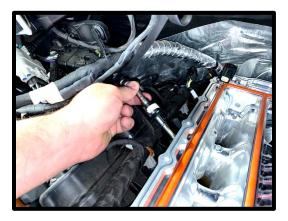
80. Connect the factory fuel inlet line to the driver side fuel fitting, press until it clicks and locks in place. Connect factory fuel psi sensor connector to sensor, press safety lock until it clicks into place.
