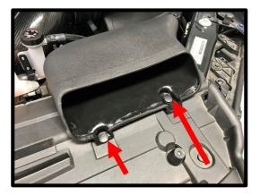
114. Install the supplied panel filter to the airbox lower. Install the upper airbox to the top of the filter. Secure the top to bottom using the supplied (6x) 6mm x 16mm BHCS. Torque to 50 in-lbs. \*Caution: Over torquing can result in pulling an insert out of plastic box.
