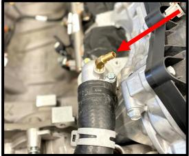
38. (**Single Alternator**) Reinstall water neck hose with supplied (1x) #24 hose clamp to new water neck.
