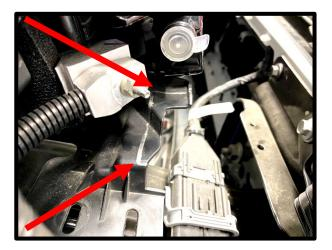
96. Install the supplied pump mount bracket (with 2x nutserts) into frame opening on **LH** side.
