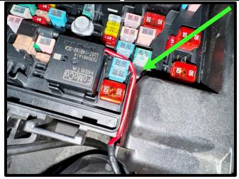
123. Test fit fuse box cover. Using small file or cutters, make small notch to lid as shown for the turn on lead.
