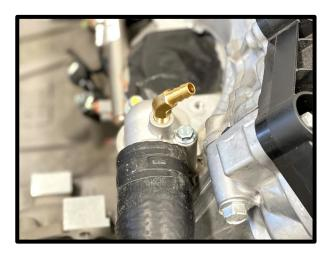
39. (**Dual Alternator**) Release the (3x) factory clamps from thermostat housing coolant lines. Pull hoses away.
