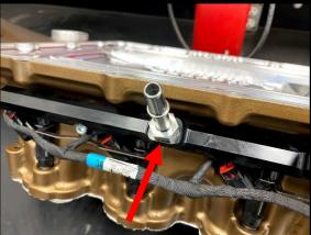
57. Install the supplied (2x) #2-906 orings to the (2x) inlet/outlet fittings. Install these (2x) fittings into rear side of fuel rails. Apply light amount of grease to oring for ease of installation. Using a ¾" wrench (or ¾" deep socket) on both the front and rear fittings, tighten both.
