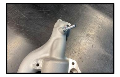
46. **(Dual Alternator)** Install the new thermostat housing assembly to engine using (3x) of the factory fasteners, leave hand tight for now.
