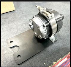
98. Mount the IC pump bracket to previously installed bracket using the (2x) 6mm x 14mm HHFCS bolts.
