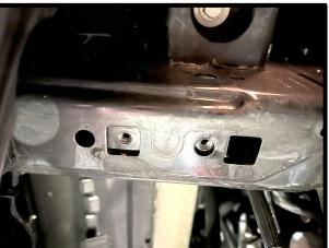
97. Mount pump to pump bracket using the supplied t-bolt clamp around the rubber section. Secure t-bolt clamp to bracket using the (2x) 6mm x 10mm HHFCS bolts. **NOTE:** Outlet fitting should be facing straight up.
