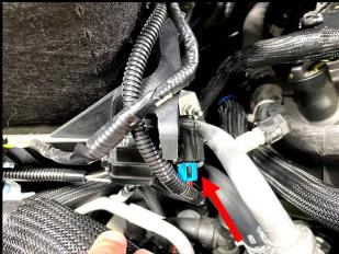
120. Using a 10mm socket, remove the nut on power stud, located on the positive stud under fuse box cover. Install the IC pump relay power eyelet (red wire) to the power stud on the battery positive (+) stud. Use a 10mm socket to secure stock and IC power wire.
