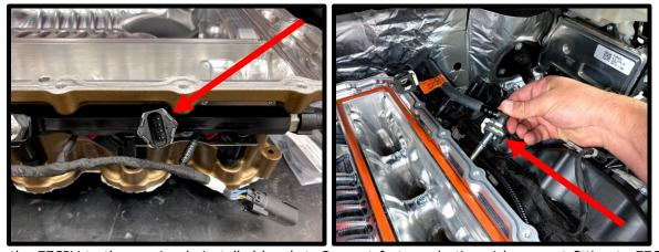
81. Slide the EECPV to the previously installed bracket. Connect factory plastic quick connect fitting to EECPV until it
