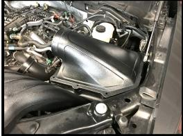
115. Install the (1x) supplied 13/16'' to 1/2'' rubber grommet into the supercharger inlet tube. Install the supplied 1/2'' to 15.82mm quick connect fitting.
