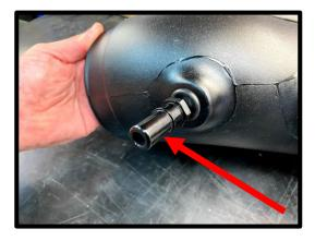
116. (**Whipple 132mm Crusher throttle body**) Install the supplied 5" ID x 2 1/2" silicone hose over air inlet tube and airbox lid. Install the 4 ¾" x 3" silicone hose over throttle body. Install the air inlet tube between the filter and throttle body. Slide silicone hose over throttle body. Secure all ends with the supplied (4x) #80 hose clamps.
