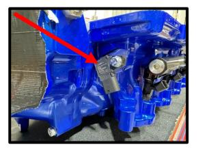
65. Install the supplied TMAP pigtail to the 3-Bar TMAP supplied, wrap up to SC inlet as this will get connected to stock harness later.
