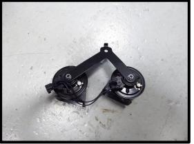
94. Reinstall new horn bracket and horns to factory location, using factory nut. Torque to 106 lbs-in. Zip-tie wire to factory harness for clean installation.
