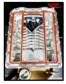
63. Install the supplied pre-formed 65.3" x .103" oring to the top sealing surface of the SC housing. Apply generous amount of grease to help ease the oring into place. **TIP:** To install oring into dove-tail groove, press vertically, vs sliding finger along.
