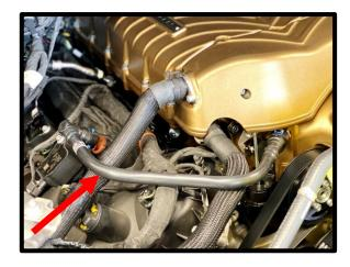
84. Connect the coolant vent line to new 5/16" 45deg barb fitting at water neck using stock clamp. Failure to do this will
