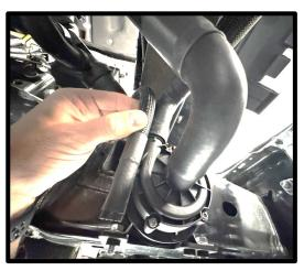
103. Install the ¾" ID x 12" rubber hose (#3103092) from the **LH (OUTLET)** IC fitting to the IC filler neck. Secure both ends with supplied #12 worm clamps. This goes under the air inlet tube. **NOTE: NEVER SWITCH THE INTERCOOLER ROUTING, BANK 2 IS ALWAYS THE OUTLET!**
