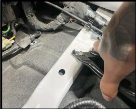
111. Remove the plastic retainer from the wiring loom.
