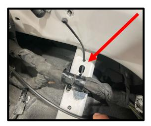
113. Install the supplied lower airbox into factory (2) hole locations. Using the supplied (2x) 1.1" L x .30" W plastic push pins, secure front of snorkel to factory location.
