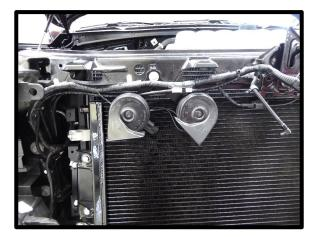
95. Using a saw or shears, cut the plastic shroud as shown, below the RH side heat exchanger fitting. This will allow proper clearance for the hose to be installed later.
