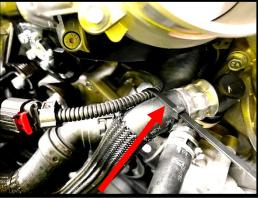
76. Reinstall the water pump pulley using a 10mm socket, torque to 14 lbs-ft.
