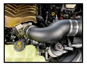
118. Install the stock make up air hose to air tube fitting previously installed. Fittings may require some rotation to properly fit.
