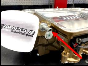
83. Install the stock PCV hose to the **RH** side valve cover. Connect other end to the supercharger inlet 15.82mm quick connect fitting. \*Note: This requires you to rotate the fittings for proper fitment. Push until it clicks and locks into place.
