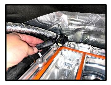
75. Install the supplied electronic throttle pigtail to the factory electrical connector. Route under front idler plate front
