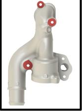
47. **(Dual Alternator)** Install the supplied #2-113 oring to new coolant tube. Install tube to thermostat housing. Secure coolant tube using the (2x) 6mm x 50mm HHFCS bolts supplied. Torque all (5x) thermostat housing bolts to 89 lbs-in.
