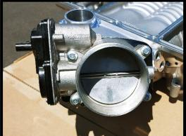
106. (**Stage 2 Whipple 132mm Crusher throttle body**) Install throttle body to supercharger inlet, use the supplied gasket between TB adapter and SC inlet. Secure with the supplied (3x) 6mm x 25mm SHCS and (1x) 6mm x 50mm SHCS using a 5mm allen socket. Torque to *89 lbs-in* on first pass, *139 lbs-in* on second pass.
