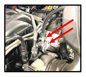
33. (**Single Alternator**) Disconnect the driver side heater tube quick connect fitting by squeezing and lifting away. Remove the heater tube overflow hose using a pinch clamp tool. Using an 8mm socket on the 1 factory bolt, remove the heater tube.
