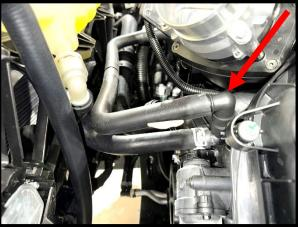
37. **(Single Alternator)** Transfer stock oring from stock water neck to new water neck (clean oring as needed). Apply pipe sealant to threads of 1/8" NPT to 5/16" 45 Deg fitting. Install fitting to water neck, rotate so it ends facing directly towards driver side. Install water neck to motor using stock fasteners (10mm socket), torque to 89 lbs-in.
