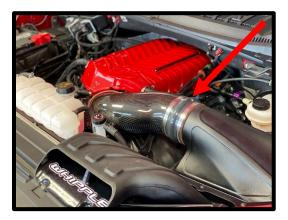
117. **(Stock throttle body installations)** Install the supplied 5" ID x 3" silicone hose over air inlet tube and airbox lid. Install the supplied reducer silicone hose over air inlet tube and stock throttle body. Connect the other end to the stock throttle body. Secure all ends with the supplied hose clamps (2x) #80, (1x) #64 and (1x) #56 on throttle body.
