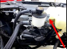
100. Install the supplied ¾" ID x 34" molded/formed hose (#3103500) with the 90deg end on the LTR bottom **LH** side fitting. Secure both ends with supplied pinch clamps. This must clear the plastic shroud and AC stud or it will wear a hole in hose. \*NOTE: Use zip-ties to secure hose to core support.
