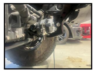
110. Install the supplied hose #3103521 to the reservoir front fitting to the pump inlet. Secure both ends with #12 hose clamps.
