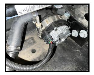
130. Using crimpers, connect the fuse tap wire to the barrel connector. Slide the supplied heat shrink over barrel crimp connector, use heat gun to shrink and seal connection. Remove the stock 10A fuse from **location #F50 HD ACC**, install into supplied fuse tap in spot previously occupied by 10A fuse. Install fuse tap to **#F50 HD ACC**. This will have the stock 10A fuse and the supplied 5A for IC pump system. NOTE: Make sure wire is clear of any potential chaffing or cutting.
