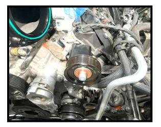
97. Torque the (5x) 6mm x 15mm SHCS pulley bolts to 119 in-lbs.
