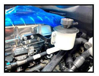
90. Install supplied 3/8" #5000360 hose to SC inlet bottom 9.89mm quick connect fitting previously installed. Install stock EVAP 90deg to end of hose. Secure to EVAP solenoid (#1).
