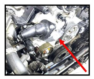
77. Route the other end of hose #50000378 back, just under water neck, behind the lower idler mount, down to the stock oil filter mount. Install the other end down to oil filter mount barb. Secure hose with supplied (1x) #6 hose clamp. Secure hose using zip ties to keep away from belt system.
