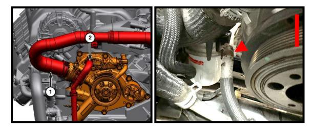
28. Using 7/16" allen socket, remove factory barbed fitting from water pump, this will not be reused.
