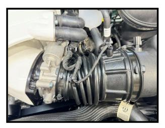
118. Install the stock breather hose to airbox lid. Route under reservoir to supplied  $\frac{1}{2}''$  hose #5000383. Couple together using supplied  $\frac{1}{2}''$  to  $\frac{3}{4}''$  coupler. Secure  $\frac{1}{2}''$  hose end to hose barb next to oil fill cap.
