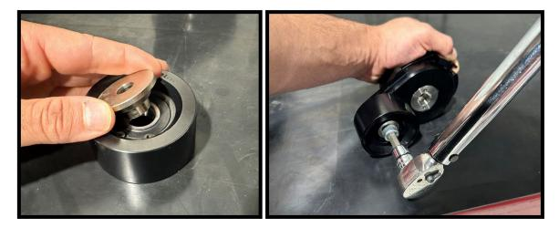
53. Mount the supplied spring-loaded tensioner to new tensioner mount using supplied (1x) 10mm x 60mm SHCS. Torque to 18 ft-lbs.
