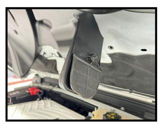
121. Install the air inlet snorkel mounting brackets to snorkel with the (5x) support brackets shown in the next steps.
