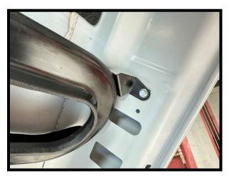
124. Secure rear RH side of snorkel using bracket 04-1000-00373 (1x). Secure brackets to airbox using (2x) 4mm x .7mm SHCS. Secure to hood using (1x) 6mm x 20mm HHFCS.
