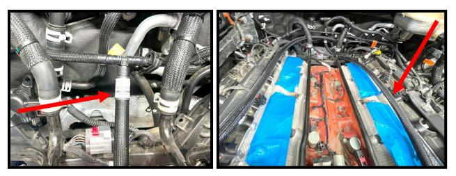
47. Preinstall the supplied #5000360 EVAP hose to the EVAP solenoid. Secure hose using (1x) #4 hose clamp. Route hose to RH side of engine for later installation.
