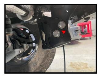
109. Mount pump and t-bolt clamp to IC pump bracket using the (2x) 6mm x 12mm HHFCS bolts.
