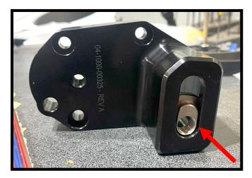
50. Using the .390" idler step spacer, 1/2" ID step washer and (1x) ½" x 2" SHCS bolt, mount the 87mm grooved idler (#36157) pulley to idler mount. Leave idler slightly loose for later belt adjustment.
