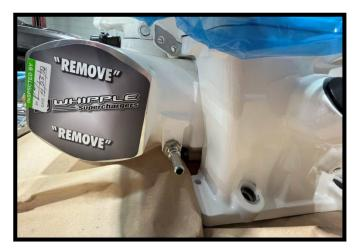
87. Install the (2x) 9.89mm fittings with the (2x) #2-906-V75BR orings, to SC inlet. Apply light amount of grease to oring to ease installation.
