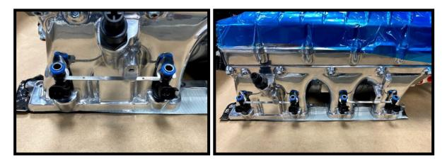
80. Secure rails to supercharger using the supplied (4x) 6mm x 16mm SHCS. Use **Blue Loctite #243** on the threads of each bolt. Torque to 80 lbs-in.
