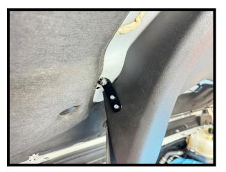
125. Secure rear LH side of snorkel using bracket 04-1000-00373 (1x). Secure brackets to airbox using (2x) 4mm x .7mm SHCS. Secure to hood using stock fastener.
