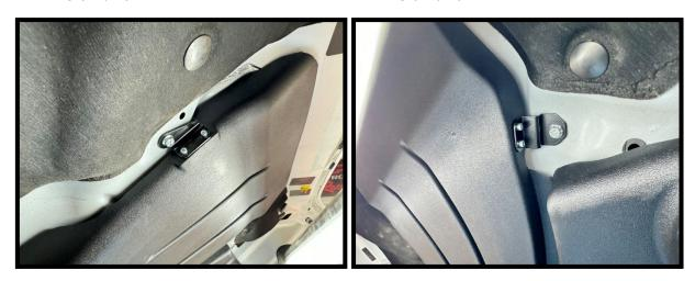
123. Secure front of snorkel using bracket 04-1000-00376 (LH front). Secure brackets to airbox using (2x) 4mm x .7mm SHCS. Secure to hood using (1x per) 6mm x 20mm HHFCS.
