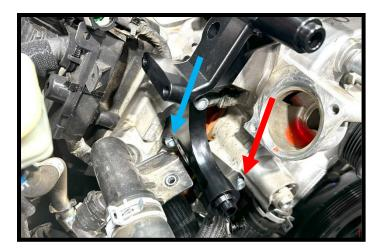
56. Install the new water neck to the factory location, above the thermostat. Secure using the supplied (2x) 8mm x 25mm SHCS. Torque to 18 ft-lbs. **NOTE**: Rear bolt requires ball head allen socket.
