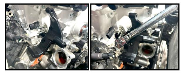
55. Install the idler pulley mount to engine block and alternator relocation bracket. Secure using the supplied (2x) 8mm x 22mm SHCS (red arrows) and (1x) 8mm x 35mm SHCS (top, blue arrow). Torque to 18 ft-lbs.
