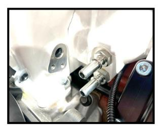
88. Install filler reservoir bracket to the LH side of supercharger lid. Use supplied (2x) 6mm x 12mm HHFCS. Torque to 89 in-lbs using 10mm socket.
