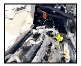
86. Install the (1x) #2-906-V75BR oring to the -6 ORB to 9.89mm fitting. Install the (1x) 9.89mm fitting in the LH side of SC inlet. Apply light amount of grease to oring to ease installation.
