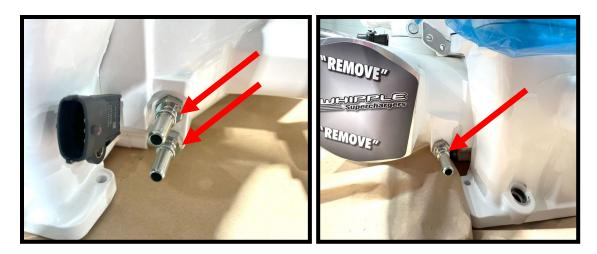
61. Apply light amount of pipe sealant to supplied (1x) <sup>1</sup>/<sub>4</sub>" NPT to <sup>1</sup>/<sub>4</sub>" barbed fitting threads. Install fitting into SC inlet.
