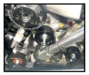
73. Install supplied 63.50mm smooth idler pulley to original tensioner mount. Use supplied (1x) 10mm ID step washer and supplied (1x) 10mm x 40mm SHCS. Torque to 21 ft-lbs.
