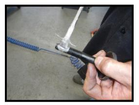
44. Remove the (8) coil electrical connectors. Remove the coils using a 10mm socket and ratchet (2 bolts per coil). Lift the coil out and use a 5/8" spark plug socket and ratchet to remove the stock spark plugs (16). Apply light amount of anti-seize to the new spark plugs, torque to 7.5 -15 ft-lbs. Reinstall stock ignition coils in same locations as they were originally removed. **IMPORTANT! Gap plugs to .032".**
