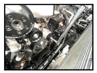
74. Install supplied 63.50mm smooth idler pulley to alternator relocation bracket. Use supplied (1x) 10mm ID step washer and supplied (1x) 10mm x 40mm SHCS. Torque to 21 ft-lbs.
