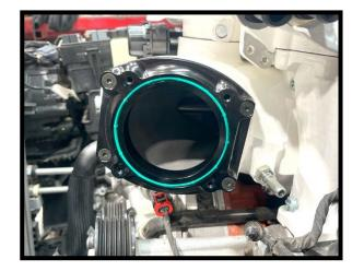
65. Remove the tape from the supercharger runners. Install the (10x) factory manifold orings to the supercharger runners. Apply light amount of grease for ease of installation. Remove the tape covering the intake runners.
