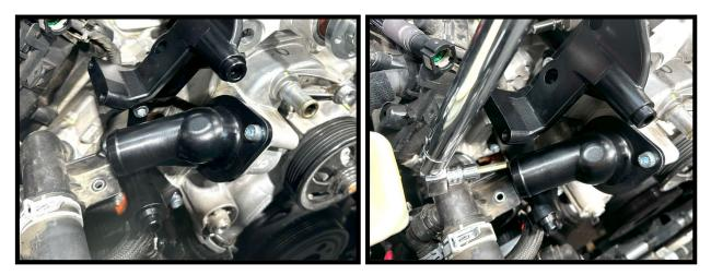
57. Install supplied water hose support bracket to idler bracket, using the (2x) 6mm x 12mm HHFCS bolts. Torque to 80 in-lbs.
