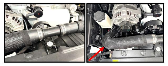
94. Install the stock alternator to the updated bracket. Use factory (2x) bolts (3 in image). Secure upper boss using supplied (1x) 8mm x 70Xmm HHFCS. Torque to 18 ft-lbs. Secure B+ using factory hardware, torque to 10 ft-lbs. Reconnect stock generator field harness connector until it clicks and locks in place.
