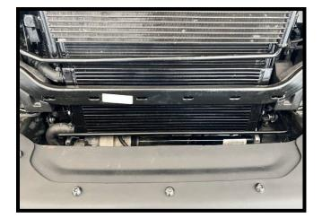
107. Install the heat exchanger brackets to vehicle and heat exchanger. Use the stock fastener to secure to vehicle, use supplied (4x) 8mm x 16mm HHFCS bolts to secure heat exchanger to brackets.
