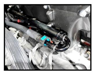
85. Reconnect stock fuel feed hose to the 9.49mm fitting you previously installed. **CAUTION:** Ensure fuel fitting clicks and locks in place.
