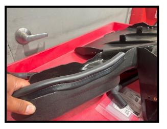
120. Transfer the rubber flaps from stock snorkel to new airbox snorkel using factory hardware.
