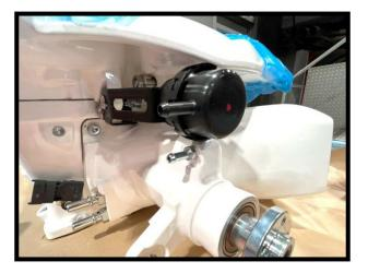
62. Install the (1x) #113 oring to PCV fitting. Apply light amount of grease to oring. Install the PCV fitting to the RH side of open passage on supercharger runner.
