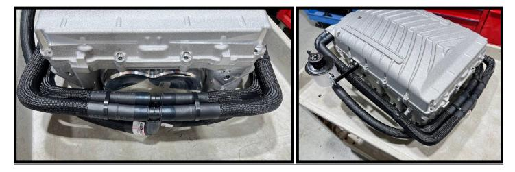
103. Connect hose #3103521 from IC pump inlet to filler reservoir forward facing fitting. Secure both ends using (2x) #12 worm clamps.
