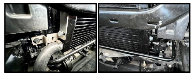
108. Install intercooler pump bracket to LH frame mount. Remove the (2x) stock fasteners, install IC pump mount bracket. Resecure using factory fasteners.
