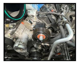
52. Install supplied 63.50mm smooth idler pulley to new spring-loaded tensioner. Use supplied (1x) 10mm ID step washer and (1x) 10mm x 40mm SHCS. Torque to 18 ft-lb
