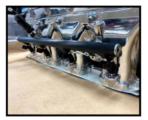
81. Install the (3x) #2-906-V75BR orings to the (2x) -6 ORB to 9.49mm and (1x) -6 ORB to 9.49mm fittings. Apply light amount of grease to orings to ease installation. Install the 9.49mm fuel feed fitting on the LH/Driver side rail -6 port. Install the (2x) 9.49mm fittings to the rear ports of each rail (fuel cross over).
