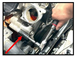
37. Remove the plastic wire retainers from block and wiring loom from LH front cylinder head.
