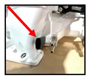
60. Install the (3x) 9.89mm fittings with the (3x) #2-906-V75BR orings, to SC inlet, (2) on RH side of inlet and (1) on LH side. Apply light amount of grease to oring to ease installation.
