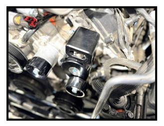
54. Install the alternator relocation bracket to factory location. Secure using supplied (4x) 10mm x 60mm SHCS. Torque to 21 ft-lbs.
