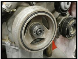
41. Use the supplied ¼" drill bit (it has a stop at roughly 2.875" from drill bit tip), drill 2 holes into the crankshaft thru the (2) holes in the pin adapter. Blow off debris when done drilling. Remove the pin adapter using an adjustable wrench.
