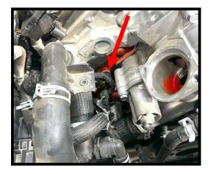
36. Remove the factory fastener from water pump, just under thermostat housing.
