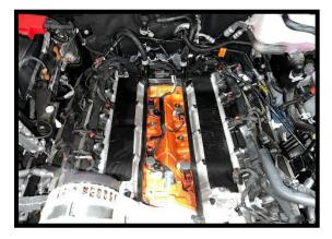
20. Using a 3/8" ratchet or breaker bar, release the tension from the spring-loaded tensioner by rotating clockwise. Remove the 6-rib belt from the engine. Using 16mm socket, remove spring loaded tensioner from engine (needed for belt system installation).
