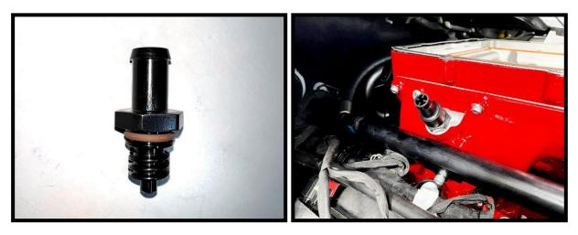
63. Remove the factory oil fill cap from stock intake manifold, transfer to supercharger LH runner oil port.
