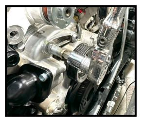
29. Remove factory thermostat housing, this will no longer be used (keep thermostat, this will stay in place).
