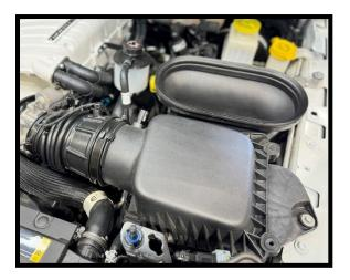
117. Install stock air inlet tube using factory clamps to throttle body and airbox. Reinstall wiring harness retainers to stock locations.
