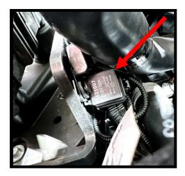
129. Route the main pump connector down, across radiator support area and to the pump. Connect to pump. Secure harness away from heat and any moving parts using zip-ties.
