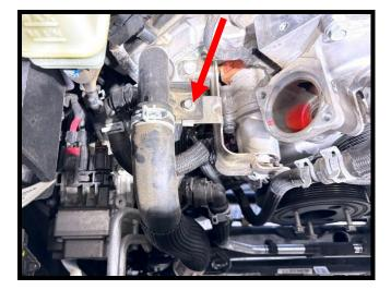
34. Remove the factory radiator hose support bracket from engine, this will no longer be used.
