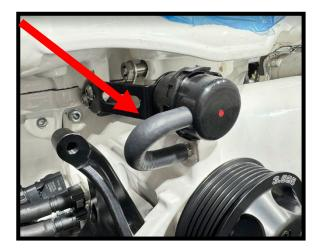
93. Install stock radiator hose sleeving over supplied radiator hose #3103424. Install the supplied radiator hose to engine. Secure end to stock coupler (1x #20 clamp) and other end to water neck using (1x) #24 hose clamp. Replace stock clamp using the (1x) #20 hose clamp. NOTE: Ensure it fits post barb at water neck or it could leak later.
