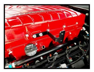
89. Install filler reservoir to bracket using the supplied (2x) 6mm x 12mm HHFCS. Torque to 75 in-lbs using 10mm socket.
