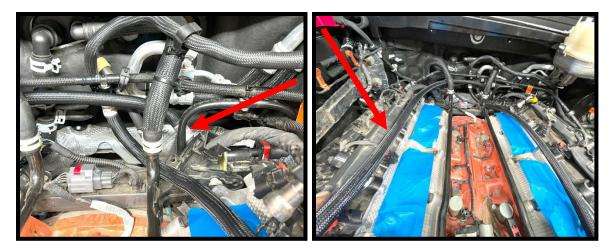
48. Apply light amount of pipe sealant to supplied (1x) 3/8'' NPT to -6AN fitting NPT threads. Install fitting into factory water pump vent port.
