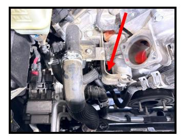
35. Remove plastic retainer and loom from RH side engine block.
