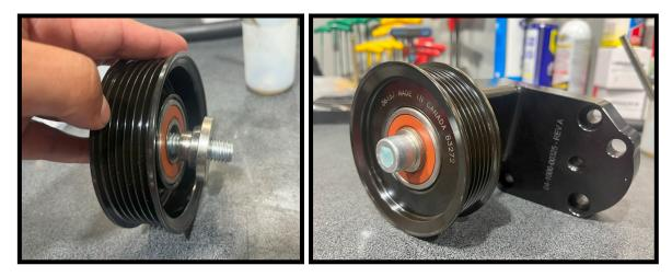
51. Mount the billet idler/tensioner mount to the LH cylinder head. Use the supplied (3x) 8mm x 60mm SHCS. Torque to 15 ft-lbs.
