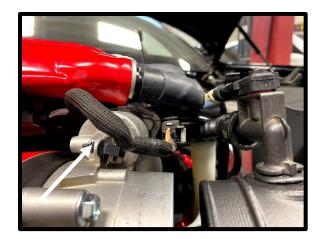
37. Install supplied rubber grommet to airbox from the inside. Install the supplied air tube, using a flat blade screwdriver to pull grommet lip away from air tube. Once in position, push edge of grommet into position. Install air filter to end and secure with stock clamp. Secure both ends of silicone hose couplers to air tube and throttle body. Secure airbox to factory mount with stock bolt. Install supplied rubber airbox seal to top of airbox.
