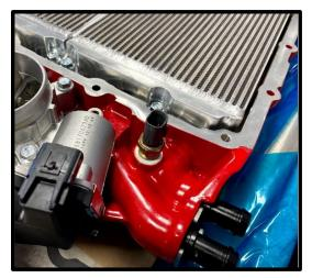
31. Assemble the intercooler hoses. For inlet (blue), take (2) of the #3103182 hose, face the short 90deg ends towards each other. Secure to tee fitting using supplied pinch clamps. Assemble hose #3103184 to tee fitting, secure with pinch clamp. For outlet (red), take (2) of the #3103182 hose, face the short 90deg ends towards each other. Secure to tee fitting using supplied pinch clamps. Assemble hose #3103183 to tee fitting, secure with pinch clamp.
