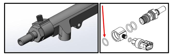
16. (**Billet fuel rails**) Install the (2x) #2-115 Viton orings to male fitting. Apply grease to oring and slide through female fitting. Install (1x) #3-908 Viton oring to fitting (shown with red arrow). Install banjo fitting to the longer fuel rail (PN# YH06-WPL83-0054). Use light amount of grease on oring. Install fitting to the RH side rear port.
