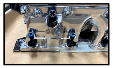
15. (**Billet fuel rails**) Install the (2x) #2-115 Viton orings to male fitting. Apply grease to oring and slide through female fitting. Install (1x) #3-908 Viton oring to fitting (shown with red arrow). Install fitting to the driver side fuel rail (rear). Install the supplied fuel PSI sensor to fuel rail adapter using (1x) #2-011 oring. Reconnect fuel PSI sensor electrical connector.
