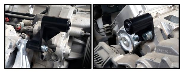
20. Install smooth 74mm supplied pulley to bracket using the step spacer and (1x) 10mm x 30mm HHFCS. Torque to 22 ft-lb.
