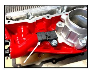
29. Lay supplied pigtail harness to LH/Driver side of supercharger. Connect the stock driver side stock TMAP sensor connector to pigtail. Plug in 3" pigtail to (LH) back of sc (back driver side of engine) post SC, post IC (#3) connector 4-way (1 =blue/green, 2 = blue/light blue, 3 = yellow/red, 4 = brown/pink). Connect female pigtail to stock to intermediate TMAP male connector. Connect end of pigtail to the (intermediate) TMAP sensor you previously installed to bottom of lid (next to bypass).
