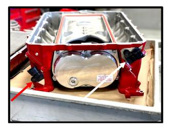
3. Install the Post SC, pre IC TMAP to the SC lid as shown. Secure using the supplied (1x) 6mm x 14mm HHFCS. Torque to 88 in-lbs using 10mm socket.
