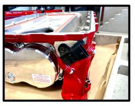
28. Install the supplied 18" MAP sensor harness to the post SC, pre-IC MAP sensor connector (back driver side of engine) (#2) connector 4-way (1 =blue/green, 2 = purple/blue, 3 = yellow/red, 4 = purple/yellow). Route to the front of engine and secure to previously installed TMAP in SC lid.
