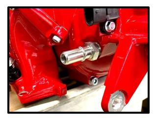
6. Install the supplied -6 ORB with oring to 9.89mm fitting to LH port on SC inlet. Use light amount of grease on oring for ease of installation.
