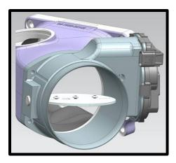
36. Reconnect the throttle body 6-way connector. Reinstall Christmas tree retainer to secure harness.
