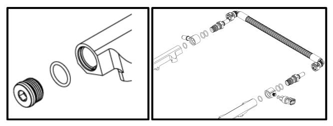
18. Install the supplied molded rubber oring to the supercharger oring groove.
