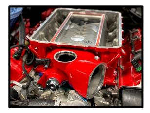
10. Install the supplied (1x) 10mm x 25 SHCS bolt to front support. Lightly torque to 42 in-lbs only to slide SC forward.
