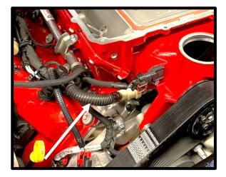
24. Connect the stock bracket booster hose to the 9.89mm fitting previously installed.
