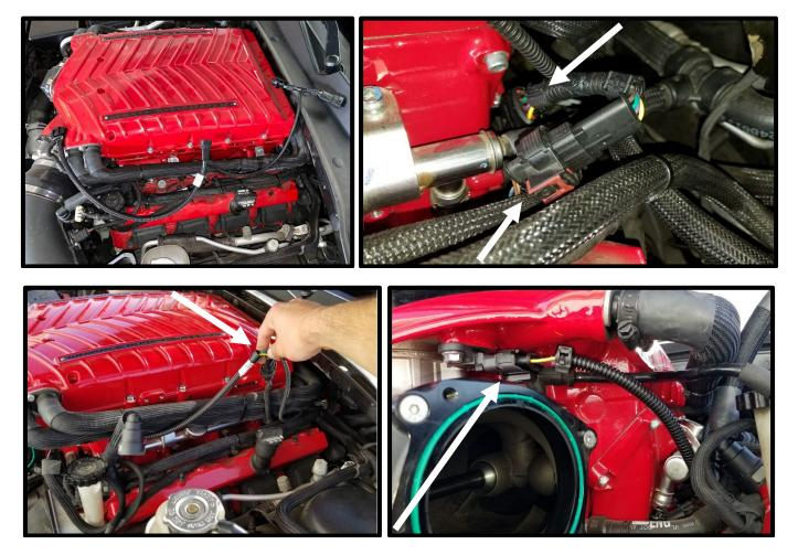
30. Install the supplied 22" IC temp sensor extension to stock 2-way connector by cutting the stock connector off 3" from end. Install pigtail using the supplied butt connectors, crimp together, then slide heat shrink over and shrink. Route to front of engine and connect to previously installed temp sensor.
