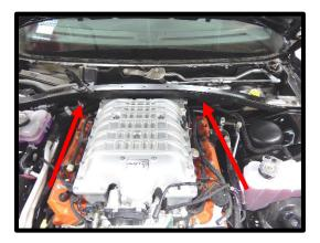
42. Reinstall the plastic cowling to the vehicle by installing the (8) push pins you previously removed. Make sure the tabs on each side lock in place.
