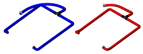
32. Install the supplied intercooler **inlet** <sup>3</sup>/<sub>4</sub>" ID hose (#3103184) to the factory inlet aluminum tubing, connect to factory line using stock pinch clamp. Connect the (2) inlet hoses to the rear most fittings on each side of the supercharger lid. Secure with the supplied black worm clamps on both inlet fittings.
