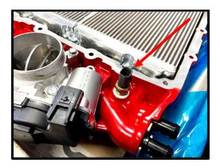
5. Install the supplied -6 ORB with oring to 15.82mm fitting to RH port on SC inlet. Use light amount of grease on oring for ease of installation.
