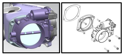
35. (**Billet throttle body**) Install supplied TB oring to TB, use light amount of grease to hold in place. Install the billet throttle body to the SC inlet using the (4x) 6mm x 25mm SHCS bolts. Use Blue Loctite #243 on threads, torque to 88 in-lbs using a 5mm allen socket.
