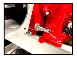
7. Install the supplied -6 ORB with oring to 3/8" barb fitting to LH top port on SC inlet. Use light amount of grease on oring for ease of installation.
