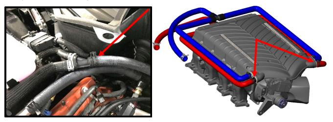
34. (**Stock throttle body**) Install the stock TB adapter to the supercharger inlet using the supplied TB adapter, supplied gasket and the (4x) 6mm x 25mm FHCS. Torque to 75 in-lbs. Install the stock throttle body oring to TB adapter, then install the throttle body using the (4x) 6mm x 35mm HHFCS bolts. Use **Blue Loctite #243** on threads, torque to 88 in-lbs using a 10mm socket.
