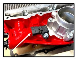
4. Install the stock IC temp sensor, using light amount of thread sealant to the Whipple lid port.
