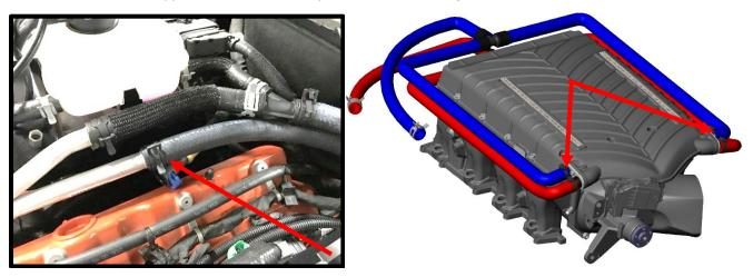
33. Install the supplied intercooler **outlet** <sup>3</sup>/<sub>4</sub>" ID hose (#3103183) the factory Y fitting using stock pinch clamp. Connect the (2) outlet hoses to the forward most fittings on each side of the supercharger lid. Secure with the supplied worm clamps on both outlet fittings.
