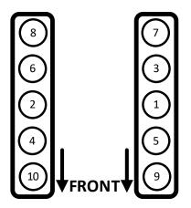
12. Torque the 10mm x 25mm HHFCS bolt you previously installed. Use a 16mm socket wrench. Torque to 30 ft-lbs.
