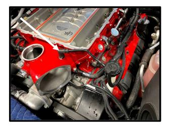
23. Connect the stock PCV hose to 15.82mm fitting previously installed.
