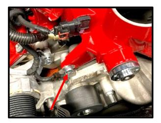
(Stock fuel rails) Apply grease to both orings on injectors. Reinstall factory locking clip to rail and injector to secure to rail (\*failure to do so could cause running issues). Mount stock fuel rail to supercharger using supplied (4x) 6mm x 14mm SHCS, apply light amount of Blue Loctite #243 to threads. Torque to 88 in-lbs using 5mm allen socket.
