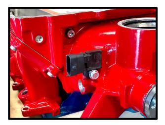
2. Install the post SC, post IC TMAP sensors (2x) in the back of the manifold using the supplied (2x) 6mm x 14mm HHFCS, torque to 88 in-lbs using 10mm socket.
