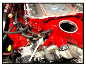
27. Install the supplied 22" MAP sensor extension to the passenger side (RH) MAP sensor connector (from front passenger side of engine) post SC, post IC (#4) connector 4-way (1 = blue/green, 2= blue/green, 3 = yellow/red, 4 = brown/blue). Route to the back of the intake manifold and connect to the passenger side (RH) TMAP sensor.
