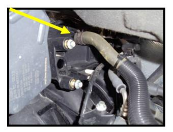
19. Pry the white plastic connector holding BEVIS electrical wires to intake manifold.
