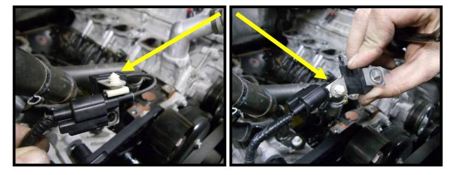
53. Install the supplied adjustable idler pulley bracket to the passenger side of engine as shown in image. Use the ([1 of 3] 8mm x 60mm SHCS) and the (1) 8mm AN washer to the capacitor hole and idler plate. Install capacitor to the backside of bolt and washer so that it's mounted against idler plate. Torque to 22 ft/lbs.
