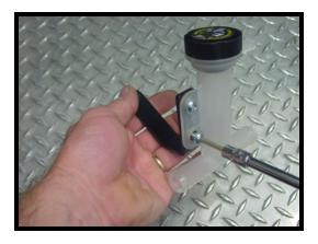
84. Install the intercooler filler neck to the passenger side valve cover. For the engines equipped with plastic valve covers, use the factory hole to mount bracket. Use the supplied (1) 6mm x 16mm HHFCS from the top side, secure the bottom side with the 6mm washer and 6mm nyloc nut to hold bracket. For engines equipped with the aluminum valve covers, use one of the factory 6mm studs to slide bracket over, secure with supplied 6mm washer and nyloc nut.
