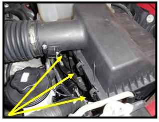
7. Disconnect the quick disconnect vent line from the passenger side of the air intake plenum. Disconnect vent line from valve cover as well. To release quick connect fittings, press tab clock-wise which will release fitting. The fittings will be used at a later step.
