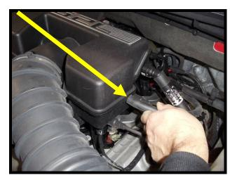
12. Disconnect the quick connect vent line from the driver side plenum. To release, press tab down and pull.
