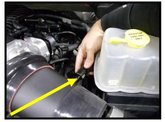
175. Install the 3/8" plastic barb fitting into the 3/8" ID rubber hose from the brake booster.
