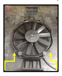
77. (Stage 2 heat exchanger install) Center fans side to side with the top bracket over the heat exchanger. Lift lower bracket and snap down into place. Repeat for second fan.
