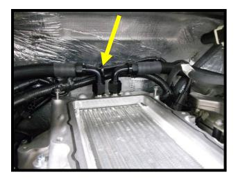
126. Reconnect the factory fuel feed line to the factory fuel rail by pressing until it clicks and locks.
