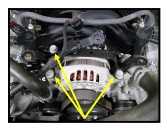
27. Remove alternator mounting bracket by removing the (4) mounting bolts (10mm socket).
