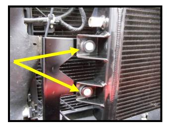
74. (Stage 2 heat exchanger install) Install the supplied adhesive backed rubber to mount surface on all four brackets.
