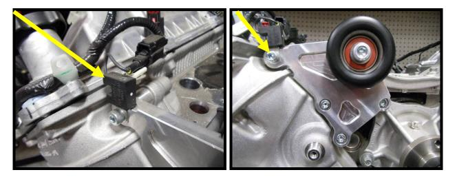
54. Install the supplied ([2 of 3] 8mm x 60mm SHCS) to the adjustable idler plate and timing chain cover on passenger side. Torque to 22 ft/lbs.
