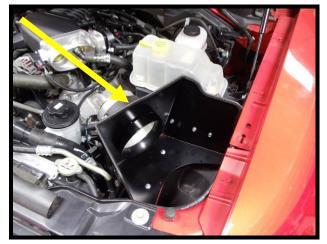
170. Install supplied air filter to the venturi ring using the supplied #104 hose clamp (5/16" nut driver). Position hose clamp so the nut area is hidden on the backside.
