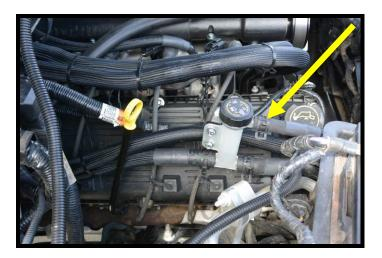
118. Route the 3/4" ID x 41" hose and the 3/8" ID x 40 ½" hoses from filler neck, and route down the frame rail, to the intercooler reservoir barb fittings. Secure with supplied pinch clamps. Secure hoses using zip-ties.
