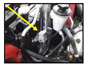
105. Run the 2-way connector and loom through the radiator support and plug connector to pump. Push connector on until it clicks and locks into place.
