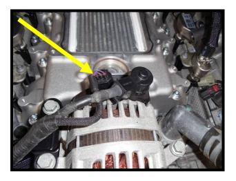
104. Mount the intercooler relay and fuse harness to the factory plastic loom coming down the radiator from main fuse box, driver side. Use a zip-tie to secure to loom.
