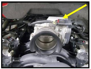
15. Pry the plastic connector holding the electronic throttle body wires to the intake manifold from manifold.
