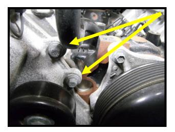
50. Remove the (1) nut from capacitor bolt on the passenger side using a 13mm wrench.
