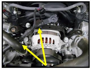
25. Carefully cut the electric tape holding the alternator wiring to the radiator shroud (plastic clip). Remove clip from radiator shroud.
