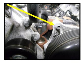
49. Remove the (2) bolts that secure the timing chain cover, passenger side (2) to block (10mm socket).
