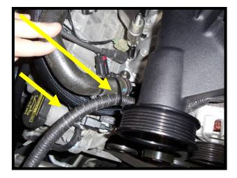
102. Reinstall the original factory ground wire to the alternator ground stud (13mm wrench). Press plastic cover back into place.
