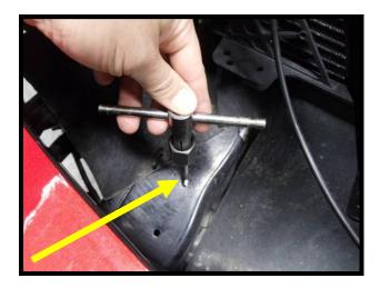
61. Remove the (2) bolts securing the headlights to the front clip as shown in image (10mm socket).
