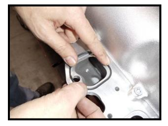
90. Remove the tape you installed to cover inlet ports. Clean cylinder head to manifold surface with carb cleaner.
