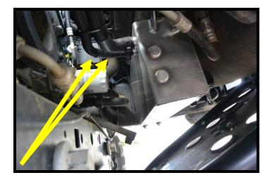
119. Route the dual 90 deg molded hose from the IC reservoir to the heat exchanger driver side fitting. Secure with supplied #16 pinch clamps.
