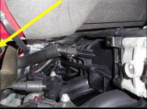
8. Loosen the hose clamp connecting the air intake plenum to throttle body using a flat head screw driver or 5/16" socket.
