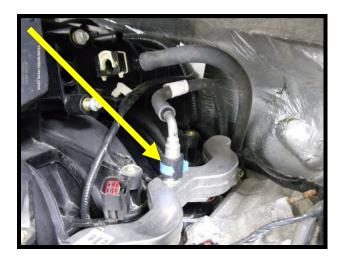
33. Remove the (4) mounting bolts holding the factory fuel rail on (8mm socket). Pull fuel rail from intake manifold.
