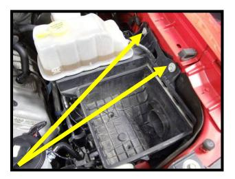
42. Remove factory air filter rubber shielding by prying out the (6) plastic push pins.
