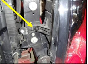
62. Route the passenger side heat exchanger bracket through the rubber shielding. Secure bracket with factory headlight/front clip bolt. Leave slightly loose for now.
