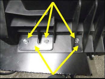
168. Install MAF element into MAF housing using supplied (2) 4mm x 10mm torx bolts. The sensor can only go in one way. Install MAF body to new air box as shown in image, use the (4) 6mm x 16mm SHCS and the plastic venturi from the inside of the air box (5mm allen). Torque to 95 in/lbs.
