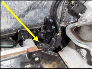
45. Remove heater hose tube from block by removing the (1) mounting bolt using an 8mm socket and pliers to remove clamp. There may be coolant left in this line, drain into clean bucket. This steel tube will not be reused. Remove tube from hose by using pliers to remove clamp.
