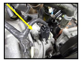
52. Remove white plastic clip from capacitor. Rotate capacitor and reinstall plastic clip as shown in image. This is for clearance when mounted to the idler plate.
