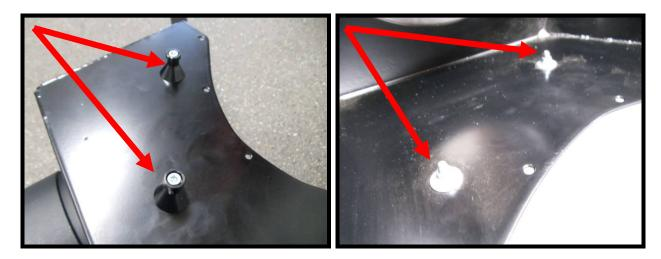
165. Install cut coolant reservoir to the new air box for mockup. Install factory bolt in the top support/fender. Hold the reservoir up against the air box and mark the (3) holes from the air box to the coolant reservoir. The measurements should be roughly 1 ¼" down from ledge, and the (3) holes should roughly be 1 ¾", 3 ¾", 6 ¾" from the ledge (fender side) as shown. Remove coolant reservoir and use a 1/4" drill bit to drill these (3) holes.
