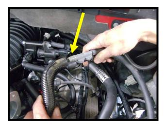
155. Install supplied 15/32" ID rubber hose by pressing hose end onto check valve assembly barb. Install 90deg fitting onto top 5/8" quick connect fitting installed on supercharger inlet.
