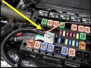
109. Pull the yellow 20amp fuse from position #78. Install the 20amp yellow fuse in the unused fuse slot on the fuse tap. Install the supplied fuse tap into position #78. Note: 20amp yellow fuse should be in bottom slot, 5amp should be in top slot.
