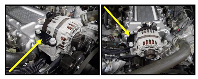
101. Pre-route the alternator ground wire and alternator 3-way connector along the heater line (this is for pulley/belt clearance). Use zip-tie to secure wires to heater lines for extra belt/pulley clearance. Note: Image shows with SC assembly installed to show best possible position.
