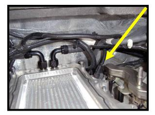
122. Install the throttle body 6-way extension harness to factory 6-way connector by pressing together until it clicks and locks. Lock the red safety lock by pressing until it clicks and locks.
