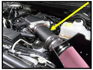
173. Install the 5/8" aluminum barb fitting into the rubber grommet installed in air inlet tube.
