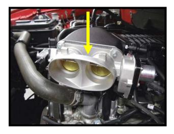
157. Route the throttle body 4-way connector under the throttle body and connect to throttle body TPS sensor. Connect by pressing together until it clicks and locks. Use a small zip-tie to secure throttle extension harness to factory harness.
