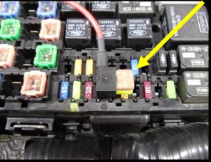
110. (Stage 2 heat exchanger installation) Connect the 12V eyelet to the factory power stud in the fuse box. Connect dual fan 2-way's to fan relay harness 2-way's. Zip tie wires for clean installation.
