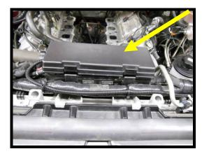
108. Run main power wire from intercooler relay harness (and stage 2 heat exchanger 12v turn-on) along radiator shroud (secure with zip-ties for clean installation) to the main fuse box. Come through the passenger side opening. Remove the factory nut from the power stud in the box. Install the power eyelet from the IC relay harness to this stud. Reinstall factory nut to the power stud until tight.
