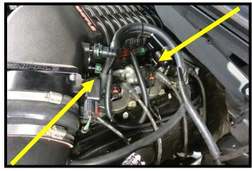
154. Remove rubber 1/2" ID hose from brake booster line and check valve assembly as shown.
