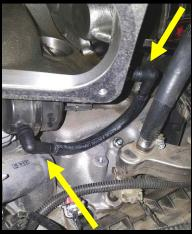
146. Install the supplied jack-shaft cover to passenger side of supercharger. Use the supplied (3) rubber grommets (insert into plastic cover 3 holes (1 is left empty) and (3) 5mm x 12mm BHCS. (2) go to the front holes, (1) goes to the back top hole.
