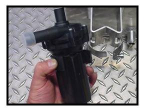
80. Install the pump to the IC reservoir tank and t-nut clamp you previously installed. Make sure the rubber strip stays in place. Face the pump with the outlet fitting directly forward and the inlet on the driver side. Install the reservoir to pump inlet hose, secure with supplied pinch clamps.
