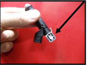
94. When installing the intake manifold, make sure to pull knock sensor wires to the passenger side, just behind the sensor as shown in the image.
