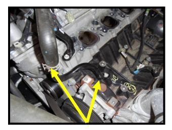
46. Install the supplied short steel heater hose tube to the factory location using the factory bolt (8mm socket). Torque to 106 in/lbs.
