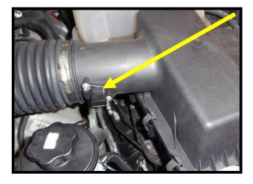
6. Loosen the factory air box lid by pushing the (3) locking tabs back. Lift air box lid from air box, this will not be reused.
