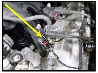
29. Disconnect spark plug wire from ignition coils (8) by pulling from ignition coil.
