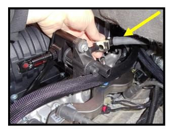
144. Connect the BEVIS 2-way electrical connector to BEVIS, push until it clicks and locks into place.
