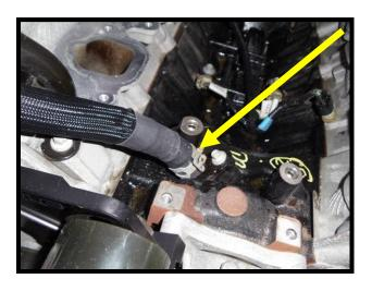
87. Secure both heater hoses using zip-ties for a nice clean installation.
