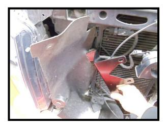
63. Install the supplied 8mm x 25mm flanged hex bolt (1 of 2) into passenger side of frame rail to secure bottom of heat exchanger bracket. Some models require the installation of the M8-1.25 clip on nuts, inserted into the open square hole. Sandwich the rubber shielding under the bracket to secure it. Carefully tighten bolt, be cautious of stripping the threads.
