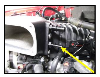
151. Use a razor blade to cut the factory shielding from the PCV line. Once removed, use a razor blade to carefully cut the factory quick connect fittings (1-90deg and 1-45deg) from the factory PCV tube. Note: There is an oring towards the bottom of the barb fitting, do not go through it. You can cut through the top area and then pry fitting out without ever touching the oring.
