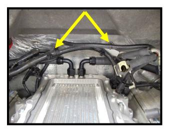
125. After pre-routing electrical wires towards the firewall, use zip-ties to secure wires together and then tuck behind the IC fittings/hose. This will allow the SC to slide into place easier. Make sure to pull wires towards driver side to give enough slack later.
