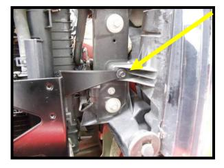
68. Install the supplied (4) rubber grommets to the heat exchanger mounts.
