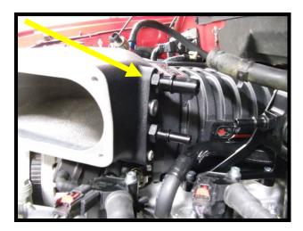
150. Install the –6AN to 3/8" barb aluminum quick connect fitting to the driver side of SC inlet, third hole from top.
