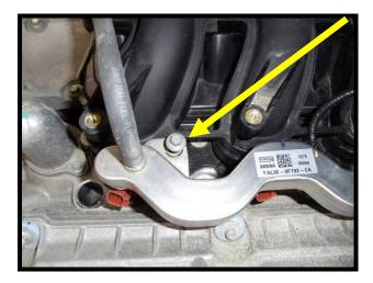
34. Remove the safety clips securing the fuel injectors to fuel rail by pulling away from open end. Remove fuel injectors from factory fuel rail, these will not be reused.
