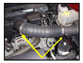
5. Remove the factory MAF sensor element from the factory air box lid. Utilize a T20 torx socket or wrench to remove. This will be installed later into the new MAF housing.
