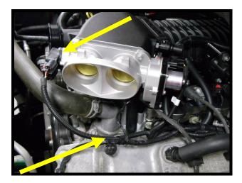
158. Connect the throttle body electronic control 2-way connector (extension) to electronic throttle motor. Push together until it clicks and locks into place.
