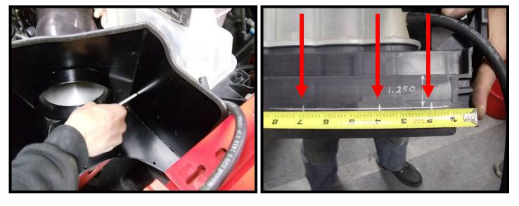
166. Remove the air box from engine bay for the coolant reservoir mounting.
