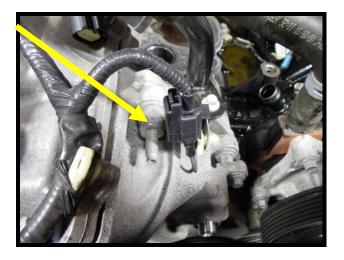
51. Remove the (1) capacitor bolt on the passenger side using a deep-well 18mm socket.
