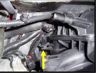
21. Using a ½" breaker bar, release tension from factory tensioner by rotating the breaker bar in a clock-wise rotation. Remove factory serpentine belt from engine once belt has extra slack.
