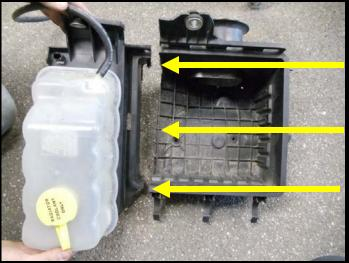
161. Mark the coolant reservoir back side straight across along the bottom supports. Cut straight across as shown in the image.
