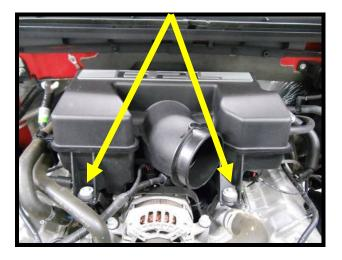
10. Release the factory rubber heater lines from factory plastic clamp on air intake plenum. To release the clamp, use a small pick through the side of it, press tab down and it will release.
