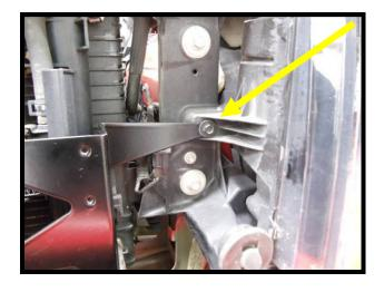
66. Install the supplied 8mm x 25mm flanged hex bolt (1 of 2) into driver side of frame rail to secure bottom of heat exchanger bracket. Some models require the installation of the M8-1.25 clip on nuts, inserted into the open square hole. Sandwich the rubber shielding under the bracket to secure it. Carefully tighten bolt, be cautious of stripping the threads.
