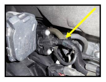
17. Remove BEVIS from engine by removing the (2) bolts (8mm socket). Disconnect quick connect fitting from BEVIS by squeezing white tabs on bottom of connector. The BEVIS will be reinstalled later in manual.
