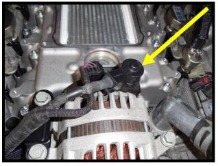
103. Reconnect alternator 3-way connector to alternator until it clicks and locks into place.
