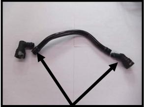
152. Install the 90deg and 45deg quick connect fittings from PCV tube to the new supplied 5/8" ID x 14" rubber hose. Connect the 90deg fitting back to passenger side valve cover, and connect 45deg fitting to Whipple fitting on passenger side of inlet. Push until it clicks and locks into place.
