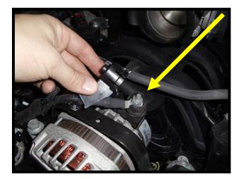
24. Pry plastic clips (3) from air intake plenum support bracket and alternator ground wire. Remove the alternator ground wire by removing the (1) nut (13mm socket). Cut these clips from the wiring harness, they will not be used.
