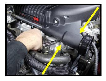
139. Torque the (1) 10mm x 30mm SHCS in the SC front support to 25 ft/lbs.
