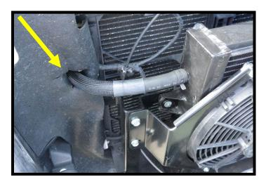
121. Pre-route the inlet air temp sensor 2-way connector to the driver side and connect to air temp sensor. This must go along the firewall to clear SC assembly.
