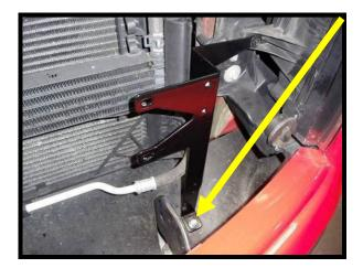
67. Carefully tighten the headlight/front clip bolt that secures the top of heat exchanger bracket on driver side (10mm socket). Be cautious of stripping the threads.
