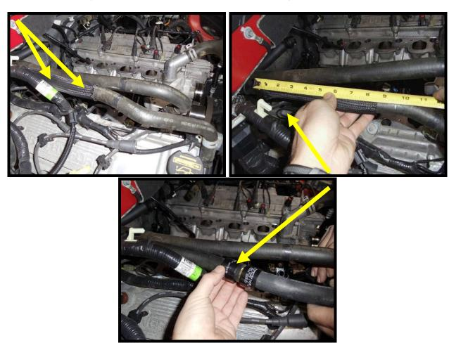
86. Route 3/4" ID rubber heater hose down along the line of other factory heater hose, install end onto previously installed 3/4" ID barb in the valley of the block. Secure with supplied #16 pinch clamp.
