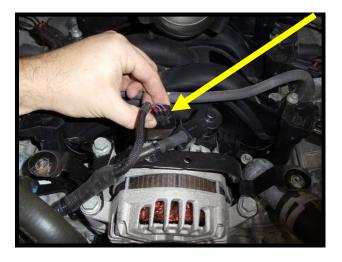
23. Open the plastic connector on the alternator ground wire. Using a 13mm socket, remove ground wire from alternator stud.
