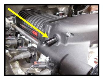
149. Install the -6AN to 5/8" barb (1 of 2) aluminum quick connect fittings to the driver side of SC inlet, top hole.
