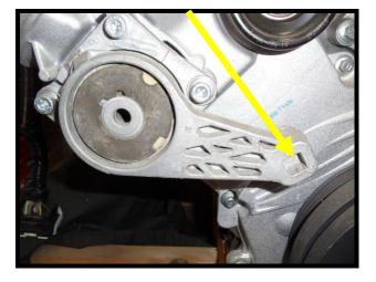
22. Disconnect the 3-way electrical connector from alternator. To unlock, squeeze connector and pull up.
