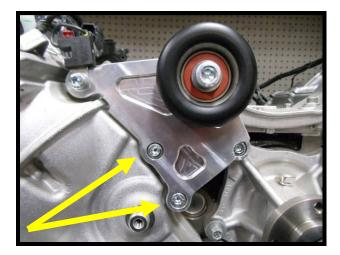
55. Install the supplied (1) 8mm x 50mm SHCS to the adjustable idler plate and water pump on passenger side.
