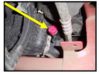
3. Disconnect the MAF (mass air flow) sensor connector. To release the connector, pull out the red locking tab, then squeeze the connector to release.
