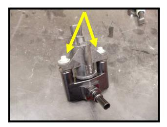
129. Install the BEVIS relocation assembly to the steel bracket using the supplied (2) 6mm x 18mm SHCS (5mm allen). Torque to 106 in/lbs.
