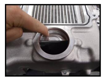
133. Pre-install (2) of the 8mm x 20mm 6-point bolts in the back 2 bolt holes. Insert these 6-point bolts 1 rotation as the SC assembly will be slid into position using these to locate it.
