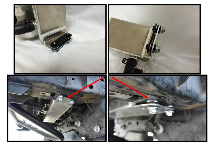
82. Mount the second intercooler reservoir support to the passenger side of frame rail. Use the supplied clip-on nut in the frame rail (8mm thread). Use the supplied (1) 8mm x 25mm hex head bolt with the 8mm washer to secure from bottom side through the clip-on nut. Torque to 120 in/lbs.
