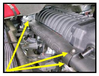
147. Install the supplied 3/8" ID x 51" fuel line hose with protective mesh covering to the factory cross-over barbs. Install on driver side first, by pressing onto barb and securing with supplied clamp (1 of 2) (7mm socket). Route behind the BEVIS relocation assembly and around the back of the SC (against firewall). Route along engine on passenger side and secure to passenger side fuel rail barb. Secure hose with supplied clamp (1 of 2) (7mm socket)
