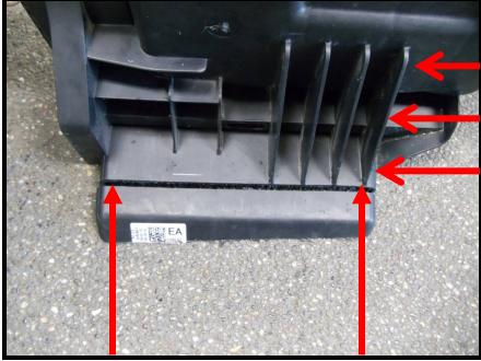
162. Cut/grind the front side of the coolant reservoir you previously cut, to a smooth flat surface as shown in the image.
