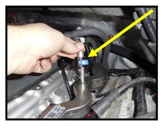
127. Install the supplied –6AN viton orings (4 of 4) to all the –6AN to 3/8" barb fittings. Install (1) of the –6AN fitting to 3/8" barb black fitting into BEVIS billet bracket.
