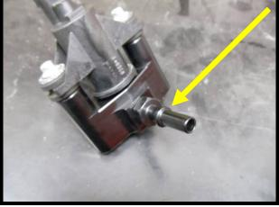
128. Install the BEVIS to the billet relocation bracket using the factory fasteners (8mm socket). Torque to 106 in/lbs.
