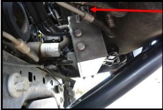
83. Locate the supplied intercooler filler tee, mounting bracket, and two 6mm flange button head cap screws. Assemble the filler tee to the mount using the two 6mm flange button head cap screws, torque to 80 in/lb.
