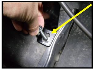
64. Carefully tighten the headlight/front clip bolt that secures the top of heat exchanger bracket on passenger side (10mm socket). Be cautious of stripping the threads.
