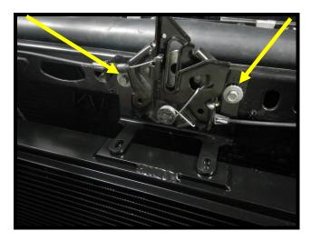
72. (Stage 2 heat exchanger install) Install heat exchanger upper mounting bolts using the (2) 6mm x 12mm HHFCS.
