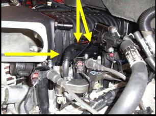
148. Install the –6AN to 5/8" barb (1 of 2) aluminum quick connect fittings to the passenger side of SC inlet.
