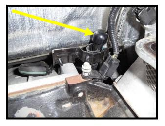
44. Remove the factory bolt (1) that secures the crank position sensor (8mm socket). Install the supplied (1) 6mm x 20mm low head socket cap using a 5mm allen wrench. Torque to 106 in/lbs.
