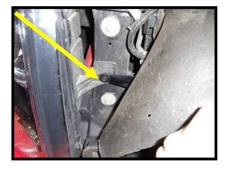
65. Install the driver side heat exchanger bracket to frame rail and headlight/front clip. Secure top with factory bolt but leave loose until bottom mount is started.
