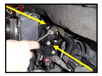
18. Remove the rubber brake booster hose from intake manifold by releasing hose clamp and pulling hose.
