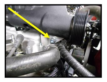
140. Reinstall the factory ignition coils using the (8) 6mm x 90mm SHCS (5mm allen), (8) 8mm AN washers and the supplied 1.75" billet spacers. Note: There are 4 driver side coils, 4 passenger side coils, do not mix up. Torque to 106 in/lbs.
