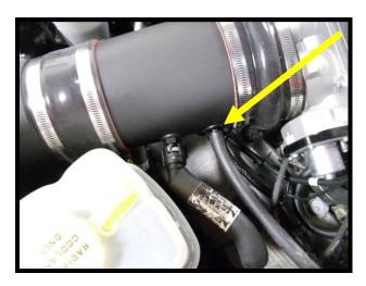
177. Install the coolant reservoir vent line down the fender, to the factory radiator fill cap.
