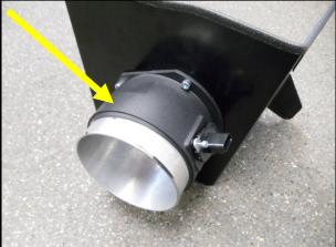
169. Mount the air box/coolant reservoir assembly back into factory location, locating on the (2) aluminum spuds into the rubber grommets.
