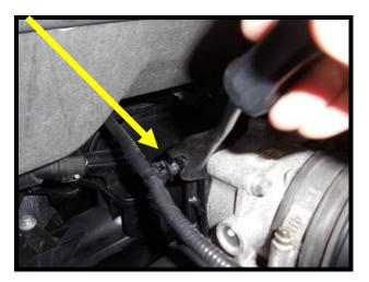
16. Disconnect the BEVIS electrical connector by pressing in the tab and pulling (tab on backside of connector). Then remove the quick connect fitting from BEVIS barb fitting. To unlock tab, release lock and pull towards firewall.
