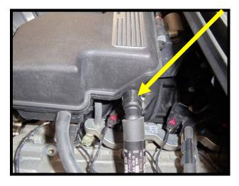
13. Lift the air intake plenum away from engine, this will not be reused.
