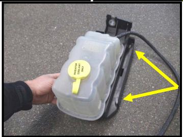
163. Cut/grind the back side of the coolant reservoir you previously cut, to a smooth flat surface as shown in the image.
