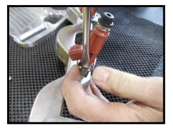
35. Using a razor blade, carefully cut the factory fuel crossover line at both barbs. Remove fuel line from fuel rail, this will not be used.
