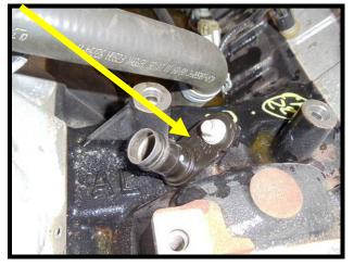
47. Remove factory 76mm idler pulley from passenger side of engine (above spring loaded tensioner) using a 13mm socket.
