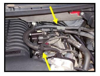
156. Install supplied throttle body to supercharger inlet along with the supplied throttle body gasket. Use the (4) 6mm x 25mm and (4) 6mm AN washers to secure throttle body to SC. Torque to 106 in/lbs.
