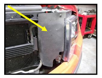
59. Remove (2) plastic push pins from passenger side rubber shielding from headlight/front clip as shown in image. The passenger side heat exchanger bracket will slide behind this.
