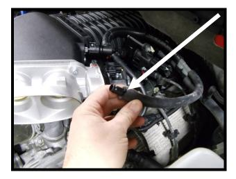
176. Install 3/8" rubber line from brake booster to air inlet tube and 3/8" plastic barb fitting.
