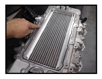
132. Apply light amount of grease on the manifold bypass oring, located in the 2.5" bypass hole. This is to help prevent ripping the oring during the installation process.
