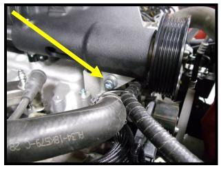
136. Install the BEVIS relocation assembly to the supercharger assembly using the supplied (2) 8mm x 25mm SHCS (hand tight).
