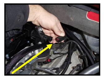
145. Connect the bypass valve's vacuum/boost actuator rubber hose by connecting the ¼" barb from the bypass actuator to the ¼" barb installed on the inlet just above it. Use the supplied (1) ¼" ID x 3" to connect the two barbs.
