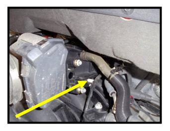
20. Pry plastic clips (4) from intake manifold on backside of engine, (2) passenger side and (2) driver side.
