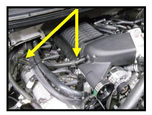
153. Install the supplied 3/8" ID x 15" rubber hose (with dual 90deg quick connect fittings) between the BEVIS and the 3/8" barb fitting on the SC inlet. Route underneath coil wires, push fitting over aluminum fitting until it clicks and locks into place.
