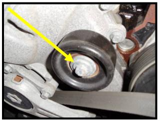
48. Remove the factory bolt that secures the water pump (1) to the block (10mm socket).
