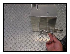
79. Wrap the rubber strip around the intercooler pump motor with the gap toward the outlet port side of the pump as shown.
