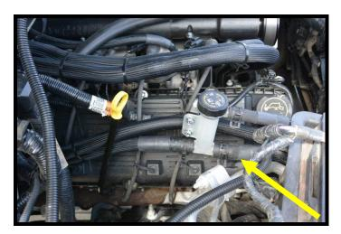
117. Install the 3/8" ID x 41" intercooler reservoir vent hose to the IC fill neck. Secure with supplied pinch clamp.
