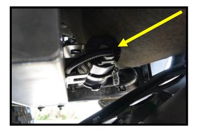
106. Remove the factory ground bolt from the frame rail (inner-side), very near the rubber air filter box grommets. Install the intercooler relay harness ground wire/eyelet (as well as Stage 2 heat exchanger relay ground) to this bolt and factory eyelet. Reinstall the factory bolt and secure to frame rail until tight.
