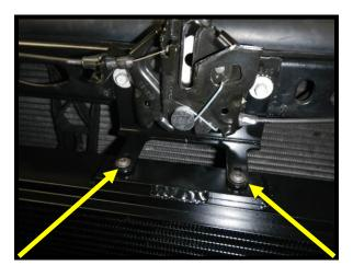
73. Install the heat exchanger to the heat exchanger brackets previously installed. The ¾" nipple will be on the bottom, driver side, and the 5/8" nipple will be on the top, passenger side. Use the supplied (4) 8mm nyloc nut to secure backside of the (4) 8mm x 35mm FHSCS bolts. Torque to 22 ft/lbs.
