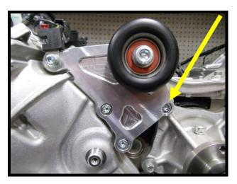
56. Reinstall the factory 76mm steel idler pulley to the factory location (13mm socket). Torque to 22 ft/lbs.
