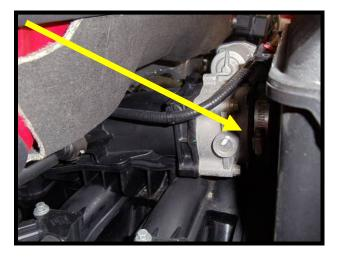
9. Using a 10mm socket, remove the bolts (2) securing the air intake plenum to the support bracket.
