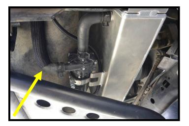
120. Route 3/4" ID x 64 ½" IC feed line through the rubber shielding between passenger side headlight and radiator, to the heat exchanger 3/4" nipple. Secure hose with supplied (1) #16 pinch clamp.
