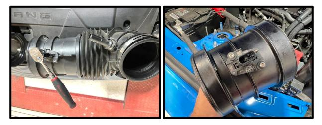
6. Using a small flat head screwdriver, remove the clamp securing fitting in air inlet tube. Using flat head screwdriver, remove the stock plastic fittings from air inlet tubes.
