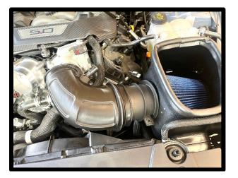
13. Install MAF housing bracket to airbox, using the (2x per) 4mm x 6mm bolts and 3mm allen. Secure MAF housing to bracket using stock fastener and 10mm socket.
