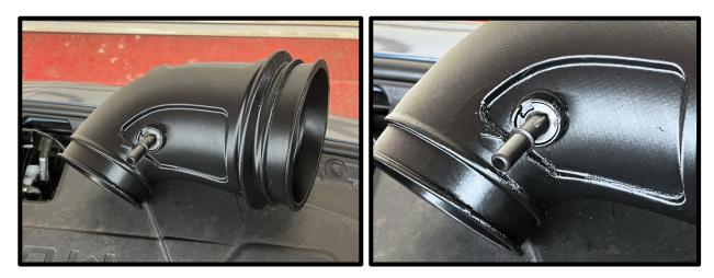
8. Remove stock airbox snorkel from air cleaner assemblies. Transfer to new airboxes.
