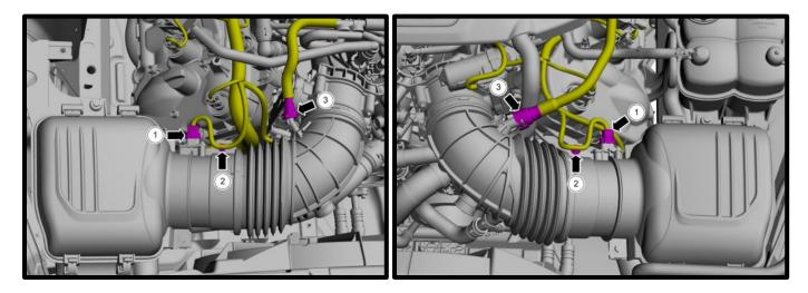
3. Remove the airbox lid bolt using a 10mm socket. Release the locking tabs and remove the airbox lid.
