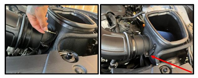
14. Secure air inlet tube to MAF using #80mm hose clamps. Secure air inlet tube to throttle body using #64mm hose clamps.
