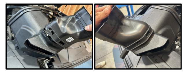
9. Install the airbox trim seal pieces to the new airbox top flange. Start in the middle, rear of box for a clean installation. **NOTE:** RH requires trim seal to be shortened 1/2" using cutting shears.
