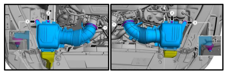
5. Remove the MAF sensor using a 10mm socket. Install factory MAF sensors to the new MAF housing using supplied (4x) 4mm x 10mm SHCS. Torque to 17 lbs-in. **\*\*DO NOT USE STOCK BOLTS\*\*. \*NOTE: Verify arrow position for airflow direction.**
