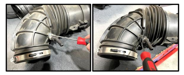
7. Install the stock fittings into the supplied inlet tube, orient them in the same stock positions by lining up the gaps.
