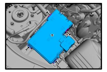
2. Disconnect the MAF sensors, MAF sensor retainers and remove make up air hose from air tubes.
