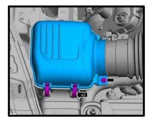
4. Loosen the hose clamps from throttle bodies using nut driver. Remove the air cleaner bolts. Detach the air cleaner boxes from grommets and remove the air cleaner assemblies.
