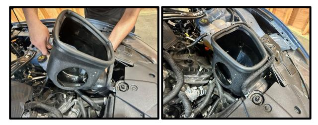
11. Set the air filter into the airbox, slide MAF housing through airbox. Slide the air filter over MAF housing. Secure with supplied clamp using 5/16" nut driver.
