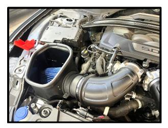
15. Reconnect factory PCV and fresh air connections to air inlet tube fittings.
