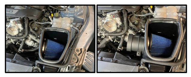
12. Install new air inlet tube from MAF to throttle body. Leave loose for now.
