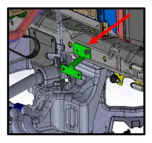
119. Mount IC pump clamp to the pump bracket using (2x) 6mm x 8mm HHFCS bolts. Install pump to clamp, pump inlet should be facing the front of the vehicle. Leave loose until IC hoses are installed.
