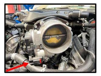
139. Install supplied (1x) ½" to 15.82mm hose adapter to the SC inlet tube (for make-up air).
