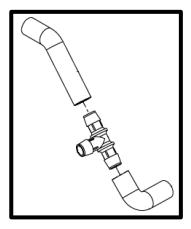
126. Install hose #3103411 from TEE forward facing fitting (outlet). Secure hose to TEE fitting using supplied #16 Black worm clamp. Route #3103411 across front of the motor to **RH forward** most IC fitting. Secure hose to tee with #16 Black clamp. Zip tie both this and the feed line that goes in the same path together.
