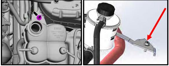
117. Mount IC reservoir to bracket using (2x) 6mm x 12mm HHFCS.
