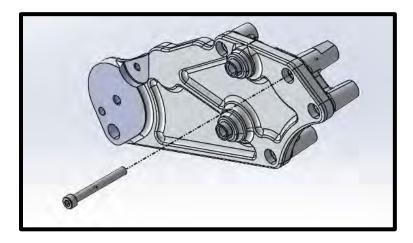
794. Torque (10x) 6mm HHFCS manifold bolts in the following pattern using a 10mm socket. First pass: 88 lbs-in. Second pass: 106 lb-in. **NOTE:** For bolt #10, a ¼" socket with 4"-6" extension, 10mm wobble is the best possible tool to get into this tight area.
