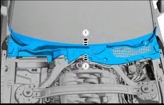
149. Install the (6x) push pins (1), (2x) retainers (2) and the clips (3) (2x).
