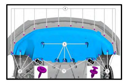
162. **(GT ONLY)** Install the (12x) fasteners to front chin splitter, torque to 18 lb-in.
