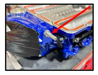
108. Mount EECPV bracket to SC lid, use (2x) 6mm x 10 HHFCS. Torque to 80 lbs-in using 10mm socket. Slide EECPV to bracket. Connect factory plastic quick connect fitting to EECPV until it clicks and locks in place. Connect 2-way electrical connector to EECPV, press locking tab back in place.
