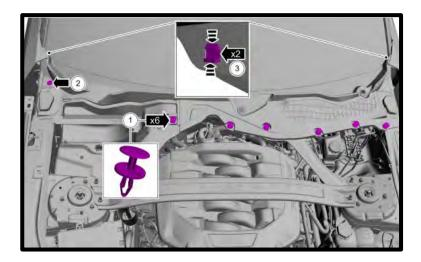
28. Remove the (5x) push pins (1) and depress the (2x) clips (2). Lift and then pull cowl panel grille out and remove.
