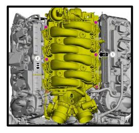
46. Disconnect the engine wiring harness electrical connectors and detach the retainers. Remove intake manifold.
