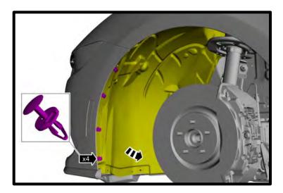
9. (DARK HORSE) On both sides, remove the (4x) fasteners and (6x) push pins from front fender splash shield.
