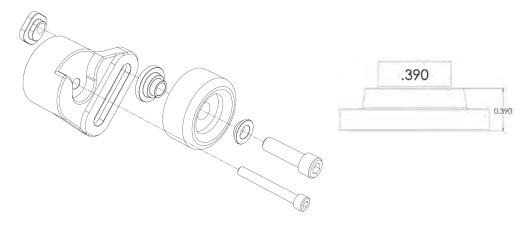
68. Assemble spring-loaded tensioner by mounting supplied spacer with female register to tensioner. Install grooved idler pulley (#36326) to tensioner and (.390") step spacer. Use supplied step washer to front face of pulley bearing and (1x) 10mm x 40mm SHCS (10-Rib uses 10mm x 60mm SHCS) bolt. Use light amount of anti-seize on threads. Torque to 18 lbs-ft. NOTE: Verify you're using the proper spacer as shown.
