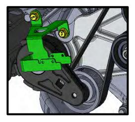
72. **(Auto Transmission)** Mount trans cooler solenoid to the supplied bracket using (4x) stock fasteners. Connect supplied extension harness to factory harness and connect to solenoid.
