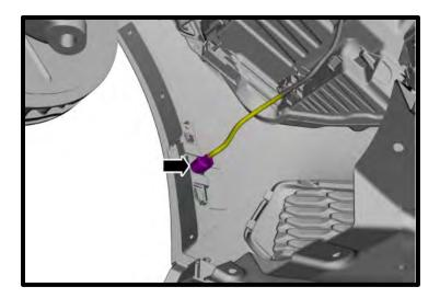
160. (GT ONLY) Install the (22x) fasteners and (3x) push pins, torque to 18 lb-in.
