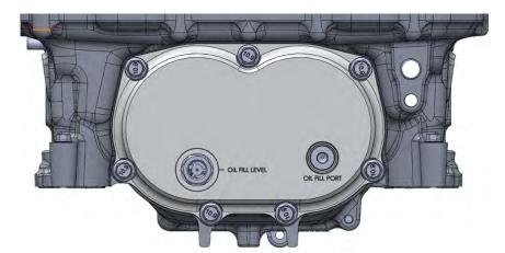
92. Install supercharger housing (without lid) to the engine. Use the supplied (4x) 6mm x 45mm HHFCS on the outer bolt holes and (6x) 6mm x 75mm HHFCS bolts with the supplied (6x) #2-009 orings on the bolt, under the head to
