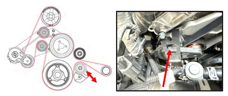
98. With belt holding the SC pulley in position, torque the supercharger (5x) 6mm x 15mm SHCS bolts to 130 lbs-in using a 5mm allen socket. Do not use Loctite on threads, it is not required.
