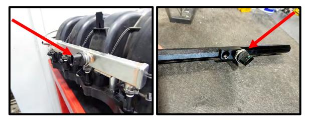
76. Install supplied (2x) #2-906 Viton oring to (2x) 45mm long 9.49mm fuel fittings. Apply light amount of grease to oring for ease of installation and install fitting. Install fittings, one per rail.
