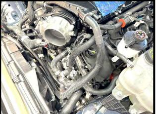
124. Install hose #3103405 from rearmost IC filler reservoir fitting to the top IC pump fitting (inlet). Use supplied #16 pinch clamps to secure hose.
