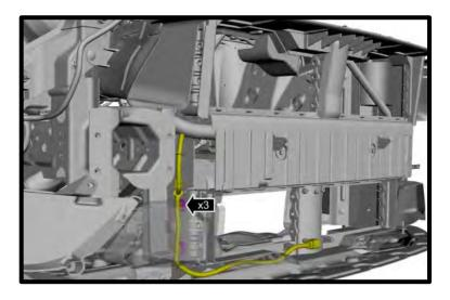
152. If equipped, reconnect the CCM wiring connector.
