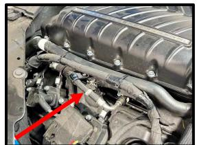
105. Connect factory fuel inlet line to the driver side fuel fitting, press until it clicks and locks in place.
