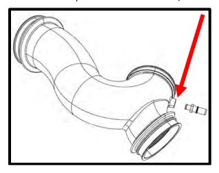
140. Install factory MAF sensors to the new MAF housings using supplied (4x) 4mm x 10mm SHCS. Torque to 17 lbs-in. \*\*DO NOT USE STOCK BOLTS\*\*. \*NOTE: Verify arrow position for airflow direction.
