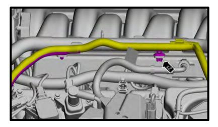
39. Detach the heater hose retainer. Remove the heater hose from both driver and passenger side of block by pulling locking tab back and pulling away. Position the heater hoses aside.
