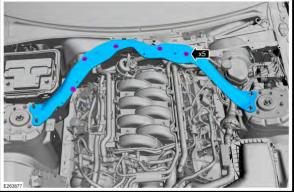
148. Install the (5x) push pins (1) and depress the (2x) clips (2).
