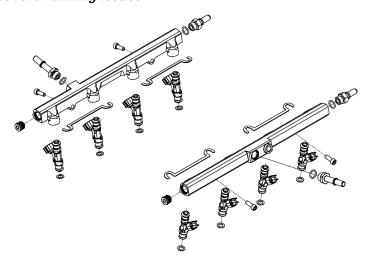
80. Apply generous amount of grease to injector orings for ease of installation. Install supplied fuel injectors, rails and lock bracket to intake manifold, secure with the (4x) 6mm x 16mm SHCS using a 5mm allen socket. Use **Blue Loctite** #243 on the threads of each bolt. Torque to 90 lbs-in.
