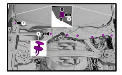
150. Install the (6x) bolts and position active grille shutter **SHELL ONLY (shutter grilles are NOT reused)**. Torque to 71 lb-in.
