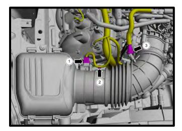
34. Loosen the hose clamp from throttle body using nut driver. Remove the air cleaner bolt. Detach the air cleaner from grommets and remove the air cleaner.
