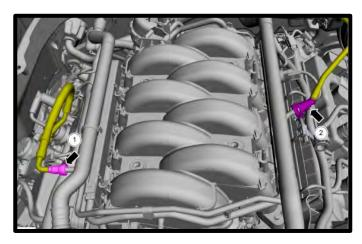
41. Remove the (4x) nuts from the top of the intake manifold, remove heater hose supports.
