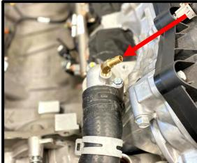
57. Trim the reservoir vent line right at the ENG printing on hose. Reinstall stock hose to new fitting. Secure with supplied #4 clamp.
