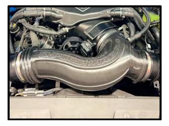
145. Install supplied ½" x 13 ¼" make up air hose to the LH valve cover. Push until it clicks and locks into place. Install other end to air inlet tube fitting previously installed.
