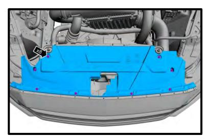
157. On both sides, install front bumper cover to fender with original push-pin and the bolts. Torque to 44 lb-in.
