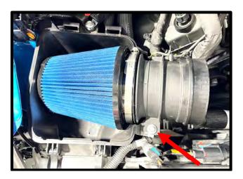
143. **(Stage 1)** Install the inlet tube to the MAFs and throttle body. Secure using the supplied clamps, (2x) #80 on MAF side and (1x) #64 to throttle body. Reconnect MAF connectors to MAF sensors.
