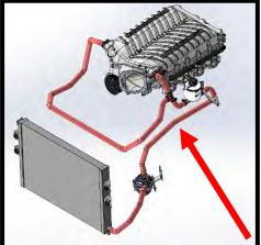
125. Install hose #3103406 from **LH forward** most IC fitting (outlet). Secure hose to IC fitting with #16 Black worm clamp. Install TEE fitting with TEE facing forward. Install supplied 90deg hose #3103158 to end of TEE and secure to front most IC filler reservoir fitting (inlet). Secure 90deg hose to tee and reservoir with #16 Black clamps.
