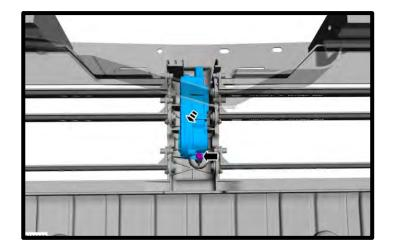
27. Remove the (6x) push pins (1), (2x) retainers (2) and depress and remove the clips (3) (2x).
