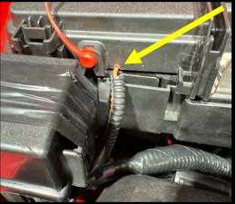
134. Using a 10mm socket, remove the 12V (+) power stud nut from the far post. Install the IC pump relay power eyelet (red wire) to the 12V stud. Use a 10mm socket to secure stock and IC power wire.
