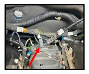
89. Install supplied wiring plug (1x) to the **LH** throttle electrical connector. Zip-tie harness away from belt system.
