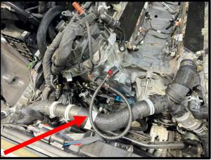
86. Remove plastic harness retainers from loom at the back of the engine.
