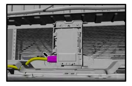
153. Reinstall airbox air ducts with stock retainers (4x per side).
