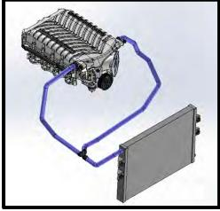
123. Install hose #3103410 from offset Y, across front of engine to **LH rear** most IC fitting (inlet). Use supplied #16 silver worm clamp to secure hose to tee and #16 Black clamp to IC fitting. **NOTE:** Routing IC hose incorrectly can result in poor performance and potential damage!
