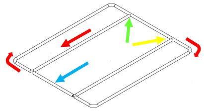
100. Install supplied pre-formed 65.3" x .103" oring to the top sealing surface of the SC housing. Apply generous amount of grease to help ease the oring into place. **TIP:** To install oring into dove-tail groove, press vertically, vs sliding finger along.
