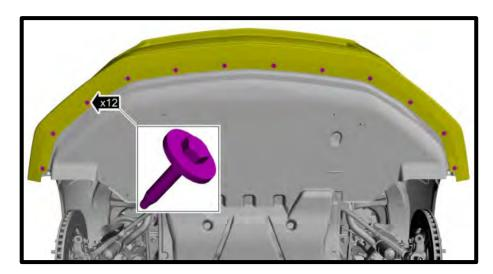
163. (**DARK HORSE**) On both sides, install the (4x) fasteners and (6x) push pins to front fender splash shield, torque to 18 lb-in.
