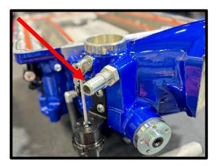
111. Install supplied 1/2" ID x 9" hose (#3103159) to the passenger side valve cover. Connect other end to supercharger inlet quick connect fitting. Push until it clicks and locks into place.
