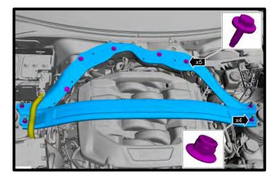
30. (RIGHT HAND DRIVE ONLY) If equipped, remove the strut tower brace by detaching the battery wire retainer. Remove the (4x) nuts and (6x) bolts. Reinstall factory nuts (4) and torque to 41 lbs-ft.
