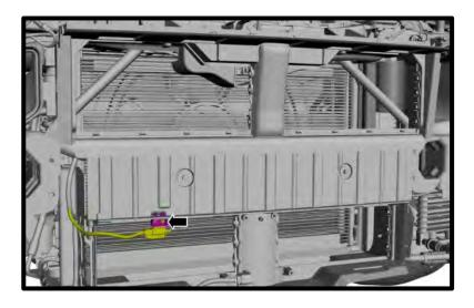
155. Install the (7x) fasteners from fascia.
