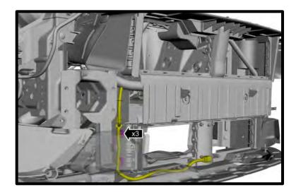
21. Remove the (6x) bolts and position active grille shutter forward.
