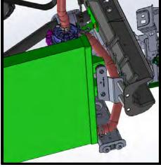
121. Install hose #3103409 from LTR **RH top** (outlet) fitting. Route to frame rail next to airbox snorkel. Install offset Y to end of hose. Use supplied #16 pinch clamps to secure hose.
