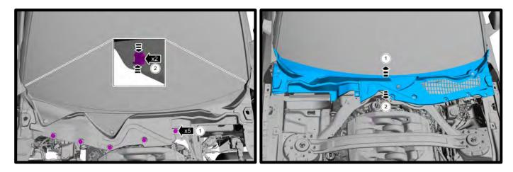
29. **(LEFT HAND DRIVE ONLY)** If equipped, remove the strut tower brace by detaching the battery wire retainer. Remove the (4x) nuts and (5x) bolts. Reinstall factory nuts (4) and torque to 41 lbs-ft.
