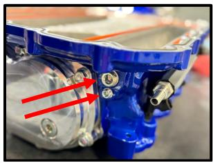
75. Using 27mm socket, remove the fuel PSI sensor from the factory fuel rail. Using 27mm socket, remove fuel PSI sensor from factory fuel rail. Install factory fuel PSI sensor to the fuel rail using a 27mm socket. Torque to 53 lbs-in, then an additional 25-degree rotation. **NOTE: Never use sealant on these threads.**
