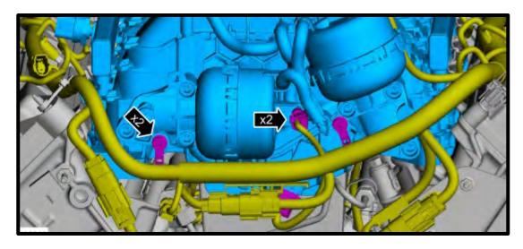
47. Remove and discard the (2x) foam inserts in the valley of the block. Clean the intake manifold to cylinder head surface using carb cleaner or acetone. Install tape over the exposed ports until manifold installation.
