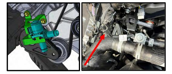
73. Install supplied (2x) smooth aluminum idler pulleys (**#3102717**) to the idler plate. Secure using the (2x) step washer through front of bearing and (2x) ½"-13 x 1 ¾" SHCS (with light amount of anti-seize on threads) bolts. Torque to 30 lbs-ft. using a 3/8" allen socket.
