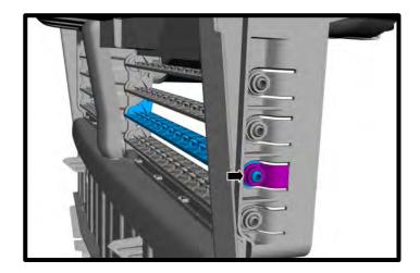
26. **(Vehicles equipped with active shutter grilles)** Remove the bolt and the active grille shutter actuator. **NOTE:** These are no longer used.
