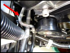
70. Install the spring-loaded tensioner to idler plate, locating the tang into position. Secure with the supplied (1x) 10mm x 60mm SHCS. Use light amount of anti-seize on threads. Torque to 25 lbs-ft.
