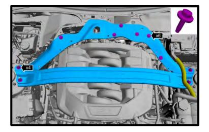
31. Lift and remove cover from the engine.
