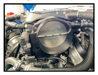
138. Connect previously installed throttle extension pigtail to the throttle body electrical connector. Secure wiring using zip-tie. **NOTE: Failure to secure wire may result in the wire catching the belt system!**
