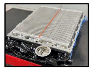
84. Install supplied 3-bar temperature manifold absolute pressure (TMAP) sensor to the front of the intake manifold using the supplied (1x) 6mm x 20mm SHCS with (1x) 6mm AN washer, apply light amount of Blue Loctite #243 to the threads. Apply generous amount of grease to oring for easy installation. Torque to 65 in-lb.
