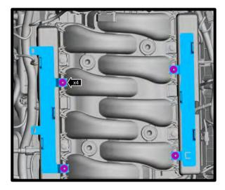
42. Remove the left and right fuel rail insulators, these will no longer be used.
