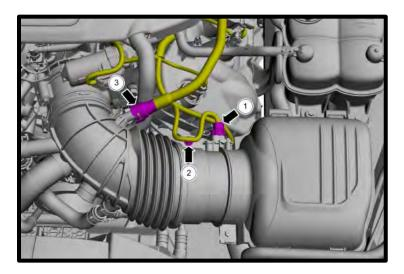
36. Loosen the hose clamp from throttle body using nut driver. Remove the air cleaner bolt. Detach the air cleaner from grommets and remove the air cleaner.
