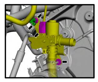
60. Remove stud from engine timing cover, this will not be reused.
