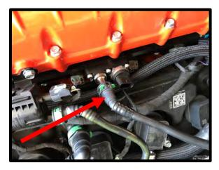
106. Connect the factory fuel PSI sensor connector to sensor, press safety lock until it clicks and locks in place.
