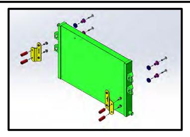
115. Slide the LTR assembly up from the bottom. Connect the LTR brackets to the coupling nuts using the supplied (4x) 8mm x 16mm hex headed flanged bolt (12mm ratchet wrench).
