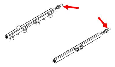
79. Install fuel injectors to the fuel rail, apply generous amount of grease to oring for easy installation. Install supplied fuel injector position lock bracket to clock the supplied fuel injectors into proper position. While installing lock bracket, secure fuel injectors so it doesn't add pressure to injector body. **CAUTION**: *Failure to clock the injector correctly can cause severe running issues*.
