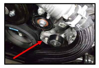
51. Remove the water pump pulley using a 10mm socket (this will be reused).
