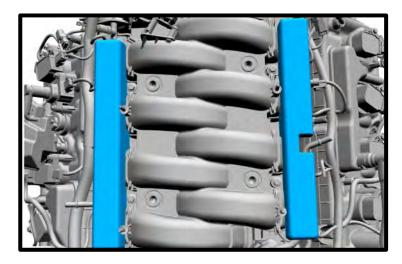
43. Loosen the (4x) bolts holding the fuel rails down, these go through to the cylinder head (10mm socket). Fuel rail does not need to be removed.
