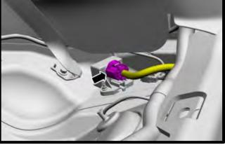
5. Locate the battery. Remove the plastic cover, (1) retaining clip and (3) retaining nuts for battery access. With an 8mm wrench disconnect both (-) battery cables from battery. Make sure the cables are far enough away from the battery that it does not accidentally touch the battery and make connection during installation.
