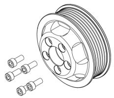
96. Reinstall water pump pulley using a 10mm socket, torque to 14 lbs-ft.
