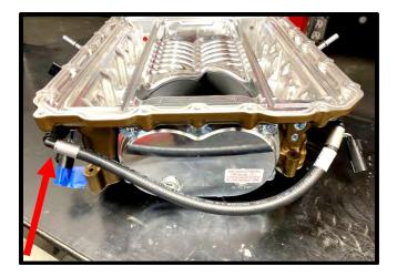
82. Install supplied ¼" ID bypass actuator to bypass nipple and ¼" 90deg nipple on SC inlet. **CAUTION:** Do not open/close bypass actuator by hand. This may damage actuator internally. It only moves properly with equal vacuum/boost at the actuator reference port.
