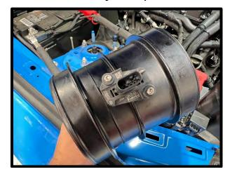
141. Install supplied filters to MAF housing, secure using supplied filter clamp. Install the MAF housings into the Y tube (for ease of installation), pre-install #80 hose clamp to Y tube, leave loose until later.
