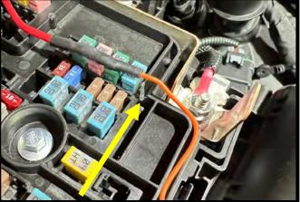
133. From fuse tap, route to slot you previously made. Route to stock slot at the front of fuse box. Add small relief in lid for wire as it comes out of the box. use small file to clean up and round edges. Test fit lid and ensure it does not interfere with this wire. Failure to route properly will lead to IC pump operation failure, resulting in poor performance.
