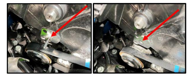
61. **(Auto Transmission)** Remove the U shape hose from the factory tee's. Cut 1 3/4" from the long end as shown.
