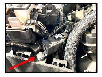
130. Locate stock ground wire stud, located on RH side of vehicle, next to strut tower brace using an 8mm socket. Install intercooler relay harness ground eyelet (black wire) along with factory ground wire. Reinstall bolt using an 8mm socket.
