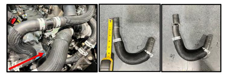
62. (Auto Transmission) Connect U shape hose back to stock tees, install/position to FRONT side of radiator hose (this stops it from getting to water pump pulley. Rotate the factory hose retainer and connect to this hose to secure in place.
