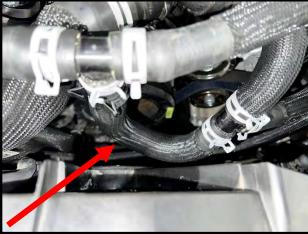
63. Using 5/16" nut driver, secure hose using supplied #24 hose clamp. Rotate the clamp at water neck towards the **LH** side for future clearance of the SC.
