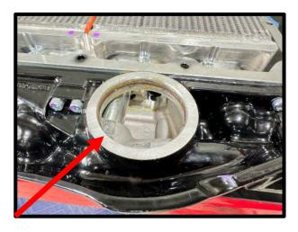
102. Apply generous amount of grease to the (1x) #2-230 Viton bypass oring. Install the supercharger lid to the supercharger housing by carefully placing the bypass down. Secure the SC lid using the (17x) 6mm x 30mm HHFCS and (3x) 6mm x 70mm HHFCS (*marked green*) using the following pattern. Torque to 90 lbs-in using an 8mm socket.
