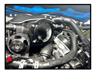
136. (Stage 1 92mm TB) Install supplied (1x) #2-045 V75BR oring to TB adapter. Install the supplied throttle body using the (4x) 6mm x 35mm HHFCS bolts using a 10mm socket.
