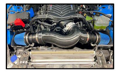
144. **(Stage 2)** Install inlet tube to the MAFs and throttle body. Secure using the supplied clamps, (3x) #80. Reconnect MAF connectors to MAF sensors.
