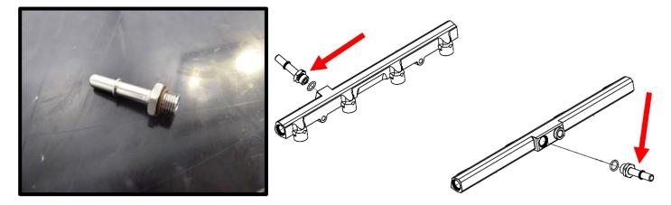
77. Apply light amount of grease to -6 ORB plugs, install the supplied (2x) -6 ORB plugs to front fuel rail ports.
