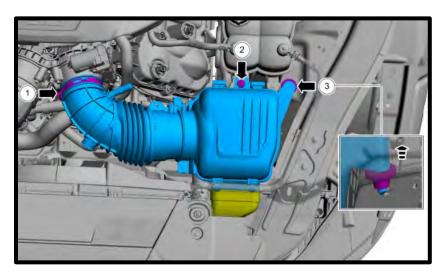
37. Disconnect the electronic throttle electrical connectors by pushing up on the safety lock and then squeezing the connector and pulling away. Remove the harness retainer from manifold.
