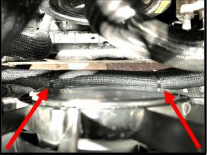
127. Secure supplied 3/8" 90deg hose to IC filler reservoir top barb using #4 hose clamp. Route down and secure hose to 3/4" IC pump feed hose using zip tie. Route down away from engine.
