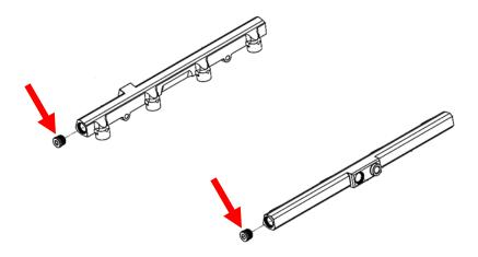
78. Install supplied (2x) #2-906 orings to (2x) -6 ORB to 9.49mm short fittings. Install the (2x) fittings into rear side of fuel rails. Apply light amount of grease to oring for ease of installation. Using a ¾" wrench (or ¾" deep socket) on both the front and rear fittings, tighten both.
