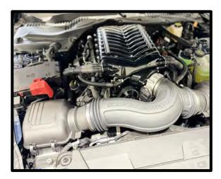
147. Reinstall the K-Brace over the studs and into position on the vehicle. Install the (2x) nuts on the studs and torque to 25 Nm using a 15mm socket. Install the (5x) mounting bolts and torque to 25 Nm using a 13mm socket. Reinstall the (7x) pushpin retainers on the cowl trim panel.
