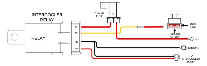
129. Mount relay and fuse holder to the factory airbox stock fastener, secure with zip-tie. Route 2-wire connector down, below radiator, along sway bar to the LH side of the vehicle. Connect to IC pump. Secure harness using zip-ties along bottom of vehicle.
