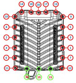
103. Install (4x) 2-117 IC fitting orings to the (4x) IC fittings. Apply grease to the (4x) 2-117 IC fitting orings. Slide fittings into lid. Secure fittings with supplied fitting retainer bracket and (2x) 6mm x 12mm SHCS bolt. Torque to 80 in-lbs.
