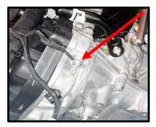
66. Use supplied (4x) 8mm x 90mm in the (3x) lower holes to secure the idler plate to the front of the **RH** side of engine, install hand tight. Using a 6mm allen, torque to 22 lbs-ft.
