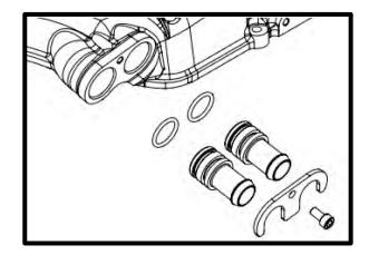
104. Connect factory passenger side rail fitting to the DI pump factory hose, press until it clicks and locks in place. NOTE:
