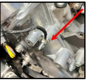
65. Using 10mm socket, remove the stock fastener (1x) from the top of the RH timing chain cover. Relocate stud with ground wire to the top timing chain cover location. Torque to 22 lbs-ft.
