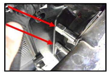
114. Install the LTR brackets to the LTR using the supplied (4x) 8mm x 35mm FHSCS bolts through the aluminum heat exchanger spuds (5mm allen socket). NOTE: HD heat exchanger mounts the same way but the inlet fitting moves to RH side (same as outlet).
