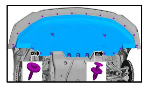
12. (DARK HORSE) Remove the (24x) fasteners and (3x) push pins from underbody shield.
