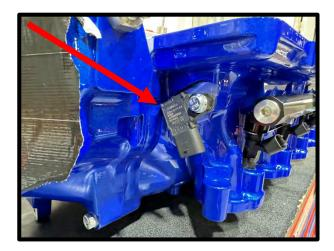
85. Install supplied electronic throttle pigtail to the factory **RH SIDE** electrical connector. Push until it locks in place, then lock the safety lock. Route to **LH** side of vehicle for later connection to throttle body. **TIP:** When pressing together, hold the wires and connector to ensure the wires cannot come loose during connection.
