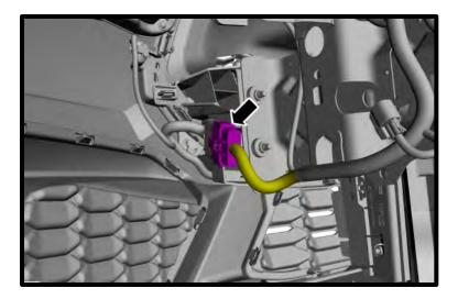
15. On both sides, remove the front bumper cover to fender push-pin and the bolts.
