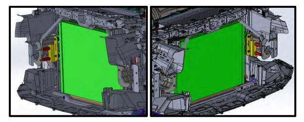
116. Remove factory coolant reservoir fastener. Install supplied reservoir bracket and secure on top of coolant reservoir. Secure using supplied (1x) 6mm x 20mm HHFCS. Torque to 71 in-lbs.
