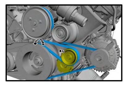
50. Remove the spring-loaded tensioner from the engine using a 13mm socket.
