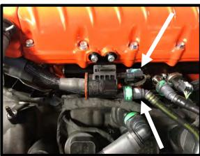
109. Install supplied 3/8" ID x 5 ½" with 55deg quick connect fitting hose (#5000030) to the EECPV barb fitting and **LH** quick connect fitting on SC inlet. Push until it clicks and locks into place.
