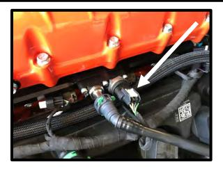
107. Install (1x) #906 oring to the supplied (1x) -6 ORB to 9.89mm quick connect fitting. Install fitting to the **LH** side port using an 11/16" socket.
