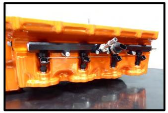
81. Install supplied 3/8" fuel cross over line around back of the supercharger by pressing until they click and lock in place. \*NOTE: The 90deg end goes to LH side.
