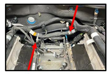
87. Install supplied TMAP pigtail to stock connector at rear of engine. Route to **LH** side of vehicle for later installation to supplied 3-Bar TMAP sensor.
