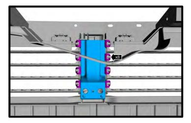
25. **Vehicles equipped with active shutter grilles**) Release the tab and remove the vane. **NOTE:** These are no longer used.
