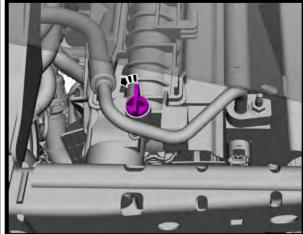
33. Disconnect the MAF sensor, MAF sensor retainer and remove make up air hose from air tube.
