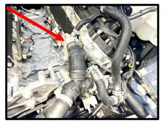
64. Using 10mm socket, remove the (3x) factory fasteners from the timing chain to head cover and (1x) from water pump (for new idler plate), this includes the factory ground wire/eyelet.
