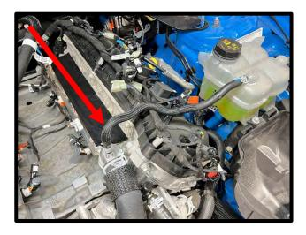
55. Loosen water Y junction. Remove water neck by removing the (2x) fasteners.
