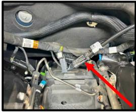
88. Install supplied IMRC electrical connector plugs (2x). Zip-tie to harness.
