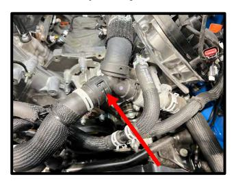
56. Transfer stock oring from stock water neck to new water neck. Apply pipe sealant to threads of 1/8" NPT to 5/16" 45 Deg fitting. Install fitting to water neck, rotate so it ends facing directly towards driver side. Install water neck to motor using stock fasteners (10mm socket), torque to 89 lbs-in.
