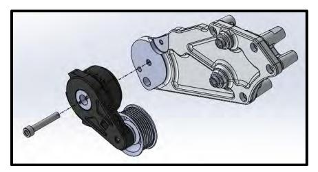
71. (**Auto Transmission**) Install supplied trans cooler solenoid bracket to the tensioner plate and engine block using (2x) 8mm x 20mm HHFCS. Torque to 120 in-lbs. \*\*Manual transmission based vehicles, discard this bracket.
