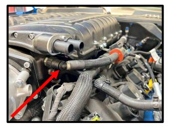
110. Install (1x) supplied #906 oring to the (1x) -6 ORB to 15.82mm quick connect fitting. Install fitting to **RH** side on the inlet using a 7/8" socket.
