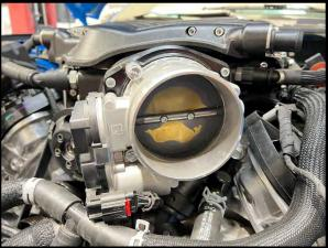
137. (**Stage 2 Whipple 112mm TB**) Install throttle body to supercharger inlet, use the supplied gasket. Secure TB with the supplied (4x) 6mm x 45mm SHCS using 5mm allen socket. Torque to 89 in-lbs.
