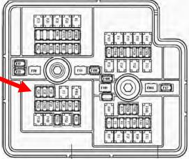
132. Use small set of cutters or file, make a small notch in fuse box cover lid and fuse box to allow wire to fit. use small file to clean up and round edges
