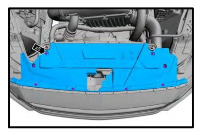
17. Remove the (7x) fasteners from fascia. Carefully pull the fascia forward.
