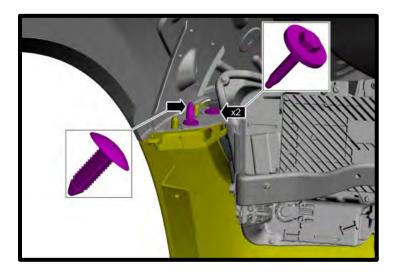
158. Connect the front bumper cover electrical connector.
