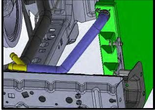
122. Install hose #3103408 from offset Y straight to **RH rear** most IC fitting (inlet). Use supplied #16 silver worm clamp to secure hose to Y and #16 Black clamp to IC fitting. **NOTE:** Routing IC hose incorrectly can result in poor performance and potential damage!
