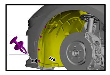
164. On both sides, install the (4x) fasteners to body side front shield, torque to 18 lb-in.
