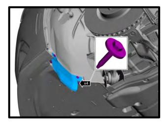
8. (GT ONLY) On both sides, remove the (4x) push pins and position aside the front fender splash shield.
