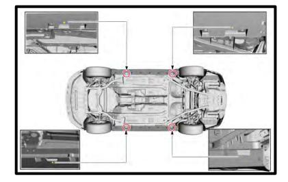
7. On both sides, remove the (4x) fasteners from body side front shield.
