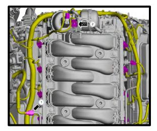
45. Loosen the (6x) manifold to cylinder head bolts using an 8mm socket. Position the manifold up and towards the front of the engine to access the rear of the manifold.
