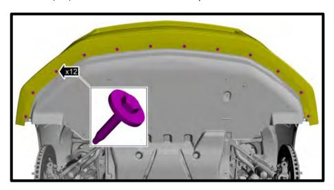
11. **(GT ONLY)** Remove the (22x) fasteners and (3x) push pin from the underbody shield. Remove shield from vehicle.
