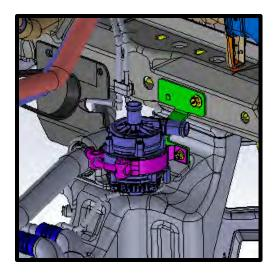
120. Install hose #3103407 from IC pump to LTR **LH low** (inlet) fitting. Secure using supplied #16 pinch clamps. Tighten IC pump clamp.
