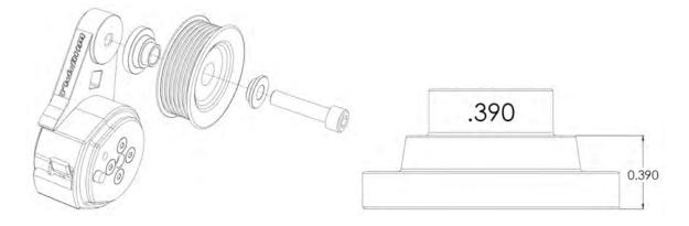
69. Carefully bend the factory AC line down and towards **RH** side. Install spring loaded tensioner to plate to check clearance. You should have a minimum of 3/8" of clearance from the tensioner to the AC line.
