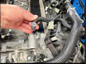
58. **(Auto Transmission)** Release the hose clamp from transmission fluid valve and hose facing down from tee. Remove plastic hose retainer from oil cooler solenoid hose.
