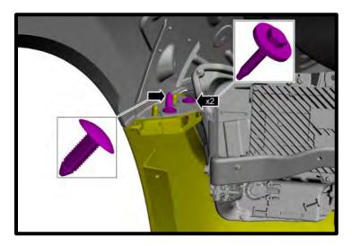
16. Remove the radiator sight shield by removing the (8x) push pins. Use a flat head screwdriver to pry the center head up. These will all be reused.
