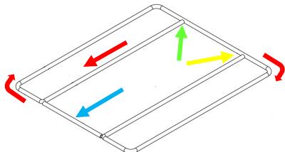
67. Install the supplied pre-formed 65.3" x .103" oring to the top sealing surface of the SC housing. Apply generous
