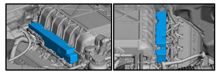
18. Disconnect all (8) fuel injectors and fuel pressure sensor electrical connectors.
