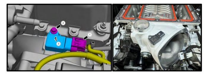
81. Install throttle body to supercharger inlet, use the supplied gasket between TB adapter and SC inlet. Secure with the supplied (3) 6mm x 25mm SHCS and (1) 6mm x 50mm SHCS using a 5mm allen socket. Torque to 106 lbs-in on first pass, 135 lbs-in in a cross-pattern. \*NOTE: Failure to torque properly can cause throttle related issues.
