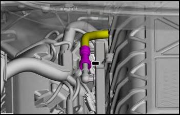
20. Detach the retainer securing fuel line to SC assembly, then remove fuel line from engine.
