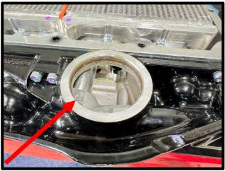
69. Apply generous amount of grease to the (1x) #2-230 Viton bypass oring. Install the supercharger lid to the supercharger housing by carefully placing the bypass down. Secure the SC lid using the (17x) 6mm x 30mm HHFCS and (3x) 6mm x 70mm HHFCS (*marked green*) using the following pattern (install EVAP bracket to 1 and 7). Torque to 90 lbs-in using an 10mm socket.
