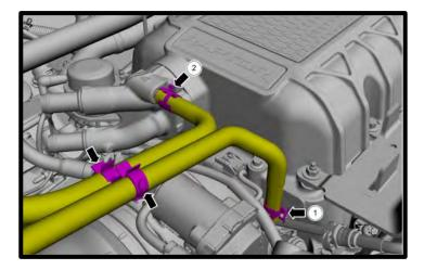
14. Disconnect the PCV line from RH valve cover and SC.
