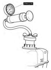
92. To pressurize the cooling system, slowly press the plunger of the pressure test pump and increase the pressure to between 124 - 138 kPa (18 - 20 PSI). Observe the gauge reading for approximately 2 minutes. Pressure should not drop during this time. If the pressure drops within this time, inspect for leaks and repair as necessary. **NOTE:** If no leaks are found and the pressure drops, the leak may be internal to the intake manifold.
