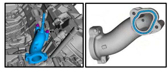
37. Install new water neck into stock location. Secure to cylinder head using the (1) 6mm x 30mm and (1) 6mm x 50mm SHCS. Secure to stock thermostat housing using factory fasteners. Get all parts hand tight before torquing. Torque the (2) nuts to 89 in-lbs first. Follow by torquing stock water neck bolts to 89 in-lbs.
