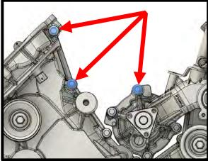
34. Install idler plate to engine using the (1) 8mm x 65mm HHFCS, (1) 8mm x 60mm SHCS and (1) 8mm x 55mm SHCS bolts to secure to timing chain cover. **Leave loose for now**.
