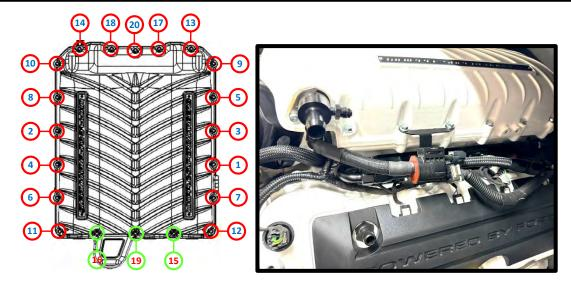
70. Install the (3x) supplied 6AN viton orings (#2-906) to the (1x) -6 ORB to 9.89mm, (1x) -6 ORB to 15.82mm and (1x) -6 ORB plug supplied. LH side, install the 9.89mm fitting in the top port using a 11/16" deep socket or wrench. LH side, install (1x) 6 ORB plug to the lower port using a 6mm allen socket. RH side, install (1x) 15.82mm fitting to port using a 7/8" deep socket.
