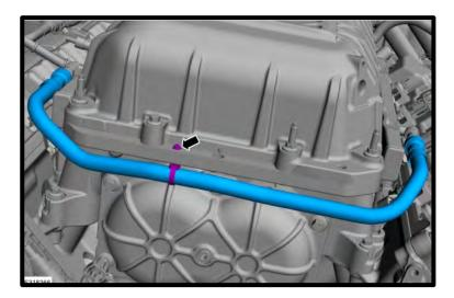
21. Remove the supercharger from engine by removing the (6) supercharger assembly bolts and (4) bolts from fuel rails (10mm socket).
