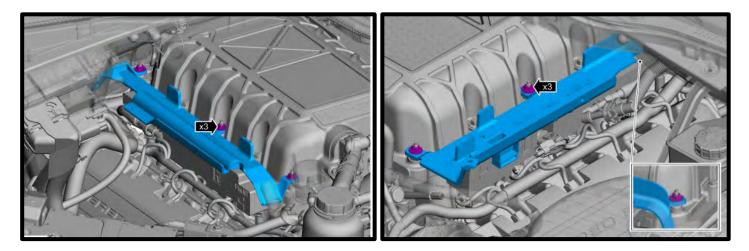
17. Remove the fuel rail insulator from both banks.
