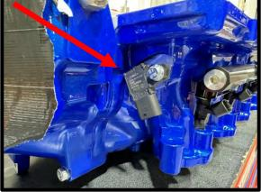
44. Install the supplied TMAP pigtail to the 3-Bar TMAP supplied, wrap up to SC inlet as this will get connected to stock harness later.
