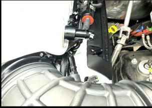
75. Install the 1/8" NPT to 6AN fitting to the IC outlet fitting. Apply light amount of pipe Teflon to pipe fitting.
