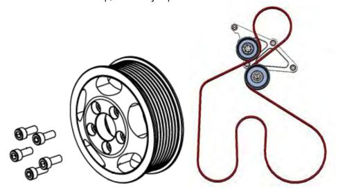
65. With the belt holding the SC pulley in position, torque the supercharger (5x) 6mm x 14mm SHCS bolts to 130 lbs-in using a 5mm allen socket. Do not use Loctite on threads, it is not required.
