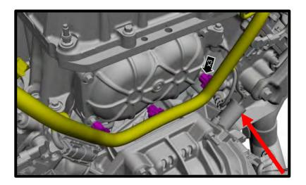
23. Disconnect the TMAP sensor from supercharger lid and TMAP (SIP) sensor from supercharger inlet. Remove both sensors from supercharger assembly for installation to new supercharger. **NOTE:** Do not mix up sensors.
