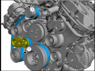
32. Remove the (3) water pump pulley bolts and water pump pulley (10mm socket).
