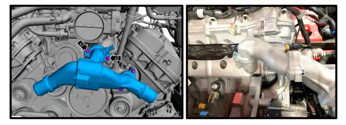
38. Apply light amount of thread sealant to threads of supplied 1/8" NPT to 5/16" fitting. Install fitting into new water neck, rotate to face LH side of engine.
