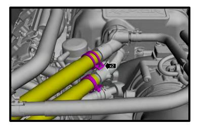
13. (1) Disconnect the hose clamps and the retainer, then position aside the hose. (2) Disconnect the supercharger cooling circuit hose clamps and retainers. These hoses will not be reused.
