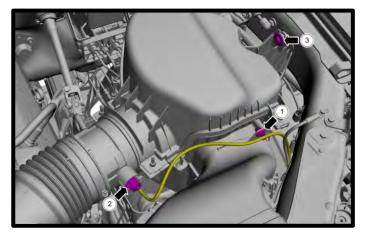
9. Disconnect the crank case vent tube and bypass vacuum line from inlet tube. Loosen clamp at throttle body. Remove the airbox mounting bolt and remove airbox assembly.
