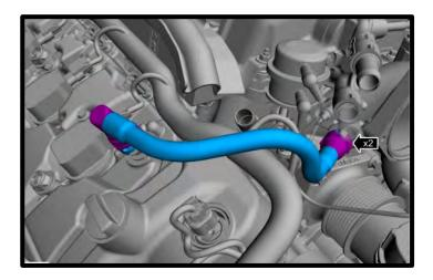
15. Cut and discard the OEM zip ties from radiator hoses. Detach retainer from coolant hoses from retainers. Detach quick connect fittings. Detach the LH and RH heater hose at the cowl panel and position hoses aside.
