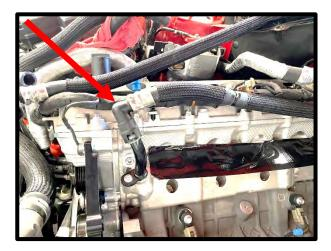
26. Remove factory ground wire by removing nut, using 10mm wrench. Relocate to valve cover bolt. Torque to 89 inlbs.
