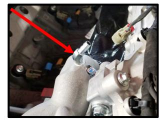
40. Remove stock coolant temp sensor from factory thermostat housing. Install supplied plug to factory location. Install coolant temp sensor in new water neck (needed for throttle body clearance).
