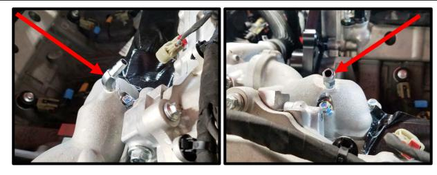
39. Preinstall stock vent hose to the 45deg fitting in water neck, secure using stock clamp. NOTE: This will later be routed to engine degas bottle.
