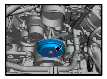
63. Reinstall stock accessory belt by releasing tension on spring loaded tensioner.
