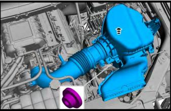
10. Disconnect throttle body electrical connector and coolant temp sensor, then detach the wire retainer.
