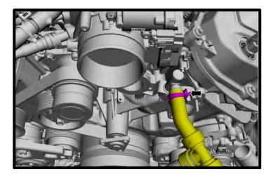
25. Disconnect RH heater quick connect fitting from water neck. Remove the heater tube from the engine.
