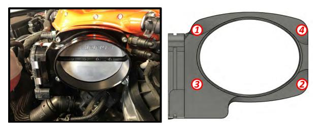
82. Separate the SIP sensor and electronic throttle harness by using razor blade to cut electric tape on stock harness, install supplied split loom, secure with automotive grade electric tape. Secure ETC and SIP sensor connectors.
