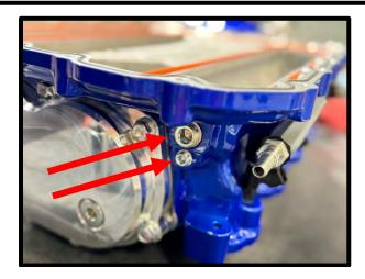
47. Install the supplied (8) manifold orings to the Whipple intake manifold to cylinder head surface, apply light amount of grease to ease installation.
