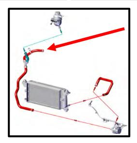
79. Reconnect factory vent line to degas bottle using stock clamp.
