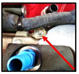
27. Install the #2-113 oring to the supplied heater tube and apply light amount of grease to oring. Install the heater tube to engine and secure using the supplied fork and stock fastener. Torque to 89 lbs-in.
