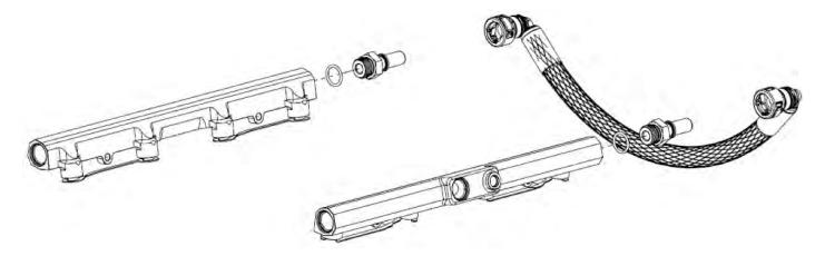
60. Install the supplied (1x) #2-906 Viton oring to the 45mm long -8 ORB to 9.49mm inlet fitting next to fuel PSI sensor. Apply light amount of grease to oring for ease of installation.
