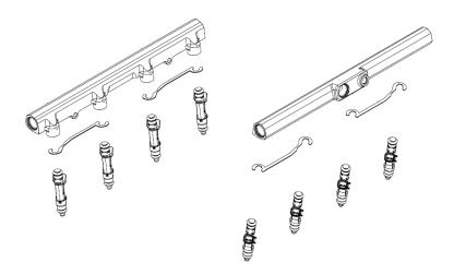
58. Apply generous amount of grease to the injector orings for ease of installation. Install the fuel injectors, rails and lock bracket to the intake manifold, secure with the (4x) 6mm x 16mm SHCS using a 5mm allen socket. Use **Blue Loctite #243** on the threads of each bolt. Torque to 90 lbs-in.
