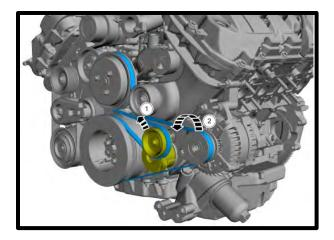
64. Install the supercharger pulley using the supplied (5x) 6mm x 14mm SHCS using a 5mm allen socket. **Leave hand tight until after belt installation**. Install the supplied supercharger belt by following the routing diagram. The spring-loaded tensioner should be 100% full open. Once in position, lock the adjustable idler pulley by torquing the
