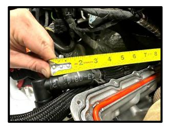
29. Install the ¾" hose coupler to the stock heater hose. Install supplied molded hose with the 90deg bend to ¾" barb. Slide 2 shrink clamps around hose/coupler. Test fit hose to heater tube previously installed. Once hose is verified, use heat gun to shrink clamps at coupler. Use supplied #16 worm clamp to secure heater hose to heater tube.
