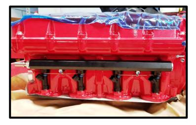
59. Install the supplied 1/2" fuel cross over line around the back of the supercharger by pressing until they click and lock in place.
