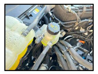
77. Using the ¾" x 10" hose, cut the factory feed hose (after IC coolant temp sensor), install supplied ¾" hose barb and (2x) shrink clamps. Apply heat to shrink clamps. Install supplied sleaving and heat shrink to cover hose. Connect hose to RH IC fitting, secure with supplied black #12 worm clamp.
