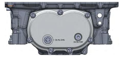
49. Install the supercharger housing (without lid) to the engine. Use the supplied (4) 6mm x 45mm HHFCS on the outer bolt holes and the (6) 6mm x 75mm HHFCS bolts with the supplied (6) #2-009 orings on the bolt, under the head. Use **Blue Loctite #243** on the threads of each bolt. Leave hand tight for now.
