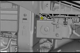
8. Detach the retainers from the air cleaner. Disconnect the IAT sensor electrical connector.
