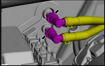
16. Remove the (6) nuts from SC lid, then remove the hose supports from both sides.
