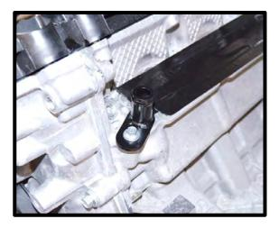
28. Move the clamp back from RH heater hose fitting. Cut approximately 1 ½" from end of hose as shown.
