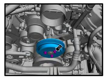
33. Remove stock idler pulley from engine using a 15mm socket. Using 13mm socket, remove the stud from timing cover. Using 10mm socket, remove the (2) stock bolts from timing cover and water pump.
