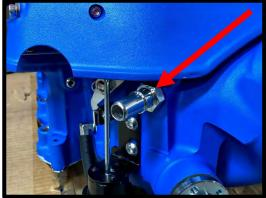
71. Connect the supplied PCV line from RH valve cover and SC.
