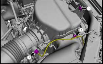
85. Connect the new inlet air tube between the airbox and throttle body. Secure using stock clamp on airbox side and supplied #80 hose clamp. Reconnect the crank case vent tube and bypass vacuum line from inlet tube.
