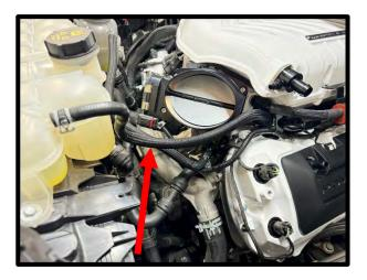
80. Using the previously removed stock TMAP sensor, install stock SIP sensor to Whipple inlet. Apply grease to oring to ease installation. Secure using supplied 5mm x 18mm HHFCS bolt. Torque to 72 in-lbs.
