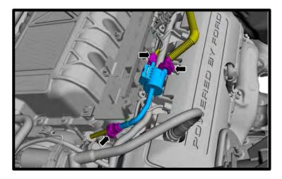
12. Mark each factory intercooler hose for future reference. Top is inlet, bottom is outlet. Remove both hoses from barbs and push aside.
