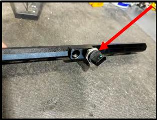
55. Install the (2x) #2-908 Viton oring to the (2x) -8 ORB to 8 AN plugs, install in front side of fuel rails.
