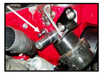
74. Install the (1x) 2-123 oring to each IC fitting. Apply light amount of grease to orings. Install fitting with 1/8" NPT port to LH fitting port. Install fitting with no port to RH side of lid. Secure fittings with forks and (1x) 6mm x 15mm SHCS per fitting. Torque to 89 lbs-in. Install the IC outlet fitting with 1/8" NPT port facing rearward on the LH side.
