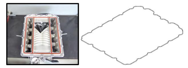
68. Install the (1x) #2-230 internal bypass oring to the lid bypass passage. Use generous amount of grease to secure oring in place and help with installation.
