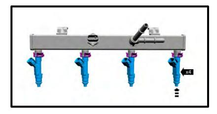
54. Using a 24mm socket, remove the fuel PSI sensor from the factory fuel rail. Using a 24mm socket, remove the fuel PSI sensor from the factory fuel rail. Install the factory fuel PSI sensor to the fuel rail using a 24mm socket. Torque to 53 lbs-in, then an additional 25-degree rotation. **NOTE: No sealant on the threads.** Connect factory electrical connector to sensor.
