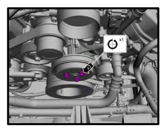
31. Rotate the accessory drive belt tensioner counterclockwise and remove belt. Rotate the supercharger belt tensioner clockwise and remove supercharger belt. Remove belt from engine.
