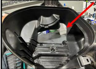
84. Reinstall stock airbox into stock location. Install new supplied air filter element. Reconnect the retainers from the air cleaner. Reconnect the IAT sensor electrical connector.
