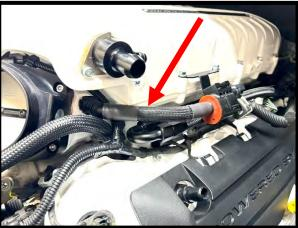
73. Apply light amount of pipe Teflon to supplied 1/8" NPT to ¼" barb fitting. Install fitting to the open port on the SC inlet (vacuum source). Install the supplied ¼" ID premade hose to the bypass actuator barb and ¼" fitting on SC inlet (goes over PCV fitting). **CAUTION:** Verify hose can't kink or bend.
