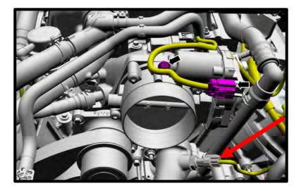
11. Disconnect the EVAP solenoid quick release coupling, release the valve from its bracket, then move out of the way.
