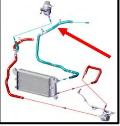
78. Using the ¾" x 19" 90deg hose, cut the factory return hose, install supplied ¾" hose barb and (2x) shrink clamps. Apply heat to shrink clamps. Install supplied sleaving and heat shrink to cover hose. Connect hose to LH IC fitting,
