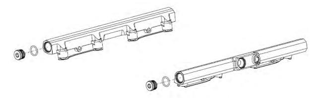
56. Install the supplied (2x) #2-908 Viton oring to the (2) -8 ORB to 12.61mm fittings. Apply light amount of grease to oring for ease of installation. Install fittings into rear fuel rail ports.
