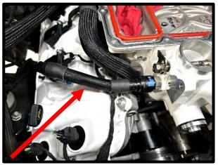
72. Slide the EECPV to bracket by sliding onto bracket. Connect factory plastic quick connect fitting to EECPV until it clicks and locks into place. Connect 2-way electrical connector to EECPV, press locking tab back in place. Install the supplied 3/8" ID x 5 ½" with 55deg quick connect fitting hose (#5000030) to the EECPV barb fitting and **upper** quick connect fitting on SC inlet. Push until it clicks and locks into place.
