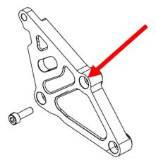
51. Torque the (10) 6mm HHFCS manifold bolts in the following pattern using a 10mm socket. First pass: 88 lbs-in. Second pass: 106 lb-in. **NOTE:** For bolt #10, a ¼" socket with 4"-6" extension, 10mm wobble is the best possible tool to get into this tight area.
