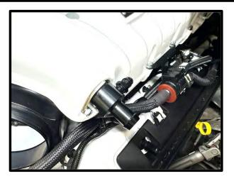
76. Install the -6 150deg push lock fitting to -6 fitting on the LH IC outlet hose. Install the supplied 3/8" x 32" hose to fitting and route to degas bottle. Secure to degas bottle using factory clamp.
