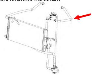
93. Install supplied ¾" hose with 90deg end to heat exchanger top fitting. Route other end to **BANK 1 (INLET)** intercooler fitting. Secure with supplied constant tension clamps. \***NOTE**: Make sure the hose does not and cannot kink during routing. **DO NOT** lay the hose on the cam sensor wires, this will lead to failure over time.
