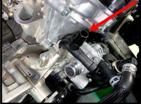
74. Install the supplied 3/8" ID with 55deg quick connect fitting hose to the EECPV barb fitting and **upper** quick connect fitting on SC inlet. Push until it clicks and locks into place.
