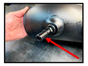
100. (Whipple 132mm Crusher throttle body) Install the supplied 5" ID x 2 1/2" silicone hose over air inlet tube and airbox lid. Install the 4 3/4" x 3" silicone hose over throttle body. Install the air inlet tube between the filter and throttle body. Slide silicone hose over throttle body. Secure all ends with the supplied (4) #80 hose clamps.
