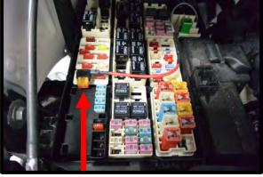
107. (**Dual fan installation**) Connect the 12V eyelet to the 3<sup>rd</sup> power stud (same as IC pump previously installed). Splice the orange turn-on wire to the IC pump (#44). Use the supplied steel bracket to use previously installed push pin to secure relay and fuse. Route the wires down on the passenger side of radiator. Connect dual fan 2-way's to fan relay harness 2-way's. Zip tie wires for clean installation.
