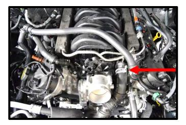
29. Remove the **LH** side heater tube from engine by removing the bolt using an 8mm socket. Install the supplied oring to the shorter heater tube and install to factory location, secure with stock bolt, torque to 89 lbs-in. Reconnect both factory hoses, secure lower hose with stock clamp.
