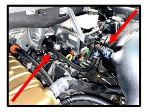
103. Connect the supplied 3-way to 4-way pigtail (driver side 3-pin IMRC connector) to the airbox MAP/Baro sensor previously installed. Secure pigtail with zip-ties.
