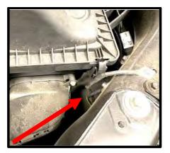
96. (Complete kits) Using a 3/8" drill bit, drill a hole for the baro/MAP sensor in the lower Whipple airbox. **NOTE:** This is to read barometric pressure, therefore its placement is not critical.
