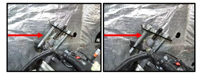
33. Reinstall the factory fuel feed line into the factory support bracket on the driver side cylinder head.
