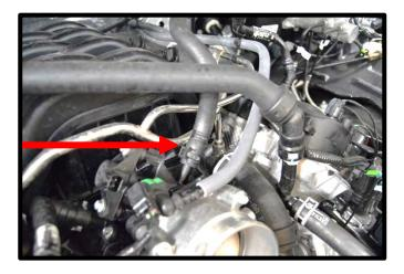
16. Carefully cut the electric tape securing the ETC wires to the throttle body. Disconnect the electronic throttle electrical connector by pushing up on the safety lock and then squeezing the connector and pulling away.
