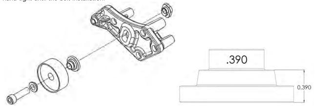
68. Install the supplied (1) grooved idler pulley #36326 to the idler plate using the (1) idler step washer and (1) ½"-13 x 2" SHCS. Torque idler pulley bolt to 30 lbs-ft. using a 3/8" allen socket. **NOTE:** Use light amount of anti-seize on threads.
