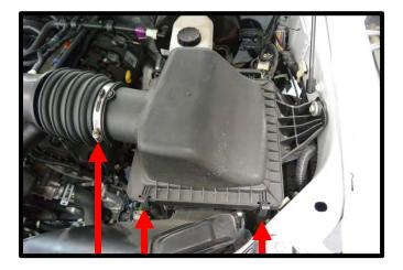
11. Using a 13mm socket, remove the (1) factory fastener securing airbox to the fender (bolt and grommet will be reused later).
