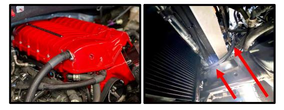
94. Install the supplied 3/4" ID hose with 90deg end from pump outlet barb to heat exchanger inlet fitting. Secure both ends with supplied pinch clamps.
