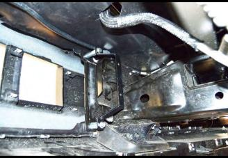
84. Install the supplied (4) rubber grommets to the LTR mounts. Install the supplied (4) aluminum LTR spuds to rubber grommets installed in LTR.
