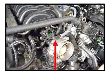
15. Remove the manifold vent hose next to the EVAP, use a pinch clamp tool to remove pinch clamp and hose.
