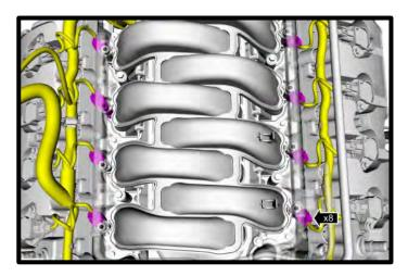
23. Loosen the 4 bolts holding the fuel rails down, these go through to the cylinder head (10mm socket). Fuel rail does not need to be removed.
