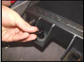
85. **(Dual fan installation)** Install the supplied (4) rubber strips to the bottom flat portion of the fan mount brackets. Clean the brackets with soap and water. Remove the protective tape from the rubber strip and install to the bracket. Install the (4) rubber feet per fan to the bottom of the fans.
