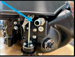
44. Using the supplied 5/16" OD silicone tube, install the (1) 80 1/2" cord. Start as shown with green arrow, go in a clockwise motion, to the front, then around the perimeter. End at yellow arrow position. Bunch it up so it has no gap at the end as any gap will be an air leak of un-intercooled air. Install the (1) 6.5" cord in the front section shown with the blue arrow.
