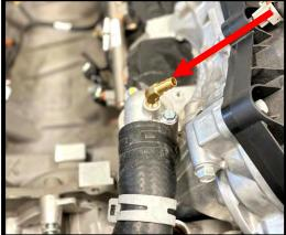
62. Connect factory heater hoses to previously installed plastic water fitting (bank 2).
