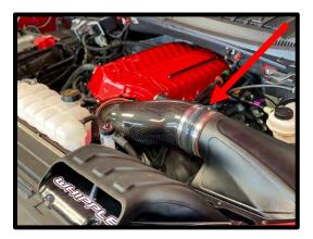
101. (Stock throttle body installations) Install the supplied 5" ID x 2 1/2" silicone hose over air inlet tube and airbox lid. Install the supplied reducer silicone hose over air inlet tube and stock throttle body. Connect the other end to the stock throttle body. Secure all ends with the supplied hose clamps (2) #80, (1) #64 and (1) #56 on throttle body.
