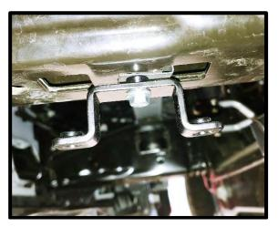
82. Remove the (4) bumper support bolts and clips using a 13mm socket. Install the supplied hex stands to the bumper support. Use the 30mm hex stands on the bottom (2) bolts. Use the 45mm hex stands on the top (2) bolts. Torque to 15 lb-ft with a 13mm socket.
