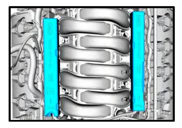
22. Disconnect all fuel injector connectors by using a flat head screw driver on one side of the clip. Pry to one side and clip will slide off.
