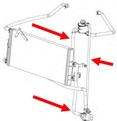
92. Install the ¾" ID x 12" rubber hose (#3103092) from the **LH (OUTLET)** IC fitting to the IC filler neck. Secure both ends with supplied pinch clamps. This goes under the air inlet tube. **NOTE: NEVER SWITCH THE INTERCOOLER ROUTING, BANK 2 IS ALWAYS THE OUTLET!**
