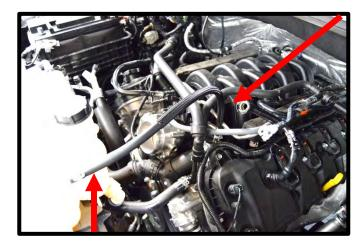
13. Disconnect the EVAP solenoid connector by squeezing locking tab and pulling away.
