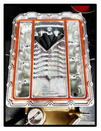
45. Install the supplied pre-formed 65.3" x .103" oring to the top sealing surface of the SC housing. Apply generous amount of grease to help ease the oring into place. **TIP:** To install oring into dove-tail groove, press vertically, vs sliding finger along.
