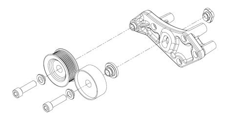
69. Install the supercharger pulley using the supplied (5) 6mm x 14mm SHCS using a 5mm allen socket. Leave hand tight until belt installation.
