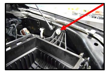
12. Using a pair of pinch clamps, remove the vent line from the coolant overflow tank to the water neck.
