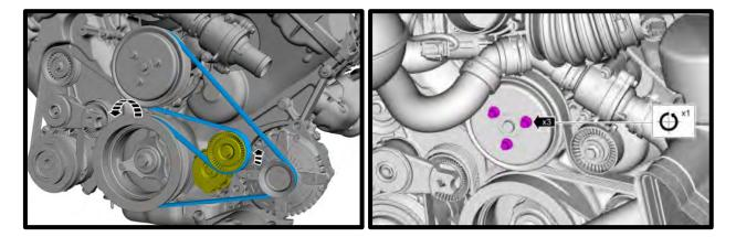
35. Using a 10mm socket, remove the (3) factory fasteners from the timing chain to head cover and (1) from water pump (for new idler plate).
