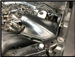
99. Install the (1) supplied 13/16" to ½" rubber grommet into the supercharger inlet tube. Install the supplied ½" to 15.82mm quick connect fitting.
