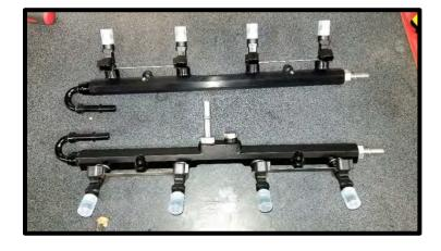
40. Apply generous amount of grease to the injector orings for ease of installation. Install the fuel injectors, rails and lock bracket to the intake manifold, secure with the (4) 6mm x 16mm SHCS using a 5mm allen socket. Torque to 90 lbs-in.
