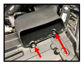
98. Install the supplied panel filter to the airbox lower. Install the upper airbox to the top of the filter. Secure the top to bottom using the supplied (6) 6mm x 16mm BHCS. Torque to 50 in-lbs. \*Caution: Over torquing can result in pulling an insert out of plastic box.
