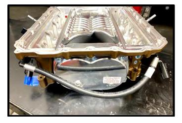
42. Route the supplied 3/8" x 50" cross over fuel hose around the back of the supercharger. (2) Adel clamps are supplied to secure to 2 SC Lid bolts across the back when installing lid later.
