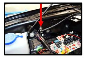
106. Pull the red 10amp fuse from position #105. Install the 10amp red fuse in the unused fuse slot on the fuse tap. Install the supplied fuse tap into position #105. Note: 10amp red fuse should be in bottom slot, 5amp should be in top slot. Make sure wire has enough room when fuse cover closes, route around fuses for clean installation.
