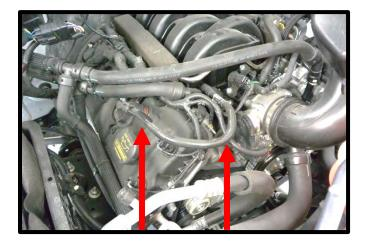
10. Unclip the airbox lid by flipping the (2) tabs to release. Using a 5/16" nut driver, loosen the factory hose clamp securing the air inlet tube to the air box lid and throttle body. Remove airbox lid from engine. Remove air filter from airbox.
