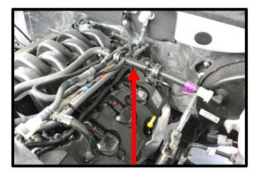
20. Carefully remove the factory fuel line by releasing the blue safety lock, then squeezing the connector and pulling back. The fuel system may still have pressure, use protective eyewear and multiple rags to catch any possible fuel leak.
