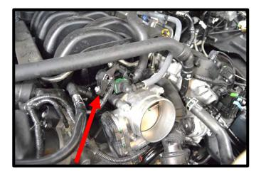
14. Remove the EVAP vent line quick connector from the EVAP solenoid by pushing the (2) locking tabs away and squeezing the tab, then pull away. Pull this line away from engine (goes down to driver side lower firewall area).
