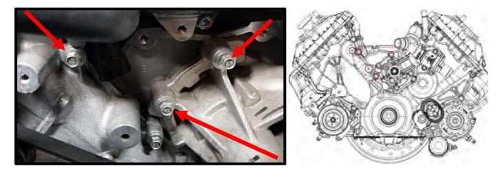
36. Use the supplied (3) 8mm x 90mm SHCS to secure the idler plate to the engine. Using a 6mm allen, torque to 22 lbs-ft.
