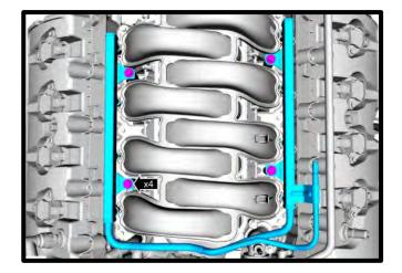
24. Loosen the (6) manifold to cylinder head bolts using an 8mm socket.
