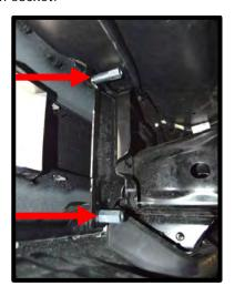
83. Install the left and right brackets to the previously installed coupling nuts. Use the supplied 8mm x 16mm flanged hex bolts to secure. Torque to 15 lb-ft with a 13mm socket.
