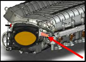
76. Install the supplied 5/8" ID x 9" PCV hose to the passenger side valve cover. Connect other end to the supercharger inlet 15.82mm quick connect fitting. Push until it clicks and locks into place.
