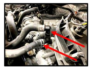
63. Connect the factory heater hose quick connect to factory heater tube (bank 1).
