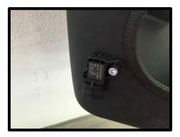
97. Install the supplied lower airbox into factory (2) hole locations. Using the supplied (2) 1.1" L x .30" W plastic push pins, secure front of snorkel to factory location.
