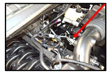
9. Remove the driver side and passenger side valve cover vent line quick connect fittings from the inlet tube by squeezing the connector and pulling away. Remove from valve cover by squeezing the connector and pulling away.
