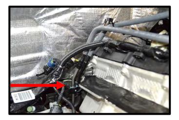
31. Cut the factory EVAP hose just below the 90deg bend (.125" below). NOTE: Make sure this cut is straight.
