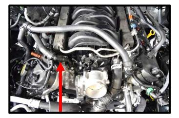
18. Remove the quick connect fitting on the heater tube, **LH**/drivers side. Push hose to the back of the engine for later use. Remove the coolant to heater tube overflow hose using a pinch clamp tool. Pull away from heater tube.
