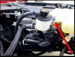
81. Install the supplied pump mount bracket frame opening on **LH** side. Slide J-nut through opening on frame. Secure bracket to J-nut using supplied (1) 6mm x 30mm HHFCS. Install pump clamp to bracket using the supplied (2) 6mm x 10mm HHFCS bolts. Mount pump in clamp using the 1" wide rubber strip around pump, secure clamp. **NOTE:** Outlet fitting should be facing straight up, inlet should be facing center of vehicle.
