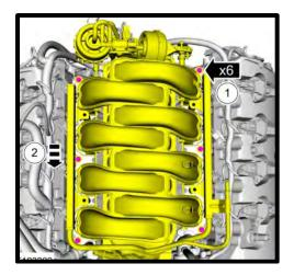
25. Remove the intake manifold from the engine. Pull up from the front then remove the (2) wire harness push pin supports from the back of the intake manifold and disconnect the (2) IMRC solenoid connectors and (2) IMRC position sensor connectors by pushing on the locking tab and pulling away IMRC solenoid. Remove from the driver side, rear of intake manifold, 4-way MAP sensor connector by pushing on the locking tab and pulling away.
