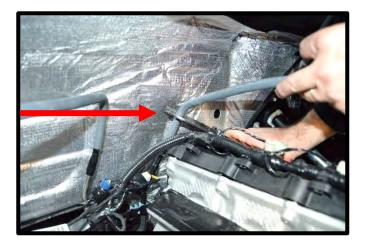
32. Using the supplied brackets (IC reservoir mounting brackets), (2) 8mm x 90mm SHCS (2) and #4 hose clamps, install the plastic coupler into the factory EVAP hose you just cut. Apply grease to plastic coupler to aid in installation. Use the hose clamps to hold the hose in place at the bottom of the hose. Slowly tighten the 8mm bolts until the coupler is fully installed.
