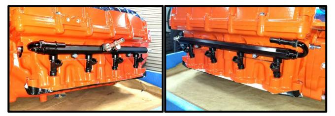
41. Install the supplied 3/8" fuel cross over line around the back of the supercharger by pressing until they click and lock in place. It's also possible to leave off until after SC is installed for easier access to rear bolts. \*Note: The 90deg end goes to bank 2 side.
