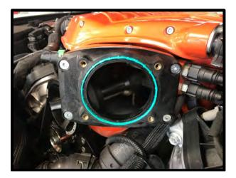
78. (Stage 1) Install the stock throttle body using the (4) 6mm x 50mm FHSCS bolts using a 10mm socket.
