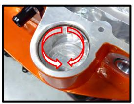
66. Apply generous amount of grease to the (1) #2-230 Viton bypass oring. Install the supercharger lid to the supercharger housing by carefully placing the bypass down. Secure the SC lid using the (17) 6mm x 30mm HHFCS and (3) 6mm x 70mm HHFCS (*marked green*) using the following pattern. Slide the EECPV bracket under bolts 3 and 5 from image (LH). Torque to 90 lbs-in using an 8mm socket.
