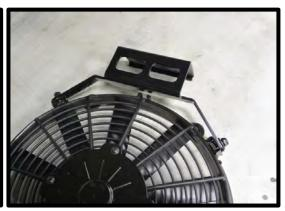
87. (Stage 2 heat exchanger installation) Carefully set both fan assemblies on top front of the LTR, space these evenly before installing.
