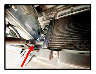
95. Lightly bend the (2) ground wire so it goes below the frame. **NOTE:** Failure to do so will rub airbox and push airbox towards firewall and cause fitment issues.
