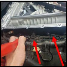
50. Install the supplied TMAP pigtail to the 3-Bar TMAP supplied, wrap up pigtail to SC inlet as this will get connected to stock harness later.
