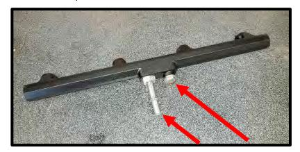
38. Install supplied (2) #2-906 orings to the (2) 9.49mm to -6 ORB inlet/outlet fittings. Install these (2) fittings into rear side of fuel rails. Apply light amount of grease to oring for ease of installation. Using a ¾" wrench (or ¾" deep socket) on both the front and rear fittings, tighten both. Install the (2) supplied 6AN 180deg swivel fittings to front port on each rail. Using a ¾" wrench, secure fittings to fuel rails.
