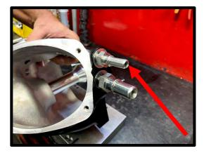
75. Install the supplied 1/2" ID x 14" with 90deg quick connect fitting brake aspirator hose (#HSF150-HS012) from the brake booster to the **lower** quick connect fitting on the supercharger inlet. Push until it clicks into place. **TIP:** For best routing, nestle in between cam cover and fuel rail, under the wiring and heater hose.
