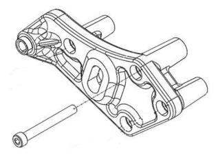
54. Torque the (10) 6mm (10) HHFCS bolts in the following pattern using a 10mm socket. First pass: 88 lbs-in. Second pass: 106 lb-in. **NOTE:** For bolt #10, a ¼" socket with 4"-6" extension, 10mm wobble is the best possible tool to get into this tight area.
