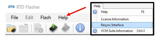
9. Once calibration is supplied, save to your PC in the same location as the stock file. Open RTD Flasher. Open the calibration by clicking file, connect to vehicle, turn key to engine run (do not start engine), push button type ignitions, hold push button down for 10 seconds to activate diagnostic mode. Click the red arrow icon (**WRITE VEHICLE**) to write the new calibration to the vehicle.
