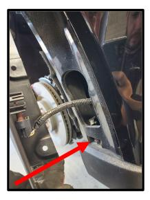
6. Remove the (2) bolts holding the bumper cover to front fender using a 10mm socket.
