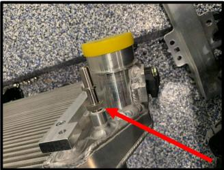
24. Install the (2) mounting brackets to the Whipple IC using the (2 per side) 6mm x 16mm HHFCS bolts. Apply light amount of Blue Loctite to threads.
