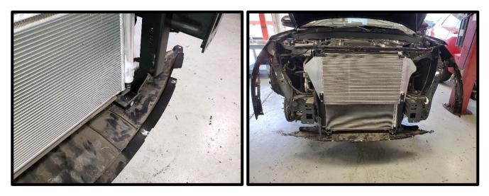
26. Install the (2) lower support brackets by setting into position on the factory frame. Secure brackets to front of intercooler using the supplied (4) 6mm x 16mm FFHCS bolts. Apply light amount of Blue Loctite to threads.
