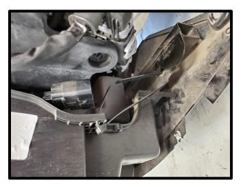
18. Remove the (4) bolts from upper shroud using an 8mm socket.
