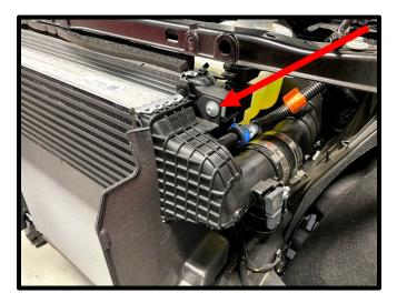
22. Remove the TMAP sensor from the stock intercooler using a Torx 30. Transfer this to the Whipple intercooler outlet tank, apply Blue Loctite to threads of supplied 6mm x 16mm HHFCS bolt.
