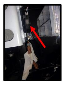
10. Unplug the headlight harness connectors and the TMAP sensor connector from intercooler.
