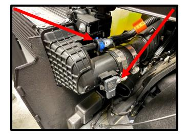
20. Loosen the intercooler clamps on the inlet and outlet connection hoses.
