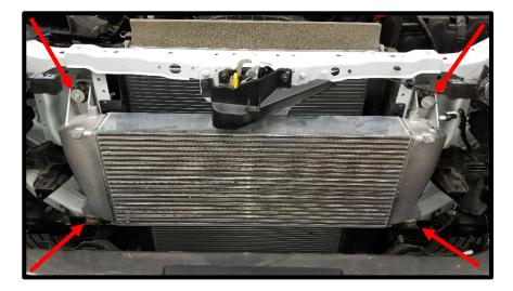
18. Reconnect inlet and outlet pipes using factory connections.
