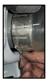
19. Remove the MAP sensor from stock intercooler by removing the (1) fastener. Apply light amount of grease to oring, install to new intercooler using supplied (1) 6mm x 16mm bolt. Reconnect factory electrical connector.
