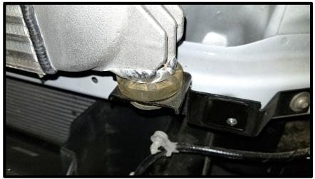
17. Secure new intercooler using the (4) factory fasteners previously removed. Torque to 97 in-lbs.
