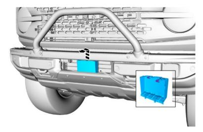
11. (When applicable) Disconnect the lower active grill shutter actuator electrical connector.
