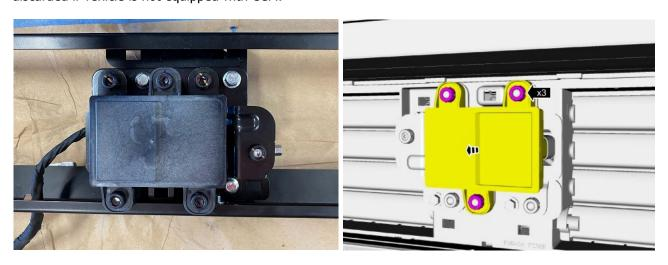
20. Remove the active grille shutter motor from assembly by remove U-shape brace, then removing shutter arms from motor. Install on new supplied bracket using the (2) supplied zip-ties.
