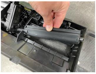
21. (When applicable) Mount the shutter motor to the bracket assembly using the (2) supplied zip-ties. Secure CCM wiring using same zip ties for a clean installation.
