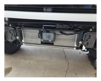
23. (When applicable) Reconnect CCM wiring connector to CCM. Reinstall plastic cover over CCM bracket, this will **NOT** fit after bumper installation.
