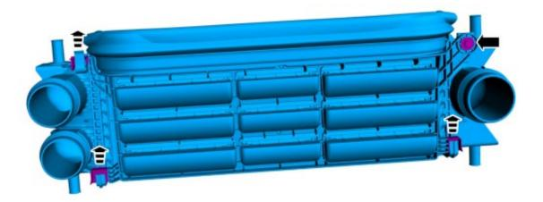
18. Set CAC to stock brackets. With the aid of a 2<sup>nd</sup> person, install the (4) bolts from the IC/tow hook brackets to install CAC. Torque to 59 ft-lb.
