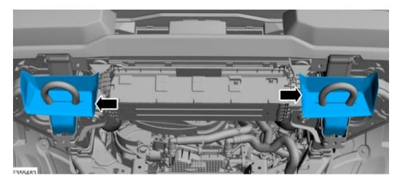
14. (When applicable) Gently release the CCM grommets from the active grille shutter CCM bracket, then remove CCM from bracket. Disconnect CCM wiring connector from CCM. NOTE: If not equipped with CCM, disregard.
