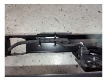
22. (When applicable) Install the new CCM bracket assembly to vehicle using the (4) factory fasteners. Torque to 62 in-lb using 8mm socket.
