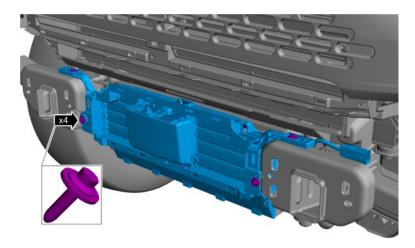
13. If equipped, remove the tow hook shields.
