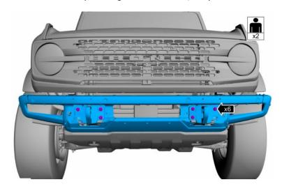
26. Reinstall the push pins and front bumper trim panel.
