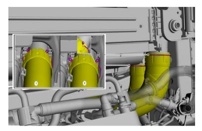
5. Release the CAC outlet pipe by spreading the retainer ends outward. Position the retainer ends in the notches locking the retainer in the open position and position aside the CAC outlet pipe.
