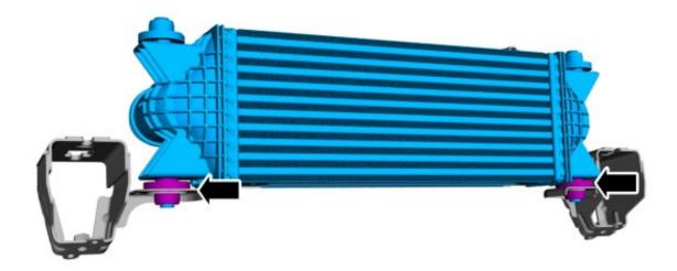
17. (If equipped) Remove the (1) bolt and dislodge the holding clips. Using factory bolt, transfer to new CAC. Torque to 62 in-lbs.
