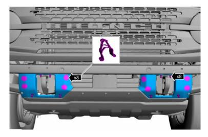
9. Remove the bolts and the front bumper using a 15mm socket.
