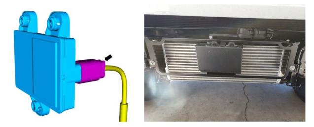
24. Reconnect the lower active grill shutter actuator electrical connector.
