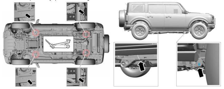
3. Remove the fasteners and the engine front under shield using 15mm socket. **NOTE:** Some models have (4), some have (6).
