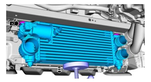
20. Connect the bypass valve electrical connector.
