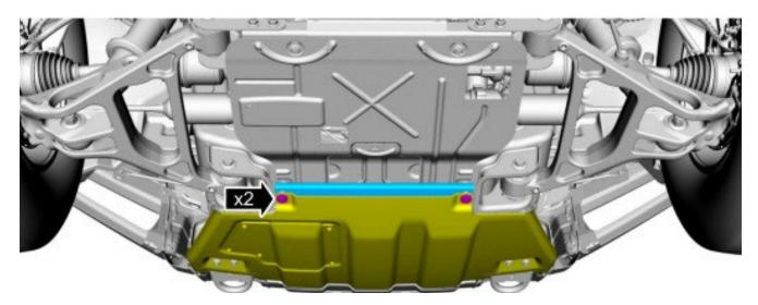
5. Remove the bolts and the front underbody skid plate.
