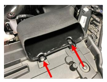
31. Install the supplied filter in the lower airbox. Install the supplied lid to filter and lower airbox. Secure using the supplied (6) 6mm x 16mm BHFCS. Torque to 50 in-lbs or snug. NOTE: Over torque can rip the brass insert out.
