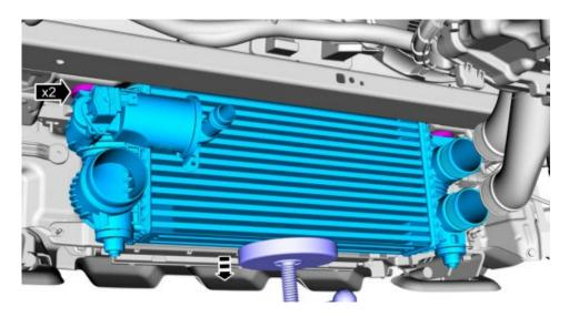
14. Remove the bolt from the turbocharger bypass valve. Rotate the bypass and remove from intercooler.
