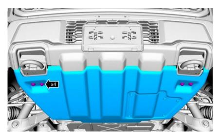
26. Install the underbody skid plate and spacer, secure with factory bolts. Torque to 41 ft-lbs.
