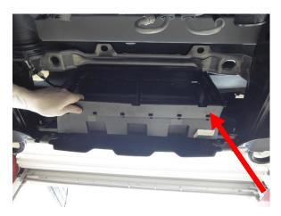
19. Raise the axle stand and install the intercooler core to vehicle.
