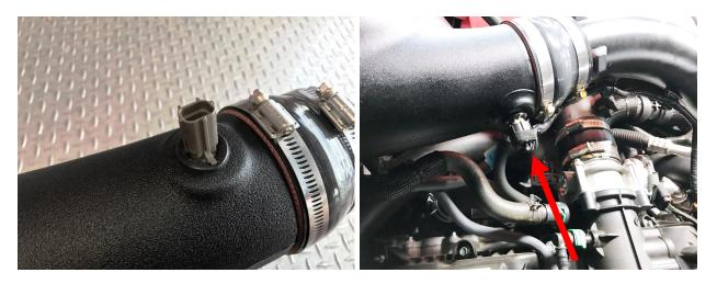
35. Install the supplied silicone hose to the Whipple air tube using the supplied clamps. Use the #64 clamp on the 4" hump hose and #56 on the 3.5" hose reducer hose.
