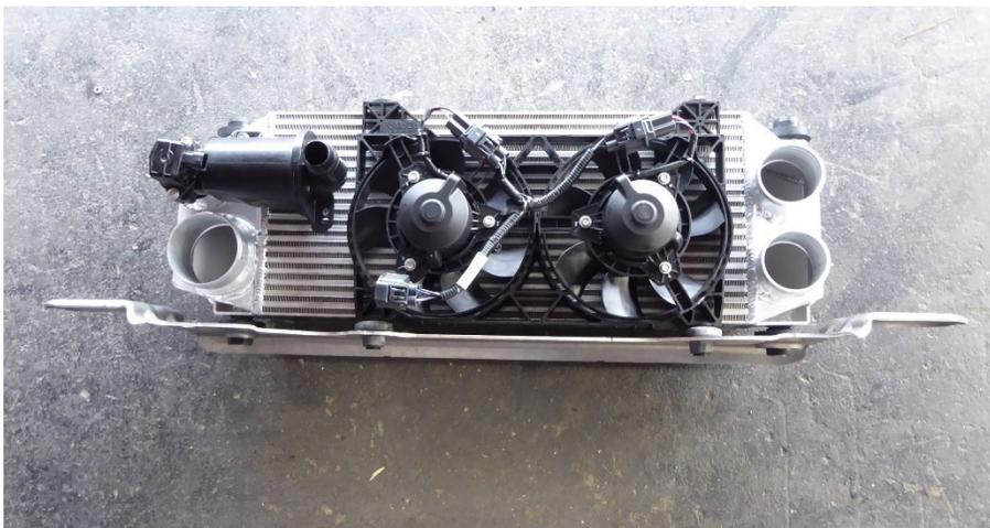
18. Remove the IC plastic trim section from the factory clips, this will not be reused with the larger intercooler core. **NOTE:** Expedition/Navigator will have to cut this for proper intercooler clearance. Give the intercooler face .25" to .50" of clearance.
