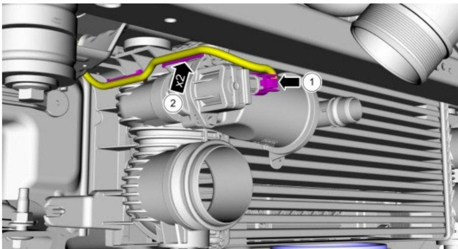
21. Connect the bypass valve tube and the supplied silicone 60deg outlet pipe. Secure outlet pipe to factory hose using supplied (1) 3.75" T-bolt clamp. Secure tube to intercooler using (1) 3.75" t-bolt clamp.
