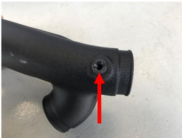
34. Install the air temp sensor into the air tube, use light amount of grease or silicone to help sensor install.
