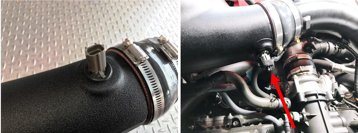
35. Install the supplied silicone hose to the Whipple air tube using the supplied clamps. Use the #64 clamp on the 4" hump hose and #56 on the 3.5" hose reducer hose.
