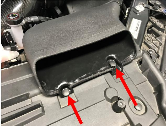
31. Install the supplied filter in the lower airbox. Install the supplied lid to filter and lower airbox. Secure using the supplied (6) 6mm x 16mm BHFCs. Torque to 50 in-lbs or snug. NOTE: Over torque can rip the brass insert out.
