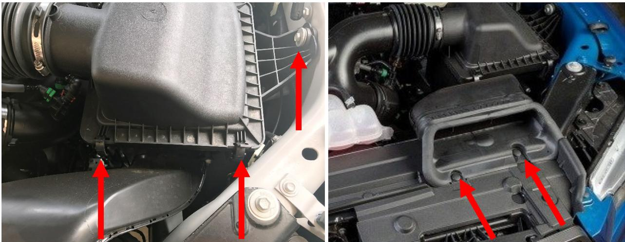
30. Install the lower airbox section to factory location. Using the supplied (2) 1" Christmas tree plastic tabs to snorkel section to secure airbox.
