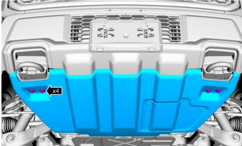
26. Install the underbody skid plate and spacer, secure with factory bolts. Torque to 41 ft-lbs.
