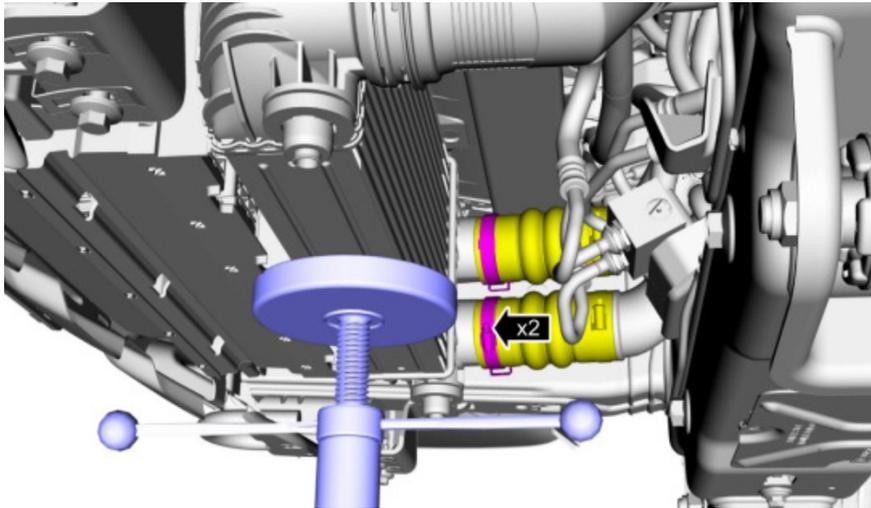
23. Install the lower bracket and fan assembly, secure with factory bolts. Torque to 30 ft-lbs.
