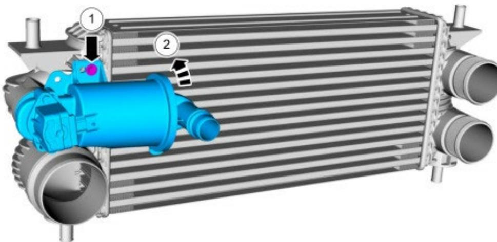
15. Mount the bypass valve to the new intercooler with the supplied 6mm x 10mm flanged hex headed bolt. Torque to 62 in-lbs.
