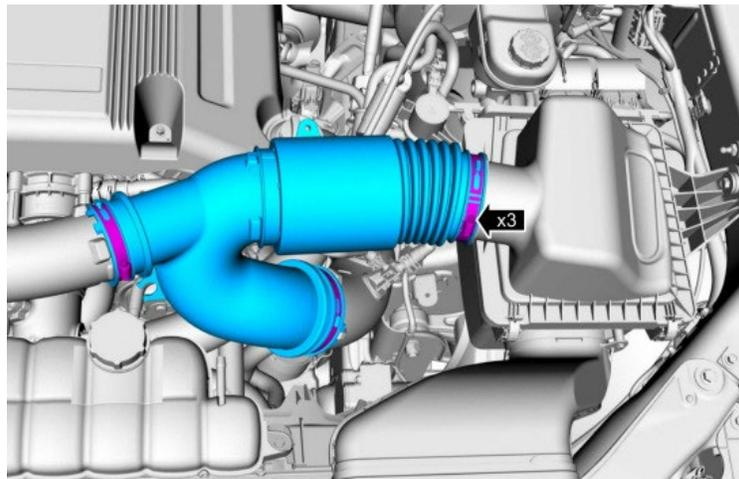
29. Unsnap the airbox retaining clips (2) and remove the factory filter, neither will be reused. Using a 10mm socket, remove the bolt securing airbox to body. Using a push pin removal tool, remove the 2 pins holding the airbox snorkel in place.
