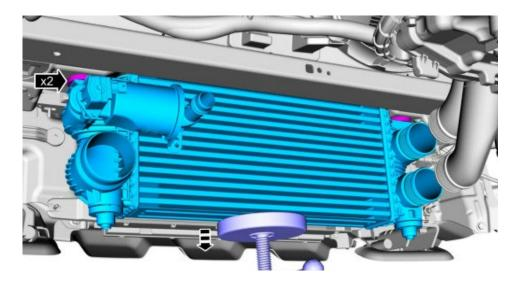
13. Remove the bolt from the turbocharger bypass valve. Rotate the bypass and remove from intercooler.
