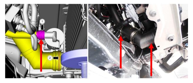
10. Remove the 45deg plastic elbow from the factory rubber hose by loosening the hose clamp (#2 in image).
