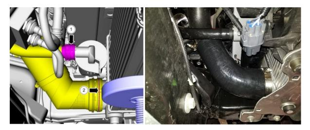
21. Install the clamps and position the intercooler intake pipes.
