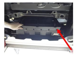
18. Raise the axle stand and install the intercooler core from vehicle.
