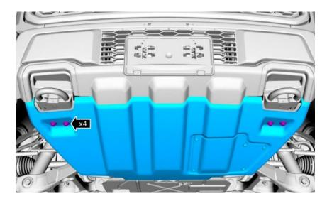
25. Install the underbody skid plate and spacer, secure with factory bolts. Torque to 41 ft-lbs.
