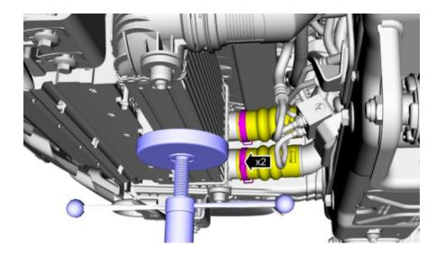
22. Install the lower bracket and fan assembly, secure with factory bolts. Torque to 30 ft-lbs.
