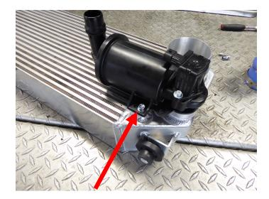
15. Transfer the rubber isolators from the OEM intercooler to the Whipple Cooler.
