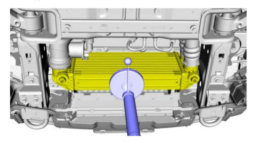
8. Loosen the clamps and position the intercooler intake pipes LH and RH aside.
