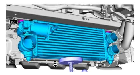
19. Connect the bypass valve electrical connector.
