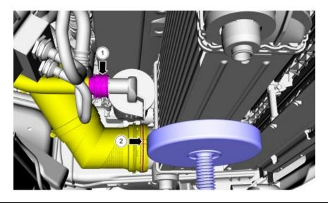
11. Disconnect the bypass valve electrical connector and place wiring harness aside.
