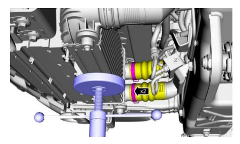
9. Disconnect the bypass valve tube. Release the clip and position the intercooler outlet pipe aside.
