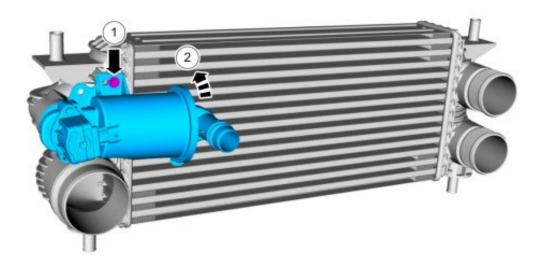
14. Mount the bypass valve to the new intercooler with the supplied 6mm x 10mm flanged hex headed bolt. Torque to 62 in-lbs.
