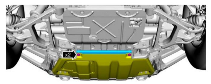
4. (Raptor Only) Remove the bolts and the front underbody skid plate (when applicable).
