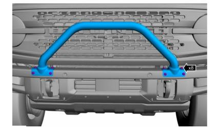
8. Remove the push pins, release the clips and remove the front bumper trim panel.
