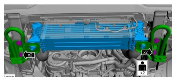
19. Remove the CCM bracket from active grill shutter using an 8mm socket. Transfer CCM bracket to supplied CCM bracket assembly using the (3) 6mm x 10mm HHFCS fasteners. Torque to 96 in-lb using a 10mm socket. Slide CCM module back on bracket. NOTE: CCM bracket is pre-positioned and should not require adjustment, CCM equipped vehicles should never modify CCM bracket or fasteners. The CCM bracket can be discarded if vehicle is not equipped with CCM.
