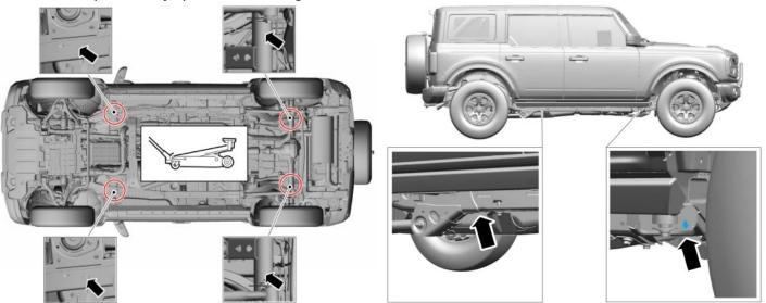
3. Remove the fasteners and the engine front under shield using 15mm socket. **NOTE:** Some models have (4), some have (6).
