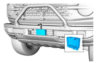
11. Disconnect the lower active grill shutter actuator electrical connector.
