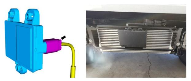
24. Reconnect the lower active grill shutter actuator electrical connector.
