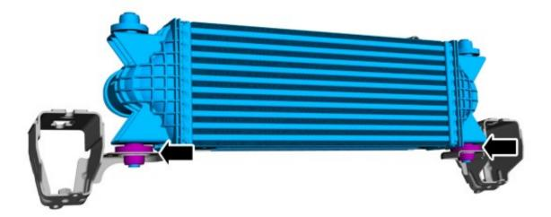
17. (If equipped) Remove the (1) bolt and dislodge the holding clips. Using factory bolt, transfer to new CAC. Torque to 62 in-lbs.
