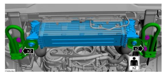
16. Remove the CAC isolators from CAC. Transfer to new CAC.
