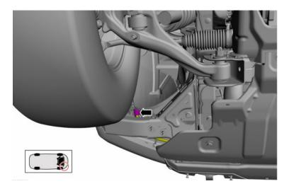
29. Reinstall the fasteners and the engine front under shield. Torque to 124 in-lbs.
