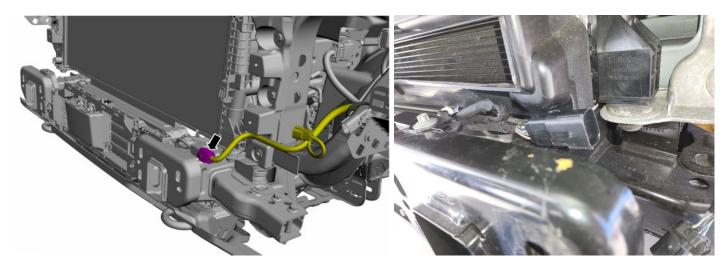
25. Install the stock bolts and the front bumper using a 15mm socket, torque to 81 ft-lb.
