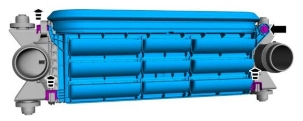
18. Set CAC to stock brackets. With the aid of a 2<sup>nd</sup> person, install the (4) bolts from the IC/tow hook brackets to install CAC. Torque to 59 ft-lb.
