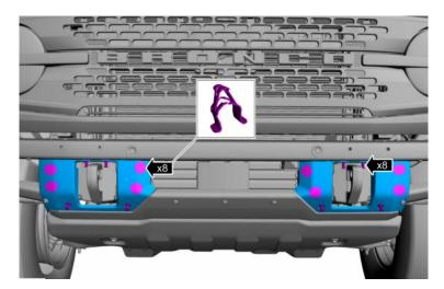
27. Reinstall the front bumper bar with the factory (8) bolts using a T40 socket. Torque to 25 ft-lb.
