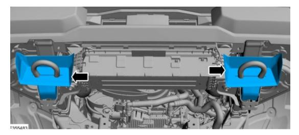
14. Gently release the CCM grommets from the active grille shutter CCM bracket, then remove CCM from bracket. Disconnect CCM wiring connector from CCM. NOTE: If not equipped with CCM, disregard.
