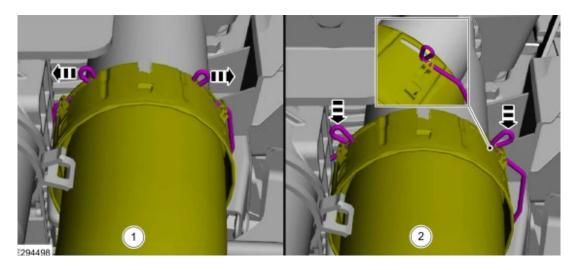
5. Release the CAC outlet pipe by spreading the retainer ends outward. Position the retainer ends in the notches locking the retainer in the open position and position aside the CAC outlet pipe.
