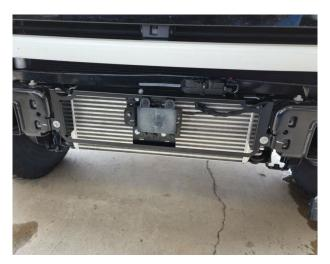
23. Reconnect CCM wiring connector to CCM. Reinstall plastic cover over CCM bracket, this will **NOT** fit after bumper installation.
