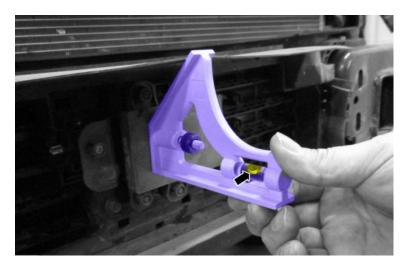
35. **NOTE:** Measurement must be taken from the non-raised side of the CCM. Keeping the combination square level on the face of the CCM, adjust the pitch by turning the adjustment screw until the CCM is vertical and level.
