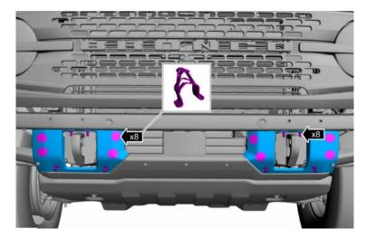
9. Remove the bolts and the front bumper using a 15mm socket.
