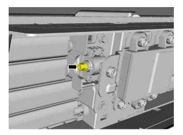
34. **NOTE:** Measurement must be taken from the non-raised side of the CCM. Place a combination square level on the face of the CCM and check the alignment.
