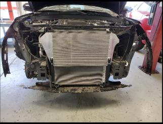
26. Install the (2) lower support brackets by setting into position on the factory frame. Secure brackets to front of intercooler using the supplied (4) 6mm x 16mm FFHCS bolts. Apply light amount of Blue Loctite to threads.
