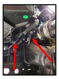
11. Disconnect electrical connector by releasing the gray tab.
