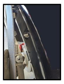
5. Disconnect the (2) proximity sensors and the (2) 7mm bolt under proximity sensor (per side).
