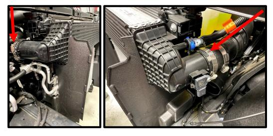
21. Remove the factory bolt from the IC mount flange using a 10mm socket. Lift intercooler up and away from vehicle.
