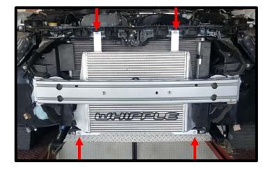
21. Couple the factory inlet and outlet hoses using the supplied aluminum coupler and silicone hose. Use the factory clamps on the factory hose. Use the supplied clamps to secure the silicone hose to the coupler.
