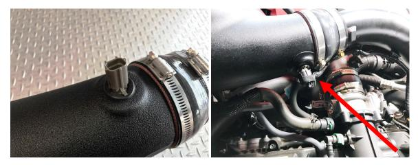
12. Install the supplied silicone hose to the Whipple air tube using the supplied clamps. Use the #64 clamp on the 4" hump hose and #56 on the 3.5" hose reducer hose.
