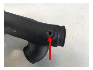
11. Install the air temp sensor into the air tube, use light amount of grease or silicone to help sensor install. Note: 18-20, install IAT extension harness.
