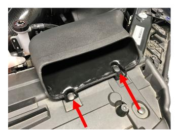
8. Install the supplied filter in the lower airbox. Install the supplied lid to filter and lower airbox. Secure using the supplied (6) 6mm x 16mm BHFCS. Torque to 50 in-lbs or snug. NOTE: Over torque can rip the brass insert out.
