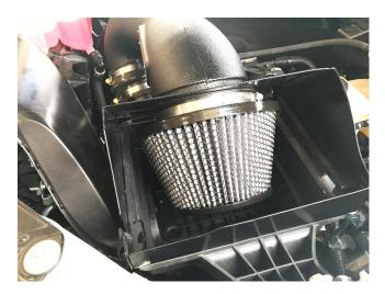
15. Install the supplied rubber shielding around the airbox edge, this will require cutting at each 90deg turn.
