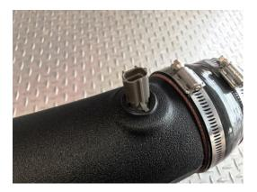
8. Install the supplied silicone hose to the Whipple air tube using the supplied clamps. Use the #64 clamp on the 4" hump hose and #56 on the 3.5" hose reducer hose.
