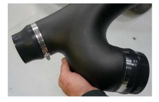
9. Install the supplied vent tube to the vent fitting that was connected to the driver side valve cover, its direction is critical, the slash cut must face the turbo inlet. This is a tight fit, it cannot rotate after installation. Ensure that the tube is fully seated against vent fitting shoulder. Reconnect the vent fitting.
