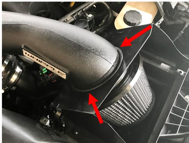
14. Secure filter to air tube using supplied clamp. Torque to 44 in-lbs.
