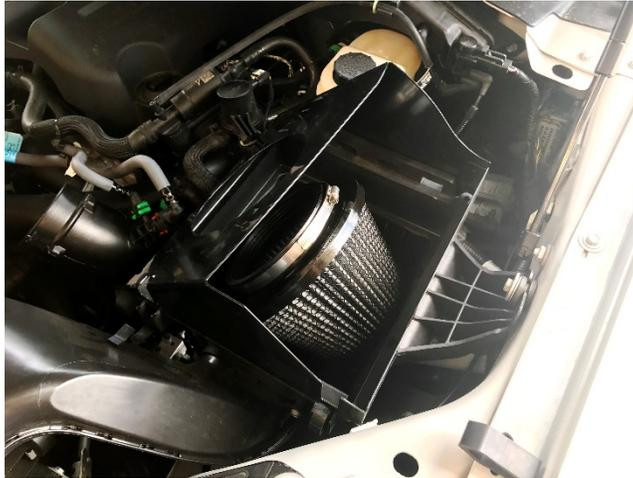
11. Install the new air tube to the engine by setting the inlet side through the airbox and installing other ends to factory air tubes. Use the #64 hose clamp on the 4" hump hose and the #48 clamp on the 2.5" reducer hose. Secure clamps, torque to 44 in-lbs.
