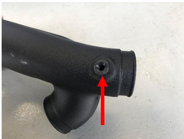
7. Install the air temp sensor into the air tube, use light amount of grease or silicone to help sensor install.
