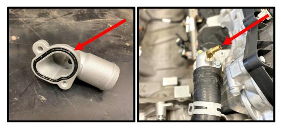
31. (**Single Alternator**) Reinstall water neck hose to new water neck. Using needle nose pliers, reinstall and rotate the factory pinch clamp at the water neck towards the driver side for future clearance of the SC. **NOTE:** Image shows clamp with SC installed to illustrate max clearance.
