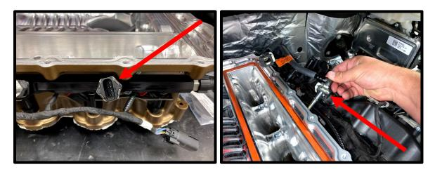
76. Slide the EECPV to previously installed bracket. Connect factory plastic quick connect fitting to EECPV until it clicks and locks into place. Connect 2-way electrical connector to EECPV, press locking tab back in place.
