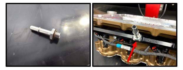
52. Install the supplied (2) #2-906 orings to the (2) inlet/outlet fittings. Install these (2) fittings into rear side of fuel rails. Apply light amount of grease to oring for ease of installation. Using a <sup>3</sup>/<sub>4</sub>" wrench (or <sup>3</sup>/<sub>4</sub>" deep socket) on both the front and rear fittings, tighten both.
