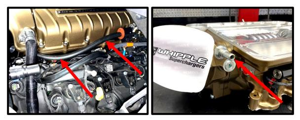
78. Install the stock PCV hose to the **RH** side valve cover. Connect other end to the supercharger inlet 15.82mm quick connect fitting. \*Note: This requires you to rotate the fittings for proper fitment. Push until it clicks and locks into place.
