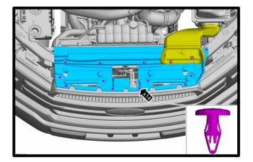
8. Disconnect the factory camera and windshield washer fluid connection from front grill area when applicable.
