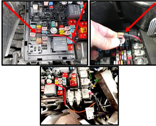
114. Install the fuse box cover, ensure the turn-on wire is clear of cover.
