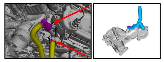
29. (Single Alternator) Install the supplied #2-113 oring to the shorter heater tube and install to factory location, secure with stock fastener, torque to 89 lbs-in. Reconnect both factory hoses, secure lower hose with stock clamp. NOTE: Some 2022 models, built without the auto start/stop pump. These are equipped with a 55deg fitting (blue arrow). Remove the stock fitting from stock hose, install the supplied 90deg fitting, secure with stock clamp.
