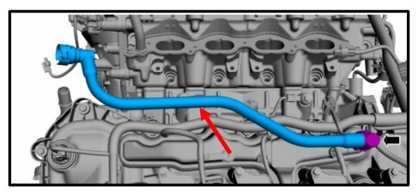
13. Disconnect the (1 or 2) quick connect fittings from air inlet tube. Using a 9/32" nut driver, loosen the factory hose clamp securing the air inlet tube to the throttle body and airbox. Carefully cut the electric tape securing the ETC wires to the throttle body. Disconnect the electronic throttle electrical connector by pushing up on the safety lock and then squeezing the connector and pulling away.
