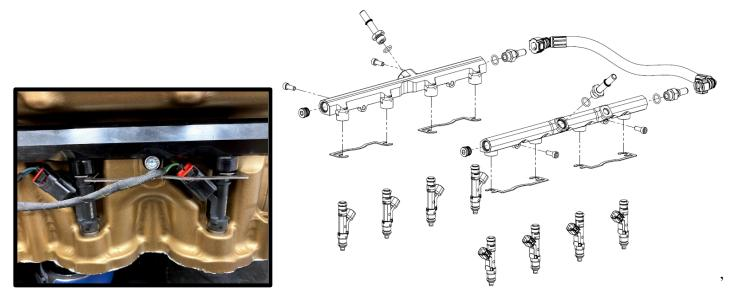
54. Apply generous amount of grease to the injector orings for ease of installation. Install the fuel injectors (*Stage 1 uses stock injectors, Stage 1R and 2 uses supplied injectors*), rails and lock bracket to the intake manifold, secure with the (4) 6mm x 16mm SHCS using a 5mm allen socket and use **Blue Loctite #243**. Torque to 90 lbs-in.
