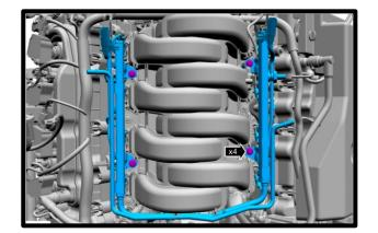
23. Disconnect all 8 fuel injectors from factory injector harness.
