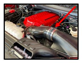
107. (**Stock throttle body installations**) Install the supplied 5" ID x 2 1/2" silicone hose over air inlet tube and airbox lid. Install the supplied reducer silicone hose over air inlet tube and stock throttle body. Connect the other end to the stock throttle body. Secure all ends with the supplied hose clamps (2) #80, (1) #64 and (1) #56 on throttle body.
