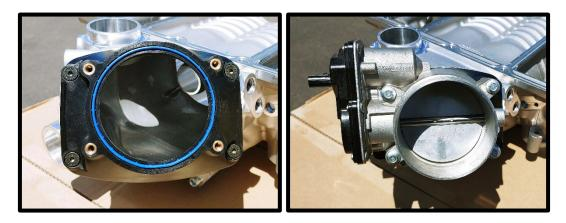
99. (Stage 2 Whipple 132mm Crusher throttle body) Install throttle body to supercharger inlet, use the supplied gasket between TB adapter and SC inlet. Secure with the supplied (3) 6mm x 25mm SHCS and (1) 6mm x 50mm SHCS using a 5mm allen socket. Torque to *89 lbs-in* on first pass, *139 lbs-in* on second pass.
