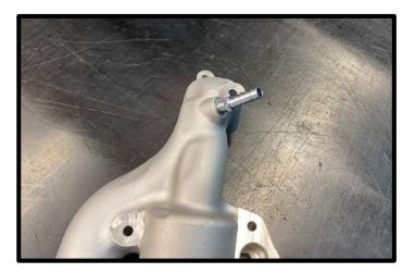
39. (**Dual Alternator**) Install the new thermostat housing assembly to engine using (3) of the factory fasteners, leave hand tight for now.
