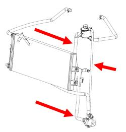
96. Install the <sup>3</sup>/<sub>4</sub>" ID x 12" rubber hose (#3103092) from the **LH (OUTLET)** IC fitting to the IC filler neck. Secure both ends with supplied pinch clamps. This goes under the air inlet tube. **NOTE: NEVER SWITCH THE INTERCOOLER ROUTING, BANK 2 IS ALWAYS THE OUTLET!**
