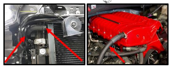
98. (Stage 1 and Stage 1R Stock throttle body) Install throttle body adapter to supercharger inlet using the (4) 6mm x 20mm FHCS bolts and supplied gasket between TB adapter and SC inlet. Apply Blue Loctite #243, torque to 65 lbs-in. Install the stock throttle body using the (4) stock bolts using a 10mm socket, torque to 80 in-lbs.
