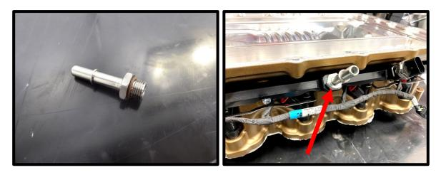
51. Install the supplied (1) #2-906 Viton oring to the (1 of 2) 45mm long 9.49mm outlet fitting. Apply light amount of grease to oring for ease of installation, install to rail.
