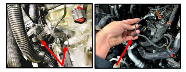
46. Loosen the (3) bolts securing the water pump pulley using a 10mm socket (while belt is on). Remove the belt from the engine by using a 15mm socket on a 1/2" breaker bar and rotating the spring-loaded tensioner in a clockwise direction. Remove water pump pulley using a 10mm socket (this will be reused).
