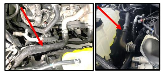
42. (**Dual Alternator**) Reconnect factory quick connect fittings to new coolant tubes. **NOTE:** Some model F150's switched the top fitting from the 90deg to a 55deg (blue arrow). Replace the 45 deg fitting with the supplied 90deg fitting.
