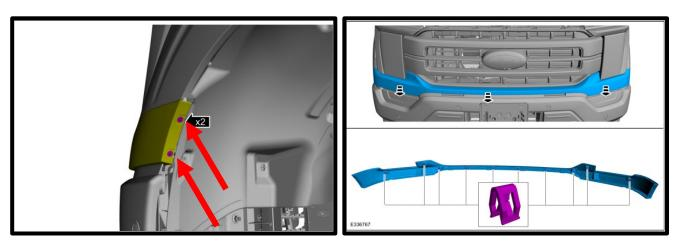
Remove the (4) bolts using a 10mm socket and the (2) push pins from the upper side of the grill shell. Remove the (2) lower bolts from the bottom side of the grill shell.
