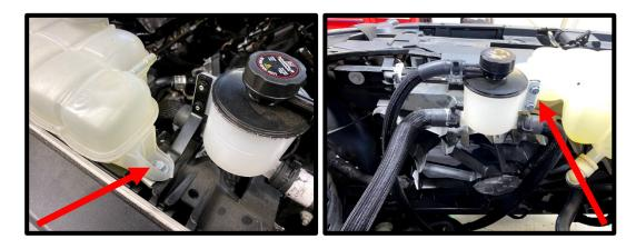
95. Install the ¾" ID x 32" hose (#3103094) and the 3/8" ID 39" (#3103098) rubber hoses to the IC filler neck. Secure with supplied pinch clamps. Connect the ¾" hose to the IC pump inlet fitting, secure with pinch clamp. Secure 3/8" vent hose with zip tie to the ¾" hose. **NOTE: Ensure that this hose cannot kink or rub anything overtime.**
