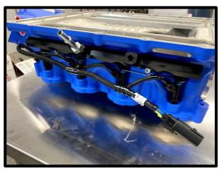
55. Install the supplied ¼" ID bypass actuator to the bypass nipple and ¼" 90deg nipple on SC inlet. **CAUTION:** Do not open/close bypass actuator by hand. This may damage actuator internally. It only moves properly with equal vacuum/boost at the actuator reference port.
