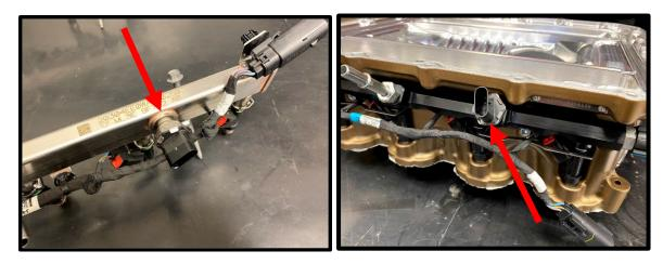
50. Install the supplied (1) #2-906 Viton oring to the (1 of 2) 45mm long 9.49mm inlet fitting to fuel rail. Apply light amount of grease to oring for ease of installation, install to rail.
