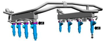
25. Using cutters, remove the clips that secure the injector harness to fuel rail. These clips will not be reused.
