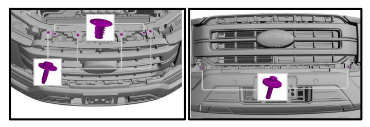
11. Remove the (4) pin-type retainer. Pull up and disengage the locating pins along the top of the grill. Pull forward on center of the grill to remove.
