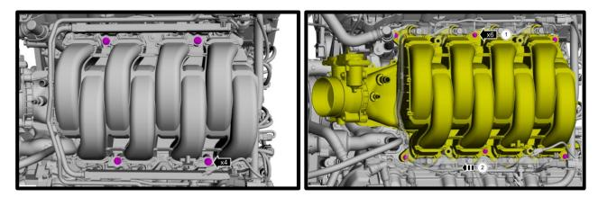
21. Use compressed air and remove any direct or foreign material from cylinder head, block and surrounding area of the fuel rail and injectors. Remove the intake manifold from the engine. To do so, remove the (5) wire harness push pin supports from the back of the intake manifold and disconnect the 4-way MAP sensor connector.
