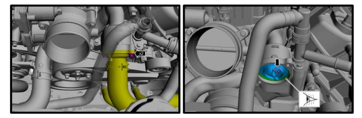
37. (**Dual Alternator**) Install the factory thermostat and thermostat oring to new housing. Install coolant inlet using the factory (2) bolts. Torque to 89 lbs-in.
