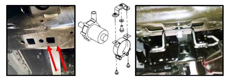
93. Install the supplied <sup>3</sup>/<sub>4</sub>" ID x 34" molded/formed hose (#3103095) with the 90deg end on the LTR bottom **LH** side fitting. Secure both ends with supplied pinch clamps. This must clear the plastic shroud and AC stud. **\*NOTE**: Use zip-ties to secure hose to core support.
