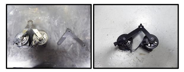
90. Reinstall new horn bracket and horns to factory location, using factory nut. Torque to 106 lbs-in. Zip-tie wire to factory harness for clean installation.
