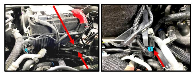
111. Using a 10mm socket, remove the nut on the power stud, located on the positive stud under fuse box cover. Install the IC pump relay power eyelet (red wire) to the power stud on the battery positive (+) stud. Use a 10mm socket to secure stock and IC power wire.
