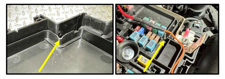
132. From fuse tap, route to slot you previously made, around to the stock slot at the front of fuse box. Add small relief in lid for wire as it comes out of the box. Failure to route properly may lead to cutting 12v wire for intercooler system.
