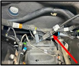
87. Install supplied IMRC electrical connector plugs (2x). Zip-tie to harness.
