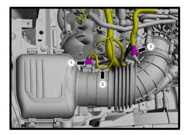
33. Loosen the hose clamp from throttle body using nut driver. Remove the air cleaner bolt. Detach the air cleaner from grommets and remove the air cleaner.
