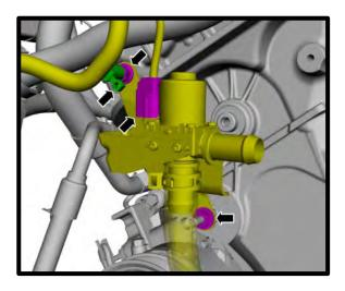
59. Remove stud from engine timing cover, this will not be reused.
