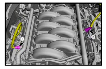
40. Remove the (4x) nuts from the top of the intake manifold, remove heater hose supports.
