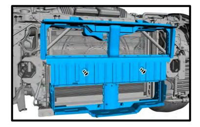
24. Remove the (6x) push pins (1), (2x) retainers (2) and depress and remove the clips (3) (2x).
