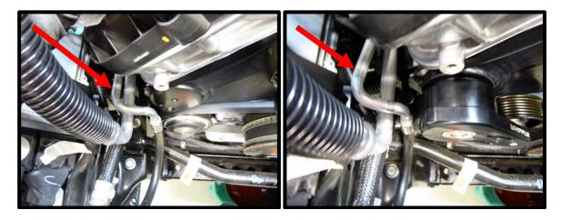
69. Install the spring-loaded tensioner to idler plate, locating the tang into position. Secure with the supplied (1x) 10mm x 60mm SHCS. Use light amount of anti-seize on threads. Torque to 25 lbs-ft.
