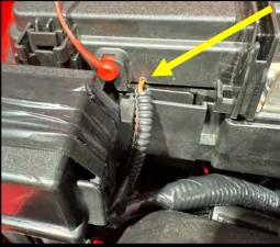
133. Using a 10mm socket, remove the 12V (+) power stud nut from the far post. Install the IC pump relay power eyelet (red wire) to the 12V stud. Use a 10mm socket to secure stock and IC power wire.
