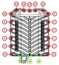
102. Install (4x) 2-117 IC fitting orings to the (4x) IC fittings. Apply grease to the (4x) 2-117 IC fitting orings. Slide fittings into lid. Secure fittings with supplied fitting retainer bracket and (2x) 6mm x 12mm SHCS bolt. Torque to 80 in-lbs.
