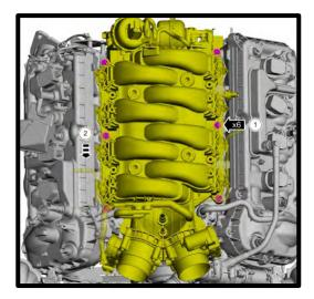
45. Disconnect the engine wiring harness electrical connectors and detach the retainers. Remove intake manifold.
