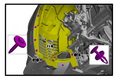
10. **(GT ONLY)** Remove the (12x) fasteners from the front chin splitter.
