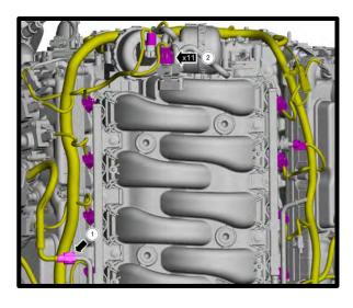
44. Loosen the (6x) manifold to cylinder head bolts using an 8mm socket. Position the manifold up and towards the front of the engine to access the rear of the manifold.
