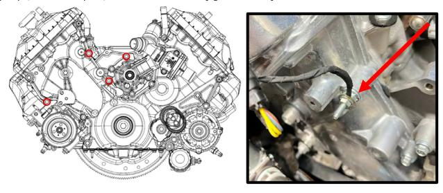
64. Using 10mm socket, remove the stock fastener (1x) from the top of the RH timing chain cover. Relocate stud with ground wire to the top timing chain cover location. Torque to 22 lbs-ft.
