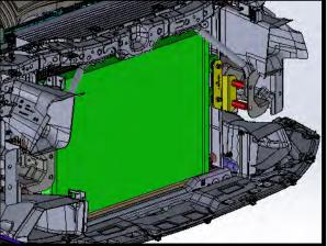
115. Remove factory coolant reservoir fastener. Install supplied reservoir bracket and secure on top of coolant reservoir. Secure using supplied (1x) 6mm x 20mm HHFCS. Torque to 71 in-lbs.
