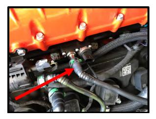
105. Connect the factory fuel PSI sensor connector to sensor, press safety lock until it clicks and locks in place.
