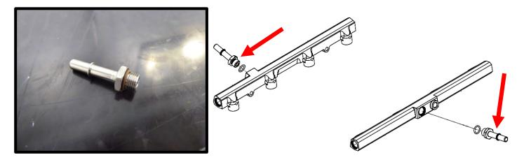
76. Apply light amount of grease to -6 ORB plugs, install the supplied (2x) -6 ORB plugs to front fuel rail ports.
