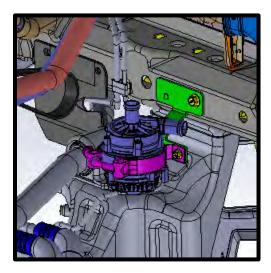
119. Install hose #3103407 from IC pump to LTR **LH low** (inlet) fitting. Secure using supplied #16 pinch clamps. Tighten IC pump clamp.
