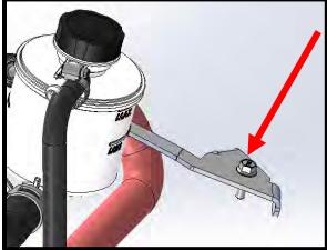
116. Mount IC reservoir to bracket using (2x) 6mm x 12mm HHFCS.
