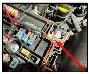
134. Use a small set of cutters to create passage for wire, use small file to clean up and round edges. Route wire through slot. Test fit lid and ensure it does not interfere with this wire. Failure to do so may result in intercooler system not working, resulting in bad/poor performance.
