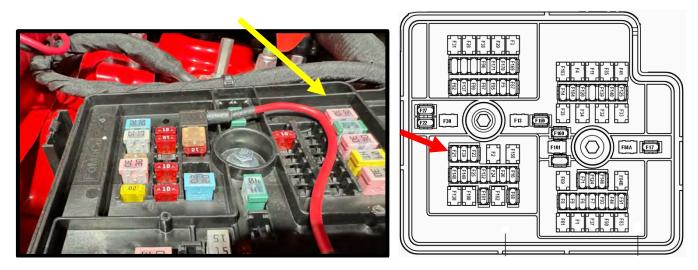
131. Use small set of cutters or file, make a small notch in fuse box cover lid and fuse box to allow wire to fit.
