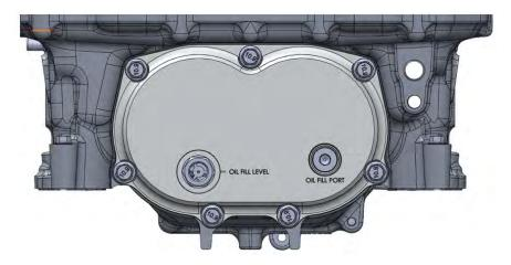
91. Install supercharger housing (without lid) to the engine. Use the supplied (4x) 6mm x 45mm HHFCS on the outer bolt holes and (6x) 6mm x 75mm HHFCS bolts with the supplied (6x) #2-009 orings on the bolt, under the head to the inner bolt bosses. Use **Blue Loctite #243** on the threads of each bolt. **Leave hand tight for now**.
