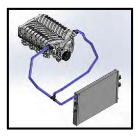
123. Install hose #3103405 from rearmost IC filler reservoir fitting to the top IC pump fitting (inlet). Use supplied #16 pinch clamps to secure hose.
