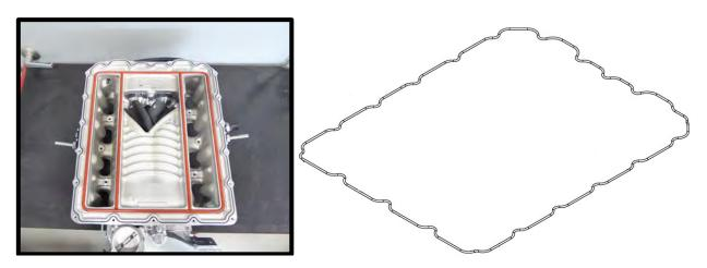
100. Install (1x) #2-230 internal bypass oring to the lid bypass passage. Use generous amount of grease to secure oring in place and help with installation.
