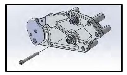
93. Torque (10x) 6mm HHFCS manifold bolts in the following pattern using a 10mm socket. First pass: 88 lbs-in. Second pass: 106 lb-in. **NOTE:** For bolt #10, a ¼" socket with 4"-6" extension, 10mm wobble is the best possible tool to get into this tight area.
