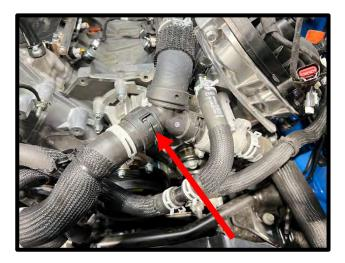
55. Transfer stock oring from stock water neck to new water neck. Apply pipe sealant to threads of 1/8" NPT to 5/16" 45 Deg fitting. Install fitting to water neck, rotate so it ends facing directly towards driver side. Install water neck to motor using stock fasteners (10mm socket), torque to 89 lbs-in.
