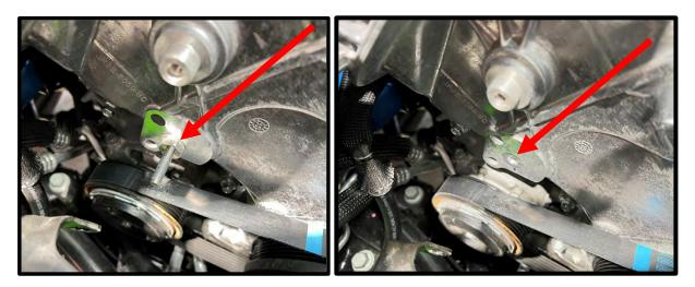
60. (Auto Transmission) Remove the U shape hose from the factory tee's. Cut 1 3/4" from the long end as shown.
