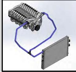
122. Install hose #3103410 from offset Y, across front of engine to **LH rear** most IC fitting (inlet). Use supplied #16 silver worm clamp to secure hose to tee and #16 Black clamp to IC fitting. **NOTE:** Routing IC hose incorrectly can result in poor performance and potential damage!
