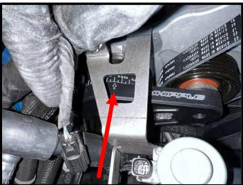
97. With belt holding the SC pulley in position, torque the supercharger (5x) 6mm x 14mm SHCS bolts to 130 lbs-in using a 5mm allen socket. Do not use Loctite on threads, it is not required.
