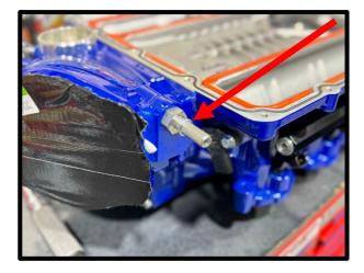
107. Mount EECPV bracket to SC lid, use (2x) 6mm x 10 HHFCS. Torque to 80 lbs-in using 10mm socket. Slide EECPV to bracket. Connect factory plastic quick connect fitting to EECPV until it clicks and locks in place. Connect 2-way electrical connector to EECPV, press locking tab back in place.
