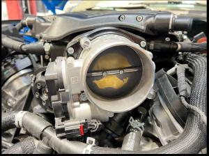
137. (Stage 2 Whipple 112mm TB) Install throttle body to supercharger inlet, use the supplied gasket. Secure TB with the supplied (4x) 6mm x 45mm SHCS using 5mm allen socket. Torque to 89 in-lbs. Install the 120mm to 112mm rubber sleeve over TB flange for later installation.
