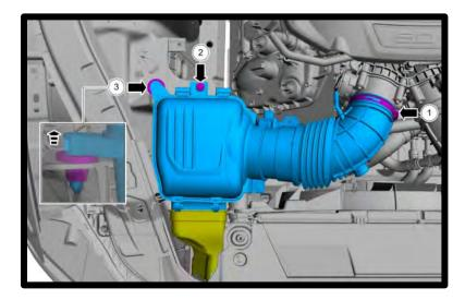
34. Disconnect the MAF sensor, MAF sensor retainer and remove make up air hose from air tube.
