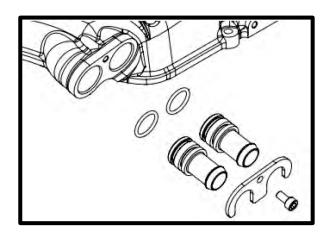
103. Connect factory passenger side rail fitting to the DI pump factory hose, press until it clicks and locks in place. NOTE:
