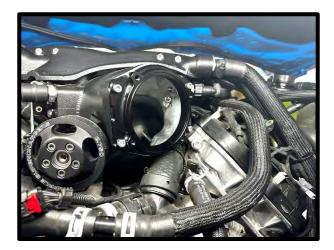
136. (**Stage 1 92mm TB**) Install supplied (1x) #2-045 V75BR oring to TB adapter. Install the stock throttle body using the (4x) 6mm x 35mm HHFCS bolts using a 10mm socket.
