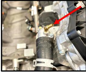
56. Trim the reservoir vent line right at the ENG printing on hose. Reinstall stock hose to new fitting. Secure with supplied #4 clamp.
