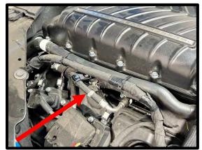
104. Connect factory fuel inlet line to the driver side fuel fitting, press until it clicks and locks in place.
