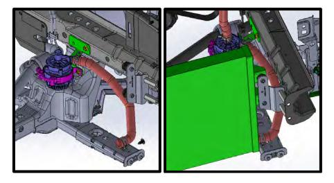
120. Install hose #3103409 from LTR **RH top** (outlet) fitting. Route to frame rail next to airbox snorkel. Install offset Y to end of hose. Use supplied #16 pinch clamps to secure hose.
