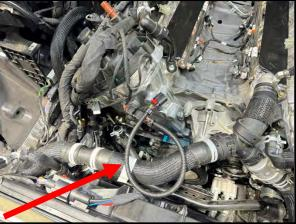
85. Remove plastic harness retainers from loom at the back of the engine.
