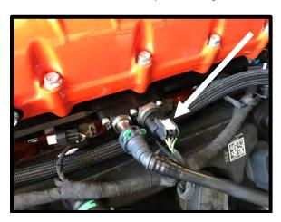
106. Install (1x) #906 oring to the supplied (1x) -6 ORB to 9.89mm quick connect fitting. Install fitting to the **LH** side port using an 11/16" socket.
