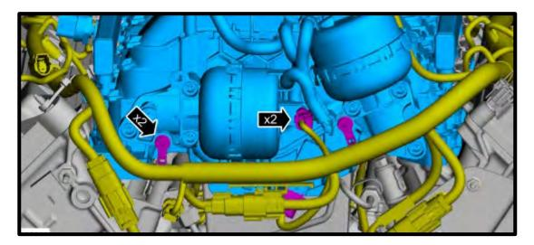
46. Clean the intake manifold to cylinder head surface using carb cleaner or acetone. Install tape over the exposed ports until manifold installation.
