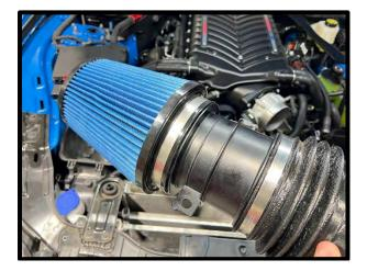
142. Install the MAF housings to the airbox brackets using supplied stock fastener to supplied brackets.
