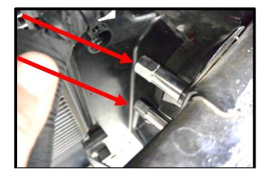
113. Install the LTR brackets to the LTR using the supplied (4x) 8mm x 35mm FHSCS bolts through the aluminum heat exchanger spuds (5mm allen socket). NOTE: HD heat exchanger mounts the same way but the inlet fitting moves to RH side (same as outlet).
