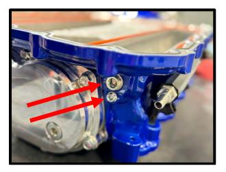
74. Using 27mm socket, remove the fuel PSI sensor from the factory fuel rail. Using 27mm socket, remove fuel PSI sensor from factory fuel rail. Install factory fuel PSI sensor to the fuel rail using a 27mm socket. Torque to 53 lbs-in, then an additional 25-degree rotation. **NOTE: Never use sealant on these threads.**
