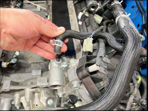
57. **(Auto Transmission)** Release the hose clamp from transmission fluid valve and hose facing down from tee. Remove plastic hose retainer from oil cooler solenoid hose.
