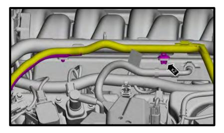
38. Detach the heater hose retainer. Remove the heater hose from both driver and passenger side of block by pulling locking tab back and pulling away. Position the heater hoses aside.
