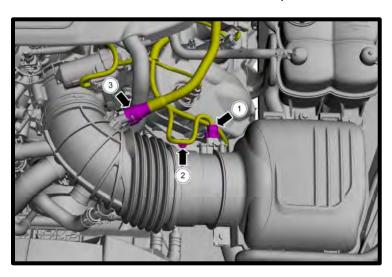
35. Loosen the hose clamp from throttle body using nut driver. Remove the air cleaner bolt. Detach the air cleaner from grommets and remove the air cleaner.
