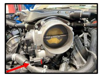
139. Install supplied (1x) 3/8" to 15.82mm hose adapter to the SC inlet tube.
