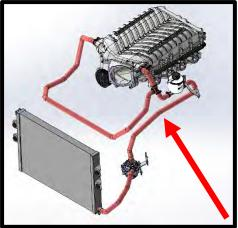
124. Install hose #3103406 from **LH forward** most IC fitting (outlet). Secure hose to IC fitting with #16 Black worm clamp. Install TEE fitting with TEE facing forward. Install supplied 90deg hose #3103158 to end of TEE and secure to front most IC filler reservoir fitting (inlet). Secure 90deg hose to tee and reservoir with #16 Black clamps.
