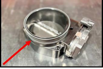
138. Connect previously installed throttle extension pigtail to the throttle body electrical connector. Secure wiring using zip-tie. **NOTE: Failure to secure wire may result in the wire catching the belt system!**
