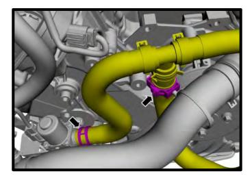
58. **(Auto Transmission)** Detach wiring harness retainer from transmission fluid valve bracket. Disconnect valve 2-way connector. Remove the fasteners to remove valve from engine.
