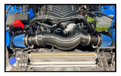
144. **(Stage 2)** Install inlet tube to the MAFs and throttle body. Secure using the supplied clamps, (3x) #80. Reconnect MAF connectors to MAF sensors.
