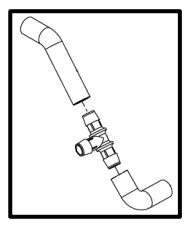
125. Install hose #3103411 from TEE forward facing fitting (outlet). Secure hose to TEE fitting using supplied #16 Black worm clamp. Route #3103411 across front of the motor to **RH forward** most IC fitting. Secure hose to tee with #16 Black clamp. Zip tie both this and the feed line that goes in the same path together.
