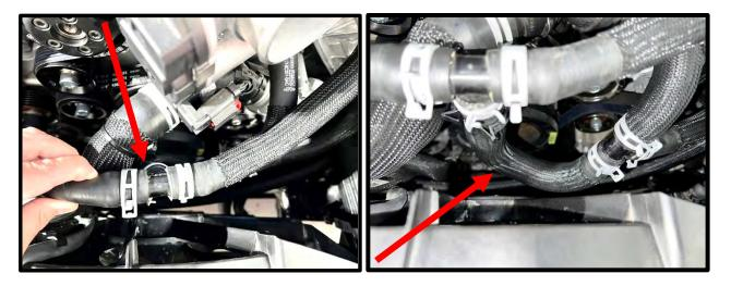
62. Using 5/16" nut driver, secure hose using supplied #24 hose clamp. Rotate the clamp at water neck towards the driver side for future clearance of the SC.
