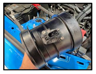
141. Install supplied filters to MAF housing, secure using supplied filter clamp. Install the MAF housings into the Y tube (for ease of installation), pre-install #80 hose clamp to Y tube, leave loose until later.
