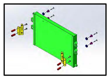
114. Slide the LTR assembly up from the bottom. Connect the LTR brackets to the coupling nuts using the supplied (4x) 8mm x 16mm hex headed flanged bolt (12mm ratchet wrench).
