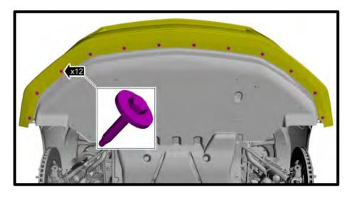
11. **(GT ONLY)** Remove the (22x) fasteners and (3x) push pin from the underbody shield. Remove shield from vehicle.
