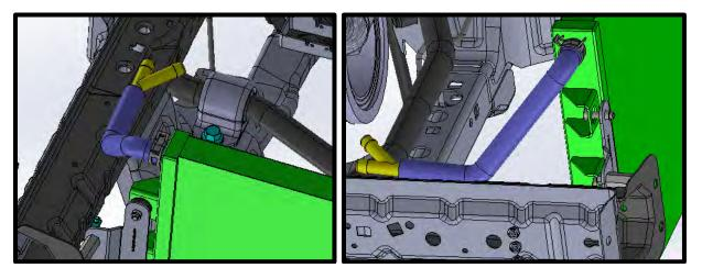
121. Install hose #3103408 from offset Y straight to **RH rear** most IC fitting (inlet). Use supplied #16 silver worm clamp to secure hose to Y and #16 Black clamp to IC fitting. **NOTE:** Routing IC hose incorrectly can result in poor performance and potential damage!
