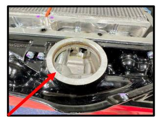
101. Apply generous amount of grease to the (1x) #2-230 Viton bypass oring. Install the supercharger lid to the supercharger housing by carefully placing the bypass down. Secure the SC lid using the (17x) 6mm x 30mm HHFCS and (3) 6mm x 70mm HHFCS (*marked green*) using the following pattern. Torque to 90 lbs-in using an 8mm socket.
