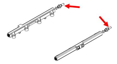
78. Install fuel injectors to the fuel rail, apply generous amount of grease to oring for easy installation. Install supplied fuel injector position lock bracket to clock the supplied fuel injectors into proper position. While installing lock bracket, secure fuel injectors so it doesn't add pressure to injector body. **CAUTION**: *Failure to clock the injector correctly can cause severe running issues*.
