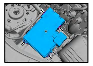
31. Fully loosen the BCM bolts. Release the clips (2x) and position aside the BCM.
