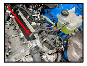
54. Loosen water Y junction. Remove water neck by removing the (2x) fasteners.
