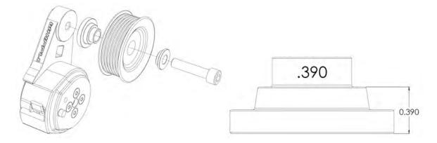
68. Carefully bend the factory AC line down and towards passenger side. Install spring loaded tensioner to plate to check clearance. You should have a minimum of 3/8" of clearance from the tensioner to the AC line.
