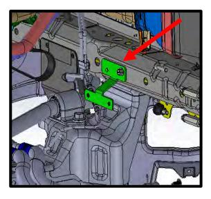
118. Mount IC pump clamp to the pump bracket using (2x) 6mm x 8mm HHFCS bolts. Install pump to clamp, pump inlet should be facing the front of the vehicle. Leave loose until IC hoses are installed.
