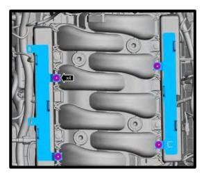
41. Remove the left and right fuel rail insulators, these will no longer be used.
