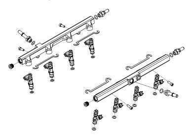
79. Apply generous amount of grease to injector orings for ease of installation. Install supplied fuel injectors, rails and lock bracket to intake manifold, secure with the (4x) 6mm x 16mm SHCS using a 5mm allen socket. Use **Blue Loctite** #243 on the threads of each bolt. Torque to 90 lbs-in.
