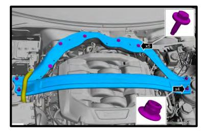
27. **(RHD ONLY)** If equipped, remove the strut tower brace by detaching the battery wire retainer. Remove the (4x) nuts and (6x) bolts. Reinstall factory nuts (4) and torque to 41 lbs-ft.
