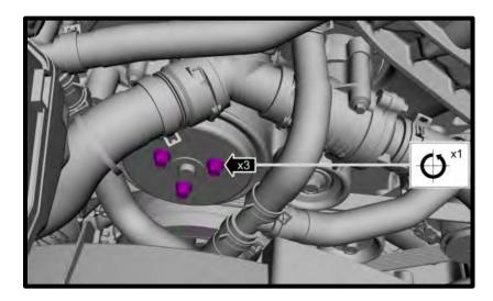
48. Remove the belt from the engine by using a 15mm socket on a ½" breaker bar and rotating the spring-loaded tensioner in a clockwise direction.
