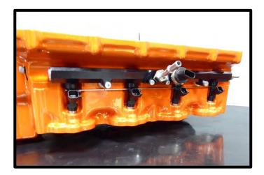
80. Install supplied 3/8" fuel cross over line around back of the supercharger by pressing until they click and lock in place. \*NOTE: The 90deg end goes to LH side.
