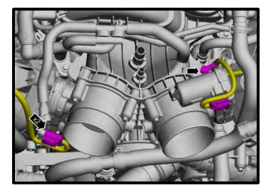
37. If equipped, detach the wiring harness retainers.
