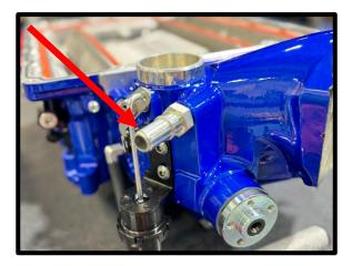
110. Install supplied 1/2" ID x 9" hose (#3103159) to the passenger side valve cover. Connect other end to supercharger inlet quick connect fitting. Push until it clicks and locks into place.
