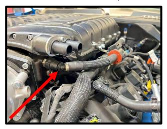
109. Install (1x) supplied #906 oring to the (1x) -6 ORB to 15.82mm quick connect fitting. Install fitting to **RH** side on the inlet using a 7/8" socket.
