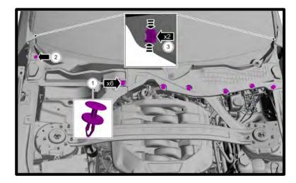
25. Remove the (5x) push pins (1) and depress the (2x) clips (2). Lift and then pull cowl panel grille out and remove.
