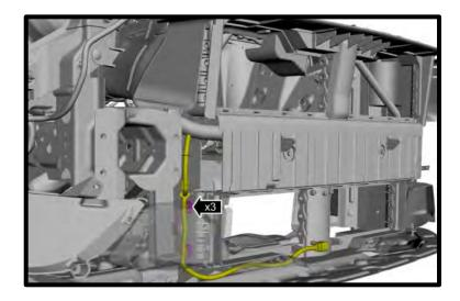
21. Remove the (6x) bolts and position active grille shutter forward.
