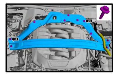
28. Lift and remove cover from the engine.
