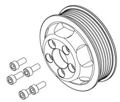
95. Reinstall water pump pulley using a 10mm socket, torque to 14 lbs-ft.
