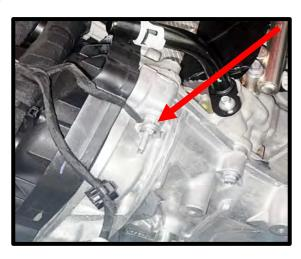
65. Use supplied (4x) 8mm x 90mm in the (3x) lower holes to secure the idler plate to the front of the passenger side of engine, install hand tight. Using a 6mm allen, torque to 22 lbs-ft.
