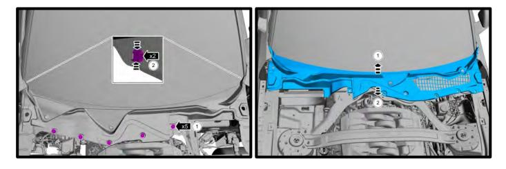
26. **(LHD ONLY)** If equipped, remove the strut tower brace by detaching the battery wire retainer. Remove the (4x) nuts and (5x) bolts. Reinstall factory nuts (4) and torque to 41 lbs-ft.
