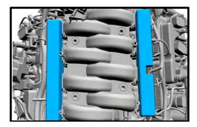
42. Loosen the (4x) bolts holding the fuel rails down, these go through to the cylinder head (10mm socket). Fuel rail does not need to be removed.
