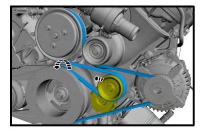
49. Remove the spring-loaded tensioner from the engine using a 13mm socket.
