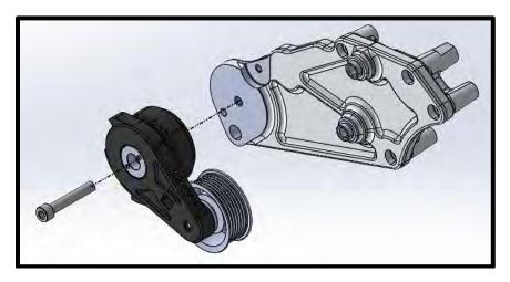
70. (**Auto Transmission**) Install supplied trans cooler solenoid bracket to the tensioner plate and engine block using (2x) 8mm x 20mm HHFCS. Torque to 120 in-lbs.
