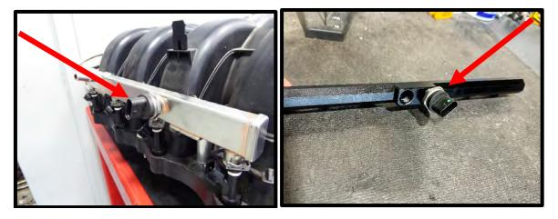
75. Install supplied (2) #2-906 Viton oring to (2x) 45mm long 9.49mm fuel fittings. Apply light amount of grease to oring for ease of installation and install fitting. Install fittings, one per rail.
