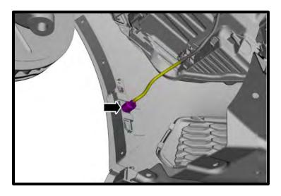
14. Disconnect the front bumper cover electrical connector.
