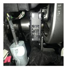
6. (Jeep Grand Cherokee/Durango) Remove the push pins on the passenger side carpet silencer panel. Connect HP Smart Access Cable to the correct connector.
