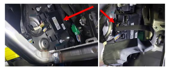
5. (Ram) Under the dash, near the E-brake, locate the security module. Connect HP Smart Access Cable to the correct connector.
