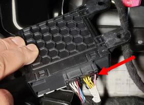
3. (Charger) Use plastic trim tool to unclip and lower dash section under steering column.
