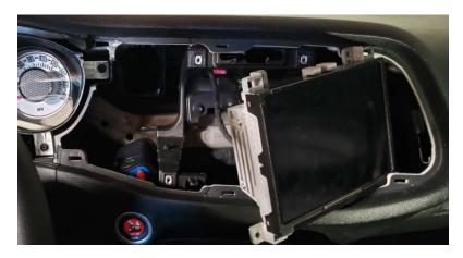
2. (Challenger) Locate the security module behind the radio. Remove the (3) screws to get access to the module. Connect HP Smart Access Cable to the correct connector (yellow and pink wires in this application).
