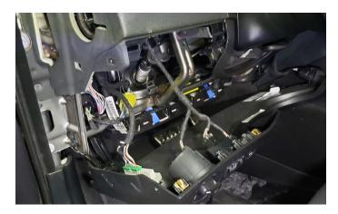
4. (Charger) Locate the security module above the OBD port. Connect HP Smart Access Cable to the correct connector (yellow and pink wires in this application).
