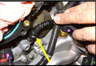
18. Remove the (8) cable ties securing the wire harness to the intake manifold cover (these will not be reused).
