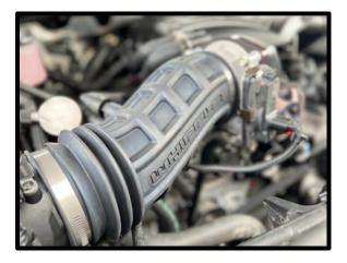
107. Route the throttle extension under the air inlet tube, connect to throttle body and stock connector. Secure harness in clips, away from the belt. **NOTE**: Support wires when pressing together on female extension to stock harness.
