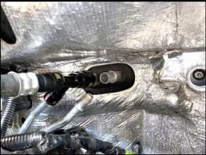
31. **(14-18 TRUCK ONLY)** Remove the two heater hoses from stock heater tube fittings for easier install. These will be reinstalled later in install.
