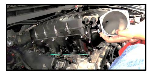
45. Apply light amount of **Loctite #242** to the (10) 6mm x 30mm HHFCS bolts. Install bolts to runners, using 10mm socket. Hand tighten at this time. **\*NOTE**: Use a ¼" socket and drive set for installation, failure to do so will potentially cause interference with a 3/8" type socket and counter bore. **\*\*These will be torqued in a later step.**
