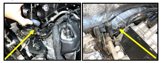
58. Install the supplied preformed IC inlet hose #3103144 to the LH rear fitting. Route around the back of the SC to RH side of engine. Install supplied Y fitting to end of this hose. Install supplied hose #3103145 to RH side, rear IC inlet fitting. Route other end to the Y fitting. Secure hose to the IC inlet fittings with supplied black 16mm-27mm black worm clamps. Secure other ends with supplied #16 pinch clamps. NOTE: DO NOT MIX UP!
