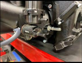
36. Install the (3) #2-906-V75BR orings to the (1) 9.89mm fitting and (2) -6 ORB plugs. Install the (1) 9.89mm fitting and (1) -6 ORB plug to the SC inlet RH side of inlet. Install the (1) -6 ORB plug to on LH side of inlet. Apply light amount of grease to oring to ease installation
