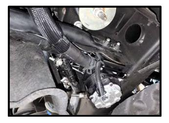
96. Install the supplied 9.49mm coupler fitting to stock fuel feed line coming from firewall. Connect the supplied female to female jumper fuel line supplied between the stock lines.
