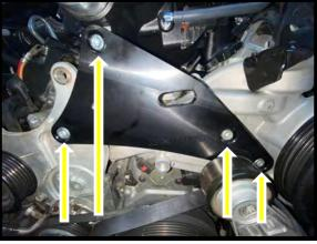
47. Secure supercharger to cylinder heads using the supplied (10) 6mm x 30mm HHFCS. Torque to 44 in-lbs on first pass, follow with a final torque to 89 in/lbs. \*NOTE: Use a ¼" socket and drive set for installation, failure to do so will potentially cause interference with a 3/8" type socket and counter bore.
