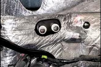
32. **(14-20 SUV ONLY)** Using a pipe over the heater tube, lightly bend towards RH (passenger side) of vehicle. For reference, the goal is to move the end of the fitting between ½" to ½" for clearance to the supercharger. This hose will be reinstalled later in install.
