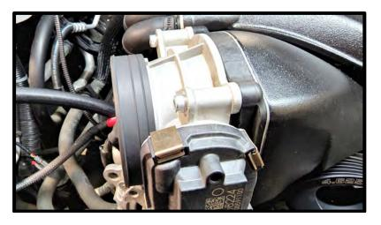
102. (5.3L Only) Install supplied rubber boot to throttle body flange.
