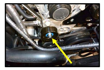
50. Reinstall alternator in stock location, using factory hardware. Torque to 25 ft-lbs. Connect the alternator 2-way connector and power wire. Reinstall AC line support bracket when applicable.
