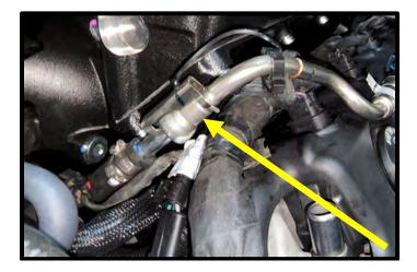
56. Install the supplied 3/8" ID PCV hose #3103248 with the dual 90deg 9.89mm fittings to the valley tray quick connect fitting (straight end). Route the hose and the 90deg up towards driver side. Connect 90deg fitting to driver's side rear fitting on inlet of SC. Push until it clicks and locks in place.
