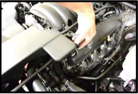
8. Disconnect the MAF sensor connector by pulling up on the red safety clip, and then squeezing the connector while pulling up.
