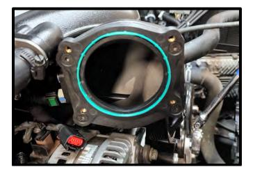
101. **(5.3L)** Use the supplied (4) 6mm x 40mm SHCS flange bolt to secure throttle body to throttle body adapter using a 10mm socket, torque to 80 in/lbs. **☞Loctite™ (#242 blue) threads.**
