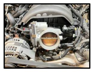
15. Remove the (2) air duct support stands from the intake manifold using a 10mm wrench or deep-well socket. Remove the (2) fasteners located in the back securing the intake manifold cover to the intake manifold using a 10mm socket.
