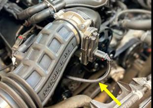
108. Install the driver side ½" x 27" PCV/Vent hose to the quick connect fitting on the passenger side valve cover. Route under the SC, to the bottom port on the inlet tube. Push until it locks in place.
