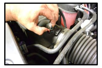
9. Loosen the hose clamp using an 8mm nut driver that secures the MAF housing to the stock air induction tube and the hose clamp holding the air induction tube to the throttle body. Lift the factory air ducting away from engine.
