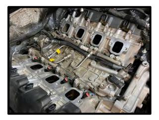
44. Install the supercharger assembly to the engine. You'll have to slide the last few inches as firewall clearance is minimal. Pay close attention to the orings, ensure they don't fall out or move. Do not tighten or secure at this time (must do after belt system is installed). NOTE: Be careful of PCV valve during installation.
