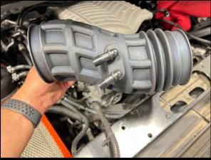
106. Install the supplied Whipple air inlet tube to the factory MAF housing and secure with the supplied #64 clamps. Install other end of inlet to the supplied silicone hose to the factory throttle body using supplied clamp.
