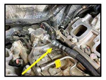
34. Route new feed line as shown, under the DI cross-over fuel line. Ensure that the line can't kink, bend or rub any sharp edges.
