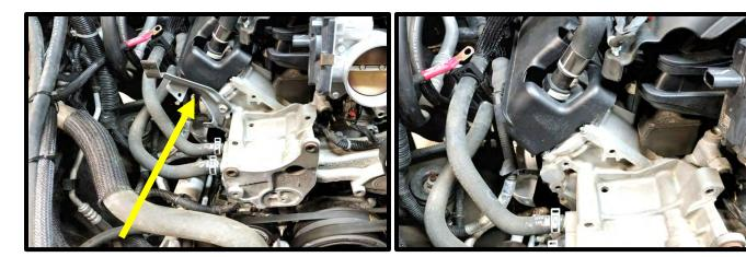
27. Disconnect coolant sensor 2-way connector. Remove vent line from thermostat housing by releasing pinch clamp. Remove thermostat housing outlet hose from thermostat housing by releasing pinch clamp. Remove coolant temp sensor temporarily.
