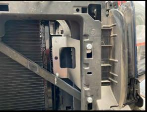
77. Mount the LTR to the brackets using the supplied (4) 8mm x 16mm FHSCS and (4) .813" sleeved washers. Torque to 16 ft-lbs. **NOTE**: Images show from the back of the LTR.
