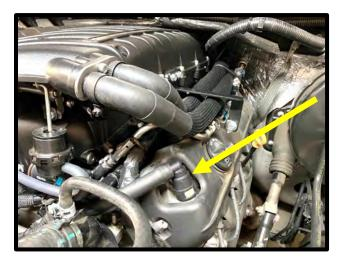
61. Reinstall stock coolant temperature sensor to factory location. Reinstall stock thermostat housing with stock oring and stock fasteners. Torque to 89 in-lbs. Reinstall degas bottle vent line to thermostat housing using stock clamp. Reinstall thermostat housing outlet hose to thermostat housing using stock clamp.
