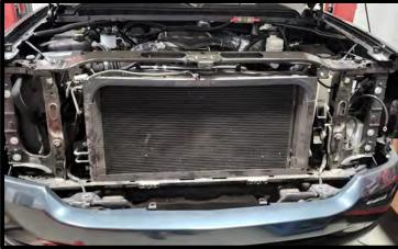
73. With the vehicle on a lift or jack stands, locate the (2) front frame support bolts (RH side of frame rail). Using a socket, loosen the 2 bolts. Install IC pump bracket over and behind stock bolts. Retorque to 22 ft-lbs.
