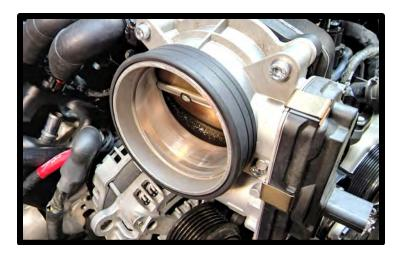
103. **(6.2L)** Install the supplied gaskets on both sides of the throttle body adapter. Use the supplied (4) 6mm x 60mm HHFCS bolts to mount the stock throttle body to the SC inlet using a 10mm socket. Torque to 89 in/lbs.
