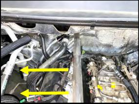
33. Install supplied fuel line to DI pump. Install the stock security lock on the fuel pump. Position to the side as shown in the image to properly clear the supercharger.
