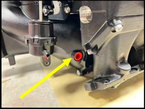
37. Install supplied bypass reference hose from bypass to SC inlet 1/4" barb fitting.
