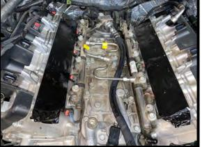
35. Apply light amount of grease to stock EVAP solenoid oring. Mount the stock EVAP solenoid to SC inlet using the stock EVAP bolt. Torque to 90 in-lbs.
