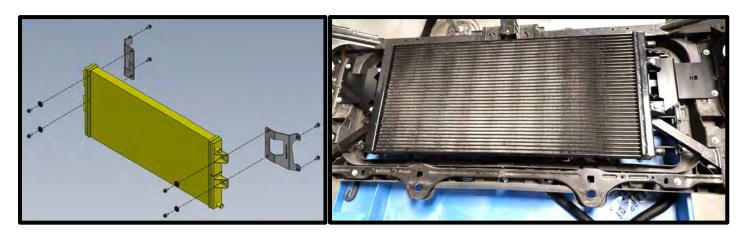
78. **(TRUCK)** Mock up the plastic radiator closeout. For top fitting, cut approximately a 2" square for hose clearance. For the bottom fitting, cut a 3" x 4" section away for hose clearance.
