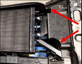
79. Pre-route the supplied IC to LTR hose. Install #3103255 to the bottom fitting. Secure with supplied pinch clamp.
