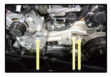
43. Remove the tape you previously installed on the intake manifold. Clean the cylinder head surface in preparation for supercharger installation.
