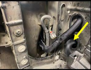
86. Install the preformed hose #3103256 from the LTR outlet (top fitting), under the airbox to the previously routed Y fitting feeding intercooler (rear fittings). Secure hose using supplied #16 pinch clamp. **NOTE**: Secure hose with zip ties for clean installation.
