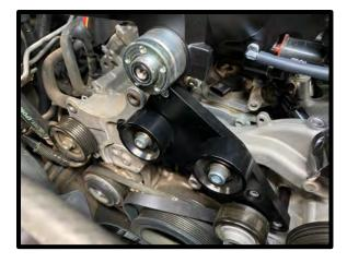
52. Install the supplied supercharger pulley using the supplied (5) 6mm x 14mm SHCS to secure. Torque to 119 in-lbs using a 5mm allen socket. Use the 6-rib belt to hold the pulley in place to torque. **NOTE:** Loctite or thread locker is not required or needed.
