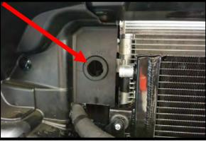
132. Route the supplied 90deg intercooler feed hose #COYO-2006 through the grommet, cut to fit as needed. Install the supplied Y fitting to the end of the hose from the outlet of the LTR, just after the grommet. Secure hose to LTR and hose to Y fitting using supplied constant tension clamps.
