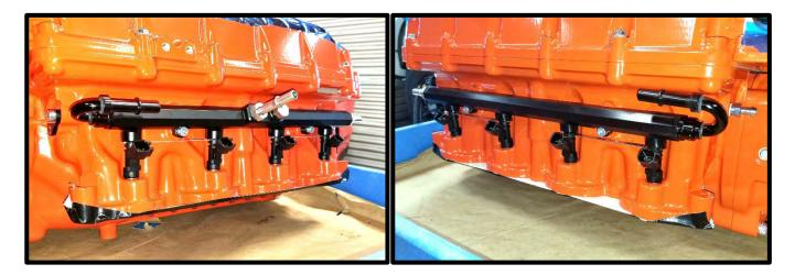
82. Install the supplied 3/8" fuel cross over line around the back of the supercharger by pressing until they click and lock in place. It's also possible to leave off until after SC is installed for easier access to rear bolts. \*Note: The 90deg end goes to bank 2 side.
