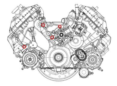
69. Use supplied (4) 8mm x 90mm SHCS to secure the idler plate to the front of the passenger side of engine, install hand tight. Using a 6mm allen, torque to 22 lbs-ft.
