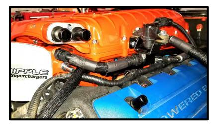
106. Install the supplied 3/8" x 20 ½" hose with dual 90deg 9.49mm quick connect fittings from the EVAP solenoid rear fitting to the EVAP fitting located under the brake booster.
