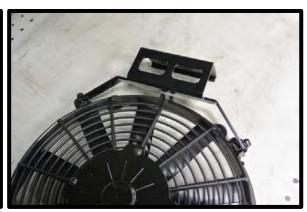
115. (Dual fan installation) Carefully set both fan assemblies on top front of the LTR, space these evenly before installing.
