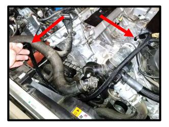
58. Reinstall the factory coolant overflow hose to the new supplied tee fitting on the driver side. Secure using factory pinch clamp.
