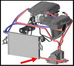
129. **(HD LTR)** Use the supplied ¾" coupler and (2) pinch clamps to couple the ¾" x 20" hose to the ¾" x 31" extension. Route the 180deg end to the LTR inlet. Secure using constant tension clamps.
