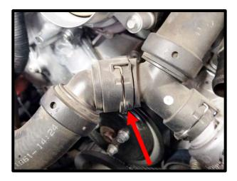
37. Carefully disconnect the factory fuel feed hose from the fuel rail. The fuel system may still have pressure, use protective eyewear and multiple rags to catch any possible fuel leak. To release, press the blue safety latch and pull the fuel fitting away from fuel rail.
