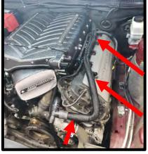
55. Transfer stock oring from stock water neck to new water neck. Apply pipe sealant to threads of 1/8" NPT to 5/16" 45 Deg fitting. Install fitting to water neck, rotate so it ends facing directly towards driver side. Install water neck to motor using stock fasteners (10mm socket), torque to 89 lbs-in.
