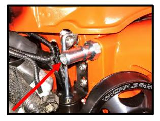
109. Install the supplied PCV hose to the passenger side valve cover. Connect other end to the supercharger inlet quick connect fitting. Push until it clicks and locks into place.
