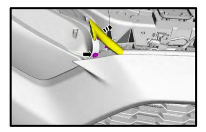
15. Remove the (6) screws from fascia. Lift the fascia up off the alignment pins, pull forward and off the vehicle. For reinstallation, torque to 48 in-lb.
