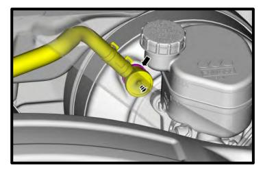
31. Remove the (4) nuts from the heater hose support using 10mm deep well socket, set heater hose aside, remove bracket.
