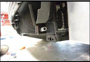
126. Install the supplied intercooler mounting bracket to IC tank using the (2) 6mm x 10mm BHCS. Mount clamp to the IC tank with the supplied (2) 6mm x 8mm HHFCS.
