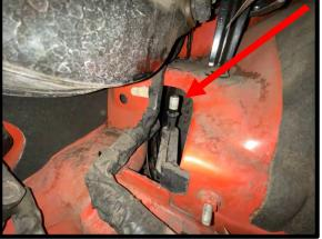
107. Install the supplied 3/8" ID x 24" with 55deg quick connect fitting. Route from brake booster to the **lower** quick connect fitting on the supercharger inlet. Push until it clicks into place. **TIP:** For best routing, nestle in between cam cover and fuel rail, under the wiring and heater hose.
