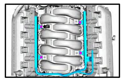
40. Loosen the (6) manifold to cylinder head bolts using an 8mm socket.
