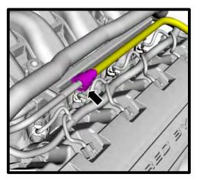
38. Remove fuel rail foam covers. Disconnect all fuel injector connectors by using a flat head screw driver on one side of the clip. Pry to one side and clip will slide off.
