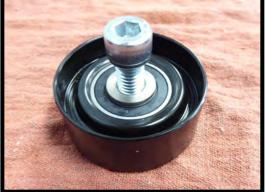
72. Assemble spring-loaded tensioner by mounting the supplied spacer with the female register to the tensioner. Install the grooved idler pulley (#36326) to the tensioner and (.390") step spacer. Use the supplied step washer to center the bearing and the 10mm x 40mm SHCS (10-Rib uses 10mm x 60mm SHCS) bolt to secure idler to tensioner. Use light amount of anti-seize on threads. Torque to 18 lbs-ft using 8mm allen socket. NOTE: Verify you're using the proper spacer as shown.
