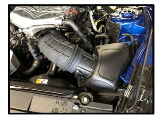
149. Install the factory MAF sensor element into the new MAF housing using the supplied (2) 4mm x 6mm SHCS. Torque to 17 lbs-in. \*\*DO NOT USE STOCK BOLTS\*\*. \*TIP: Verify arrow position for airflow direction.
