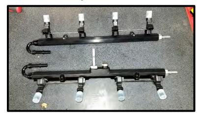
81. Apply generous amount of grease to the injector orings for ease of installation. Install the fuel injectors, rails and lock bracket to the intake manifold, secure with the (4) 6mm x 16mm SHCS using a 5mm allen socket. Torque to 90 lbs-in.
