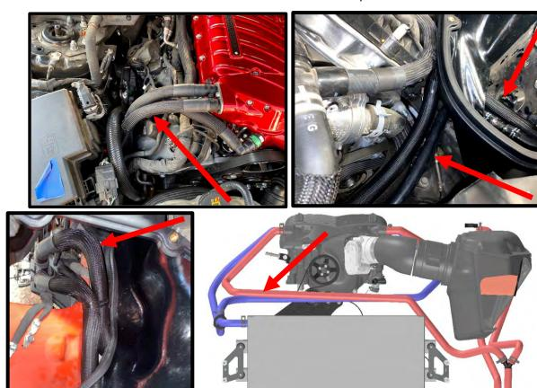
136. Install the supplied ¾" ID IC tank to filler tee, ¾" bank 1 intercooler outlet to the plastic Y fitting. Install the 3/8" ID IC filler tee to IC reservoir hose to 3/8" barbs. Secure all with supplied constant tension clamps.
