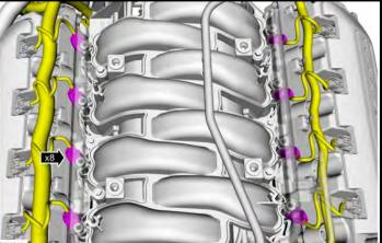
39. Loosen the 4 bolts holding the fuel rails down, these go through to the cylinder head (10mm socket). Fuel rail does not need to be removed.
