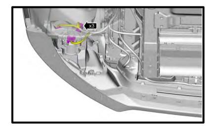
11. Remove the bolt and separate the front bumper cover from the fender bracket. For reinstallation, torque to 15 in-lb.
