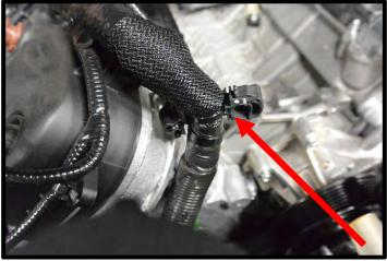
26. Disconnect the couplings and remove the crankcase vent tube. Disconnect EVAP purge valve electrical connect and disconnect EVAP tube.
