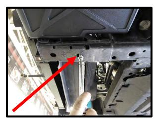
125. (**Standard LTR**) Using a hacksaw, notch the plastic shrouding next the heat exchanger inlet fitting. Use the supplied <sup>3</sup>/<sub>4</sub>" ID x 20" hose with 90deg end (from pump outlet to LTR inlet). Secure both ends with constant tension clamps supplied.
