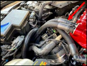
134. Install the supplied preformed 3/4" x 48" hose to upper Y-fitting and secure with constant tension clamp. The straight end goes to the Y. Route between the engine and radiator to LH side of vehicle. Leave this end loose until airbox installation. Secure hose to factory heater lines using zip-ties. **NOTE:** Failure to secure line will result in hose hitting belt system.
