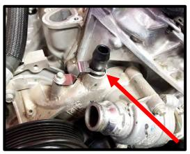
53. Install the supplied tee and 90deg hose to the driver side heater tube you just installed. Secure with supplied constant tension clamp on the 90deg hose to heater tube.
