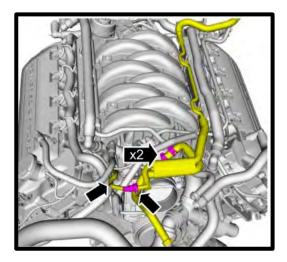
25. Carefully cut the electric tape securing the ETC wires to the throttle body. Disconnect the electronic throttle electrical connector by pushing up on the safety lock and then squeezing the connector and pulling away. Remove the harness support plastic tab from the block ground stud. Remove plastic tab from loom, this will be too close to belt leter.
