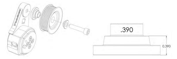
73. Carefully bend the factory AC line down and towards passenger side. Install spring loaded tensioner to plate to check clearance. You should have a minimum of 3/8" of clearance from the tensioner to the AC line.
