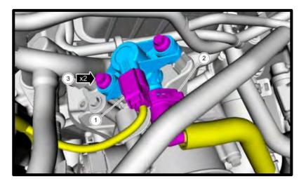
29. Remove the EVAP tubing from driver side valve cover (remove support from valve cover) and down below brake booster.
