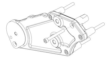
91. Torque the (10) 6mm HHFCS manifold bolts in the following pattern using a 10mm socket. First pass: 88 lbs-in. Second pass: 106 lb-in. **NOTE:** For bolt #10, a ¼" socket with 4"-6" extension, 10mm wobble is the best possible tool to get into this tight area.
