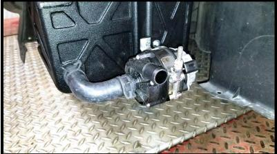
128. Install the supplied 180deg hose to the IC pump outlet. Route to LTR LH inlet fitting. Secure with constant tension clamps.
