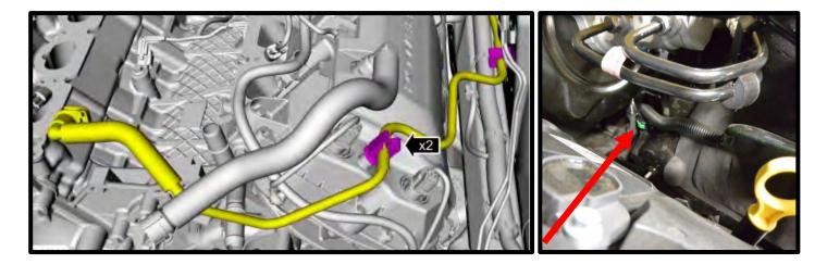
30. Using a pinch clamp tool, remove the brake booster line that connects the brake aspirator rubber line from brake booster check valve.
