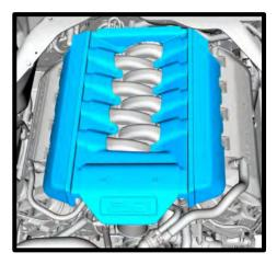
19. Remove the upper cowling for K-brace access. Remove the (7) push pin retainers and (2) tabs on the cowling. Lift up the cowl trim panel and remove the (4) nuts and (5) bolts from the K-Brace using a 13mm socket, remove from vehicle for later installation.
