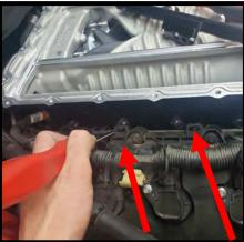
89. Install the supercharger housing (without lid) to the engine. Use the supplied (4) 6mm x 55mm HHFCS on the outer bolt holes and (6) 6mm x 80mm HHFCS bolts with the supplied (6) #2-009 orings on the bolt, under the head. Use **Blue Loctite #243** on the threads of each bolt. Leave hand tight for now.
