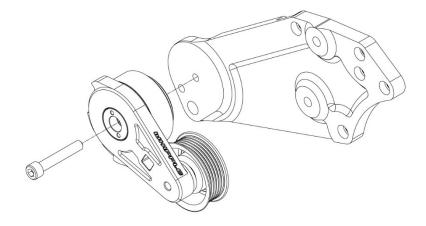
75. Install supplied (2) smooth aluminum idler pulleys (#3102717) to the idler plate using the (2) (.317") step spacers. Sandwich the idler pulley to the (2) (.317") step spacer using the supplied (2) step washer, (2) ½"-13 x 2" SHCS. Torque to 30 lbs-ft. using a 3/8" allen socket. Use light amount of anti-seize on threads. NOTE: Verify you're using the proper spacer as shown.
