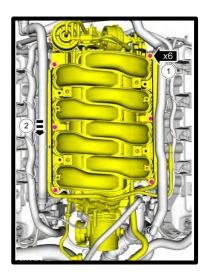
41. Remove the intake manifold from the engine. Pull up from the front then remove the (2) wire harness push pin supports from the back of the intake manifold and disconnect the (2) IMRC solenoid connectors and (2) IMRC position sensor connectors by pushing on the locking tab and pulling away IMRC solenoid.
