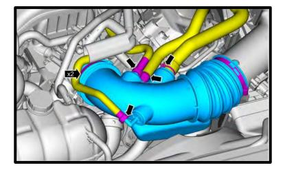
21. Disconnect the factory MAF connector by pulling back on the safety lock, then squeezing the unlocking tab and pulling back. Remove harness support from airbox lid, cut zip-tie from wire harness (not needed).
