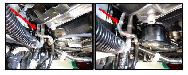
74. Install spring-loaded tensioner to idler plate, locating the tang into position. Secure with the supplied (1) 10mm x 60mm SHCS. Use light amount of anti-seize on threads. Torque to 25 lbs-ft using 8mm allen socket.
