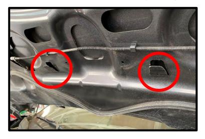
44. Using shears or saw, cut the stock stud from firewall .50" (to clear SC lid). Leave the clip as is to retain the firewall shrouding.
