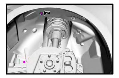
9. Remove the push pins and position the inner fender liner aside.
