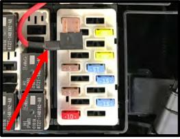
64. Mount the relay and fuse holder to the factory wire harness, secure with zip-tie. Route the 2-wire connector along the top of the condenser, to the LH side of the vehicle (near headlight) for later connection to IC pump. Secure harness using zip-ties.
