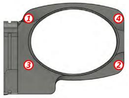
142. Install the supplied 38" 90deg rubber weather stripping to opening of airbox. This seals the bottom of the box to the inner fender area.
