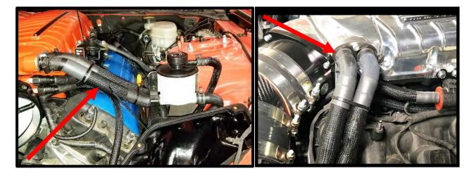
138. Connect the intercooler pump electrical connector to pump until its fully seated. Zip tie wires for clean installation.
