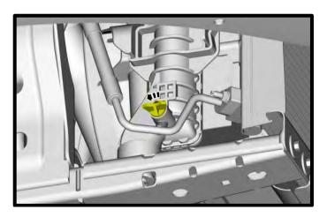
17. If equipped, remove the strut tower brace by removing the (4) factory nuts using a 15mm socket. This will not fit over the supercharger. Reinstall factory nuts (4) and torque to 25 lbs-ft.
