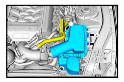
23. Remove the nuts from hose retainer bracket. Position heater hose aside and remove heater hose support.
