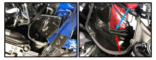
144. Install the steel MAF mounting plate to the airbox lid (to the inside of box). Install the (4) 5mm x 8mm FBHSCS bolts to secure plate to airbox lid. Install the MAF housing to the lid and venturi using the supplied (4) 6mm x 20mm SHCS bolts.
