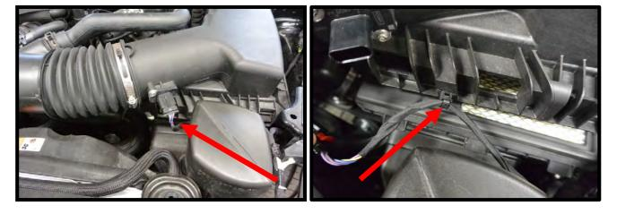
22. Detach the sound box from airbox. Remove the bolts securing airbox to vehicle, lift and remove airbox from vehicle.
