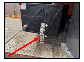
127. Install the intercooler pump to the water reservoir (leave slightly loose to position after hose installation). Install the supplied 90deg rubber hose and constant tension clamps to reservoir and intercooler pump. Once pump is in position, tighten clamp holding IC pump to reservoir. **Note**: Make sure pump outlet is facing directly out (not up or down).
