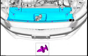
13. If equipped, remove the screws and the license plate bracket.
