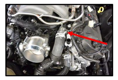
36. Remove the quick connect water fitting from the water neck to thermostat housing tee. Pull the locking metal wire, then pull connector back away from tee.
