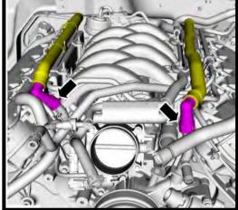
34. Remove the coolant to heater tube overflow hose using a pinch clamp tool. Pull away from heater tube.
