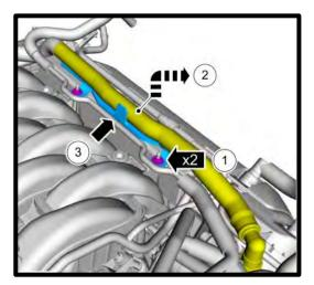
24. Disconnect the vacuum tube retainer and disconnect vacuum tube.
