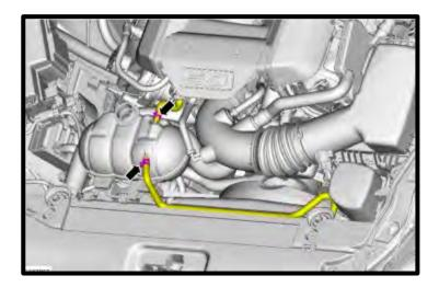
46. Remove the (2) bolts securing degas bottle and lift up and out of the way for easier installation of SC.
