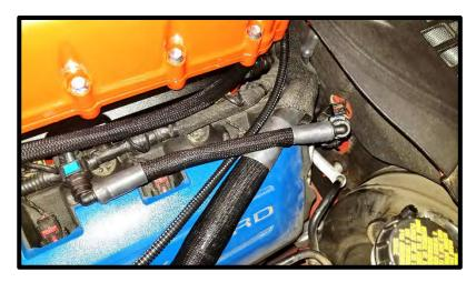
103. Install the (2) supplied 6AN viton oring (#906) to the (2) -6 ORB to 9.89mm quick connect fittings. Install these fittings to the passenger side lower 6AN fittings on the inlet using an 11/16" socket.
