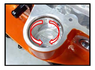
101. Apply generous amount of grease to the (1) #2-230 Viton bypass oring. Install the supercharger lid to the supercharger housing by carefully placing the bypass down. Secure the SC lid using the (17) 6mm x 30mm HHFCS and (3) 6mm x 70mm HHFCS (*marked green*) using the following pattern. Torque to 90 lbs-in using an 10mm socket.
