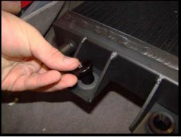
119. Install the LTR brackets to the LTR using the supplied (4) 8mm x 35mm FHSCS bolts through the aluminum heat exchanger spuds (5mm allen socket). **NOTE**: HD heat exchanger mounts the same way but the inlet fitting moves to RH side (same as outlet).
