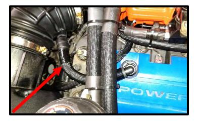
155. Connect the previously routed 1/4" vent line to the stock overflow tank, secure with stock clamp. Secure this hose to the radiator hose and heater hose using multiple zip-ties.
