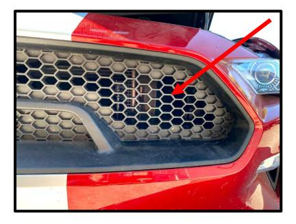
Stock fascia and grill has the main air feed through the center radiator area, the air makes a 90deg turn to factory snorkel.
