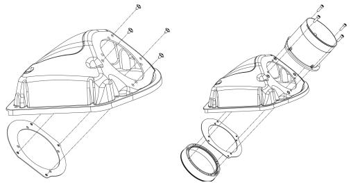
145. Install the high flow filter to the venturi ring you previously installed. Secure with supplied hose clamp.
