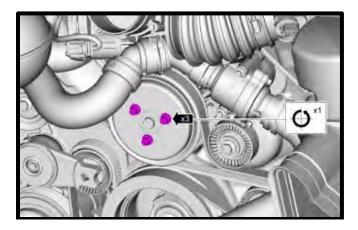
93. Install the supercharger pulley using the supplied (5) 6mm x 14mm SHCS using a 5mm allen socket. Leave hand tight until after belt installation.
