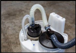
162. **(Stage 2)** Install the new connector harness supplied with the DW kit, the additional static ground inserts into the slot on the assembly filter, the same as OE.
