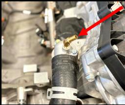
56. Using needle nose pliers, rotate the factory pinch clamp at the water neck towards the driver side for future clearance of the SC. **NOTE:** Image shows clamp with SC installed to illustrate max clearance.
