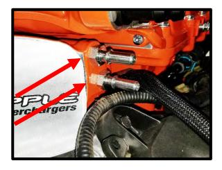
104. Install the EVAP to the supplied billet adapter with the electrical connector facing the back of engine. Install the supplied 9.89mm quick connect fitting and 6AN oring to billet adapter. Secure supplied EVAP bracket to the supercharger lid using the supplied (2) 6mm x 10mm HHFCS bolts. Secure EVAP assembly to bracket using the supplied (2) 6mm x 20mm HHFCS bolts.
