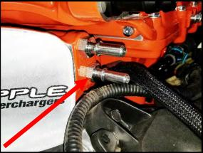
108. Install the (1) supplied -6AN viton oring (#906) to the (1) -6 ORB to 15.82mm quick connect fittings. Install this fitting to the RH side 6AN fittings on the inlet using a 7/8" wrench.
