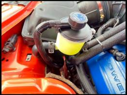
152. Install the previously routed hose from the Y fitting, to the LH core inlet fitting. Secure with worm clamp. **TIP: For hood clearance, ensure that the nut of the clamp is not on top**. Secure inlet and outlet lines with zip-ties for clean installation and protection from the belt.
