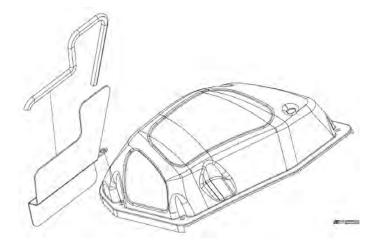
148. Install the supplied 3/8" to 5/8" hose adapter to the SC inlet tube. Install the inlet tube to the MAF and throttle body. Secure using the supplied clamps. #80 on MAF side, #56 for stock TB, #80 for 132mm TB, #88 for 150mm TB.
