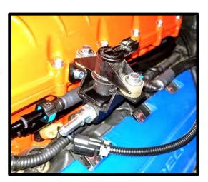
105. Install the supplied 3/8" ID x 4 ½" hose to the EECPV barb fitting and **upper** quick connect fitting (55 Deg) on SC inlet. Push until it clicks and locks into place.
