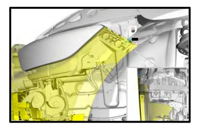
12. Using a panel puller, remove the factory inner hood insulator. This will not clear the SC system and will not be reused. Remove the factory plastic radiator shroud by pulling the center of the (8) push pins and then out. Use a flat head screw driver to pry the center head up. This will all be reused.
