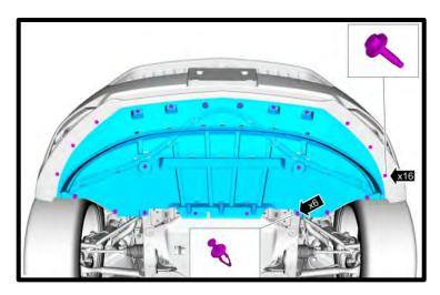
8. Remove the inner fender push pins.
