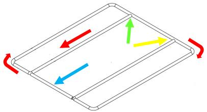
99. Install the supplied pre-formed 65.3" x .103" oring to the top sealing surface of the SC housing. Apply generous amount of grease to help ease the oring into place. **TIP:** To install oring into dove-tail groove, press vertically, vs sliding finger along.
