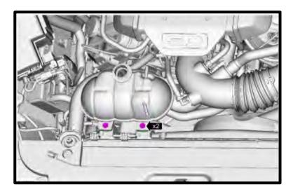
47. Remove the heater tubes from engine by removing the (1) bolt using an 8mm socket.
