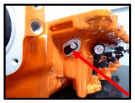
77. **(Complete Kits)** Install the supplied air temp sensor to the 3/8" NPT port on the back of the intake manifold. Be careful, as the plastic sensor can break if over torqued. Use light amount of oil on threads.
