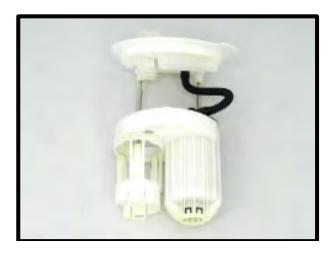
159. (Stage) Remove the (3) locating tabs and smooth the pump receptacle to the diameter of the DW400 (46mm).
