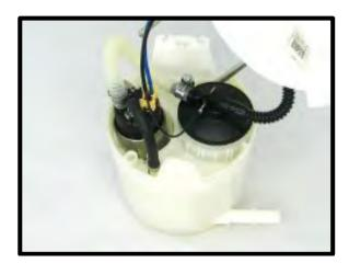
163. (**Stage 2**) Reinstall the hat to the assembly in the center/buckets assemblies and connect the electrical connector harness to the hat assembly.
