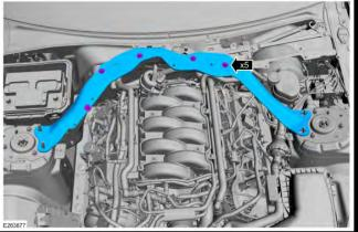
20. Disconnect and position aside the brake booster tubes, crankcase ventilation tube and resonator air inlet tube. Loosen the 2 clamps and remove the air cleaner outlet pipe.
