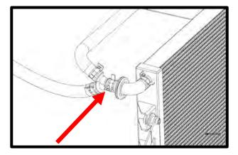
133. Connect the ¾" x 31" hose to the Y fitting lower fitting, secure with pinch clamp. Route to RH intercooler inlet, the rear most water cross fitting. Secure with the supplied worm clamp. For max hood clearance, ensure that the hex is not on top.
