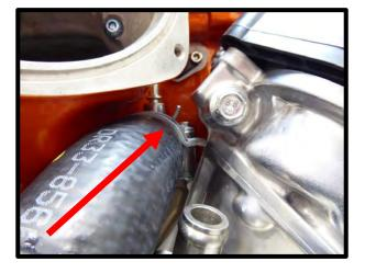
57. Install the supplied 1/4" to 3/8" (COYO-2700-R1) formed hose from the water neck vent line, route towards overflow tank for later installation. Secure with stock clamp.
