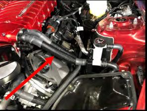
151. Install the supplied 3/8" ID x 31 ½" IC vent line (COYO-1400) and the ¾" ID x 24 ½" IC rubber hose (COYO-1300) to the filler neck. Both use the 90deg on the filler tee. Secure both with supplied pinch clamps. Route both below the airbox, to the IC reservoir. Secure both ends with supplied pinch clamps. Use multiple zip-ties to secure hoses together. Watch for hose kinks!
