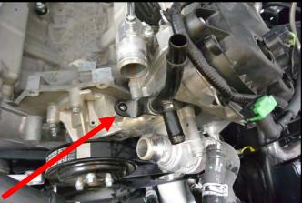
48. Loosen the (3) bolts securing the water pump pulley (while belt is on) using a 10mm socket. Remove the belt from the engine by using a 15mm socket on a ½" breaker bar and rotating the spring-loaded tensioner in a clockwise direction. Remove the spring-loaded tensioner from the engine using a 13mm socket (bolt will be reused later). Using 10mm socket, remove water pump pulley from engine (will be reused later).
