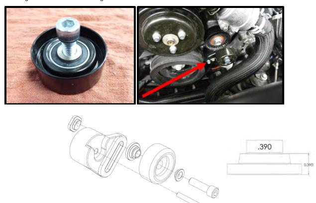
71. Remove factory plastic smooth idler pulley from the engine using 15mm socket. Replace with the supplied steel idler pulley (#36101). Use the factory fastener to secure. Torque to 18 lbs-ft with a 3/8" allen socket. **NOTE:** Image shows proper direction of idler pulley assembly.
