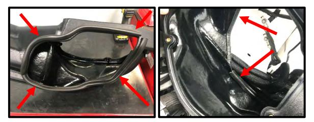
143. Install the supplied lower airbox to the vehicle by slipping over the factory air duct. Make sure the ¾" and 3/8" IC tank to filler tee hoses go in the allotted area. These should be zip-tied together for clean installation and free of any kinks.
