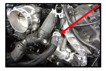
35. Remove the water neck hose using a pinch clamp tool. Pull away from water neck.
