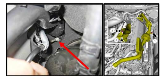
28. Remove EVAP purge valve from intake manifold for later installation.
