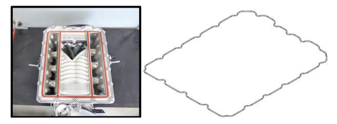
100. Install the (1) #2-230 internal bypass oring to the lid bypass passage. Use generous amount of grease to secure oring in place.
