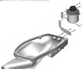
147. Install the filter lid to lower airbox by sliding filter into lower and tilting MAF side up. Once filter is in, you can lower the MAF side. Install the supplied heat shield to the front bolt hole closest to the radiator. Secure heat shield and the rest of the airbox lid with the (4) 6mm x 12mm FBHSCS bolts. Install the supplied 11" long rubber weather stripping to the top and rear lip of heat shield.
