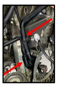
137. Install the supplied ¾" ID molded hose (enclosed air kit hose #18MST-1001A) (open air kit hose #18MST-1001) from the IC OUT fitting to the airbox area for later installation. Secure end with supplied worm clamp. TIP: The (2) hoses on this side should match in shape/form, therefore ensure it fits correctly. CAUTION: For hood clearance, ensure that the nut of the clamp is not on top.
