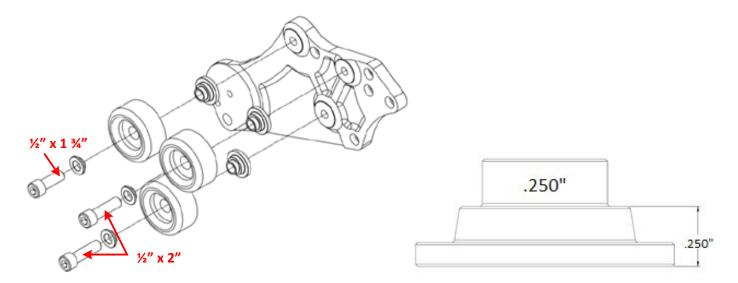
23. Install the supplied billet 10-rib grooved alternator pulley and secure using the supplied steel nut.
