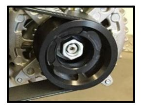
24. Install the supplied 10-rib water pump pulley. (15-17) Use the supplied (3) 8mm x 20mm SHCS. (11-14) Use the supplied (4) 8mm x 20mm SHCS. Torque to 14 ft-lbs.
