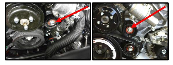
14. Using a 10mm socket, remove the (3) factory fasteners from the timing chain to head cover and (1) from water pump (for new idler plate).
