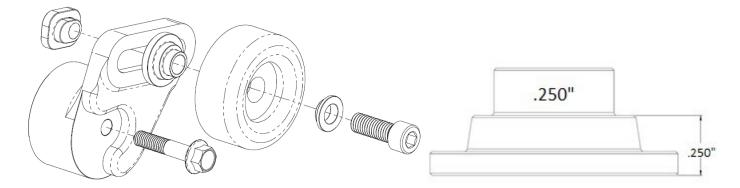
13. Remove the 6-rib smooth idler pulley from the engine. Replace with the supplied 10-rib "DEEP BORE" billet smooth idler pulley with the .260" back spacing to the factory location (PN #3102271), with the snap ring facing the engine. Use the supplied 8mm x 35mm SHCS with the **8mm step washer** to secure. Torque to 22 lbs-ft. **NOTE: This pulley is different spacing than all other pulleys supplied, it does NOT use a step spacer.**
