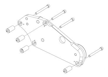
17. Preinstall the supercharger support bracket by installing on the back of the idler plate. Secure with the (1) 8mm x 70mm SHCS and (1) 8mm x 25mm SHCS, leave loose until supercharger assembly.
