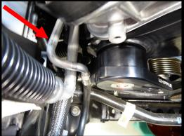
21. Install the spring-loaded tensioner to idler plate, locating the tang into position. Secure with the supplied (1) 10mm x 60mm SHCS. Use light amount of anti-seize on threads. Torque to 25 lbs-ft.
