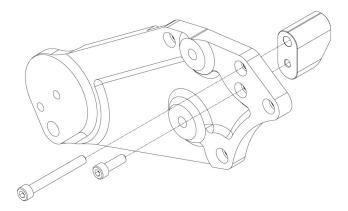
19. Assemble the spring-loaded tensioner by mounting the supplied spacer with the female register to the tensioner. Install the grooved idler pulley to the tensioner and (.390") step spacer. Use the supplied step washer to center the bearing and the 10mm x 50mm HEX bolt to secure idler to tensioner. Use light amount of anti-seize on threads. Torque to 18 lbs-ft.
