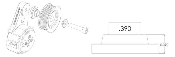
20. Carefully bend the factory AC line down and towards passenger side. Install spring loaded tensioner to plate to check clearance. You should have a minimum of 3/8" of clearance from the tensioner to the AC line.
