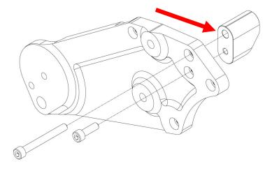
18. Using a 6mm allen socket, secure the (1) 8mm x 70mm SHCS and (1) 8mm x 25mm HSCS to the front support bracket. Torque to 22 lbs-ft. NOTE: If there is a fitment issue to SC inlet here, you will need to loosen the (10) supercharger to cylinder head bolts to relieve SC, torque inlet to plate and then retorque supercharger to heads.
