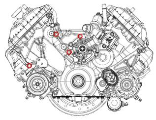
15. Install the (4) support stands to the front idler plate. These are loose fit; therefore, you must tilt backwards during installation or the stands will fall. You can use masking tape to help hold in place during installation if installation becomes difficult. *Each support stand is marked with an identifying number, as well as the idler plate for ease of placement*. **TIP:** Assemble together with the number facing out for future reference.
