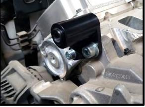
60. Install smooth 74mm supplied pulley to bracket using the step spacer and (1x) 10mm x 30mm HHFCS. Torque to 22 ft-lb.
