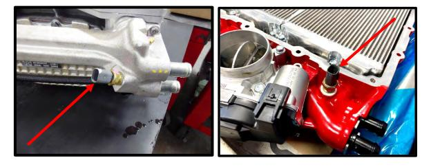
43. Install the supplied -6 ORB with oring to 15.82mm fitting to RH port on SC inlet. Use light amount of grease on oring for ease of installation.
