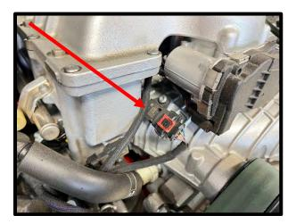
14. Remove EVAP vent line from supercharger inlet duct. Release vent line from plastic clamp located on intake manifold.
