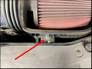
19. Remove stock cold air snorkel from airbox for later installation to Whipple airbox.
