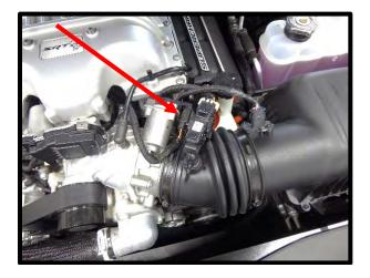
13. Disconnect inlet pressure sensor on supercharger inlet.
