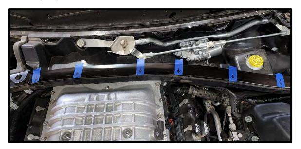
29. Remove the (4) factory fasteners from cowl cross brace using a 13mm socket (2 per side).
