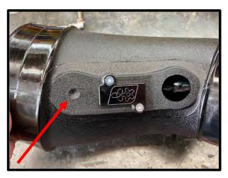
81. **(MY2017+ Challenger/Charger)** Install the supplied 1.0625" OD to .75" ID rubber grommet. Install the stock IAT sensor into plastic adapter, twist and lock in position. Install IAT into air tube.
