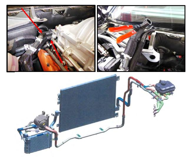
31. Disconnect intercooler water temp sensor connector at the back of the supercharger assembly.
