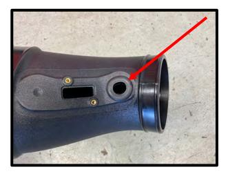
78. (MY2015-MY2016 Hellcat) Install the factory crank case pressure sensor assembly to the plastic air tube.
