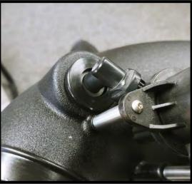
85. **(2019+ Trackhawk/Durango)** Install supplied 1.0625" OD to .75" ID rubber grommet into top port of air inlet tube. Install stock air temp sensor into supplied plastic adapter. Insert air inlet temp sensor into air tube.
