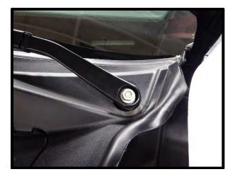
26. Remove the cabin air filter cover from plastic cowling.
