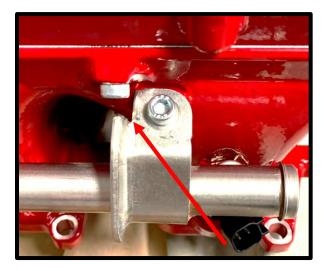
53. (Stock fuel rails) Transfer the stock fuel injectors to new supercharger assembly. Apply grease to both orings on injectors. Reinstall factory locking clip to rail and injector to secure to rail (\*failure to do so could cause running issues). Mount stock fuel rail to supercharger using supplied (4) 6mm x 14mm SHCS, apply light amount of Blue Loctite #243 to threads. Torque to 88 in-lbs using 5mm allen socket.
