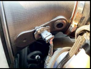
91. **(MY2015-MY2016 Hellcat)** Install the supplied ½" new make-up air hose. Connect 55deg fitting to factory valve cover barb and 90deg to sensor. Route around P/S reservoir and connect to air inlet tube.
