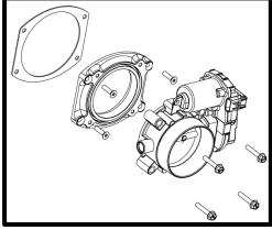
75. (**Billet throttle body**) Install supplied TB oring to TB, use light amount of grease to hold in place. Install the billet throttle body to the SC inlet using the (4) 6mm x 25mm SHCS bolts. Use Blue Loctite #243 on threads, torque to 88 in-lbs using a 5mm allen socket.
