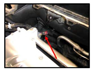
32. Carefully disconnect factory fuel line. Caution, this could be under pressure, use a rag to protect from spray.
