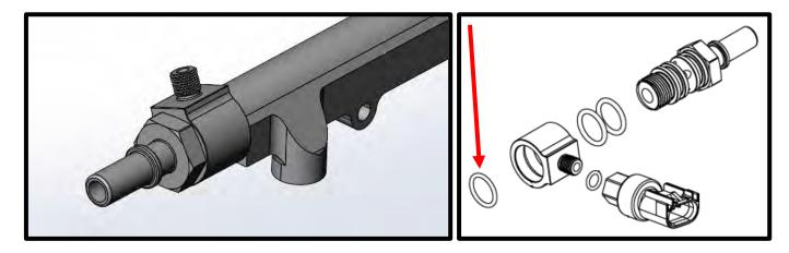
56. (**Billet fuel rails**) Install the (2) #2-115 Viton orings to male fitting. Apply grease to oring and slide through female fitting. Install (1) #3-908 Viton oring to fitting (shown with red arrow). Install banjo fitting to the longer fuel rail (PN# YH06-WPL83-0054). Use light amount of grease on oring. Install fitting to the RH side rear port.
