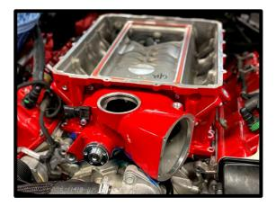
48. Install the supplied (1x) 10mm x 25 SHCS bolt to front support. Lightly torque to 42 in-lbs only to slide SC forward.
