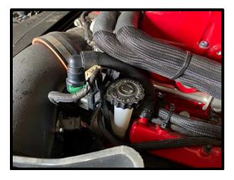
92. **(MY2017+ Challenger/Charger)** Install supplied ½" to 15.82mm quick connect fitting into ½" grommet. Install supplied 5/8" x 12" hose from 45deg barb to stock barb.
