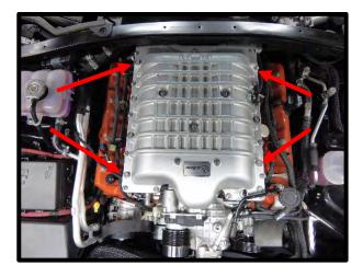
35. Clean the intake manifold surface, cover each port with tape.
