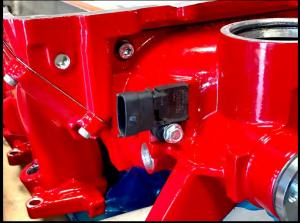
39. Remove both TMAP sensors from the passenger front and driver side rear of intake manifold using a T30 torx.
