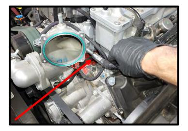
23. Using a 3/8" breaker bar or ratchet, release tension from the factory 6-rib spring loaded tensioner. Remove belt from the engine (this will be reused).
