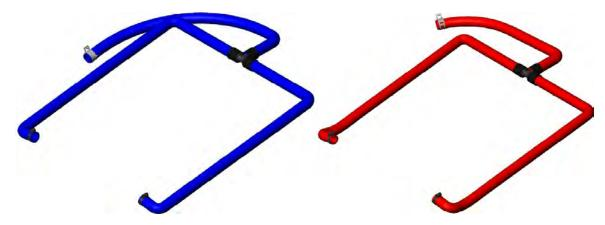
72. Install the supplied intercooler **inlet** ¾" ID hose (#3103184) to the factory inlet aluminum tubing, connect to factory line using stock pinch clamp. Connect the (2) inlet hoses to the rear most fittings on each side of the supercharger lid. Secure with the supplied black worm clamps on both inlet fittings.
