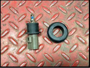
82. **(2018 Trackhawk)** Install supplied 1.0625" OD to .75" ID rubber grommet into air inlet tube. Install stock air temp sensor into supplied plastic adapter. Insert air inlet temp sensor into air tube.
