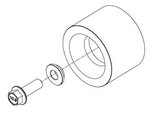
61. Install supercharger pulley using the supplied (5) 6mm x 14mm SHCS. Secure bolts hand tight. Install supplied SC belt in stock routing, by releasing tension on tensioner using a 13mm socket. Torque supercharger pulley bolts to 130 in-lbs using 5mm allen socket. **NOTE:** Aftermarket balancers and idlers will affect the belt lengths. Whipple only supplies parts for stock applications.
