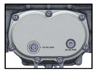
47. Using the supplied gasket set (stock Helicat or Cometic AFM ONLY), install supercharger assembly to engine. Use the supplied (10x) 8mm x 30mm HHFCS bolts to locate SC in place. Lightly run bolts down hand tight DO NOT TORQUE at this time. WARNING: DO NOT RUN PAPER GASKETS! STOCK OR WHIPPLE/COMETIC AFM TYPE GASKETS ONLY!
