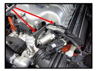
15. Disconnect and remove the driver side valve cover to air inlet tube hose. Remove sensor and 90deg plastic assembly from tube by lightly rotating and pulling. This part will be reused. (2017+ Hellcat/Redeye and 2019+ Trackhawk/Durango) Use a razor blade, cut the factory nylon hose from crank case sensor barb, this hose will be replaced.
