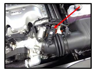
12. Disconnect the drive by wire connector from stock throttle body.
