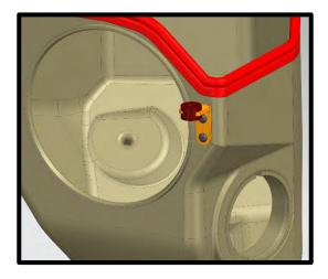
89. Connect air tube to throttle body using supplied silicone hose and supplied clamps.
