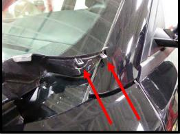
99. Reinstall the cabin air filter cover to the plastic cowling. Reinstall the windshield wipers using a 15mm socket. Use the factory (2) marks to center the wipers. Reinstall factory plastic cover.
