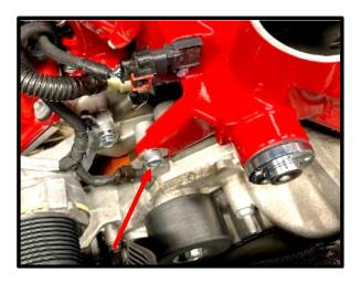
52. **(Stock fuel rails)** Test fit the stock rails to SC assembly, note that each rail needs 1 mounting bracket modified to clear bolt head. Grind small notch in bracket as required to clear.
