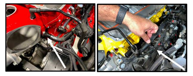
64. Connect the stock PCV hose to 15.82mm fitting previously installed.
