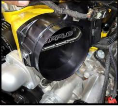
76. (Stage 1) Reconnect the throttle body 6-way connector. Reinstall Christmas tree retainer to secure harness.
