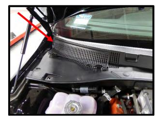
27. Remove the plastic cowling from the vehicle by removing the (8) push pins. Note there are (2) tabs on each side, pull towards center to release tabs before lifting away. Remove the wiper motor cover, this can only be reused if cut to fit.
