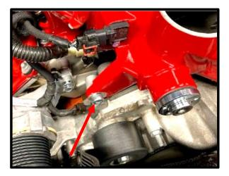
51. Torque the 10mm x 25mm HHFCS bolt you previously installed. Use a 16mm socket wrench. Torque to 30 ft-lbs.
