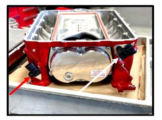
41. Remove the upper (intermediate) TMAP sensor from the factory lid, post SC, pre-IC using a T30 torx. Install the Post SC, pre-IC TMAP to the SC lid as shown. Secure using the supplied 6mm x 14mm HHFCS. Torque to 88 in-lbs using 10mm socket.
