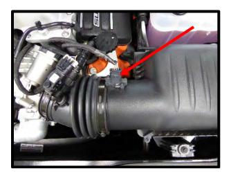
11. (When applicable) Disconnect inlet crank case pressure sensor from air duct tubing.
