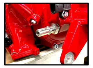
44. Install the supplied -6 ORB with oring to 9.89mm fitting to LH port on SC inlet. Use light amount of grease on oring for ease of installation.
