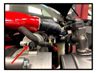
77. (MY2015-MY2016) Install supplied 1.06" OD to .875" ID grommet into pre-existing hole in air inlet tube.
