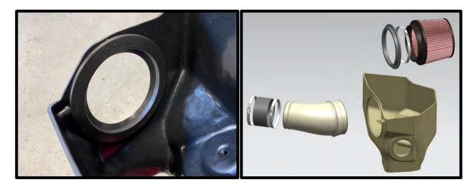
88. Mount the supplied airbox mounting bracket using the (2x) 5mm x 8mm BHCS. Secure using factory bolt through factory rubber grommet.
