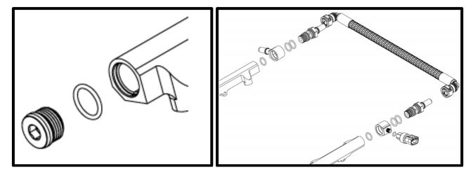
58. Install the supplied molded rubber oring to the supercharger oring groove.
