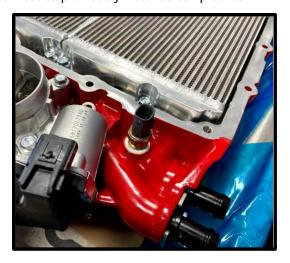
70. Install the (4) 2-117 IC fitting orings to the (4) IC fittings. Apply grease to the (4) 2-117 IC fitting orings. Slide fittings into lid. Secure fittings with supplied fitting retainer bracket and 6mm x 12mm SHCS bolt. Torque to 80 in-lbs.
