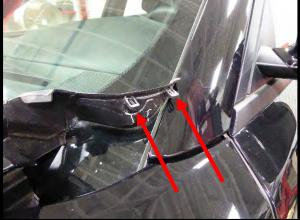
28. Remove the (6) push pins from cowl cross brace.
