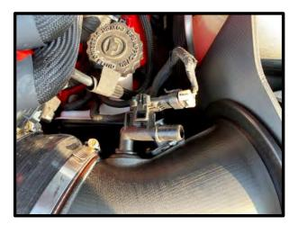
79. **(MY2017+ Challenger/Charger)** Install the MAF block off adapter using the (2) 4mm x 10mm SHCS.
