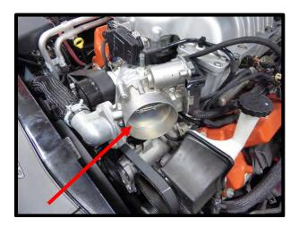
22. Remove brake booster hose from supercharger inlet.
