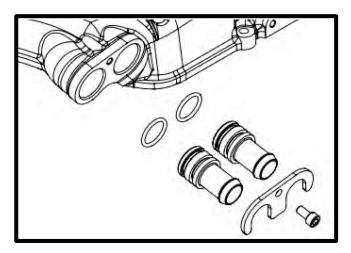
71. Assemble the intercooler hoses. For inlet (blue), take (2) of the #3103182 hose, face the short 90deg ends towards each other. Secure to tee fitting using supplied pinch clamps. Assemble hose #3103184 to tee fitting, secure with pinch clamp. For outlet (red), take (2) of the #3103182 hose, face the short 90deg ends towards each other. Secure to tee fitting using supplied pinch clamps. Assemble hose #3103183 to tee fitting, secure with pinch clamp.
