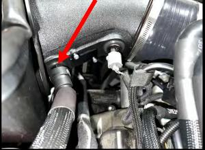
93. **(2019+ Trackhawk/Durango)** Install supplied 5/8" to 15.82mm 90deg quick connect fitting to make up air barb on valve cover. Install other end to crank case pressure sensor barb.
