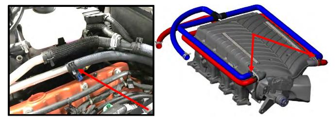
73. Install the supplied intercooler **outlet** ¾" ID hose (#3103183) the factory Y fitting using stock pinch clamp. Connect the (2) outlet hoses to the forward most fittings on each side of the supercharger lid. Secure with the supplied worm clamps on both outlet fittings.
