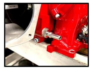
45. Install the supplied -6 ORB with oring to 3/8" barb fitting to LH top port on SC inlet. Use light amount of grease on oring for ease of installation.
