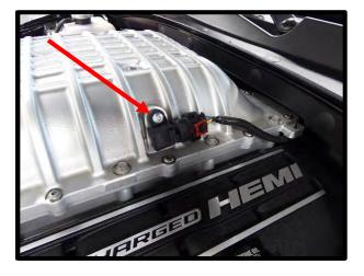
10. (2015-2016 Only) Disconnect MAF sensor connector from MAF housing. NOTE: 2017+ doesn't use MAF sensor.
