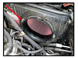
18. Using a 5/16" socket, remove the (1) retaining bolt for airbox lower. Lift the airbox back and up, disconnecting snorkel at the same time. **NOTE:** Redeye version, fascia needs to be removed to get snorkel out.
