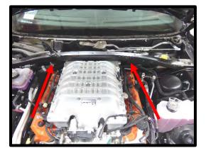
98. Reinstall the plastic cowling to the vehicle by installing the (8) push pins you previously removed. Make sure the tabs on each side lock in place.
