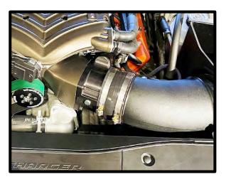
90. (MY2015-MY2016) Install factory MAF sensor element using the (2) 4mm x 10mm SHCS. Reconnect factory MAF connector to MAF sensor.
