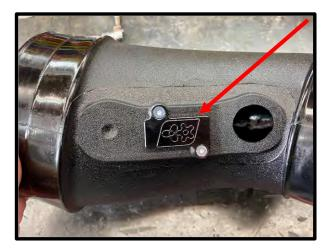
80. **(MY2017+ Challenger/Charger)** Using a 13/16" hole saw, drill the air tube (drill point shown). Clean air tube and install supplied .80" OD to .50" ID rubber grommet. Install supplied ½" to 15.82mm quick connect fitting. Clean air tube from any debris.
