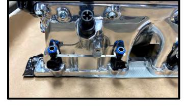
55. (Billet fuel rails) Install the (2) #2-115 Viton orings to male fitting. Apply grease to oring and slide through female fitting. Install (1) #3-908 Viton oring to fitting (shown with red arrow). Install fitting to the driver side fuel rail (rear). Install the supplied fuel PSI sensor to fuel rail adapter using (1) #2-011 oring. Reconnect fuel PSI sensor electrical connector.
