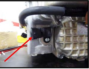
40. Install the post SC, post IC TMAP sensors (2) in the back of the manifold using the supplied 6mm x 14mm HHFCS, torque to 88 in-lbs using 10mm socket.
