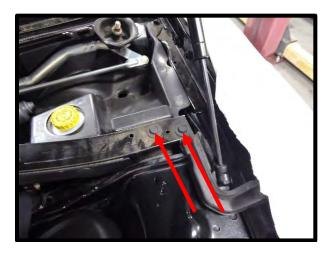
30. Disconnect the (2) intercooler lines by removing the factory pinch clamps. Lower fitting, remove from intercooler fitting. Top fitting, remove just after the factory Y fitting. Clamp the lines with a hose crimp plier to limit leaking.
