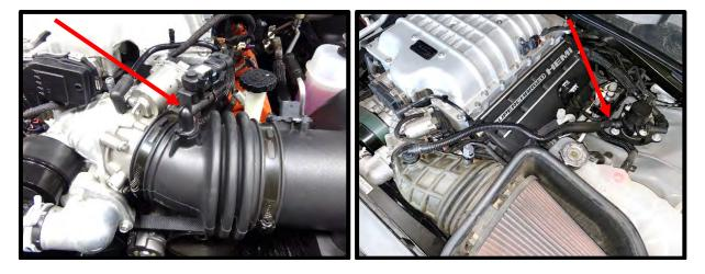
16. **(Hellcat)** Using a 5/16" nut driver, loosen the clamps on the rubber air tube between airbox and supercharger. Using the same tool or a phillips screw driver, remove the (3) airbox bolts on standard Hellcats. Remove air tube out of the way. Standard Hellcats, remove air box lid and air filter from vehicle.
