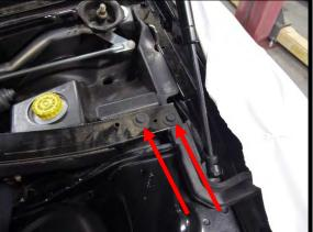
97. Reinstall the (6) push pins in the cowl cross brace. **NOTE:** Windshield wiper cover can be cut around supercharger to fit
