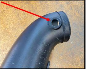
84. **(2019+ Trackhawk/Durango)** Using a 1" hole saw, drill the air tube as shown. Install supplied 1.06" OD to .875" ID grommet into air tube. Install crank case pressure sensor to air tube, using the (2) 35mm and (1) 51mm spacers. Secure using (2) 4mm x 45mm and (1) 4mm x 65mm BHCS.
