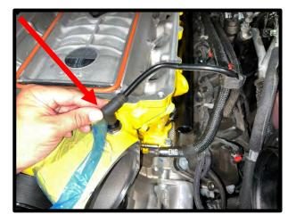
63. Connect the stock brake booster hose to the 9.89mm fitting previously installed. NOTE: Remove harness retainer from EVAP brake booster and EVAP lines.
