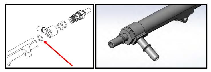
57. **(Billet fuel rails)** Install supplied -8 ORB plugs to front fuel rail ports, with #3-908 Viton oring. Use light amount of grease on oring. Install supplied ½" cross over hose at the rear fittings.
