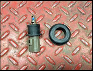
83. **(2018 Trackhawk)** Remove the 90deg plastic fitting from factory air inlet tube. Using a 1" hole saw, drill the supplied inlet air tube as shown. Install supplied 1.06" OD to .875" ID grommet into air tube. Install the 90deg PCV fitting to .875" grommet. Connect stock make up air hose with crank case pressure sensor.
