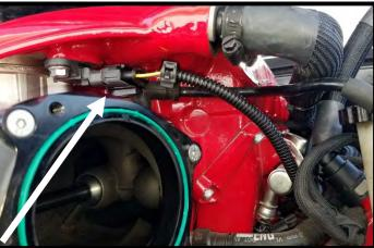
69. Install the supplied 22" IC temp sensor extension to stock 2-way connector by cutting the stock connector off 3" from end. Install pigtail using the supplied butt connectors, crimp together, then slide heat shrink over and shrink. Route to front of engine and connect to previously installed temp sensor.
