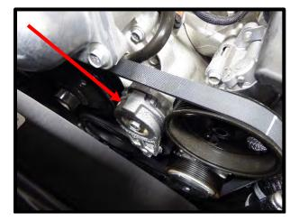
24. Using a 15mm socket, release the tension from the supercharger spring loaded tensioner. Remove the supercharger belt from the engine.
