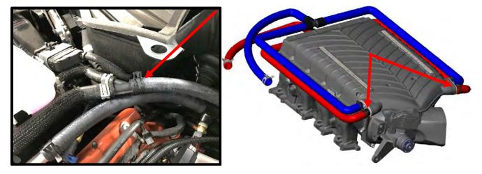
74. (Stock throttle body) Install the stock TB adapter to the supercharger inlet using the supplied TB adapter, supplied gasket and the (4) 6mm x 25mm FHCS. Torque to 75 in-lbs. Install the stock throttle body oring to TB adapter, then install the throttle body using the (4) 6mm x 35mm HHFCS bolts. Use Blue Loctite #243 on threads, torque to 88 in-lbs using a 10mm socket.
