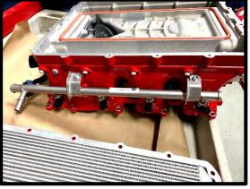
54. (**Billet fuel rails**) Transfer the stock fuel injectors to new supercharger assembly. Apply grease to both orings on injectors. Install supplied locking brackets to fuel injectors (\*failure to do so will cause running issues). Mount billet fuel rails to supercharger using supplied (4) 6mm x 35mm SHCS, apply light amount of **Blue Loctite #243** to threads (PN# YH06-WPL83-0054 is passenger side). Torque to 88 in-lbs using 5mm allen socket. \***NOTE**: For stock injectors only.
