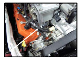
21. Remove the throttle body from the engine using a T30 Torx and socket wrench.
