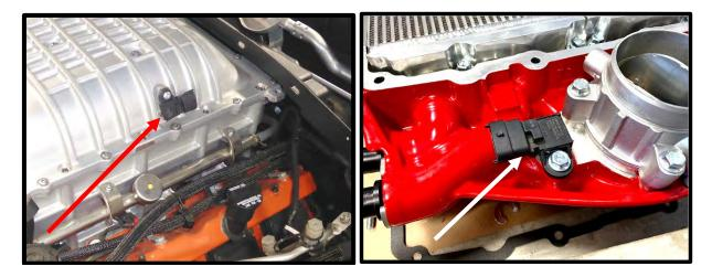
42. Remove the intercooler water temp sensor from the IC water cross over using a 19mm socket or wrench. Install the stock IC temp sensor, using light amount of thread sealant to the Whipple lid port.
