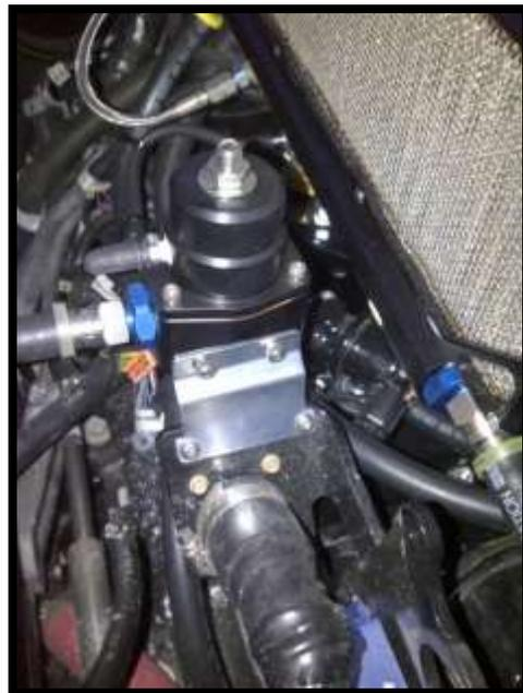
Picture is an example of remote mounting regulator
