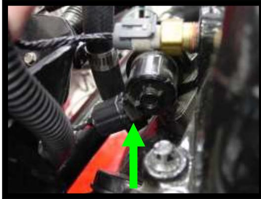
5. Remove 3/8" rubber hose from IAC motor to factory throttle body.
