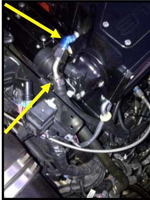
37. Fill supercharger with Whipple SC oil to middle of sight glass. **DO NOT OVERFILL SUPERCHARGER OIL LEVEL. MAX LEVEL IS 6.8 FL OZ (200ax).**
