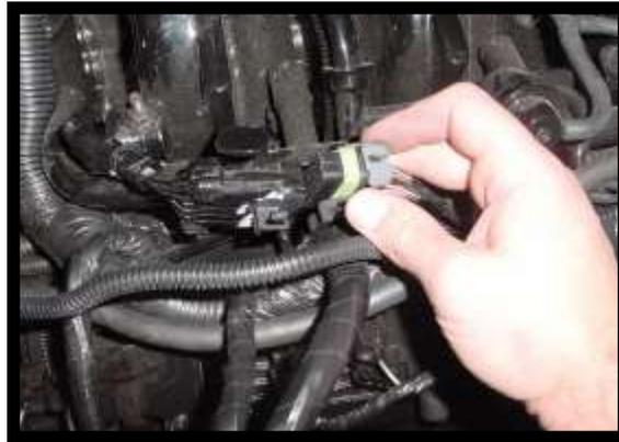
7. Remove factory computer support bracket from intake and exhaust manifold. Pull bracket and wiring back for easier access to engine.
