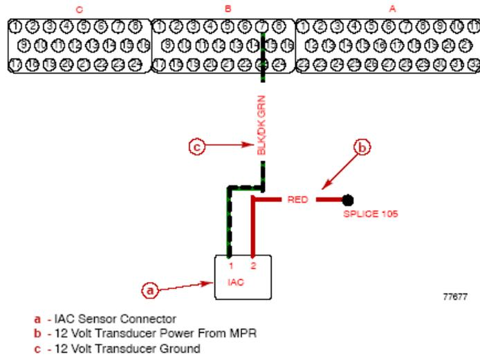
The idle air control (IAC) valve is a 12 volt circuit powered by the MPR. It is located at the top rear of the engine. The normal resistance value for the IAC at 21 degrees C (70 degrees F) is 10.1 ohms.
