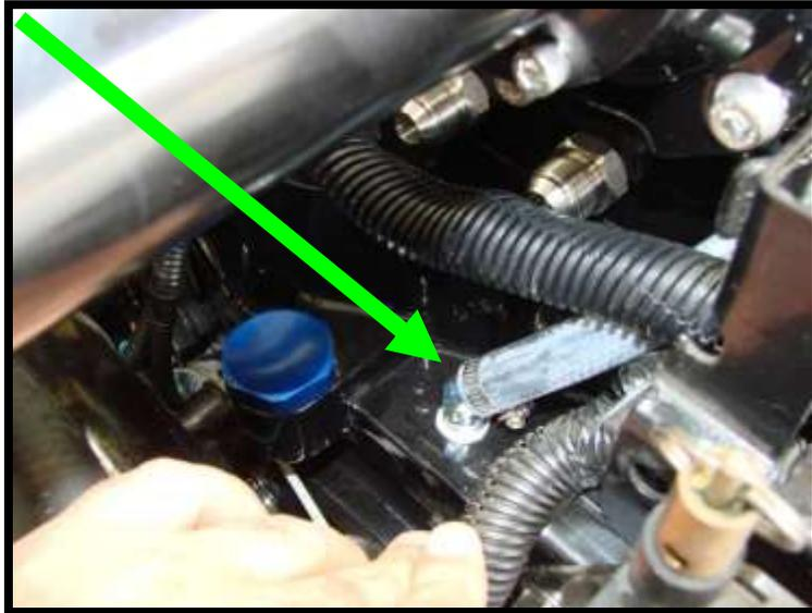
35. Locate the PCV valve installed on the backside of the intake manifold.
