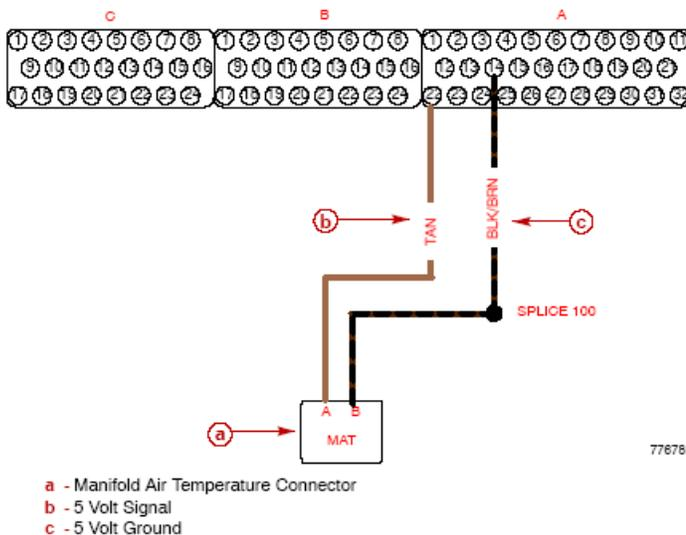
The manifold air temperature (MAT) sensor is a thermistor that controls signal voltage to the PCM. It is located at the rear of the engine in the intake manifold plenum. When intake air is cold, the sensor resistance is high. As the air temperature rises, resistance lowers. At normal engine operating temperature, 71-82 degrees C (160-180 degrees F), the voltage will measure about 1.5 to 2.0 volts. The normal resistance value for the MAT sensor at 21 degrees C (70 degrees F) is 3.14 kohms.
