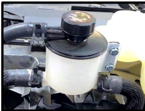
121. Cycle the ignition to the ON position again and repeat until the sound of the electric pump is continuous without any pulsation and the fluid level is met at the filler cap. **NOTE: During water pump start-up, it is normal for a slight pulsation to occur. Once the pump has reached its maximum cycle speed, no pulsations should be present. If any pulsations occur, there is air in the system. NEVER GO WOT UNTIL AIR IS BLED OUT!**
