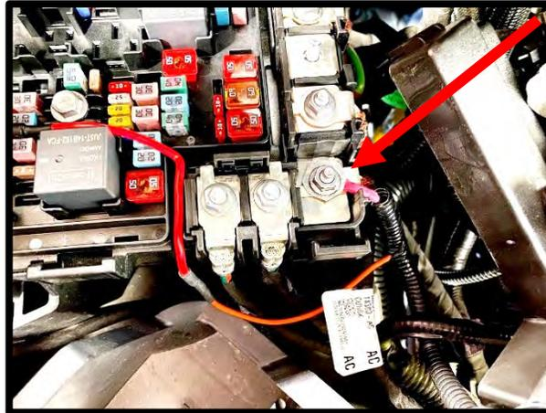
112. Remove the ground bolt from the **RH** side frame, next to the battery using an 8mm socket. Install IC pump relay ground eyelet here. Secure with factory bolt using an 8mm socket.
