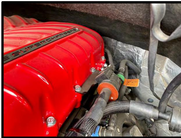
74. Connect the factory high pressure **RH** side rail fitting to the DI pump factory hose, press until it clicks and locks in place. **NOTE: THIS FUEL LINE HAS A CHECK VALVE, NEVER FLIP ORIENTATION FROM STOCK DIRECTION.**
