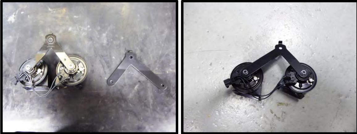
90. Reinstall new horn bracket and horns to factory location, using factory nut. Torque to 106 lbs-in. Zip-tie wire to factory harness for clean installation.
