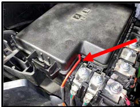
115. Secure the relay/fuse with zip-ties along with the harness for a clean installation. Route IC pump connector down below radiator, secure to IC pump previously mounted. Ensure all other wires are clear of the belt system, use zip-ties to eliminate any potential interference.
