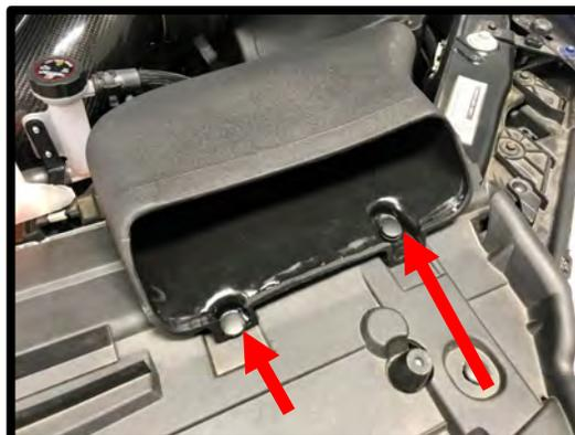
104. Install the supplied panel filter to the airbox lower. Install the upper airbox to the top of the filter. Secure the top to bottom using the supplied (6) 6mm x 16mm BHCS. Torque to 50 in-lbs. **\*Caution:** Over torquing can result in pulling an insert out of plastic box.
