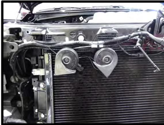
91. Using a saw or shears, cut the plastic shroud as shown, below the RH side heat exchanger fitting. This will allow proper clearance for the hose installed later.
