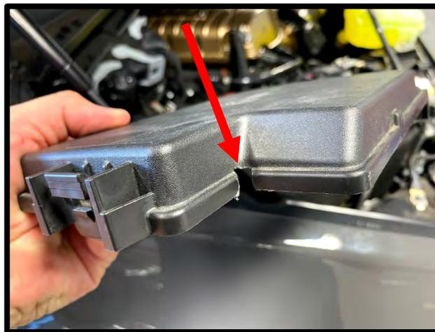
110. Locate the stock hole in the battery box as shown below. Use the supplied plastic push pin to secure the intercooler relay and fuse holder to the battery box. Route power and ground around box to fuse box area.
