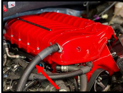
98. **(Stage 1 and Stage 1R Stock throttle body)** Install throttle body adapter to supercharger inlet using the (4) 6mm x 20mm FHCS bolts and supplied gasket between TB adapter and SC inlet. Apply **Blue Loctite #243**, torque to 65 lbs-in. Install the stock throttle body using the (4) stock bolts using a 10mm socket, torque to 80 in-lbs.
