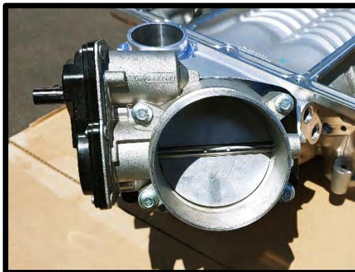
99. (Stage 2 Whipple 132mm Crusher throttle body) Install throttle body to supercharger inlet, use the supplied gasket between TB adapter and SC inlet. Secure with the supplied (3) 6mm x 25mm SHCS and (1) 6mm x 50mm SHCS using a 5mm allen socket. Torque to *89 lbs-in* on first pass, *139 lbs-in* on second pass.
