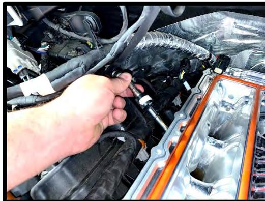
75. Connect the factory fuel inlet line to the driver side fuel fitting, press until it clicks and locks in place. Connect factory fuel psi sensor connector to sensor, press safety lock until it clicks into place.
