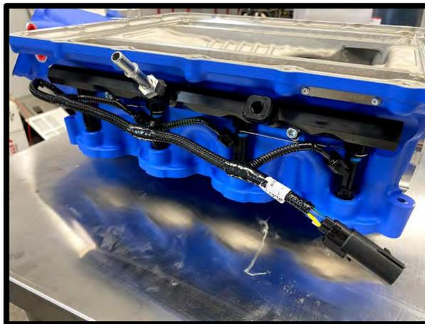
55. Install the supplied 1/4" ID bypass actuator to the bypass nipple and 1/4" 90deg nipple on SC inlet. **CAUTION:** Do not open/close bypass actuator by hand. This may damage actuator internally. It only moves properly with equal vacuum/boost at the actuator reference port.
