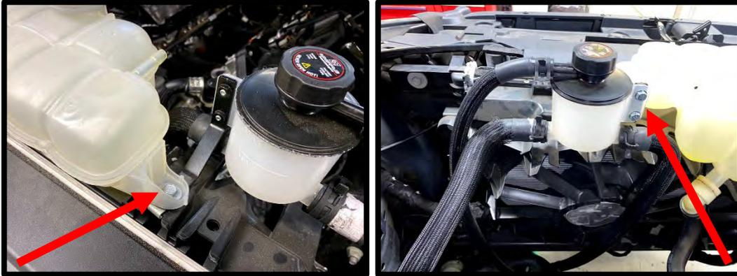
95. Install the 3/4" ID x 32" hose (#3103094) and the 3/8" ID 39" (#3103098) rubber hoses to the IC filler neck. Secure with supplied pinch clamps. Connect the 3/4" hose to the IC pump inlet fitting, secure with pinch clamp. Secure 3/8" vent hose with zip tie to the 3/4" hose. **NOTE: Ensure that this hose cannot kink or rub anything overtime.**
