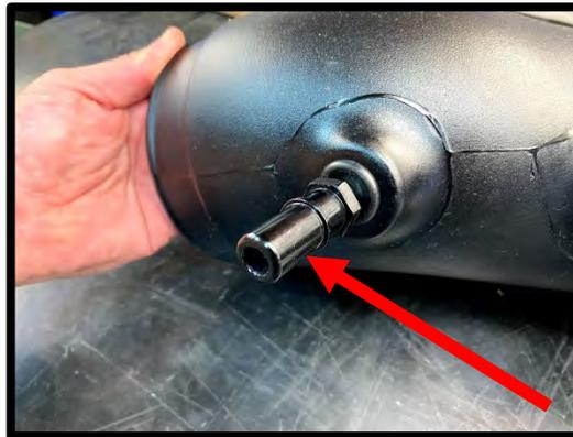
106. **(Whipple 132mm Crusher throttle body)** Install the supplied 5" ID x 2 1/2" silicone hose over air inlet tube and airbox lid. Install the 4 3/4" x 3" silicone hose over throttle body. Install the air inlet tube between the filter and throttle body. Slide silicone hose over throttle body. Secure all ends with the supplied (4) #80 hose clamps.
