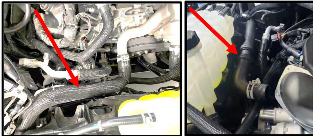
42. **(Dual Alternator)** Reconnect factory quick connect fittings to new coolant tubes. **NOTE:** Some model F150's switched the top fitting from the 90deg to a 55deg (blue arrow). Replace the 45 deg fitting with the supplied 90deg fitting.
