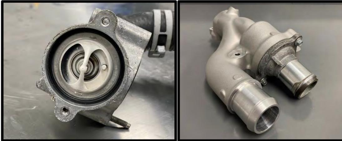
38. **(Dual Alternator)** Apply pipe sealant to threads of supplied 1/8" NPT to 5/16" barbed fitting, install to open 1/8" port on housing.
