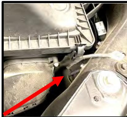
103. Install the supplied lower airbox into factory (2) hole locations. Using the supplied (2) 1.1" L x .30" W plastic push pins, secure front of snorkel to factory location.
