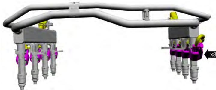
24. **(Stage 1)** Remove the (8) safety clips from injectors. Remove the injectors from fuel rail. Remove the top and bottom orings from stock injectors. Use Berryman B-12 Carburetor cleaner to clean orings or soak orings for a couple hours in a cleaner such as 409 or similar. If orings have any cuts or damage, replace prior to installing. Once clean, reinstall orings to stock fuel injectors.
