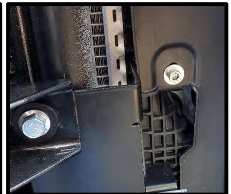
89. Remove the horns from the factory bracket and relocate them to the new supplied bracket as shown.
