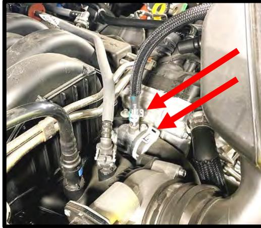
28. **(Single Alternator)** Disconnect the driver side heater tube quick connect fitting by squeezing and lifting away. Remove the heater tube overflow hose using a pinch clamp tool. Using an 8mm socket on the 1 factory bolt, remove the heater tube.
