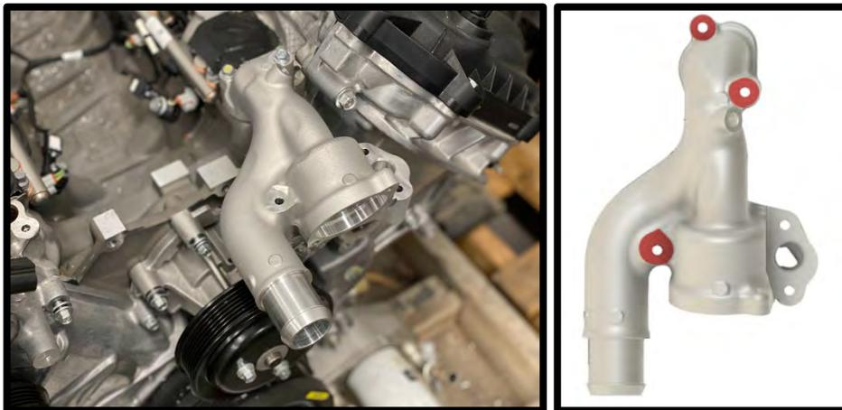
40. **(Dual Alternator)** Install the supplied #2-113 oring to new coolant tube. Install tube to thermostat housing. Secure coolant tube using the (2) 6mm x 50mm HHFCS bolts supplied. Torque all (5) thermostat housing bolts to 89 lbs-in.
