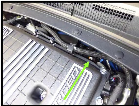
20. Using a 10mm socket, remove the (10) bolts from the supercharger (8 inside, 2 outside).
