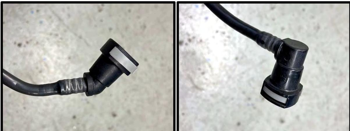
38. Install the 3/8" x 45" vent hose 45deg fitting in driver side valve cover. Route hose around the back and then around to the RH side of engine. Connect other end to OEM catch can, center most fitting as shown.
