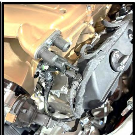
29. Apply light amount of pipe Teflon to threads of supplied 1/8" NPT to 1/4" barb fitting. Install fitting to RH 1/8" NPT port on SC inlet.
