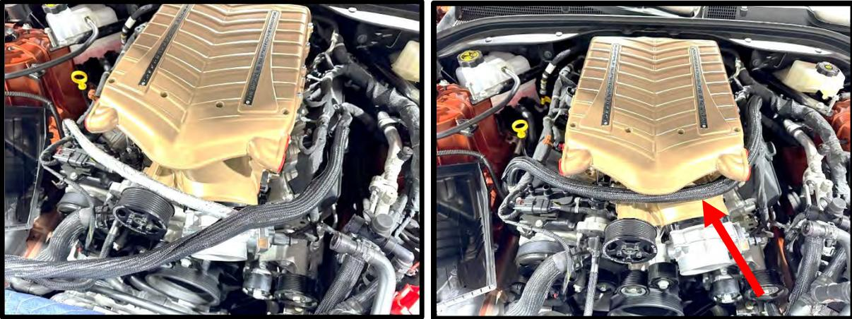
53. Install factory make-up air hose from middle catch can fitting to air inlet tube. Secure wire loom to this hose above supercharger using zip-ties.
