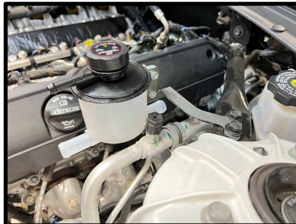
43. Install the supplied preformed IC outlet hose #3103182 to the RH front fitting. Route around the back of the SC to supplied TEE fitting. Install the supplied hose #3103182 to RH side front IC inlet fitting. Install supplied 3/4" hose to TEE fitting and route to rear fitting of the reservoir. Secure hose to the IC inlet fittings with supplied black 16mm-27mm black worm clamps. Secure other ends with supplied #16 pinch clamps. **NOTE: DO NOT MIX UP!**
