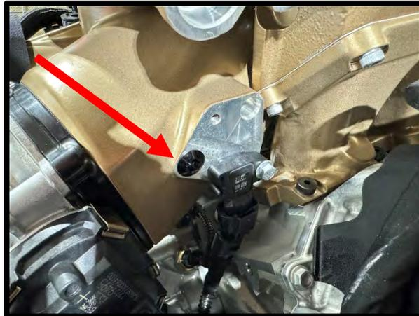
27. Install the factory EVAP solenoid to the inlet casting. Secure using the factory hex head bolt, torque to 96 in-lbs (10mm socket).
