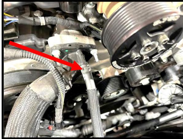
50. Install the throttle body adapter to SC inlet with 112mm gasket to SC. Secure using (4) 6mm x 25mm FHCS bolts. Install stock oring to throttle adapter. Mount TB to adapter using (4) 6mm x 40mm HHFCS bolts. Torque to 96 in-lbs (10 mm socket). Reconnect factory TB electrical connection.
