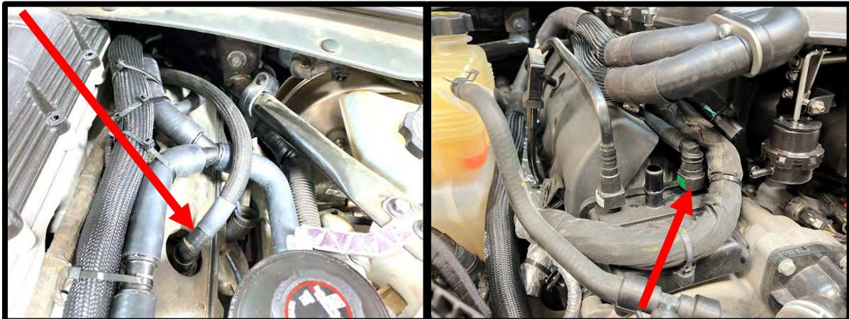
39. Connect the 3/8" x 45" EVAP hose previously routed to the EVAP solenoid.
