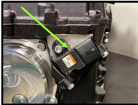
25. Using a T30 Torx socket, remove the factory pre-SC MAP sensor (SIP 1-bar). Install into the boss located at the top of the inlet of the Whipple SC. Apply light amount of grease to oring before installing. Secure to manifold using the supplied 6mm x 20mm HHFHCS. Torque to 90 in-lbs. Reconnect factory SIP sensor electrical connector.
