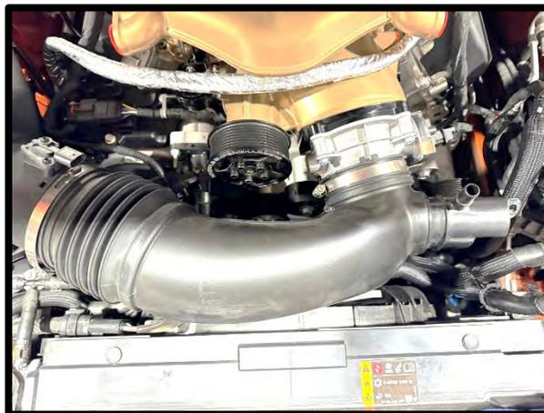
55. Refill the Engine coolant. Verify that your coolant drain is closed, and use a filter/strainer to pour the recycled coolant/water mixture that you drained from the radiator. If necessary, top off with a **GM approved engine coolant**. Whipple also recommends running 2 bottles of Redline Water Wetter which can be found at most automotive parts stores. **⚠ WARNING!! NEVER USE TAP WATER, THIS WILL CAUSE CORROSION IN THE SYSTEM.** Start engine to completely fill system.
