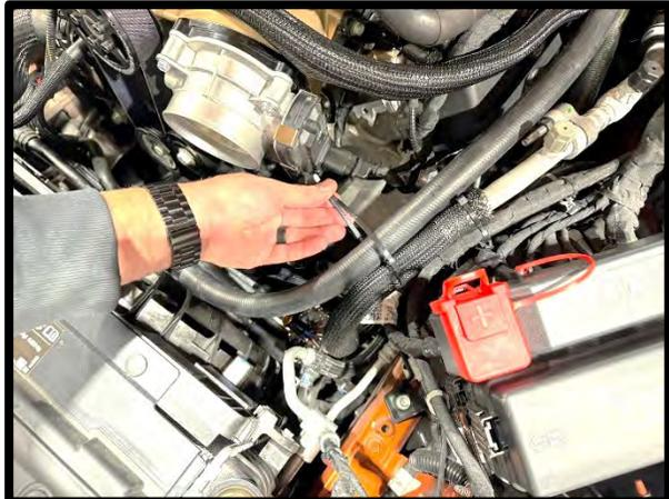
45. Install the reservoir to IC pump  $\frac{3}{4}$ " hose from reservoir to IC pump top barb fitting. Secure hose to reservoir using #16 pinch clamp and to pump using stock clamp. Secure hose away from idler and belt with zip-ties.
