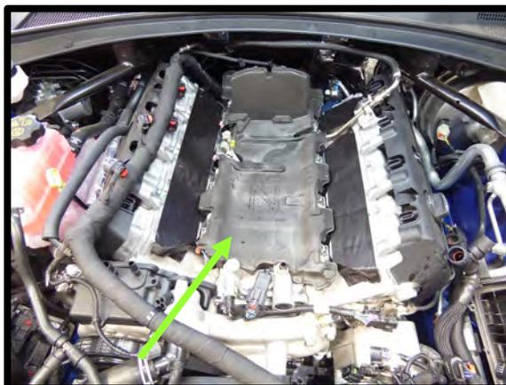
23. **HIGHLY RECOMMENDED.** Replace stock spark plugs with new OEM replacement plugs, #12642722, **gap at .032"**. Apply a small amount of anti-seize on the threads. Torque to 11 ft-lbs
