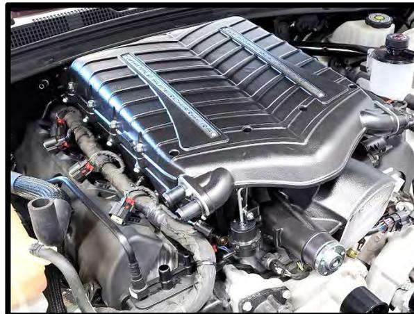
34. Apply light amount of **Loctite #242** to the (10) 6mm x 30mm HHFCS bolts. Install bolts to runners, using 10mm socket. Hand tighten all bolts. Torque to 44 in-lbs on first pass, second pass, torque to 89 in-lbs, third pass, redo 89 in-lbs.
