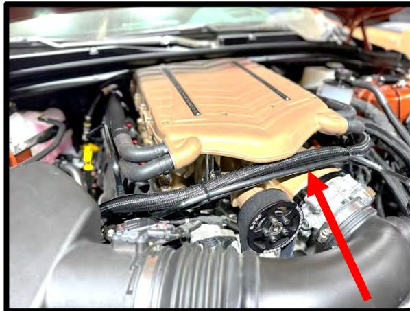
54. Install the stock rubber 90deg inlet tube using stock hose clamps to throttle body and airbox. Install factory airbox lid, secure using factory fasteners.
