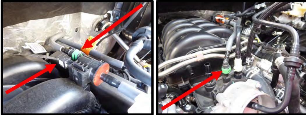
18. Remove the second brake booster quick connect line from intake manifold by squeezing locking tab and pulling away.
