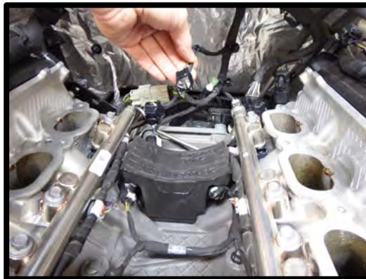
33. **(Complete kits)** Install the supplied TMAP pigtail to the stock MAP sensor connector, lay on valve cover for later installation to new TMAP sensor.
