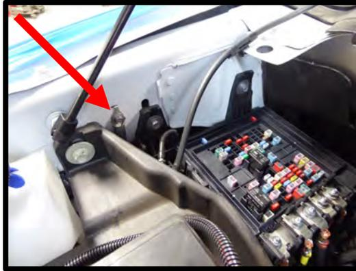
107. Pull the red 10amp fuse from position #F17 (ABS). Install the 10amp red fuse in the unused fuse slot on the fuse tap. Install the supplied fuse tap into position #F17 (ABS). **Note:** 10amp red fuse should be in bottom slot, 5amp should be in top slot. Make sure wire has enough room when fuse cover closes, route around fuses for clean installation.
