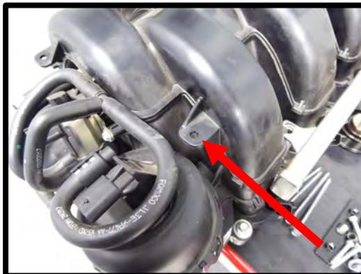
30. Remove the intake manifold from the engine. To do so, remove the (3) wire harness push pin supports from the back of the intake manifold, disconnect the (3) IMRC connectors by pushing on the locking tab and pulling, disconnect the 4-way MAP sensor connector and disconnect the 12-way DI injector harness by releasing the locking tab and pulling apart.
