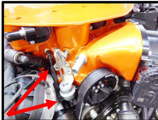
50. Install the (3) supplied 6AN viton orings (#906) to the (1) 6 ORB to 9.89mm and the (2) 6 ORB to 15.82mm quick connect fittings supplied. Bank 2 side, install (1) 15.82mm fitting to the lower port using a 7/8" deep socket and the 9.89mm fitting in the top port using a 11/16" deep socket. Bank 1 side, install (1) 15.82mm fitting to the lower port using a 7/8" deep socket. Install the supplied 6AN plug with oring to lower port, bank 1 using a 6mm allen.
