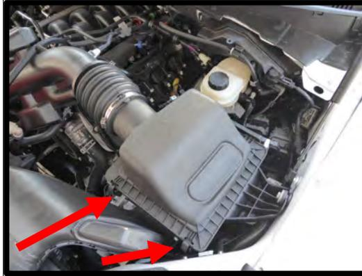
15. Using a 13mm socket, remove the (1) factory fastener securing airbox to the fender.
