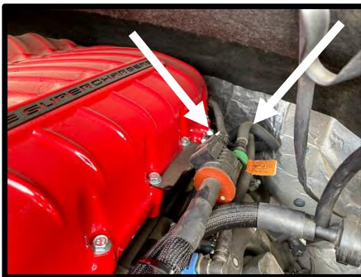
66. Install the supplied 3/8" ID x 12" with 55deg quick connect fitting hose (#18F150-HS011) to the EECPV barb fitting and **upper** quick connect fitting on SC inlet. Push until it clicks and locks into place.
