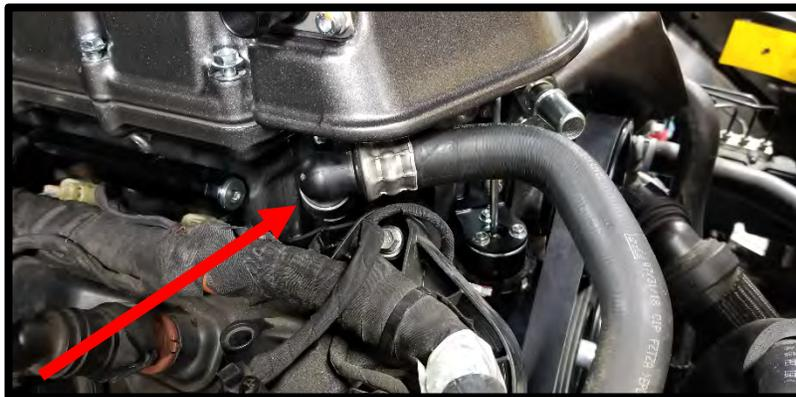
72. Connect factory heater hoses to previously installed plastic water fitting (bank 2).
