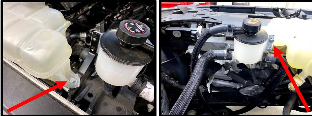
97. Install the 3/4" ID rubber hose (#18F150-HS006) from the **Bank 2 (OUTLET)** IC fitting to the IC filler neck. Secure both ends with supplied pinch clamps. **NOTE: NEVER SWITCH THE INTERCOOLER ROUTING, BANK 2 IS ALWAYS THE OUTLET!**
