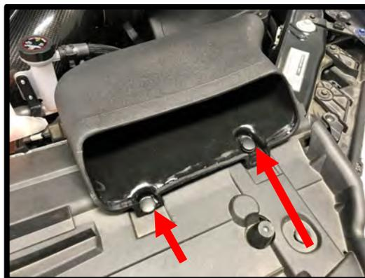
99. Install the supplied panel filter to the airbox lower. Install the upper airbox to the top of the filter. Secure the top to bottom using the supplied (6) 6mm x 16mm BHCS. Torque to 50 in-lbs. **\*Caution:** Over torquing can result in pulling an insert out of plastic box.
