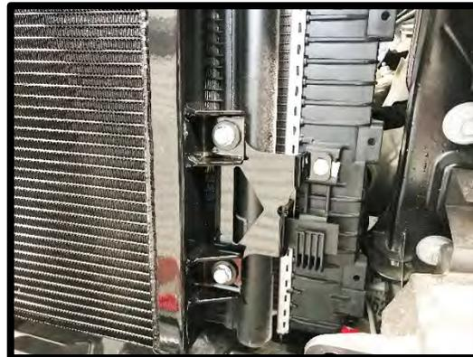
84. Reinstall new horn bracket and horns to factory location, using factory nut. Torque to 106 lbs-in. Zip-tie wire to factory harness for clean installation.
