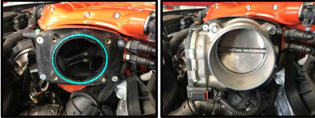
94. **(Stage 2 Whipple 132mm Crusher throttle body)** Install throttle body to supercharger inlet, use the supplied gasket between TB adapter and SC inlet. Secure with the supplied (3) 6mm x 25mm SHCS and (1) 6mm x 50mm SHCS using a 5mm allen socket. Torque to 88 lbs-in.
