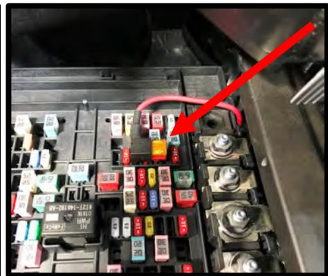
108. Secure the relay/fuse with zip-ties along with the harness for a clean installation. Ensure all other wires are clear of the belt system, use zip-ties to eliminate any potential interference.
