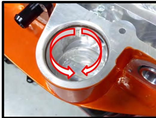
62. Apply generous amount of grease to the (1) #2-230 Viton bypass oring. Install the supercharger lid to the supercharger housing by carefully placing the bypass down. Secure the SC lid using the (17) 6mm x 30mm HHFCS and (3) 6mm x 70mm HHFCS (marked green) using the following pattern. Slide the EECPV bracket under bolts 3 and 5 from image (bank 2). Torque to 90 lbs-in using an 8mm socket.
