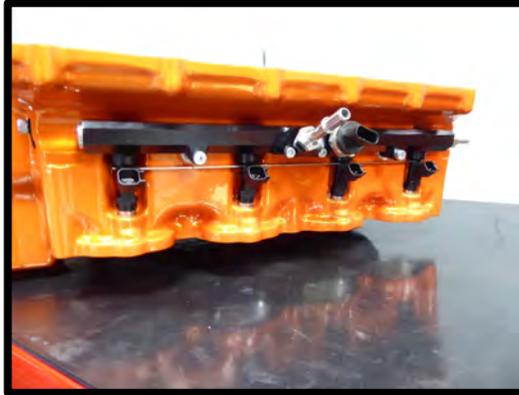
48. Install the supplied 3/8" fuel cross over line around the back of the supercharger by pressing until they click and lock in place.
