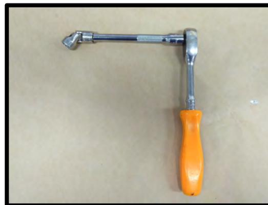
60. Reinstall the water pump pulley using a 10mm socket, torque to 14 lbs-ft.
