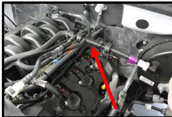
20. Carefully cut the electric tape securing the ETC wires to the throttle body. Disconnect the electronic throttle electrical connector by pushing up on the safety lock and then squeezing the connector and pulling away.
