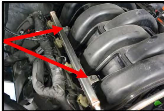
28. Loosen the (8) manifold to cylinder head bolts using an 8mm socket.
