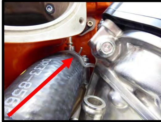
37. Remove stock oring from factory bank 2 heater tube, install on supplied heater tube. Install the supplied plastic heater tube into bank 2 heater port. Secure with supplied stepped bracket and factory bolt.
