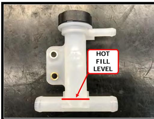
117. Cycle the ignition to the ON position again and repeat until the sound of the electric pump is continuous without any pulsation and the fluid level is met at the filler cap. **NOTE: During water pump start-up, it is normal for a slight pulsation to occur. Once the pump has reached its maximum cycle speed, no pulsations should be present. If any pulsations occur, there is air in the system. NEVER GO WOT UNTIL AIR IS BLEDED OUT!**
