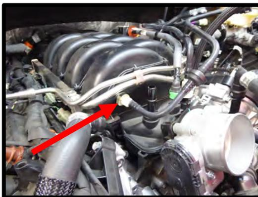
17. Disconnect the EVAP solenoid electrical connector by squeezing locking tab and pulling away. Disconnect the EVAP solenoid quick connect fitting hose from the EVAP solenoid and from the intake manifold by releasing locking tab and pulling away.
