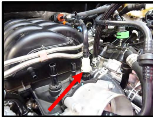
19. Remove the brake booster vacuum line from check valve and IMRC vacuum lines from brake booster line (separate where the arrow points). The check valve closest to the brake booster connector will be utilized.
