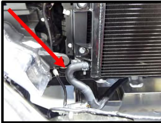
89. Connect the 3/4" ID molded/formed (33") hose (#18F150-HS009A) from the LTR driver side bottom fitting that you previously installed, to the IC pump outlet barb. Secure with supplied pinch clamp. **NOTE: Ensure that this hose cannot kink or rub anything overtime.**
