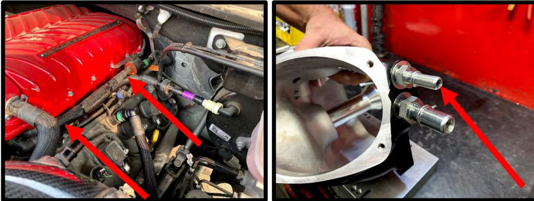
67. Install the supplied 1/2" ID x 14" with 90deg quick connect fitting brake aspirator hose (#HSF150-HS012) from the brake booster to the **lower** quick connect fitting on the supercharger inlet. Push until it clicks into place. **TIP:** For best routing, nestle in between cam cover and fuel rail, under the wiring and heater hose.
