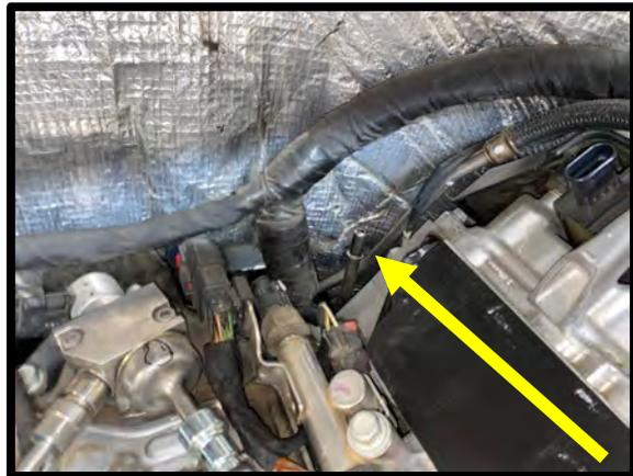
14. Remove the stock throttle body from the engine by removing the (4) fasteners using a 10mm socket.
