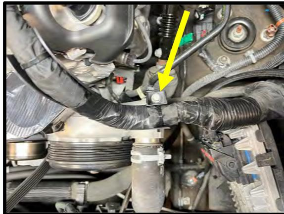
30. **(14-20 SUV ONLY)** Remove the two heater hoses from stock Tee fittings. Remove the center most tee fitting.
