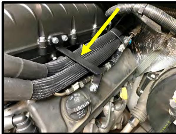
98. (14-20 SUV ONLY) Remove the stock crimp fitting and stock straight quick connect fitting from heater hose. Use the supplied 90deg 15.82mm quick connect fitting to end of stock hose. Secure hose using supplied #8 hose clamp. Reinstall the stock Tee fitting previously removed. Install this fitting to end of stock tee fitting. Route under other heater line, secure to tee fitting.
