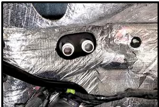
32. **(14-20 SUV ONLY)** Using a pipe over the heater tube, lightly bend towards RH (passenger side) of vehicle. For reference, the goal is to move the end of the fitting between  $\frac{1}{4}$ " to  $\frac{1}{2}$ " for clearance to the supercharger. This hose will be reinstalled later in install.
