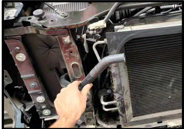
81. Loosely mount the LTR and headlight/grille bracket assembly back to vehicle using the factory hardware. Route the LTR to IC feed hose #3103256 to the top fitting. Secure with supplied pinch clamp.
