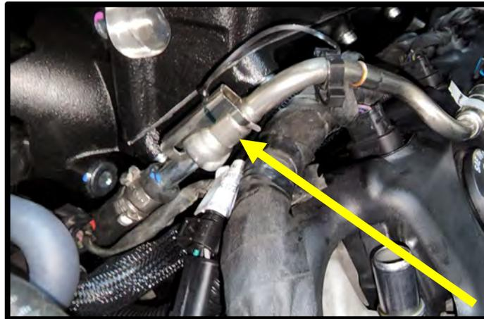
56. Install the supplied 3/8" ID PCV hose #3103248 with the dual 90deg 9.89mm fittings to the valley tray quick connect fitting (straight end). Route the hose and the 90deg up towards driver side. Connect 90deg fitting to driver's side rear fitting on inlet of SC. Push until it clicks and locks in place.
