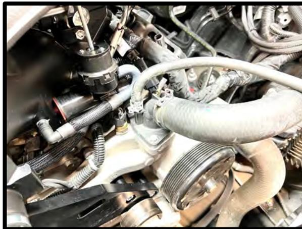
62. Install the IC filler reservoir bracket to the RH front fender support brace. Remove the stock bolt using a 13mm socket. Secure bracket using supplied 8mm x 18mm HHFCS, torque to 18 ft-lbs.
