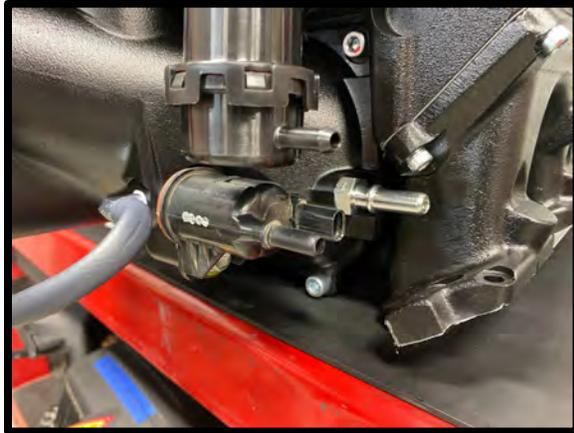
36. Install the (3) #2-906-V75BR orings to the (1) 9.89mm fitting and (2) -6 ORB plugs. Install the (1) 9.89mm fitting and (1) -6 ORB plug to the SC inlet RH side of inlet. Install the (1) -6 ORB plug to on LH side of inlet. Apply light amount of grease to oring to ease installation
