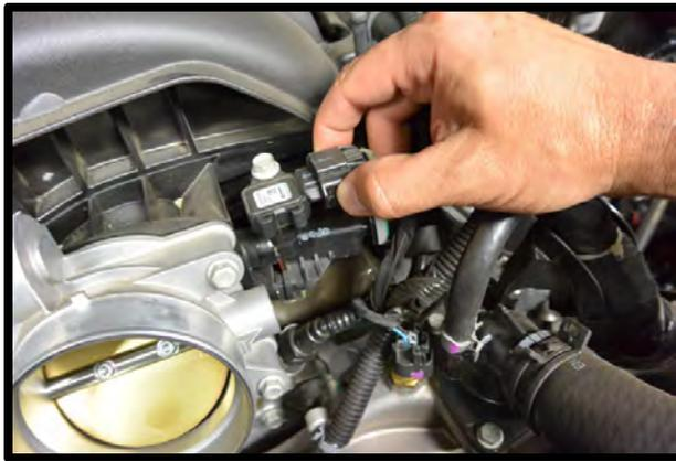
13. Disconnect the factory EVAP solenoid quick connection from solenoid by squeezing the connector and pulling away. Remove EVAP line from port at back of engine LH side. Remove the EVAP solenoid from the intake manifold using a 10mm socket and hang to the driver side of engine for later installation.
