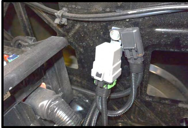
94. Route the IC pump 2-way connector up front under driver side headlight area, below bumper and to the IC pump. Push connector until it clicks and locks in place.
