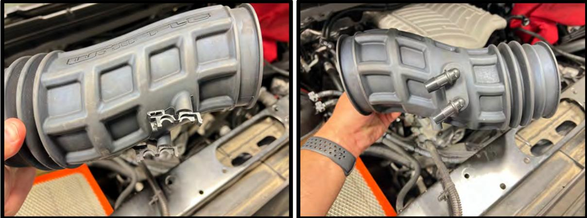
106. Install the supplied Whipple air inlet tube to the factory MAF housing and secure with the supplied #64 clamps. Install other end of inlet to the supplied silicone hose to the factory throttle body using supplied clamp.
