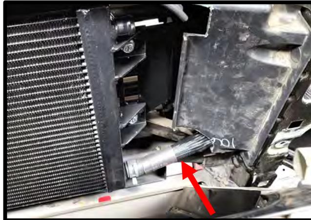
80. Route the LTR to IC feed hose #3103256 through the headlight weather shield (some require small X notch for hose).
