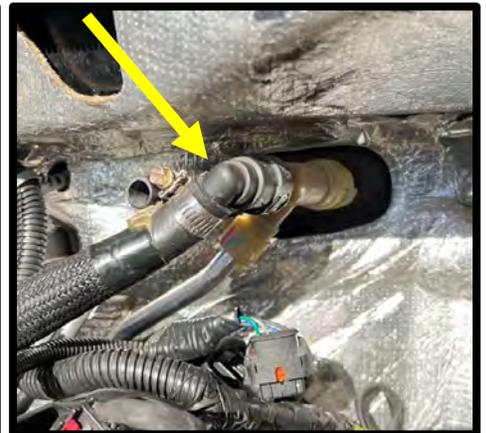
99. **(14-18 TRUCK ONLY)** Reinstall stock heater tube quick connect fittings.
