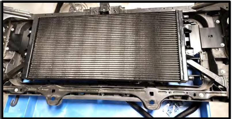
78. (TRUCK) Mock up the plastic radiator closeout. For top fitting, cut approximately a 2" square for hose clearance. For the bottom fitting, cut a 3" x 4" section away for hose clearance.
