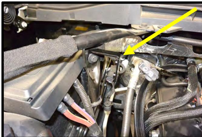
63. Install the IC filler reservoir to the bracket using the supplied (2) 6mm x 14mm HHFCS (10mm socket). **NOTE:** 3/8" barb should face forward.
