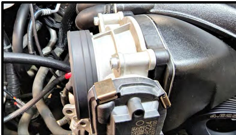
102. **(5.3L Only)** Install supplied rubber boot to throttle body flange.
