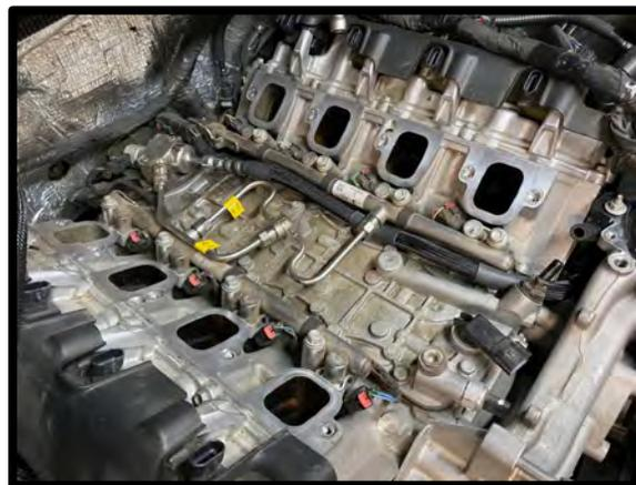
44. Install the supercharger assembly to the engine. You'll have to slide the last few inches as firewall clearance is minimal. Pay close attention to the orings, ensure they don't fall out or move. Do not tighten or secure at this time (must do after belt system is installed). NOTE: Be careful of PCV valve during installation.
