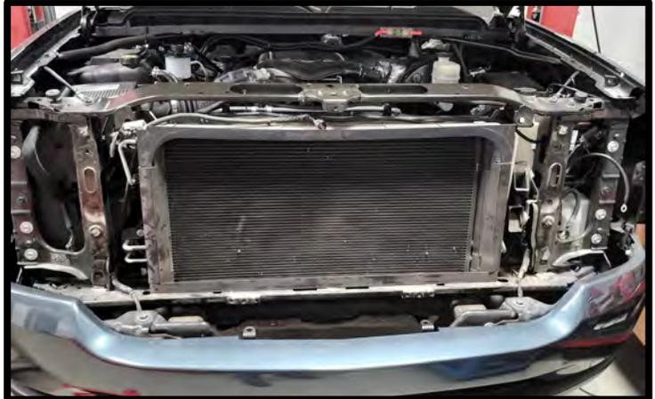
73. With the vehicle on a lift or jack stands, locate the (2) front frame support bolts (RH side of frame rail). Using a socket, loosen the 2 bolts. Install IC pump bracket over and behind stock bolts. Retorque to 22 ft-lbs.
