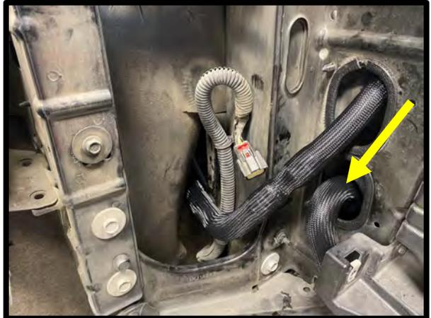
86. Install the preformed hose #3103256 from the LTR outlet (top fitting), under the airbox to the previously routed Y fitting feeding intercooler (rear fittings). Secure hose using supplied #16 pinch clamp. **NOTE:** Secure hose with zip ties for clean installation.
