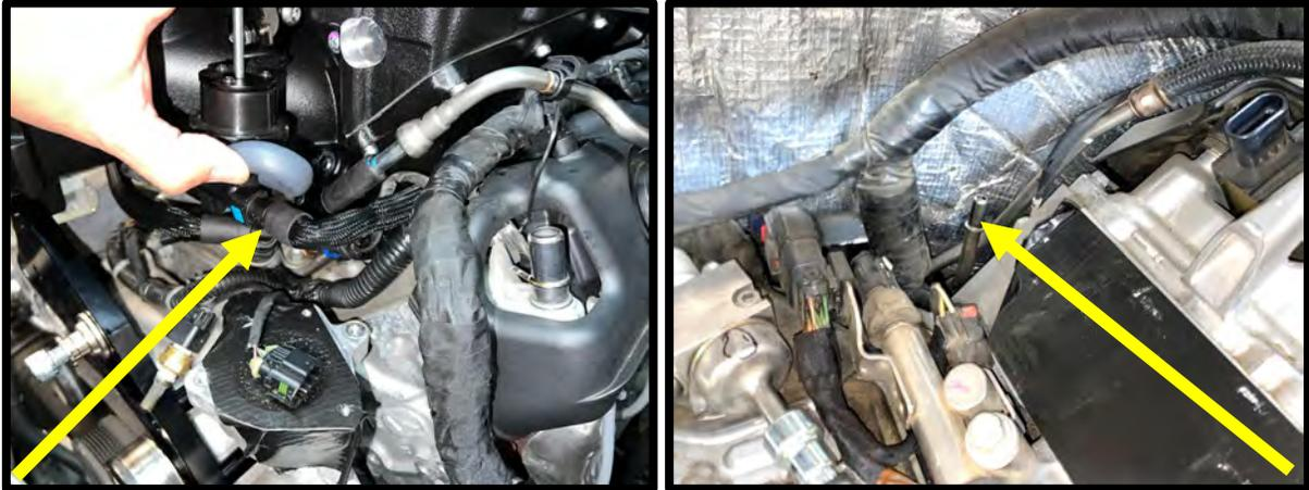
58. Install the supplied preformed IC inlet hose #3103144 to the LH rear fitting. Route around the back of the SC to RH side of engine. Install supplied Y fitting to end of this hose. Install supplied hose #3103145 to RH side, rear IC inlet fitting. Route other end to the Y fitting. Secure hose to the IC inlet fittings with supplied black 16mm-27mm black worm clamps. Secure other ends with supplied #16 pinch clamps. **NOTE: DO NOT MIX UP!**
