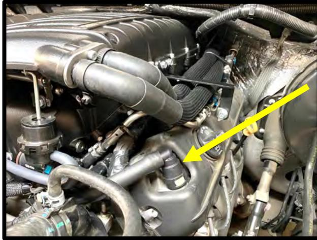
61. Reinstall stock coolant temperature sensor to factory location. Reinstall stock thermostat housing with stock oring and stock fasteners. Torque to 89 in-lbs. Reinstall degas bottle vent line to thermostat housing using stock clamp. Reinstall thermostat housing outlet hose to thermostat housing using stock clamp.
