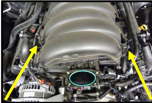
16. Remove the valve cover to air duct plastic vent tubes from valve covers by squeezing the connector and pulling up.
