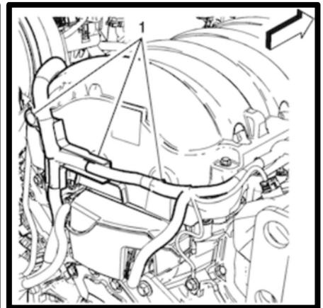
20. Clean the intake manifold surface using carb cleaner or other like chemicals. Cover intake ports with masking tape or duct tape. Remove the fuel pump foam insulator from valley of block.
