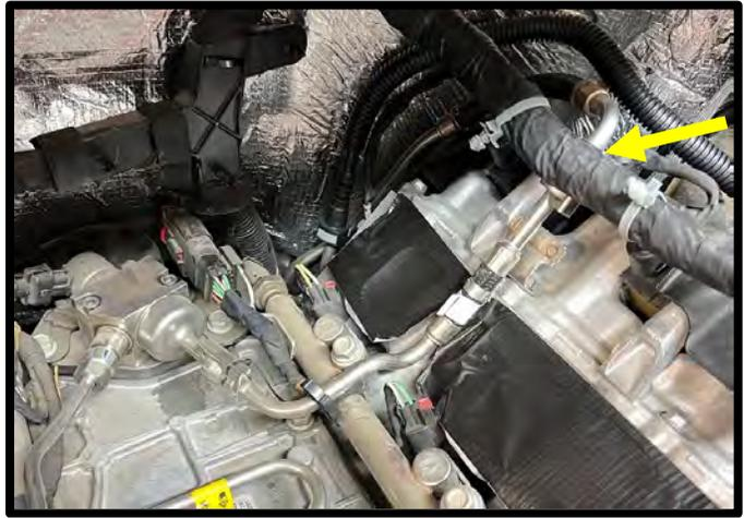
24. Using a 10mm socket, remove the stock bolt securing fuel line to motor. Disconnect the fuel feed pipe metal collar fittings from the fuel line. Remove DI pump feed hose. Reinstall stock bolt, torque to 108 in-lbs.
