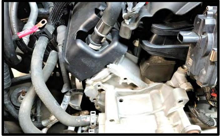
27. Disconnect coolant sensor 2-way connector. Remove vent line from thermostat housing by releasing pinch clamp. Remove thermostat housing outlet hose from thermostat housing by releasing pinch clamp. Remove coolant temp sensor temporarily.
