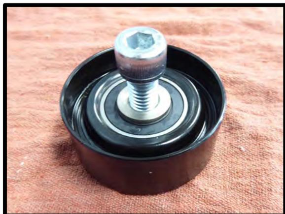
49. Install the supplied grooved idler pulley to the factory tapped hole below the alternator. Use the supplied step spacer with the 10mm ID hole and the 10mm ID step washer on the front of the pulley. Use the supplied 10mm x 35mm SHCS to secure pulley to factory bracket (8mm allen socket), use light amount of anti-seize. Torque to 28 ft-lbs.
