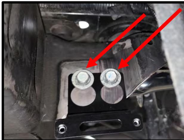
74. Install the supplied intercooler electric water pump to the supplied T-bolt clamp. Install pump and T-bolt clamp to supplied bracket using the (2) 6mm x 10mm HHFCS. NOTE: Cover open ports of IC pump to ensure debris can't contaminate pump.
