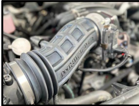
107. Route the throttle extension under the air inlet tube, connect to throttle body and stock connector. Secure harness in clips, away from the belt. **NOTE:** Support wires when pressing together on female extension to stock harness.
