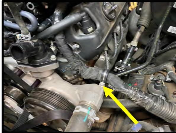
55. Install the stock jumper fuel line previously removed to the previously routed line under the SC. Press until they click and lock in place. Secure with secondary lock. **NOTE:** Leave other end loose until after intercooler hose routing.
