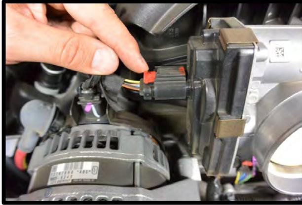
12. Disconnect the factory MAP sensor electrical connector by squeezing the connector and pulling away.
