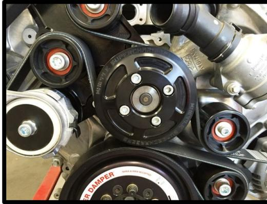
25. Install the supercharger pulley using the supplied 6mm SHCS using a 5mm allen socket. Leave hand tight until belt installation. Rotate each pulley by hand to verify each rotates freely.
